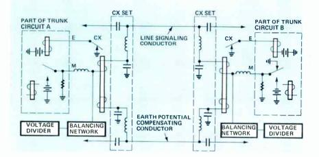
Figure 3. A composite signaling circuit with E&M lead control for one voice channel.
