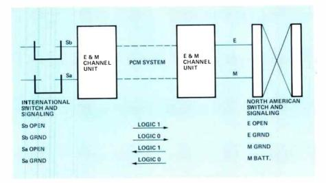
Figure 4. Block diagram of a North American switching and signaling system interfaced with an international type of system, both having E&M or equivalent leads.
