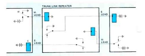
Figure 6. A typical trunk link repeater interconnecting two trunks which have incompatible E&M signaling interfaces.
