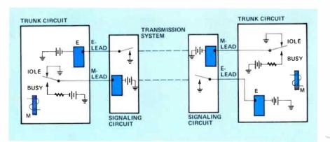
Figure 1. Traditional two-wire E&M interface (Type 1) designed for electromechanical switches. Current between switching and signaling equipment returns over a common ground.
