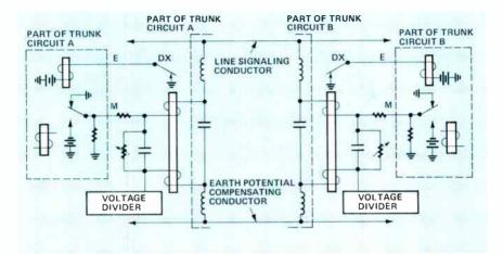
Figure 4. A duplex signaling circuit employing E&M lead control. The balanced circuitry provides self-compensation for ac and dc induced currents.
