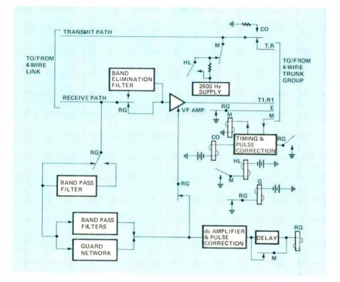
Figure 2. A typical SF signaling system using 2600 Hz as the signaling frequency. The primary function of the vf amplifier is to prevent noise or speech from interfering with the operation of the signal detector.
