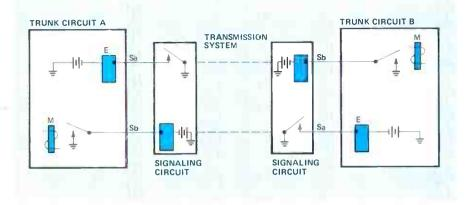
Figure 6. A representative international interface using F&M lead control. The Sa-Sb lead designations are typical of European products.
