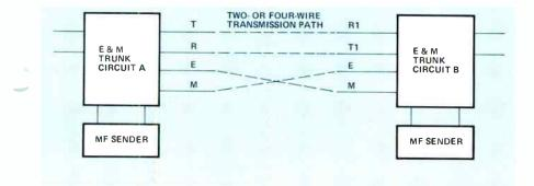
Figure 3. Block diagram of a multifrequency signaling system with E&M leads.
