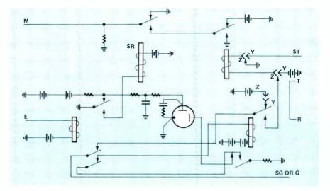
Figure 8. A typical ARI-type converter used with trunk circuits or signaling circuits equipped to receive 20-IIz signals.
