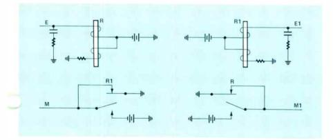
Figure 5. Pulse link repeater between two E&M interfaces of the same type.
