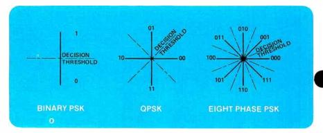
Figure 4. Relative phases and amplitude of PSK signals. The decision thresholds represent levels where the receiver must decide which signal has been received.
