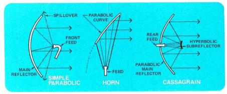
Figure 3. Three versions of the parabolic antenna, showing placement of rf feed and path of reflected energy. The Cassagrain is the most practical type for satellite communications.
