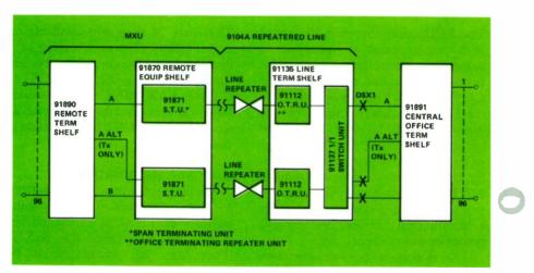
Figure 2. MXU/COT Pair Gain System (2:1 Concentration with Protection)
