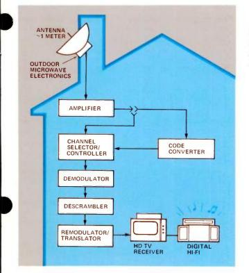
Figure 2. Direct Broadcast Satellite Home Receiver For High Definition TV.
