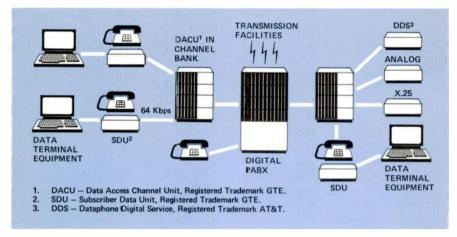
Figure 2. Star Topology — Second Generation PBX digital switching. Data is accommodated through data ports. Some intelligence is in the terminals.
