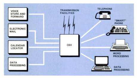
Figure 3. Star Topology — Third Generation PBX. The CBX functions primarily as a switch to connect the user with specialized processors as well as data processors. Speed, code and protocol conversions may also be provided depending on the computer's capacity. Some intelligence is in the terminals.
