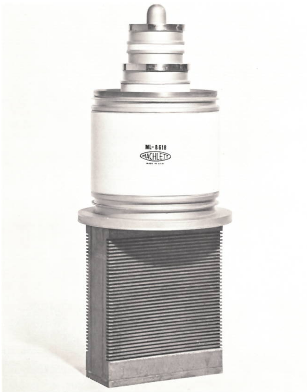
Figure 5 — Complete ML-8618 Showing Large Anode to Grid Seal Area.
