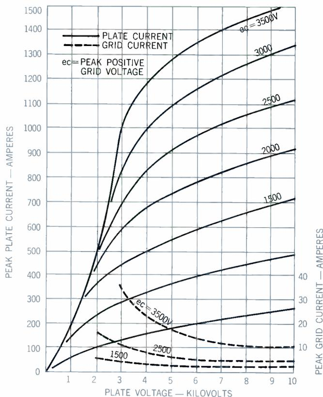
Figure 5 — ML-8549 Constant Grid Voltage Characteristics. (Tentative)
