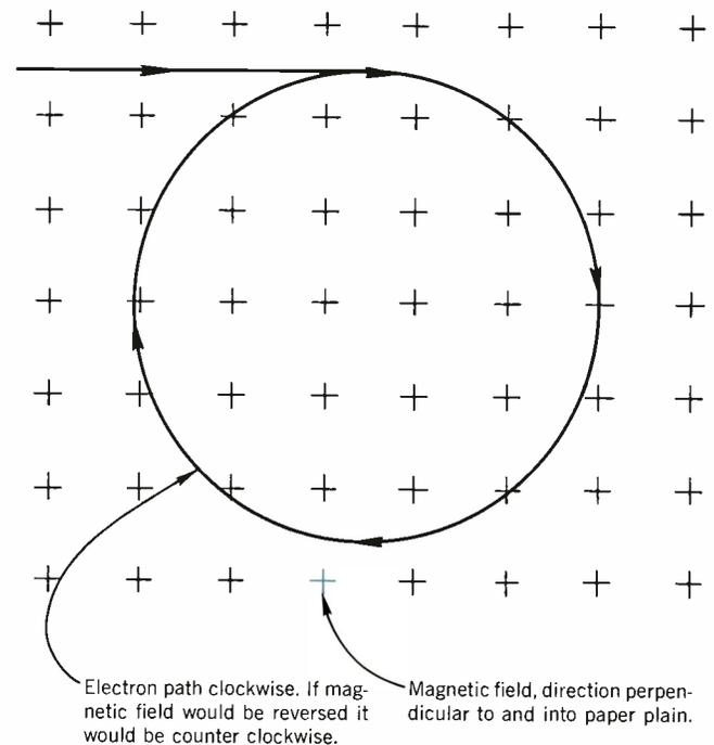
Figure 5A — Electron trajectories in a uniform magnetic field. Initial electron velocity is at right angle to magnetic field.
