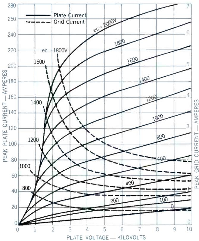
Figure 7 — Constant grid current characteristics of the ML-LPT14 with magnet of about 700 Gauss.
