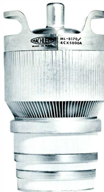
Figure 6 — Completed ML-8170/4CX5000A.
