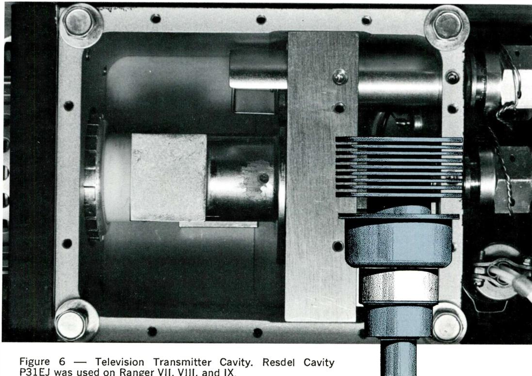
Figure 6 — Television Transmitter Cavity. Resdel Cavity P31EJ was used on Ranger VII, VIII, and IX. (Photograph courtesy of Jet Propulsion Laboratory.)
