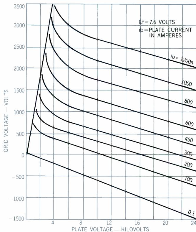
Figure 6 — ML-8549 Constant Plate Current Characteristics. (Tentative)
