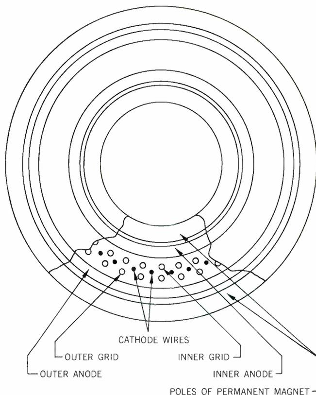
Figure 1 — Schematic of Magnetically Beamed Triode.
