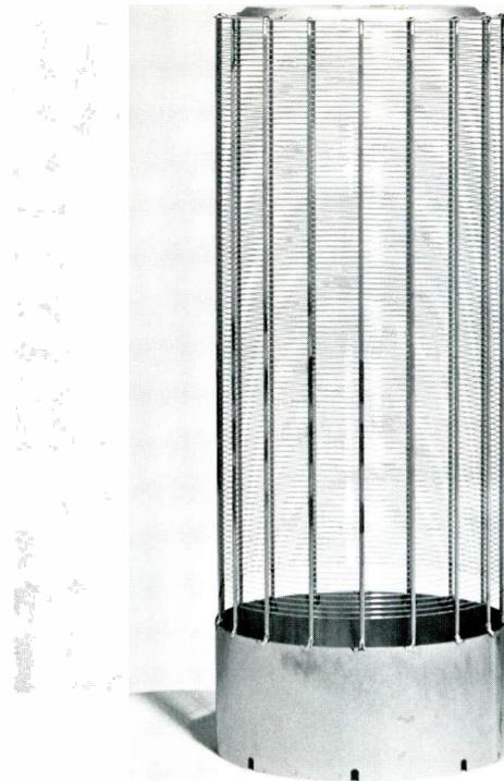
Figure 2B — Screen grid with heavier helix but with pitch same as Control Grid.
