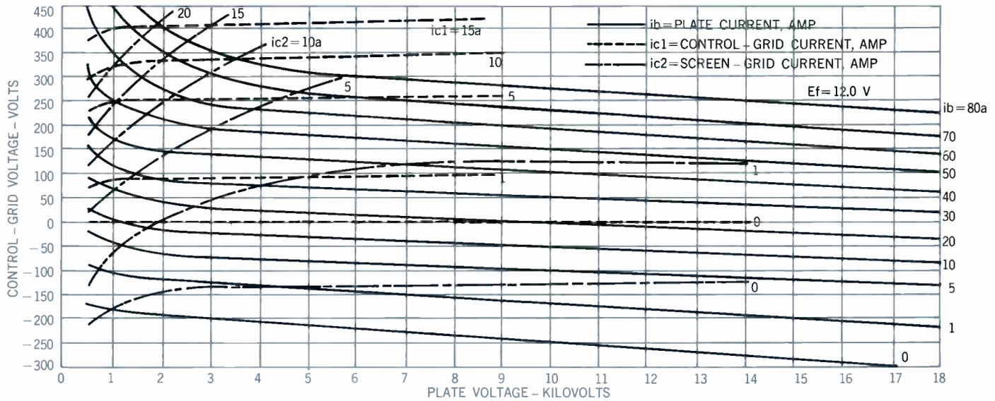
Figure 6 — Constant Current Characteristics showing screen-grid potential at 750 volts.
