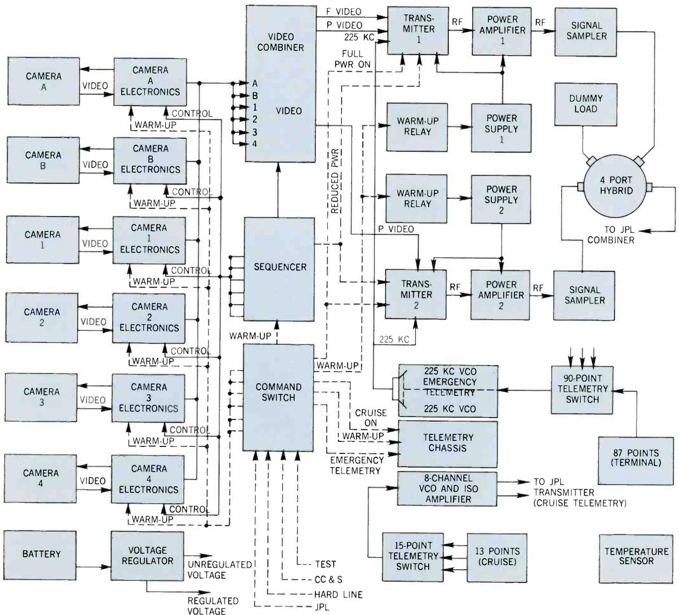
curacy and linearity, modulates the 225 kc oscillator, the signal from which is combined with the video of the modulator input. The 225 kc base band thus achieved is transmitted using the 19 db gain of the directional antenna.
