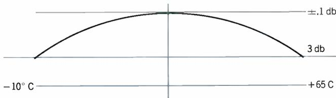
Figure 11 — Quad cavity power output over  $80^{\circ}\text{C}$  range, from  $-10^{\circ}\text{C}$  to  $+65^{\circ}\text{C}$ .
