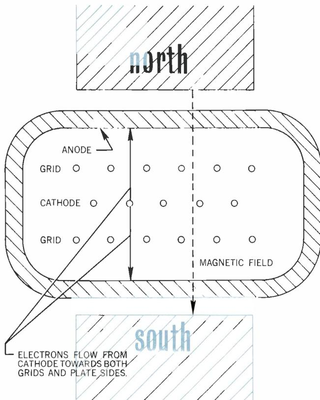
Figure 1 — Schematic Cross Section through Magnetically Beamed Tube.
