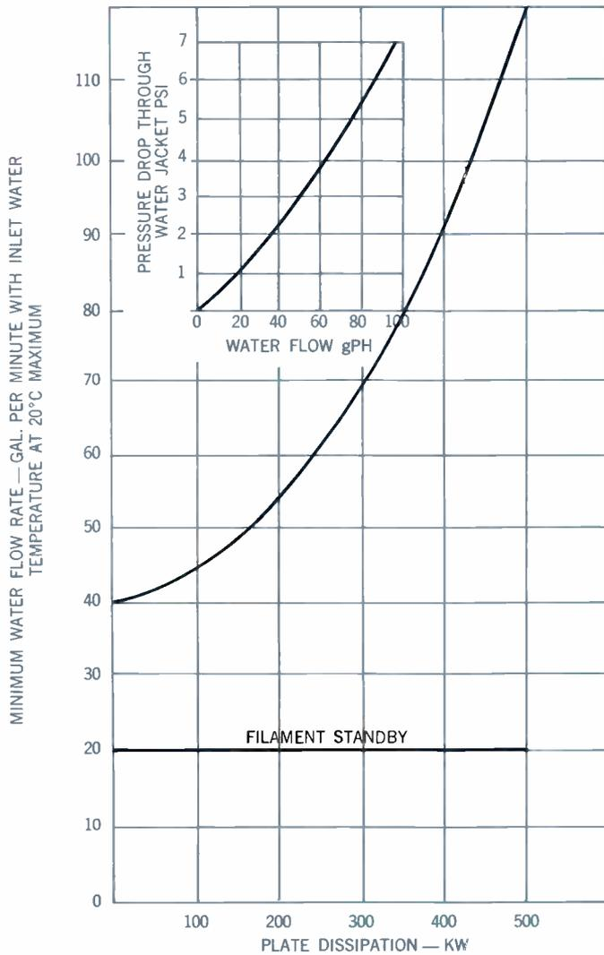
Figure 8 — ML-8549 Anode-Water Cooling Characteristics.
