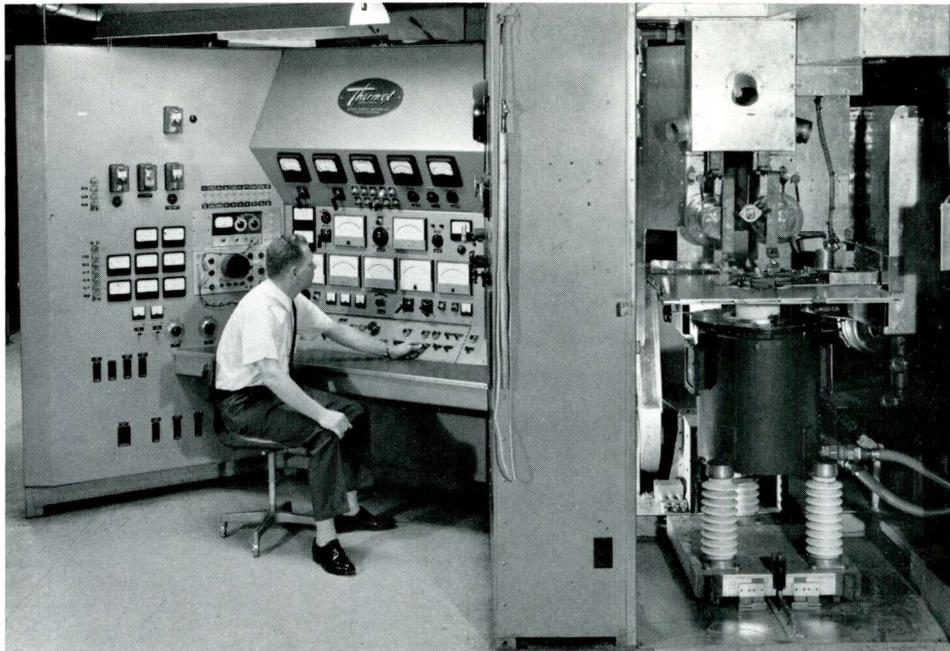
Figure 5 — ML-8545 is shown in the Machlett 1.2 Mw Test Set. Screen anode insulator is just visible above the Vapor-Jacket Condenser Cooling Unit. For pictorial purposes, here, the interlock door to test chamber has been left open.
