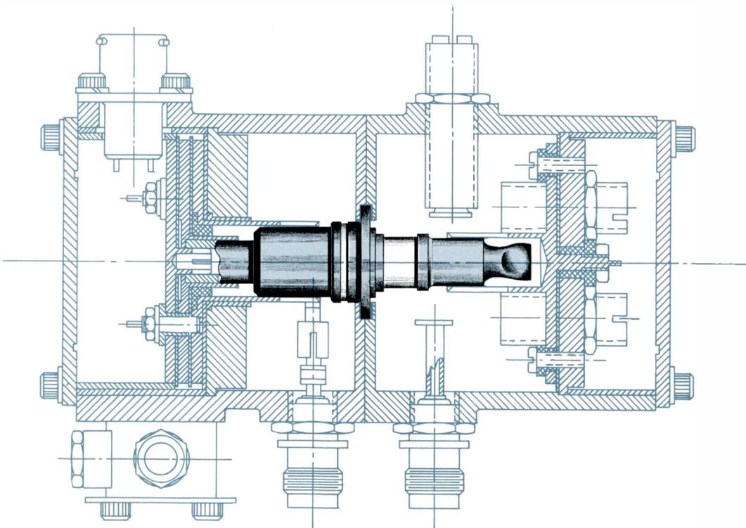
a Phormat cathode — provided a high margin voltage stability, Phormat cathodes having operated satisfactorily without arcing at voltages which destroy conventional cathodes.) The second of the two figures, Figure 7B plots the actual amplifier response operated for Ranger IX. These response curves show how well the predicted and the actual
