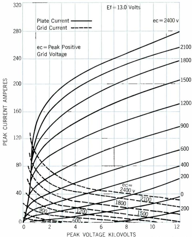
Figure 10 — Constant grid voltage characteristics for the ML-6696.
