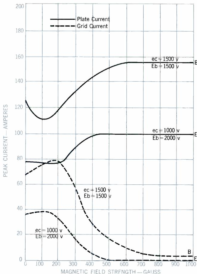
Figure 9 — ML-LPT14 plate and grid currents vs. different magnetic field strength.
