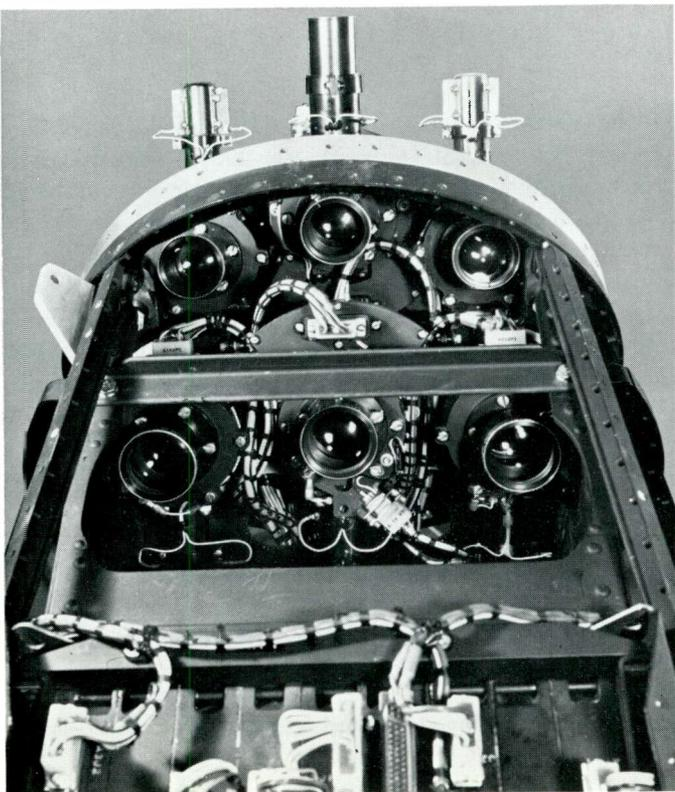
Figure 2 — Ranger IX television payload, showing camera aperture. Omnidirectional antenna is at the top of the structure. (Photograph courtesy of Jet Propulsion Laboratory)
