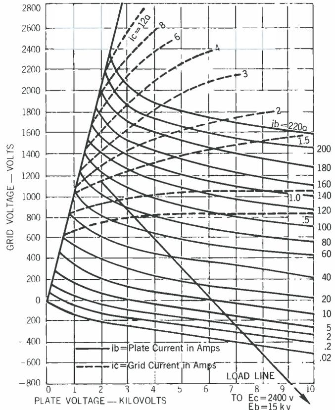
Figure 11 — Constant current characteristics for the ML-LPT14.
