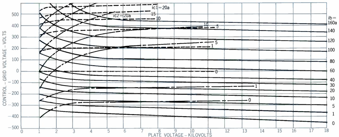
Figure 7 — Constant Current Characteristics showing screen-grid potential at 1500 volts.
