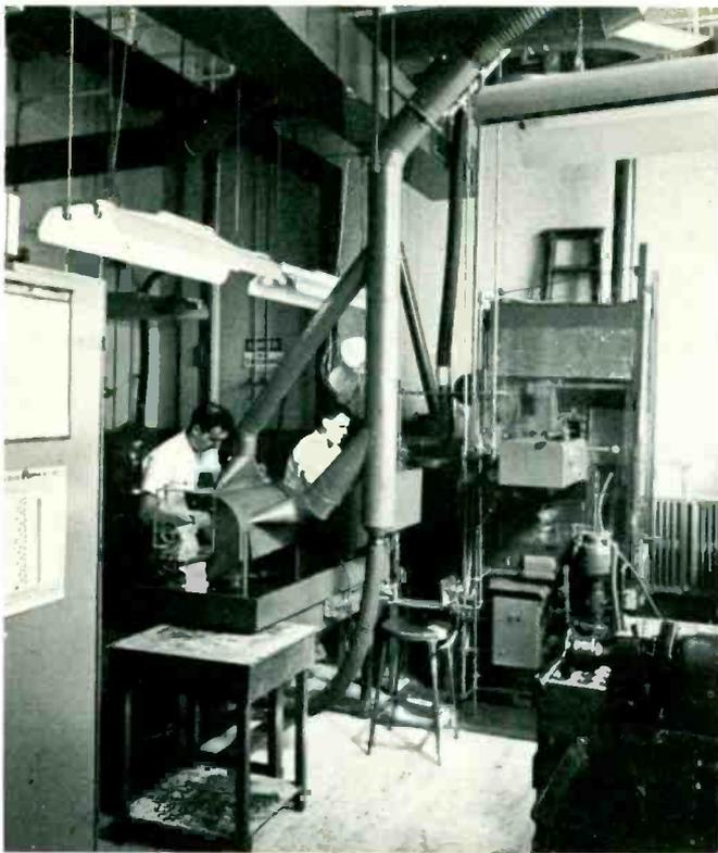
In modern beryllium processing every operation is surrounded with every possible safeguard. Here in this closed, air conditioned room, special suction tubes, like giant vacuum cleaners, draw every particle of dust away from every point where the metal is worked.
