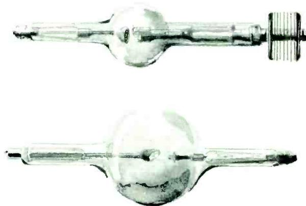
Coolidge tubes handled by Machlett as distributor about the time of World War I. Upper, a diagnostic tube "recommended for fluoroscopy and radiography only. It should never be used for therapy." Lower, "For treatment and general picture work."
