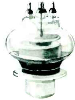
The ML 880 tube was made during the war at Norwalk for the armed forces which used it as a transmitter tube for overseas radio communications and for high power radar jamming. Later it became the cornerstone in the development of Machlett's power tube line—the first high-power radio transmitting tube to bear the Machlett name.
