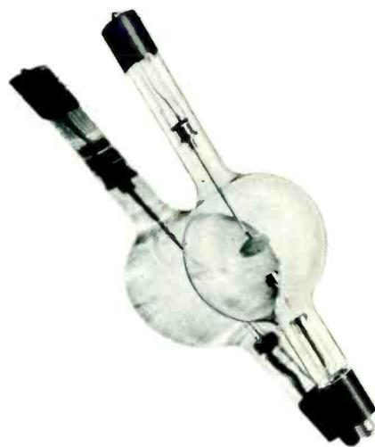
A therapy x-ray tube of the Coolidge type made by Machlett in the early 1930's. Note the light target, supported on a slender stem. Heavy copper anodes were yet to come.
