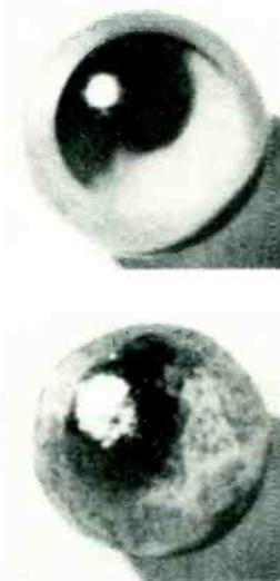
Above: a steel ball bearing silver coated by the process worked out by Machlett, after 500 hours of continuous operation at intense heat in high vacuum shows no sign of wear or of breakdown in the lubricating coat of silver. Below: an uncoated steel ball bearing after the same test shows serious deterioration.
