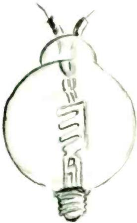
The original DeForest audion tube, forerunner of today's radio tubes. Machlett made experimental tubes of this general type and shape for DeForest. (Adapted from Encyclopedia Britannica illustration.)
