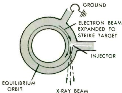
Schematic diagram of the Betatron. The upper diagram, shows the Donut, in cross section, between the upper and lower halves of the transformer. Below, a simplified plan of the Donut itself shows the circular path in which electrons are whirled to accelerated speed, and the track they follow when released, to strike the target and produce x-rays.
