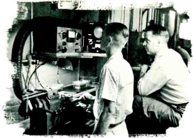
An unusual piece of equipment, delicate and precise far beyond the ordinary, insures parallelism of electrodes in an assembly destined for a high-vacuum triode.
