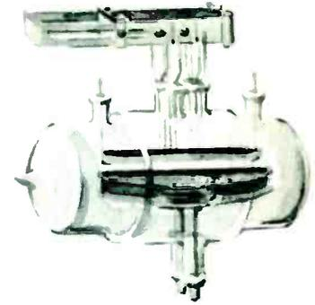
The VT 158 tube, made to Signal Corps designs as a compact, light source of UHF energy for a portable radar system was a complex assembly in a glass envelope of unusual shape. Yet Machlett Laboratories trained people, previously untrained in assembly or in glass-blowing, to make this difficult tube in large quantities.
