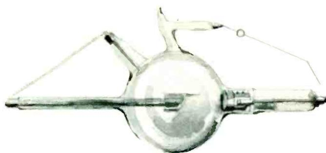
The Bellevue tube for interrupterless transformer current in the form made by Machlett from about 1912—the small spear-point projecting from the face of the anode produced, in some degree, the effect of a valve or rectifier, to suppress some of the inverse impulses necessarily inherent in the alternating current then necessary to produce high voltages in x-ray equipment.
