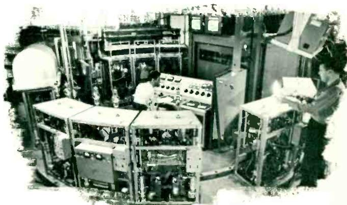
Newest version of the mobile exhaust system is an endless-track circuit. Tubes being sealed into pump-bearing dollies at right, progress through outgassing stages accurately controlled from the instrument board at center.
