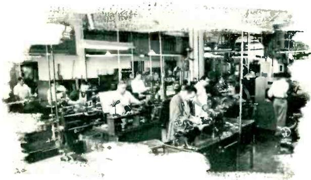
In the Model Shop expert machinists and glass workers fabricate pre-production tube components.
