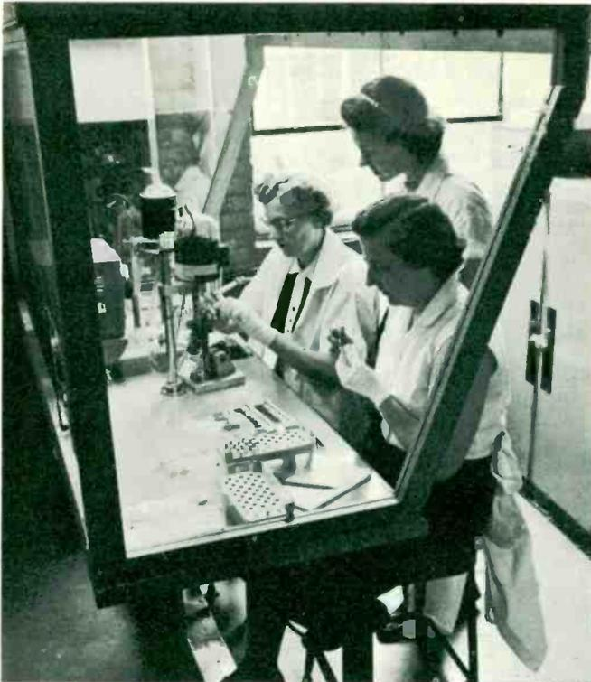
In this typical air-conditioned area, precision parts for the 2C39A tube are assembled to very close tolerances.
