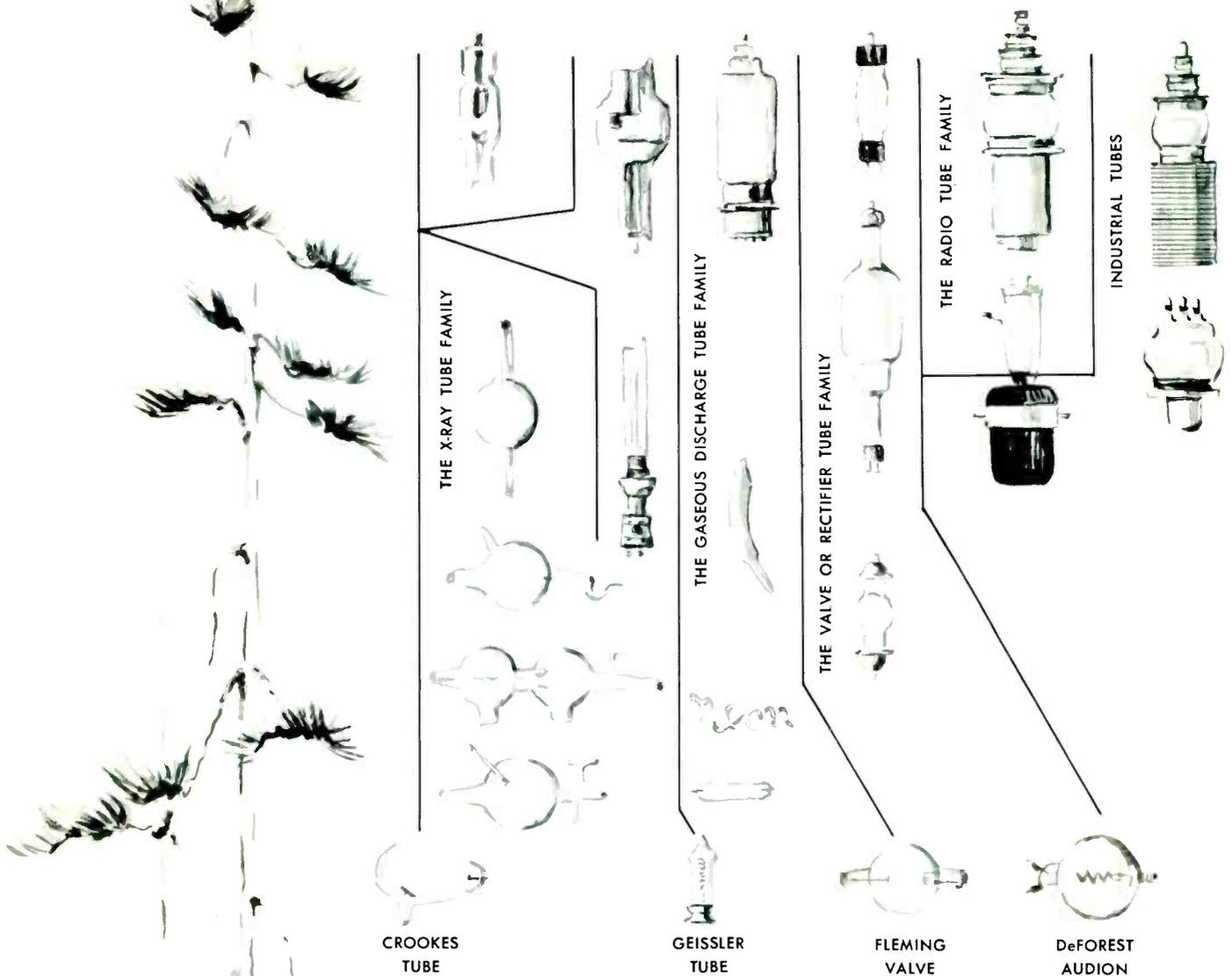
FOUR TUBES DEVELOPED FROM 1897 - 1905 FORMED THE BASIS OF FOUR FAMILIES OF TUBES.
