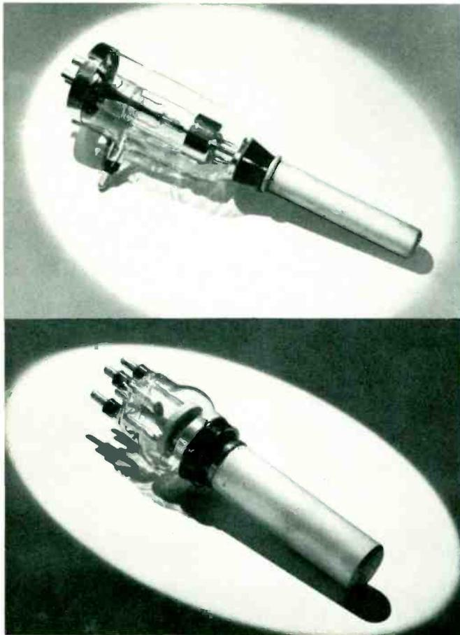
The redesign of a tube of conventional broadcast transmitter type (upper) into a rugged form (lower) which is not only suitable for gruelling industrial applications, but at the same time better for broadcast use. Its basic electronic characteristics remain the same.
