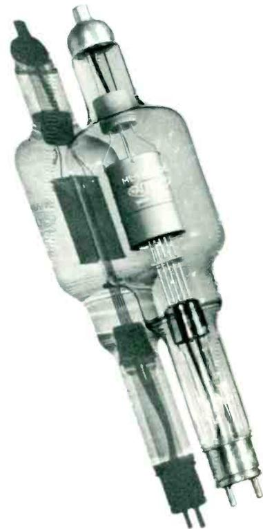
A modern, high-power rectifier tube, typical of those used in many industrial installations.
