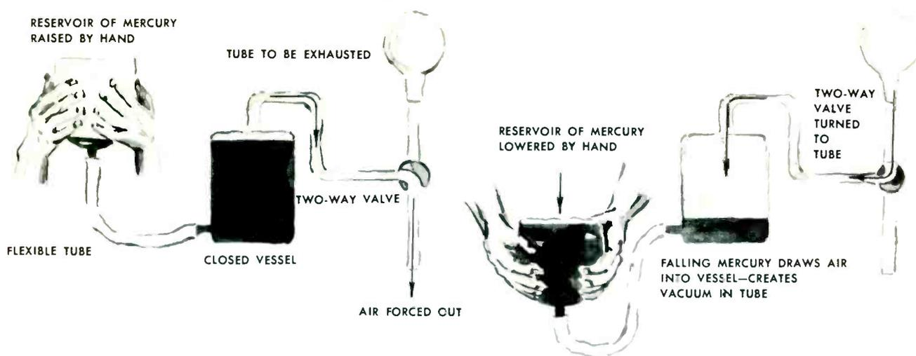
It took a strong man to operate the Geissler mercury vacuum pump, here shown in schematic diagram.
