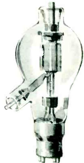
The 6C21 pulse modulator tube, heart of the transmitter in early-warning and gun-laying radar systems, was Machlett's first big assignment in defense production work.
