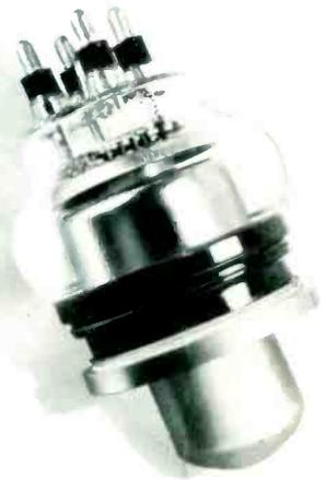
The well-known and widely used type 880 tube (sketched above) was "ruggedized" by repeated small but effective changes in design and construction, into the type 5658—a tube which replaces the 880 in existing equipment and gives superior performance.
