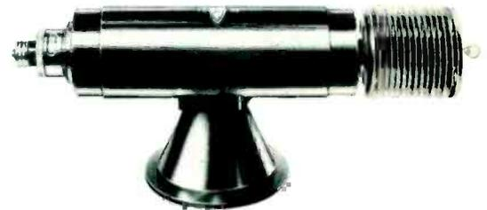
Machlett's CYR tube of 1934 was the first ray-proof x-ray tube, compact and light for easy positioning. It achieved these advantages by using what has since become widely known as "geometry of design"—a hallmark of Machlett engineering.
