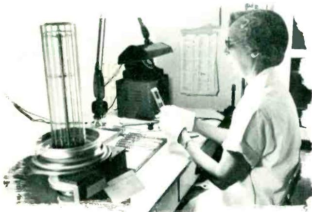
It takes a special gift for care and unfailing accuracy, to inspect electrodes for any kind of Machlett tube, prior to sealing-in.
