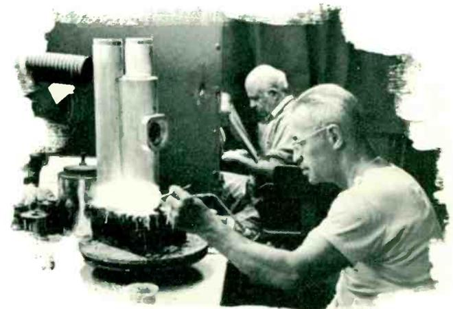
In the fabrication of aluminum housings for high-voltage x-ray tubes, shown here, operators take unremitting care to achieve an absolutely sound bond between aluminum components and shockproof housings.
