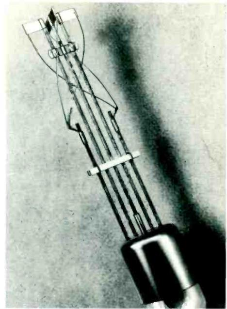
The catenary type of filament developed at Machlett for low voltage drop and greater structural rigidity under the severest operating conditions.
