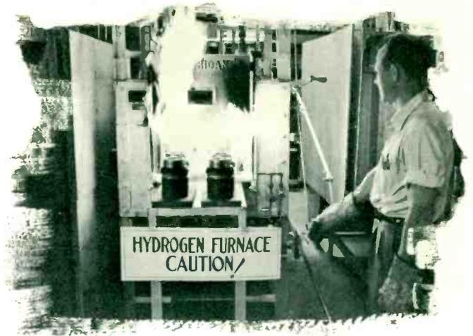
Metal parts are brazed in the intense heat of hydrogen flames.
