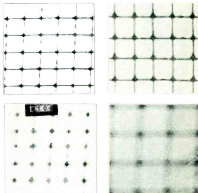
Machlett's screen test. The image of a half-inch square of wire screen, 8 inches above the plate and 16 inches below the tube, demonstrated (upper two views) the sharp image produced by the Bellevue tube, as compared with the fuzzy images produced by tubes with more widely diffused target spots.
