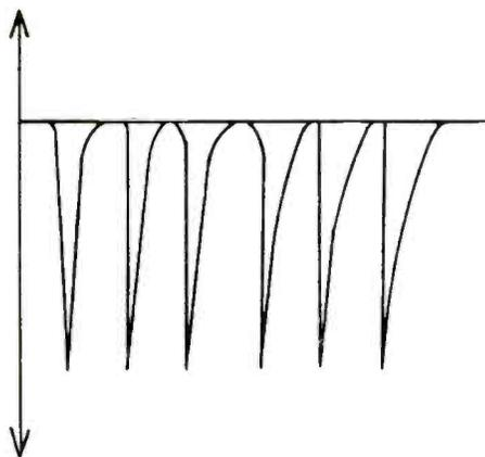
Effect of valve tubes on Ruhmkorff coil current.
