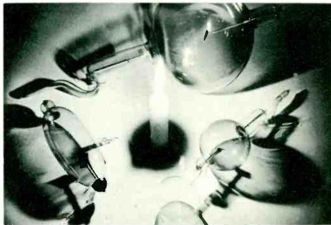
Early Machlett tubes—of the Jackson type. The anode is directly in line with the cathode and bears a target set to receive the full stream of electrons and angled to direct the shower of x-rays to one side. Other protuberances from the tube are incidental to creating or maintaining a vacuum.
