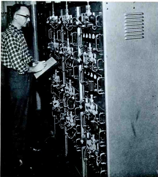
Figure 1 — Multiple unit life test equipment for ML-6442; contains plate pulse cavity oscillators. Test parameters: Pulsed Oscillation F = 3450 mc minimum;  $e_{py} = 3000$  v;  $R_g/1b = 2.5$  mode;  $tpv = 1.0$  usec  $\pm 10\%$ ;  $trv = 0.1$  usec., maximum;  $tfr = 0.2$  usec, maximum;  $pr\Omega/Du = 0.001 \pm 5\%$ ;  $E_r = 6.0$  V.
