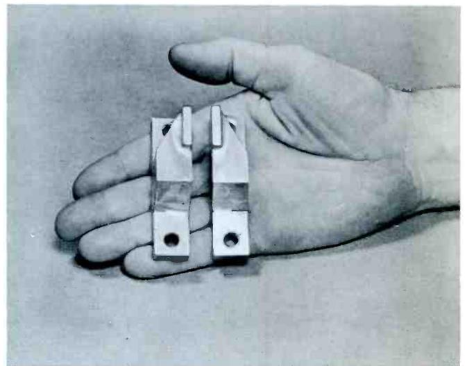
Figure 6 — High frequency resistance welding contacts.
