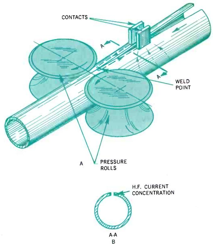
Figure 3 — High frequency resistance tube welding.
