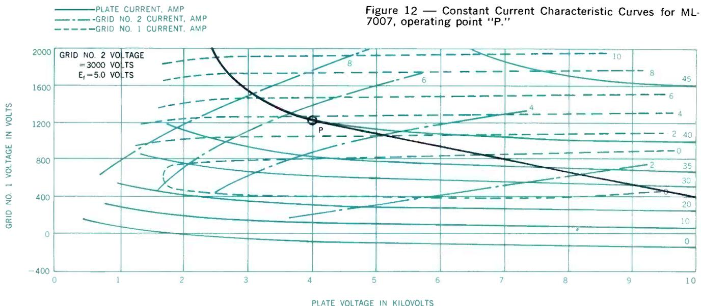
Figure 12 — Constant Current Characteristic Curves for ML-7007, operating point "P."
