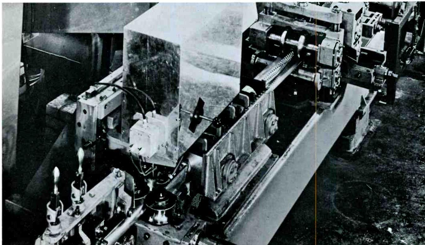
Figure 4 — High frequency cable sheathing mill.
