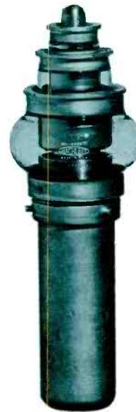
Operating conditions of final amplifier tubes of the Thermatool induction heaters, VT-60 (1 — ML-6696) and VT-140 (2 — ML-6696's), employed for high frequency resistance welding:
