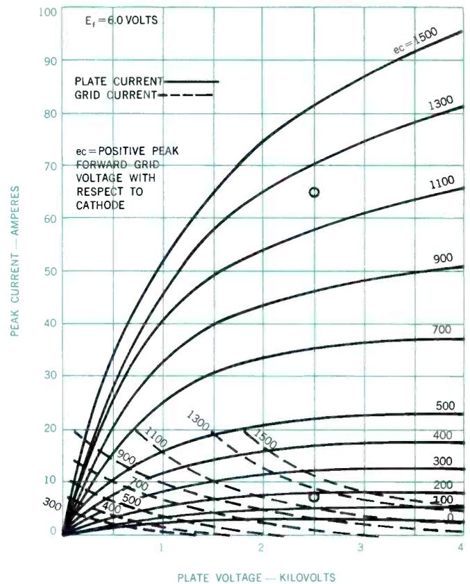
Figure 10 — Constant Grid Voltage Characteristic Curves of ML-6544.
