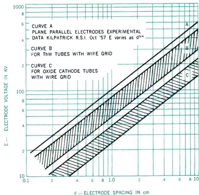
Figure 3 — Anode Voltage Rating versus Outer Grid to Anode Spacing.
