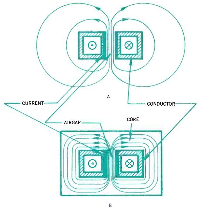
Figure 2 — Proximity effect in go and return circuit.
