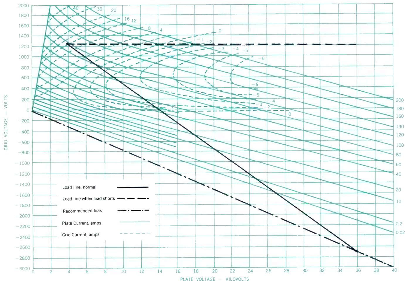
grid drive lines represented by A, B, C, etc., do not all follow down the diode line given by  $i_p = \sigma e_p$  and curves A, B, C . . . are more or less rounded off as they approach the limit line on minimum plate current. Nevertheless, these curves can be used to determine with fair accuracy the effects of variations in grid drive, screen grid voltage and plate voltage, provided the changes are small.
