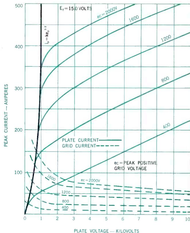
Figure 8 — Constant Grid Voltage Characteristic Curves of ML-8547, showing effect of reduced grid anode spacing on the Diode Curve  $i_b = i_k^{3/2}$ .
