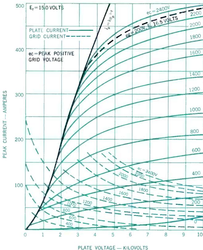
Figure 7 — Constant Grid Voltage Characteristic Curves of ML-7560 showing End-of-Load Line Point and Diode Curve  $i_b = i_k^{3/2}$ .
