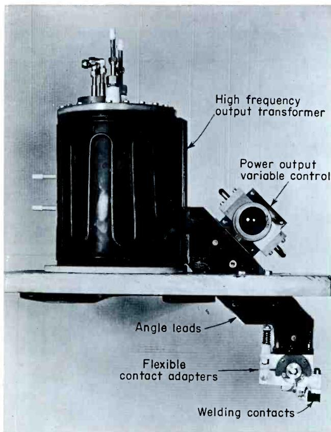
Figure 5 — Welding head.
