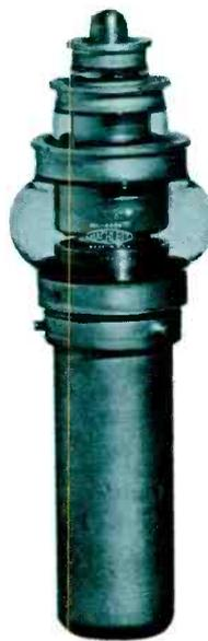
Operating conditions of final amplifier tubes of the Thermatool induction heaters, VT-60 (1 — ML-6696) and VT-140 (2 — ML-6696's), employed for high frequency resistance welding:
