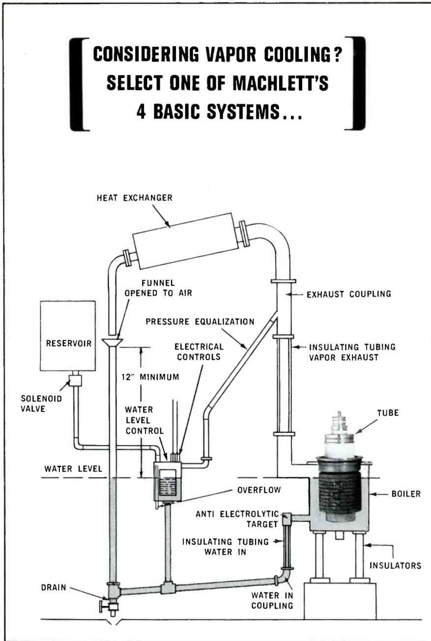
**From 50kW to 500kW, Machlett offers four basic Vapor Cooling Systems for cooling high power electron tubes:**
