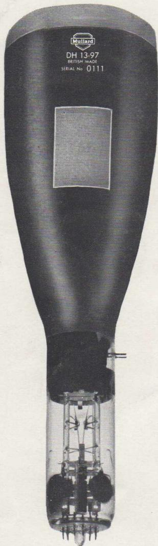
The most interesting feature of this five-inch tube is its use of graded post-deflection acceleration. Two successive bands (a4 & a5) are used giving a high ratio between the voltage on the final gun anode and the final acceleration voltage.
