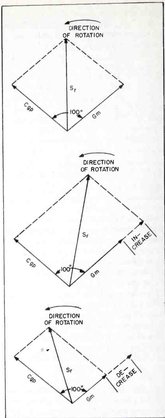
Figure 3. Vector Diagram Showing Effect of Modulation
