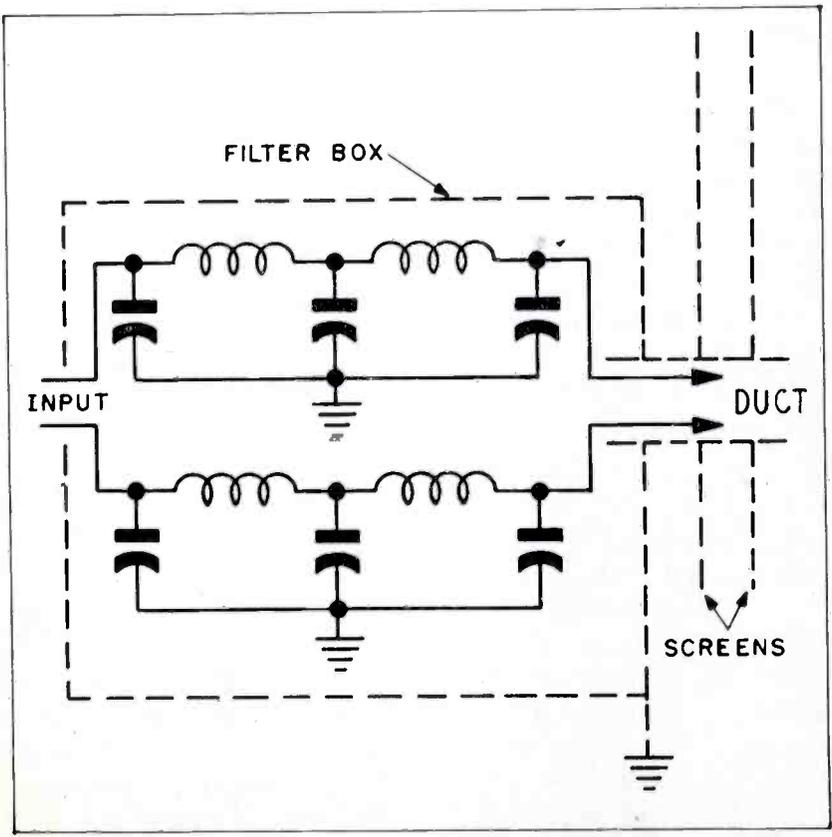
Figure 4. Typical Power-Line Filter
