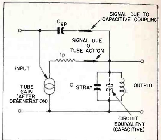
Figure 2. Equivalent Circuit of Phase Modulator
