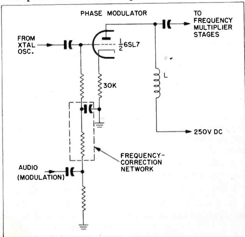
Figure 1. Schematic Diagram of Phase Modulator
