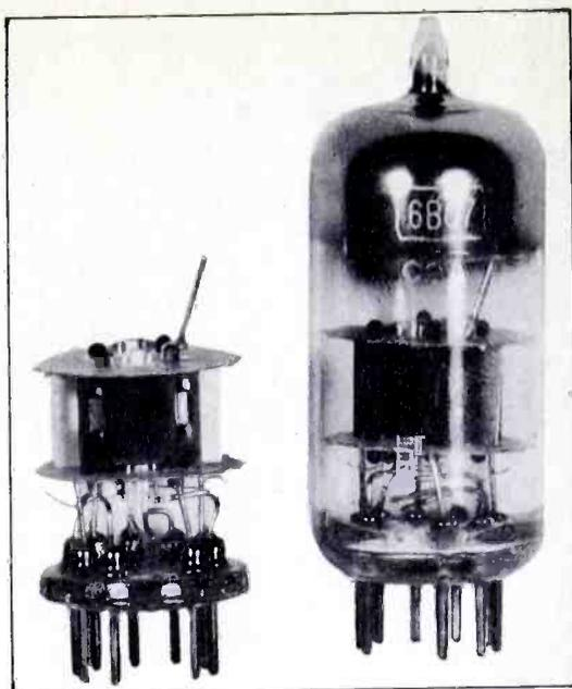
Figure 10. Left—An Assembled 6BQ7 Tube (less getter assembly), Prior to Insertion into Envelope
