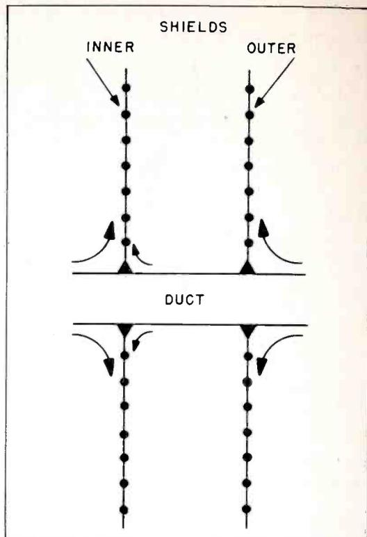
Figure 5. Paths Taken by Interference When Duct for Power Line is Soldered to Both Shields
