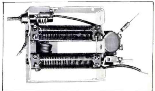
**Figure 4. Tapered-Line Input Section**
