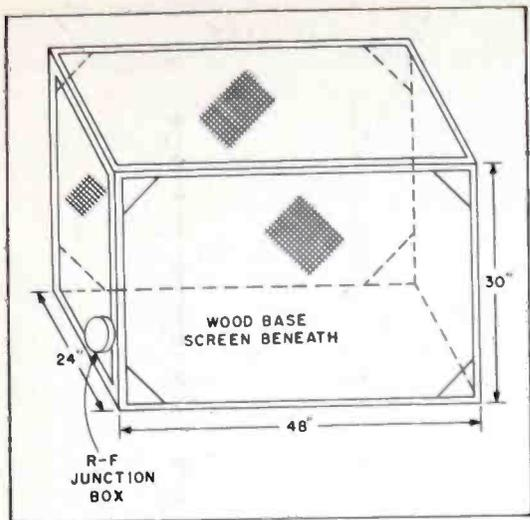
Figure 6. Poor Man's Screen Room
