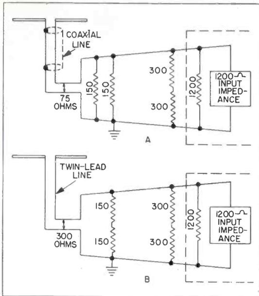
**Figure 3. Simplified Diagram of Tapered-Line Input Section**
