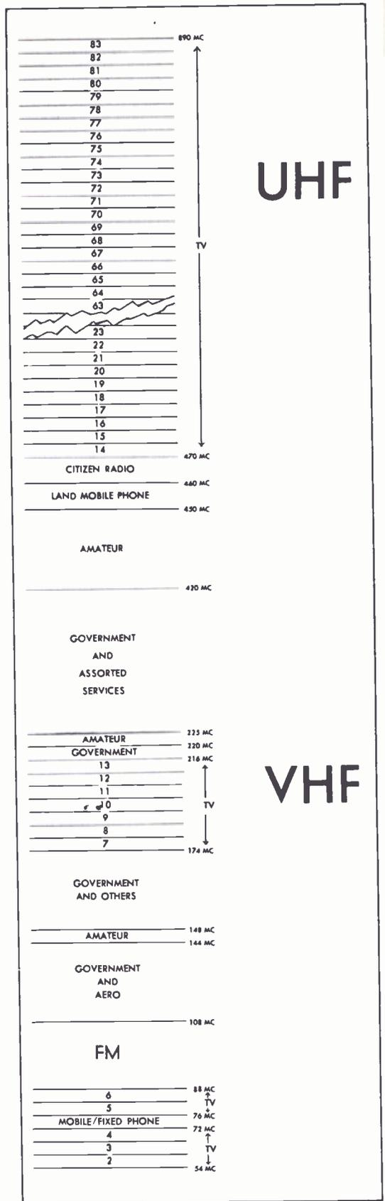
Figure 1. TV-Channel Frequency Allocations
