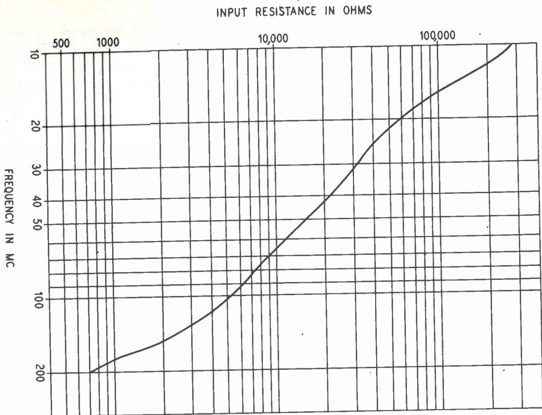
Figure 5. Input Resistance of a 6AG5 at Various Frequencies
