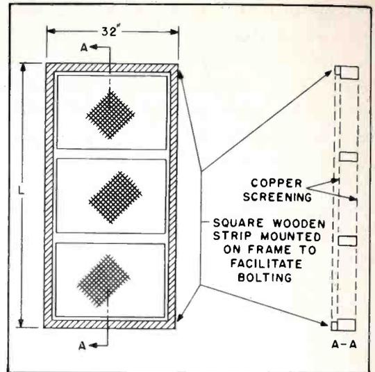
Figure 3. Construction of a Typical Cell
