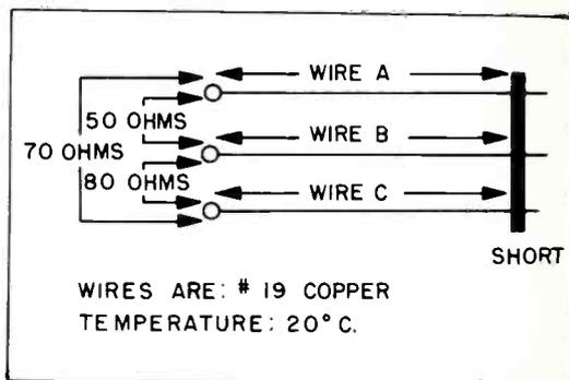
*Wire-to-Wire Resistance Measured on Shorted Three-Wire Circuit*
