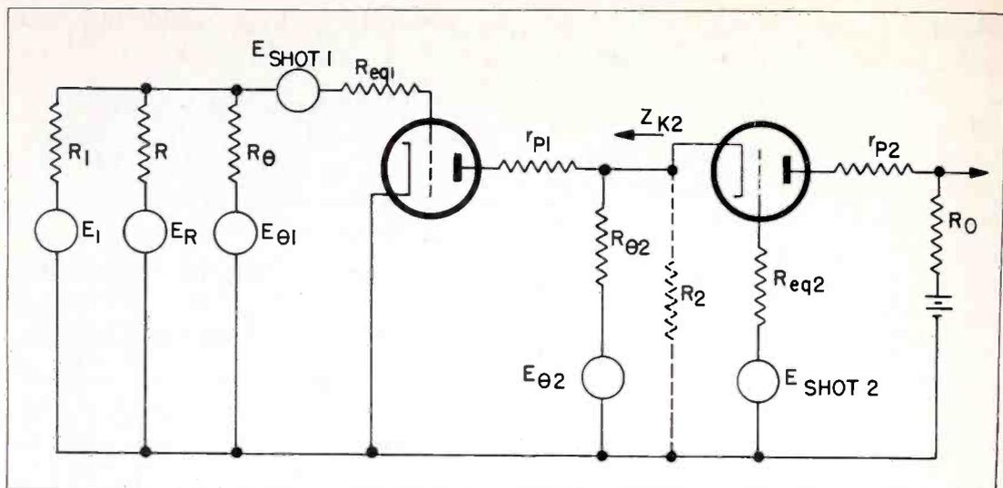
Figure 8. Noise Sources in a Modified Cascode Amplifier
