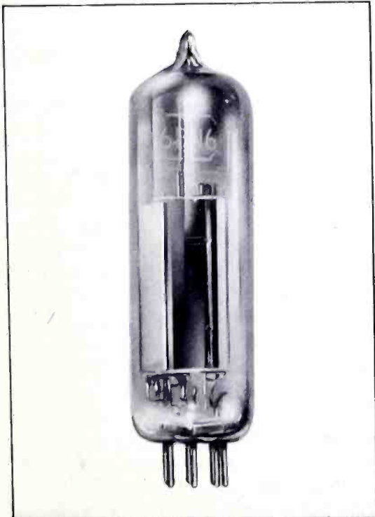
Figure 6. Type 6BN6 Gated-Beam Tube
