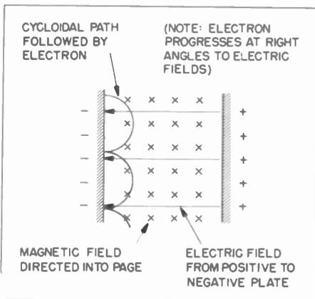
**Figure 5. Motion of an Electron in Combined Electric and Magnetic Fields**
