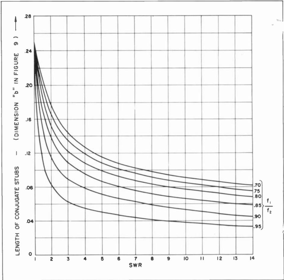
Figure 11. Chart for Determining Length of Conjugate Stubs (See figure 9.)
