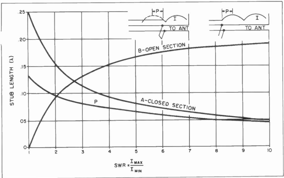
Figure 8. Chart for Determining Length and Position of Stub When SWR is Known
