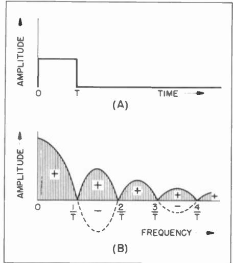
Figure 24. Graph of D-C Pulse with Corresponding Frequency Spectrum
