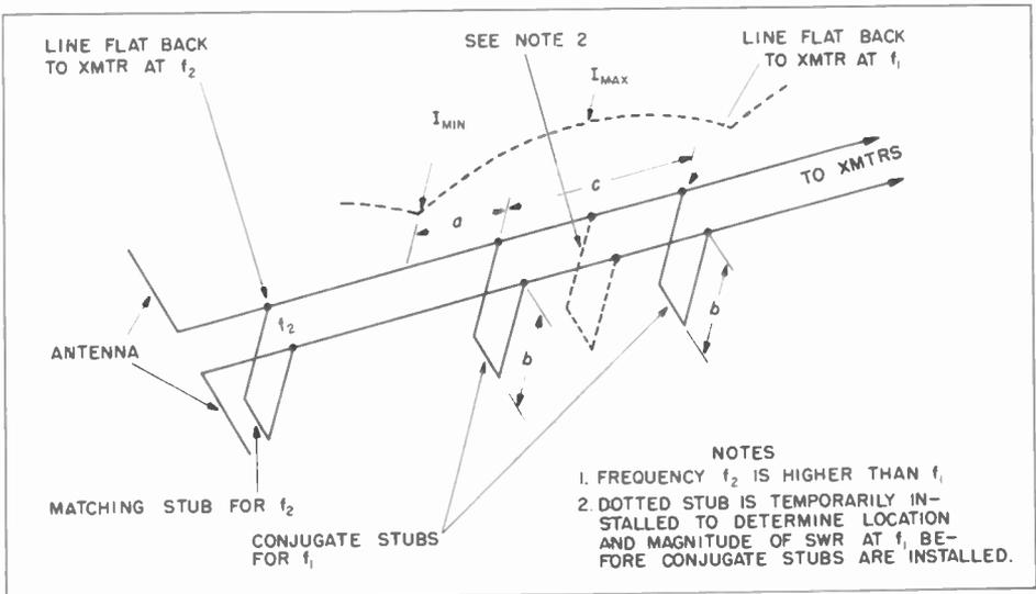
Figure 9. Sketch of System for Matching Antenna to Transmission Line at Two Frequencies (A simple, closed stub is used to flatten the line at highest frequency,  $f_1$ , and a pair of conjugate stubs to flatten the line at lowest frequency,  $f_2$ , without affecting the line at  $f_1$ . See figures 10, 11, and 12 for dimensions a, b, and c.)
