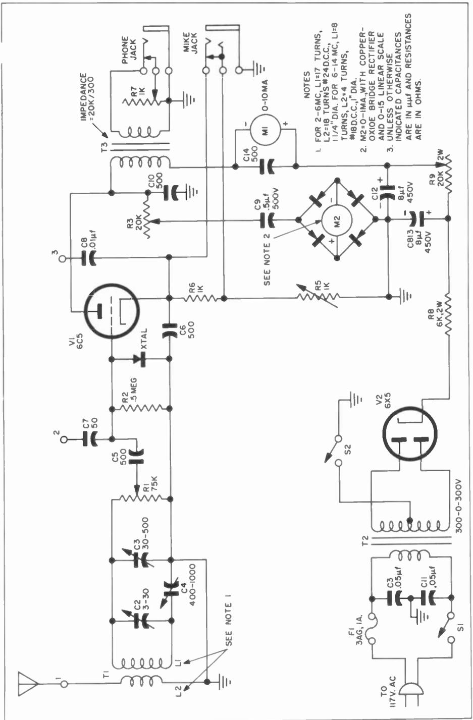
**Figure 2. Schematic Diagram of Transmitter Monitor (The numbers of turns indicated for L<sub>1</sub> are approximate. It is suggested that L<sub>1</sub> be wound with 20% additional turns, and then trimmed as necessary.)**
