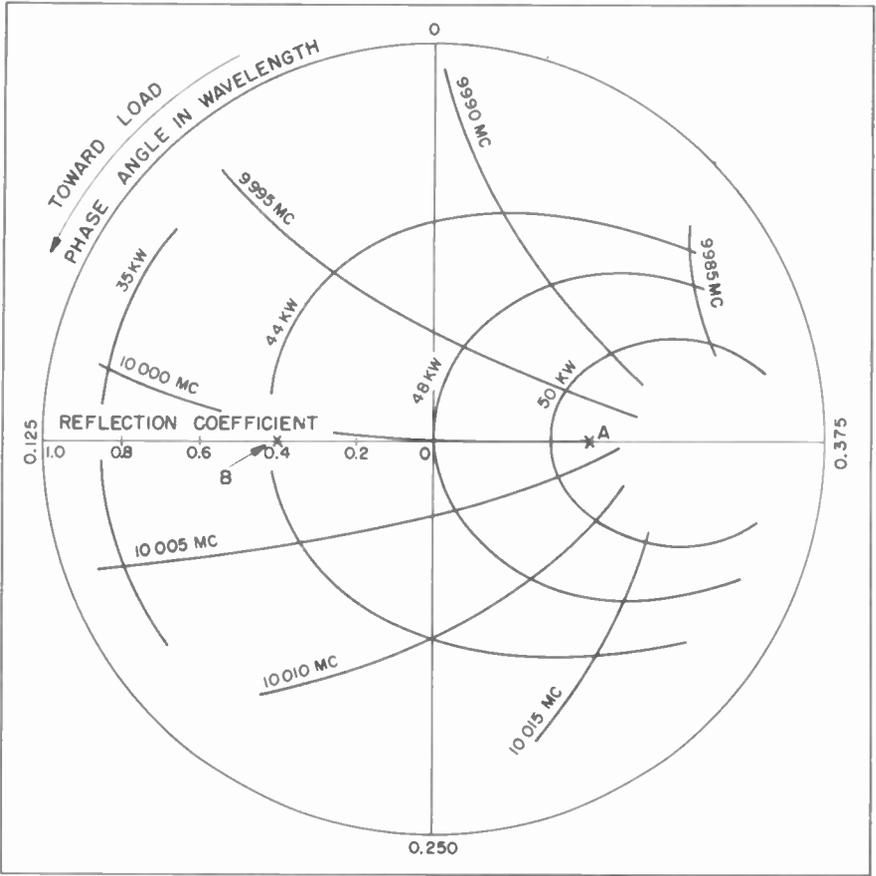
Figure 21. Typical Magnetron Rieke Diagram
