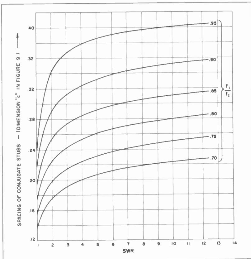
Figure 12. Chart for Determining Spacing between Conjugate Stubs (See figure 9.)
