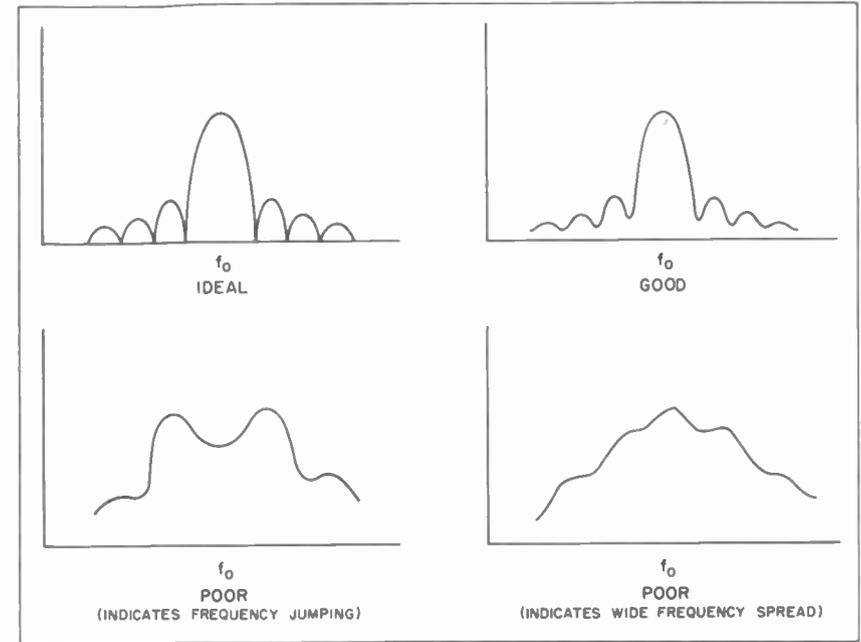
Figure 27. Typical Spectra of R-F Pulse
