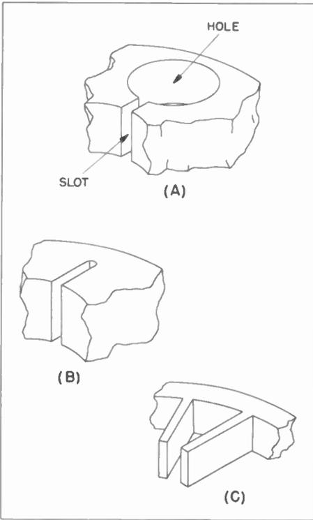
**Figure 6. Various Magnetron Cavity Types**
