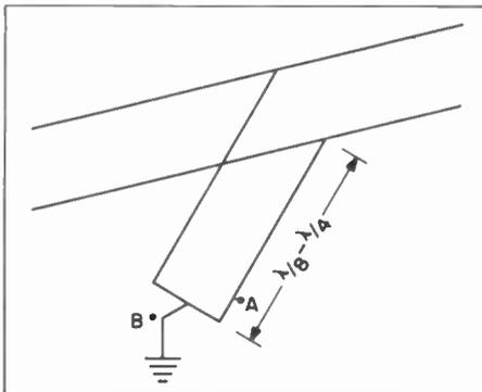
Figure 7. Temporary Building-Out Section (Stub)
