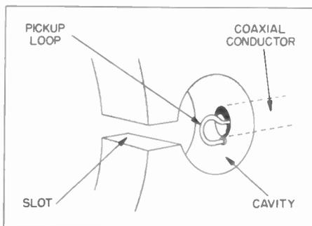
**Figure 15. Common Method of Coupling Energy from Magnetrons Operating at Wavelengths Longer than 3 Cm.**
