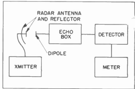
**Figure 26. Typical Test Setup Used in Spectrum Analysis**
