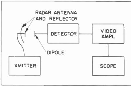
**Figure 28. Typical R-F Envelope Indicator Test Setup**
