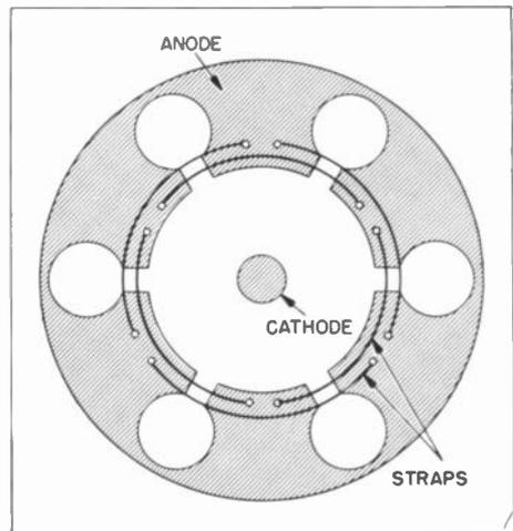
Figure 14. Strapping Arrangement in a Six-Cavity Magnetron (Double-Ring Strapping)
