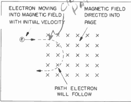
**Figure 4. Path of Electron Projected into Magnetic Field Oriented Perpendicularly to Electron's Initial Path**
