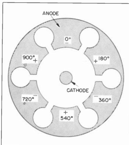
Figure 11. Six-Cavity Magnetron Operating in  $\pi$  Mode, or Mode 3
