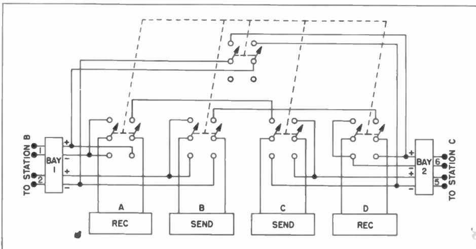
Figure 3. Schematic Diagram of Switching Circuit Installed at Each Station (Circuit shown is for station A; however, wiring system is identical at all three.)
