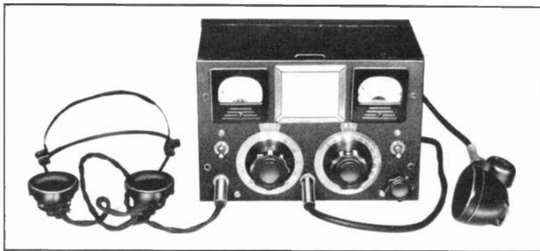
**Figure 1.** Front-Panel View of Test-Model Transmitter Monitor (The power-input cable and the three binding posts used for various transmitter tests are on the back of the unit.)
