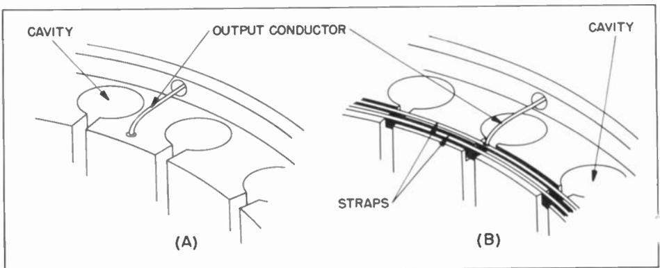
**Figure 17. Other Common Methods of Coupling Energy from a Magnetron**
