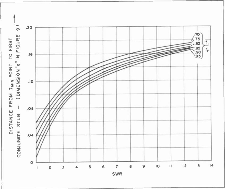
Figure 10. Chart for Determining Distance from  $I_{min}$  Point to First Conjugate Stub (See figure 9.)
