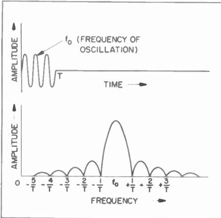
**Figure 25. Frequency Spectrum of R-F Pulse**
