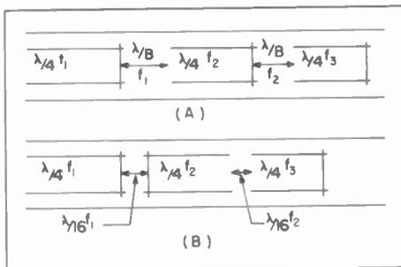
Figure 15. Minimum End-to-End Spacing for Adjacent Coplanar Coupling Sections
