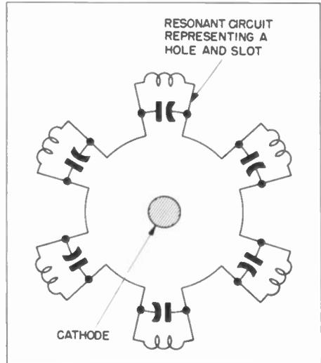
**Figure 7. Equivalent Circuit of a Six-Cavity Magnetron**
