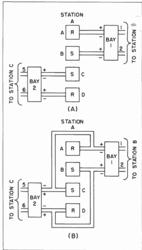
Figure 2. (A) Block Diagram for Normal Operation at Station A (B) Block Diagram for Relay Operation at Station A
