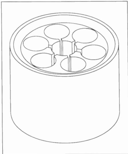
**Figure 2. Anode Block of the First British 10-Cm. Magnetron**
