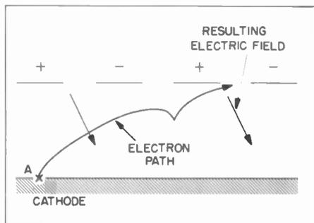
**Figure 9. Path of Electron Which Is Aiding Oscillation**
