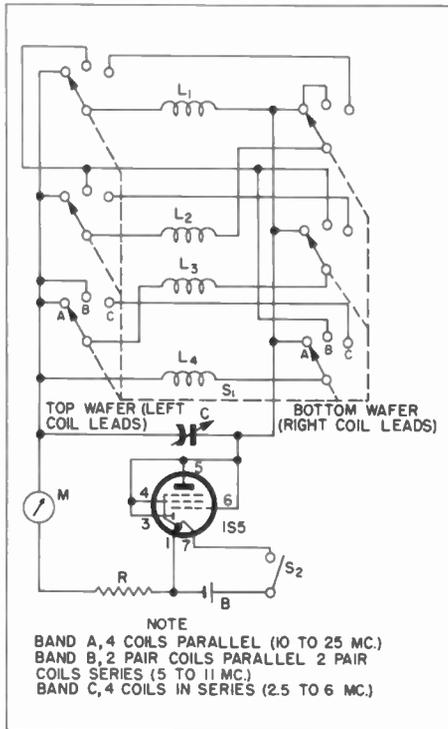
Figure 6. Schematic Diagram of Trolley Meter Shown in Figure 5
