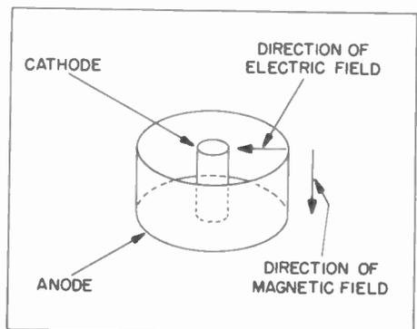
Figure 1. Basic Magnetron Arrangement
