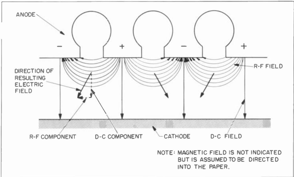
**Figure 8. Simplified Drawing of a Cavity Magnetron, Showing Electric-Field Configuration**
