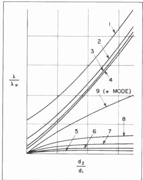
**Figure 19. Typical Mode Spectrum of a Rising-Sun Magnetron ( $\lambda/\lambda_\pi$  is ratio of the mode wavelength to the  $\pi$ -mode wavelength, and  $d_2/d_1$  is the ratio of the large resonator depth to the small resonator depth.)**
