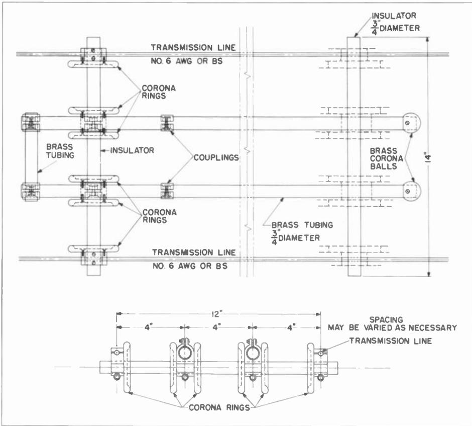
Figure 14. Construction Details of Coplanar Section (Top View of Mounted Section and Cross-Sectional View of One Support)
