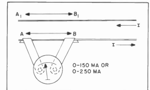
Figure 4. Shunt-Milliameter Method for Checking Balance of Transmission Line
