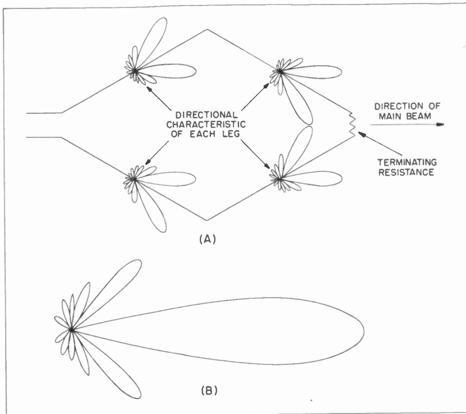
Figure 2. Radiation Pattern of Typical Terminated Horizontal Rhombic, Showing (A) Radiation from Individual Legs, and (B) Resultant Pattern
