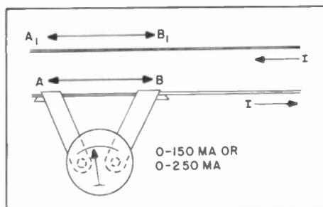
Figure 4. Shunt-Milliameter Method for Checking Balance of Transmission Line
