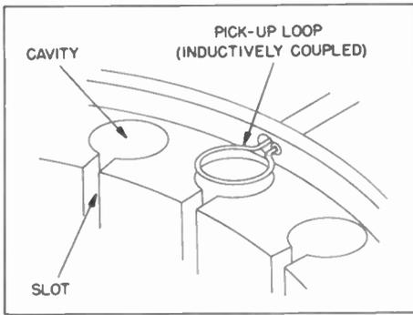
**Figure 16. Coupling Method for Magnetrons Operating at Wavelengths Shorter than 3 Cm.**
