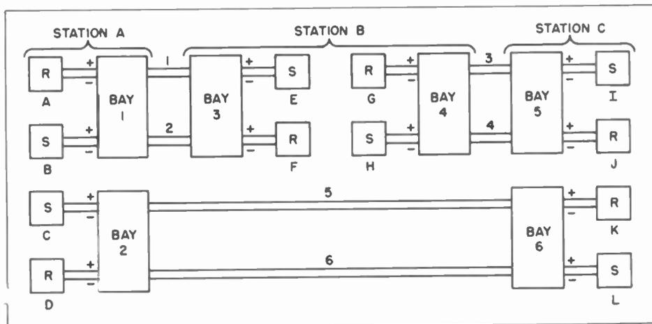
Figure 1. Block Diagram of Typical Three-Station Teletype System
