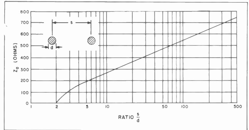
Figure 3. Graph of Characteristic Impedance ( $Z_0$ ) of Two-Wire Line
