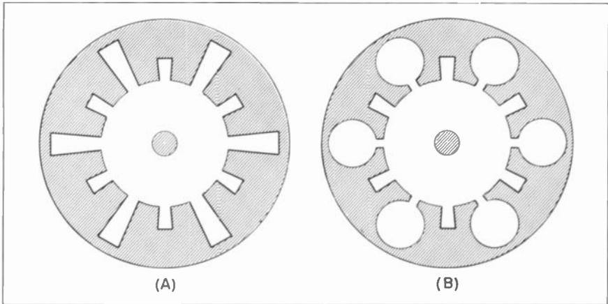
**Figure 18. Typical Designs of Anode Blocks Used in Rising-Sun Magnetrons**
