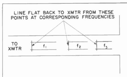
Figure 13. Schematic Diagram of Circuit in Which Inductively Coupled Matching Sections (Coplanars) are used to Match an Antenna to a Transmission Line at Three Frequencies
