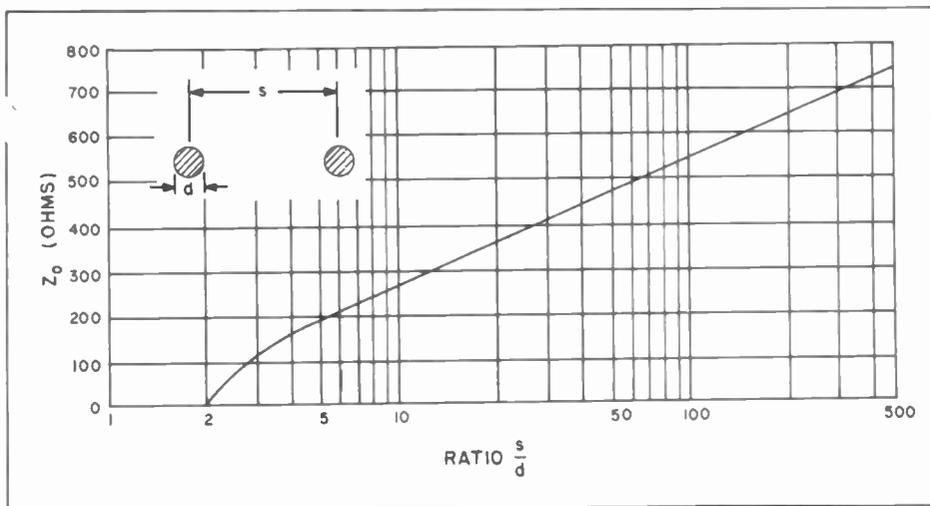
Figure 3. Graph of Characteristic Impedance ( $Z_0$ ) of Two-Wire Line
