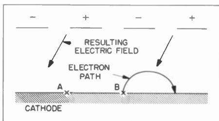
**Figure 10. Path of Electron Which Is Opposing Oscillation**
