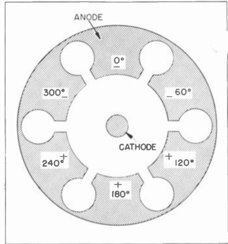
Figure 13. Six-Cavity Magnetron Operating in Mode 1
