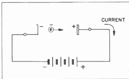
**Figure 3. Diode Circuit to Indicate the Effect of Electron Motion**
