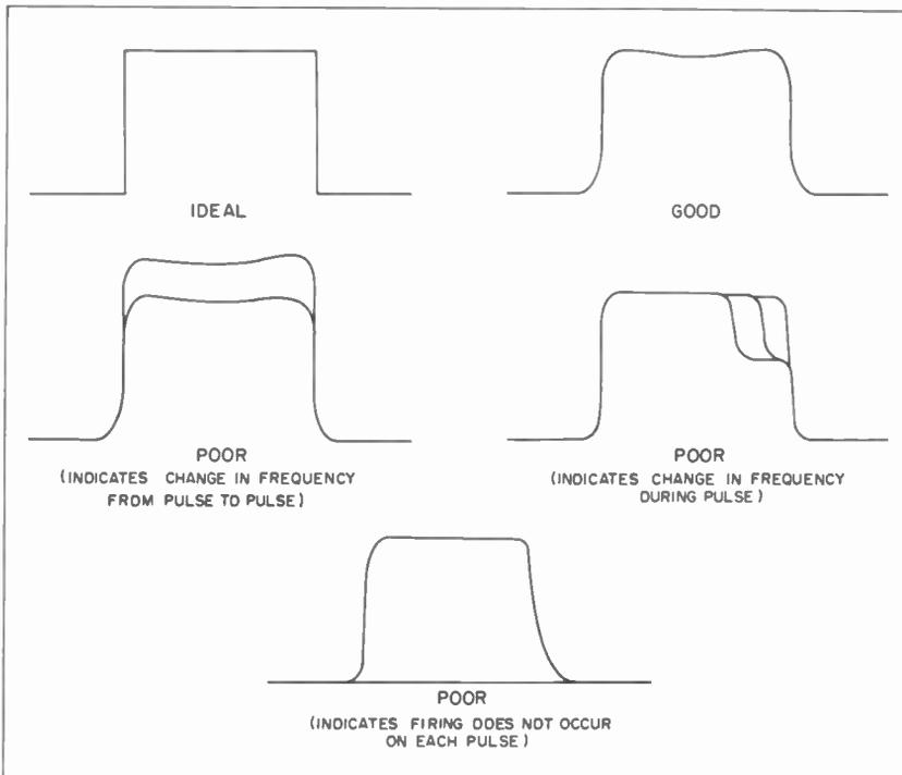
**Figure 29. Typical Waveforms Obtained with R-F Envelope Indicator, Showing Ideal, Good, and Poor Magnetron Operation**
