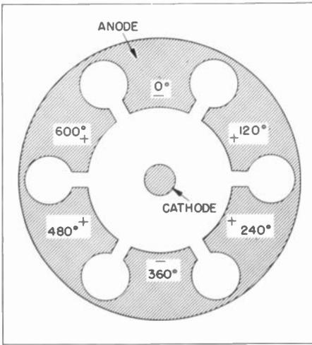
Figure 12. Six-Cavity Magnetron Operating in Mode 2
