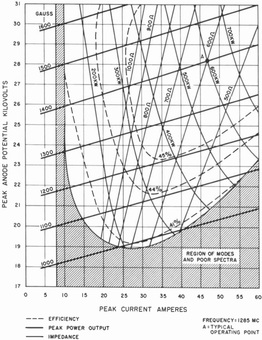
*Figure 20. Typical Magnetron Characteristic Curves*
