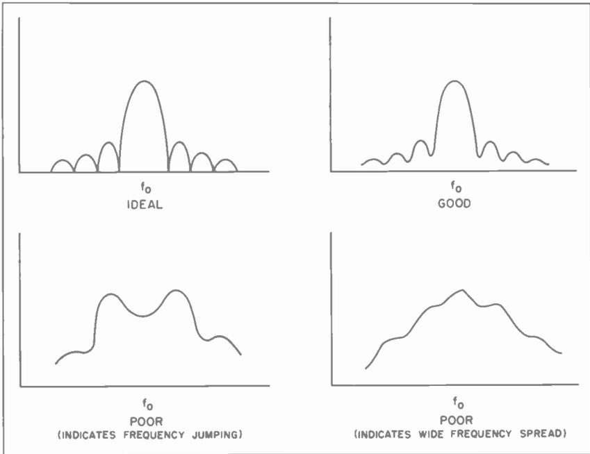
Figure 27. Typical Spectra of R-F Pulse
