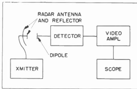
Figure 28. Typical R-F Envelope Indicator Test Setup
