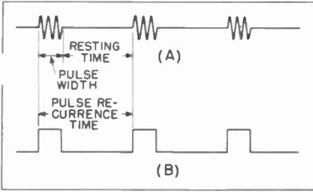
Figure 22. Magnetron Test Waveforms
