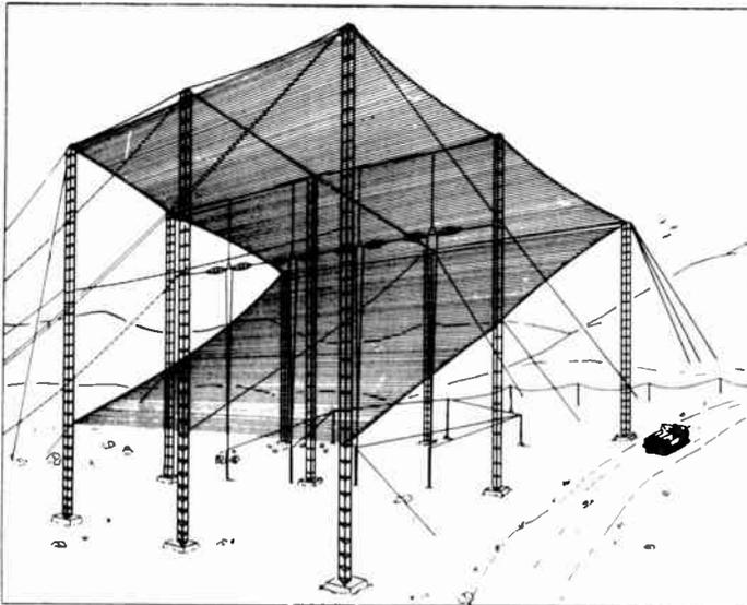
*Figure 5. Large Corner Antennas, Designed and Constructed by E. C. Page Consulting Radio Engineers in Cooperation with the National Bureau of Standards, Are Being Studied for Effectiveness in Comparison With Other Types of Antennas*
