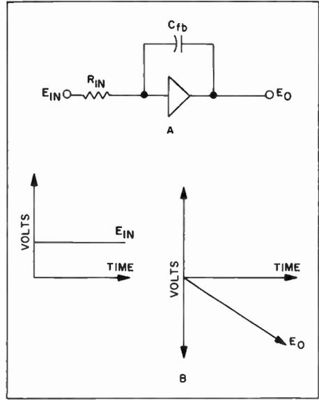
Figure 8. Integrating Circuit Employing a Computing Amplifier (Part A), and Steady Input Voltage and Integrating Output Voltage (Part B)
