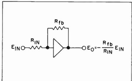
Figure 2. Multiplier Circuit Employing a Computer Amplifier
