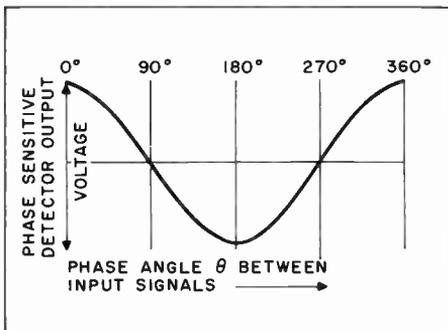
Figure 9. Response Curve for a Typical Phase-Sensitive Detector
