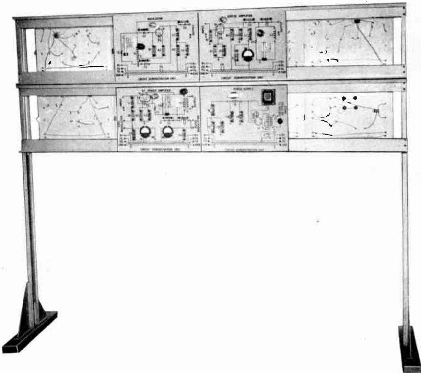
*Figure 2. The Philco Lecture Demonstrator Rack with Transmitter Circuit Demonstration Panels Displayed. Notice the Backs of the Circuit Demonstration Panels Which Are Displayed on the Other Side of the Rack.*
