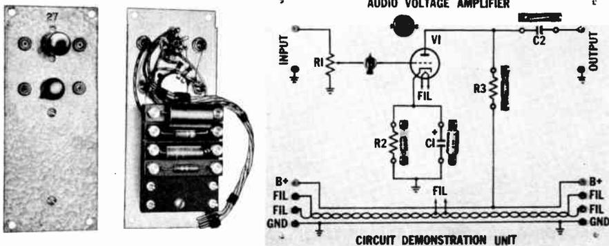
Figure 4. Philco Audio Amplifier Laboratory Circuit Analysis Chassis Number 27 (Front and Rear Views) at Left, and Audio Amplifier Lecture Demonstration Panel at Right
