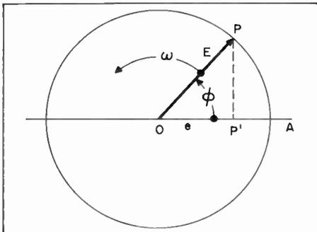
Figure 1. Vector Representation of a Sinusoidal Voltage of Frequency  $f$  and Initial Phase Angle  $\phi$
