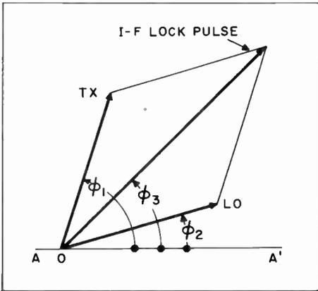
Figure 5. Combination of TX and LO Signals to Provide Lock Pulse
