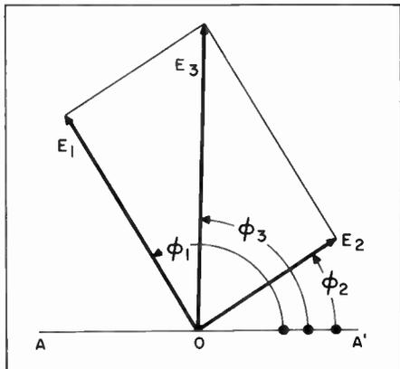
Figure 3. Addition of Conventional Vectors  $E_1$  and  $E_2$  to Obtain Resultant Vector  $E_3$
