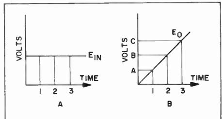
Figure 6. Graphical Representation of Integration of a Voltage
