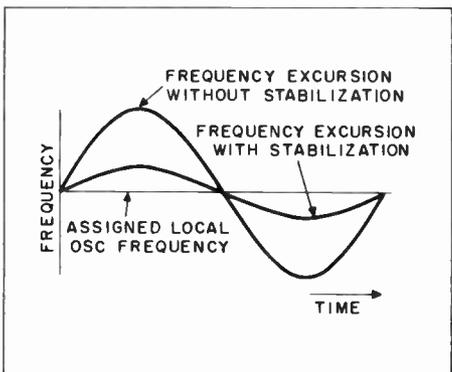
Figure 15. Effect of Frequency Stabilization Upon Local-Oscillator Signal
