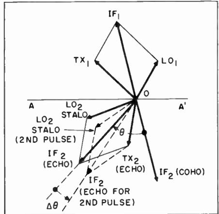
Figure 12. Effect of Pulse-to-Pulse Drift in Stalo Frequency
