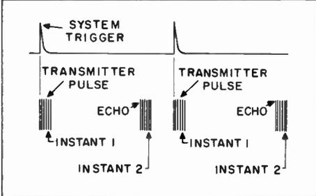
Figure 6. Timing Diagram for Radar Pulses
