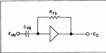
Figure 5. Differentiating Circuit Employing a Computer Amplifier
