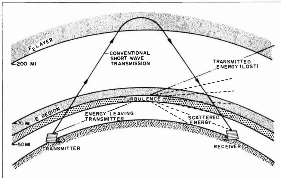
Figure 2. Comparison of Conventional Ionospheric Reflection of Radio Waves and Ionospheric Scatter of Radio Waves
