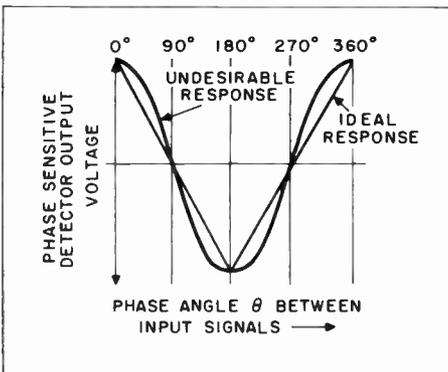
Figure 14. Comparison of Response Curves for a Phase-Sensitive Detector
