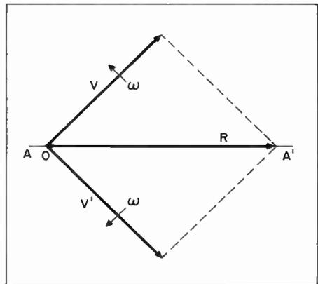
Figure 2. Representation of an Alternating Voltage by Contra-Rotating Vectors
