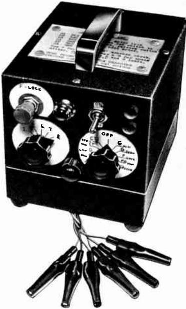
Figure 2. Utility Synchro Test Set
