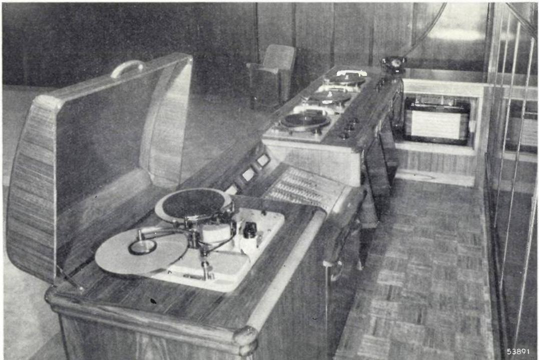
Fig. 5. Desk (5 in fig. 2) accomodating (from front to rear): Philips-Miller playback equipment, master control panel with push-buttons and pilot lamps, programme level-meters, three gramophones (each with three different pick-ups), radio receiver.
