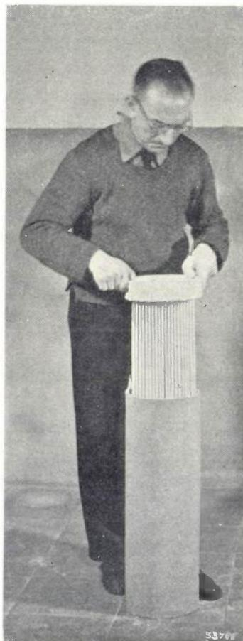
Fig. 4. One type of sagger used for loading ceramic articles into the kiln; it prevents soiling of the articles by the combustion gases.
