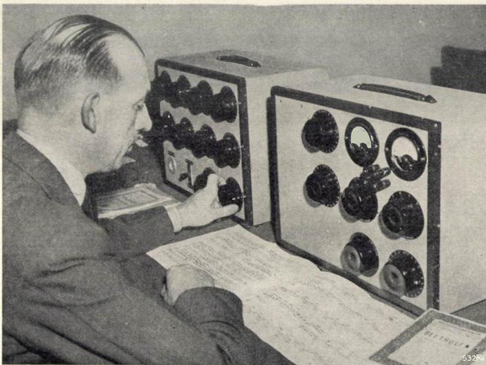
Fig. 2. Mixing and control panel in operation during the recording of a concert. The mixing and „volume compression” is effected with the musical score and the experience gained during rehearsals as a guide. The control knobs referred to in fig. 1 can be easily identified from the photograph: a number of plug sockets will also be seen, these being employed for the connection of different meters, a telephone and a communication microphone (e.g. for speaking to the conductor).
