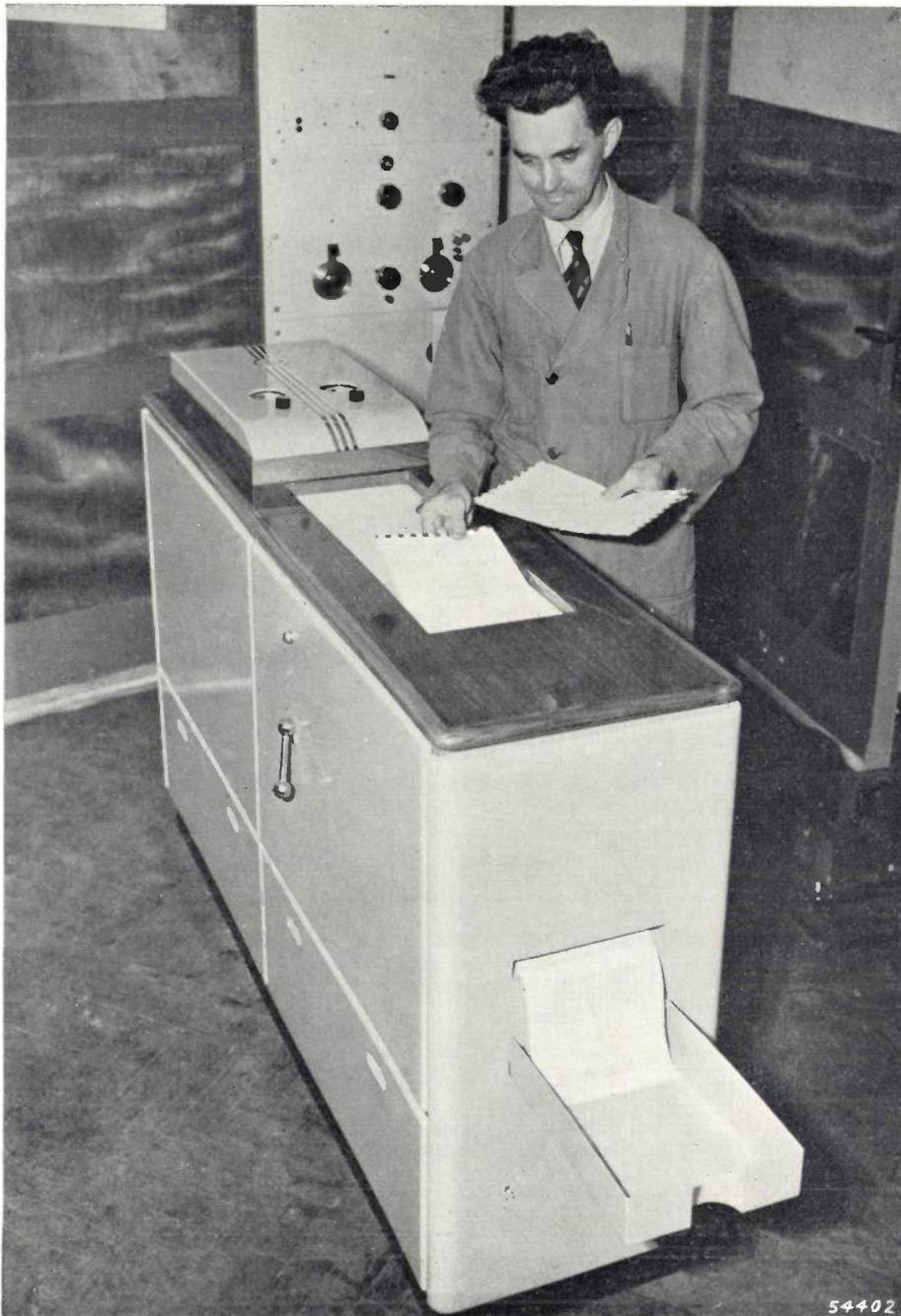
Fig. 2. Transmitter of the Philips high-speed facsimile equipment in operation. Documents of any size up to 22 cm in width are placed on an endless belt running just below the aperture in the table top. When finished with, they fall into the collecting tray seen at the front end of the unit.
