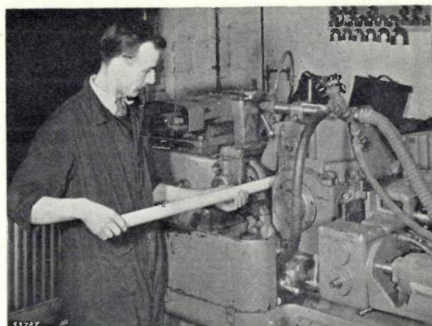
*Fig. 6.* Grinding ceramic rods and bars on a centreless grinder.
