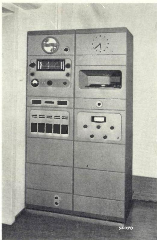
Fig. 6. Rack containing receiver for directional radio reception, monitor speaker, gramophone, programme level-meter and switch panel with correcting filters.
