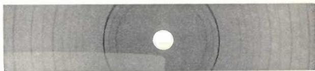
Fig. 3. Diffraction pattern of a specimen obtained on a photographic film. The "lines" (rings) are the intersections of the film with the series of cones shown in *fig. 2*. (The shadow along the lower left hand edge of the pattern is produced by a thin nickel filter, offering a means of identifying undesired  $K\beta$ -lines of the copper radiation<sup>8</sup>.)
