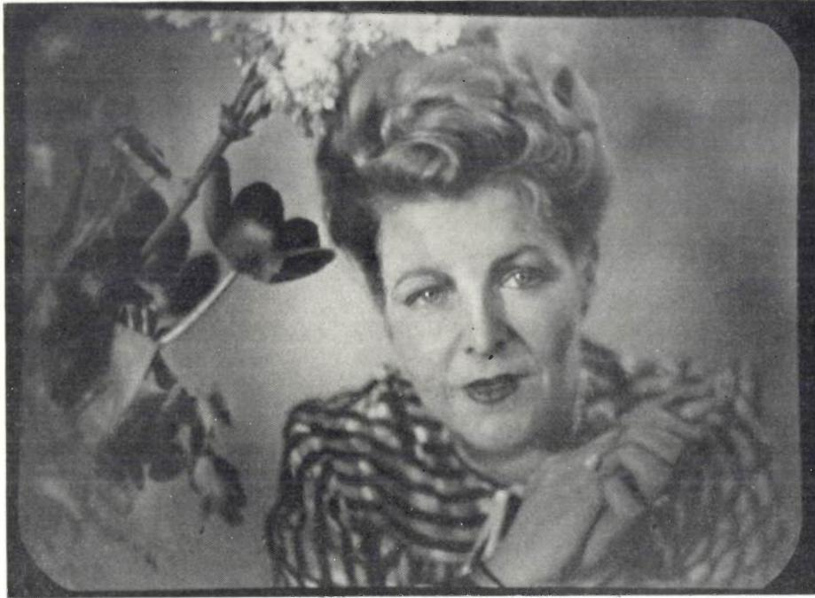
Fig. 10. Photograph of a television picture transmitted from the experimental station at Eindhoven and received with an apparatus of the type illustrated in fig. 1. Number of lines 567 (interlaced scanning <sup>9)</sup>), 50 frames per second
