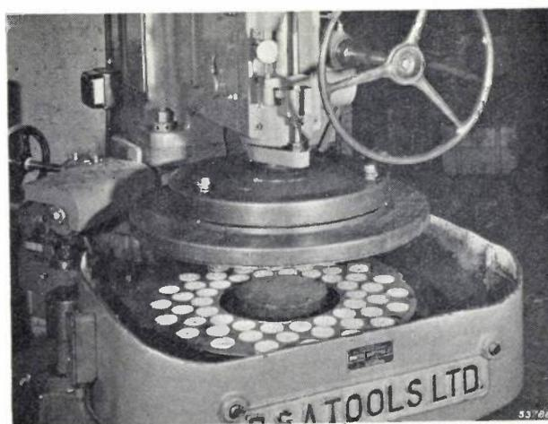
*Fig. 7.* Grinding machine as used for finishing ceramic discs. These are ground between two flat plates until they are themselves quite flat and parallel.
