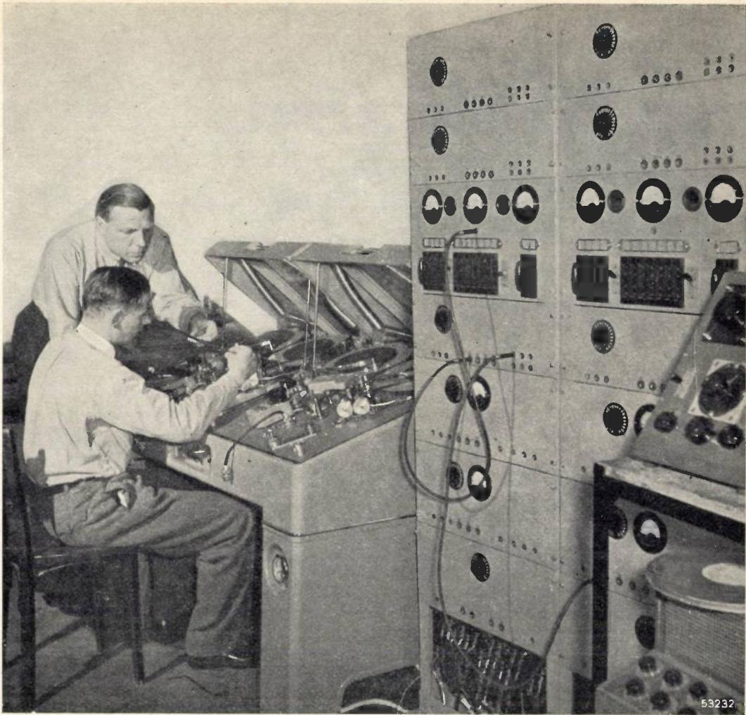
Fig. 3. The Philips-Miller unit, showing some of the amplifier racks etc. installed in the Concertgebouw, Amsterdam.
