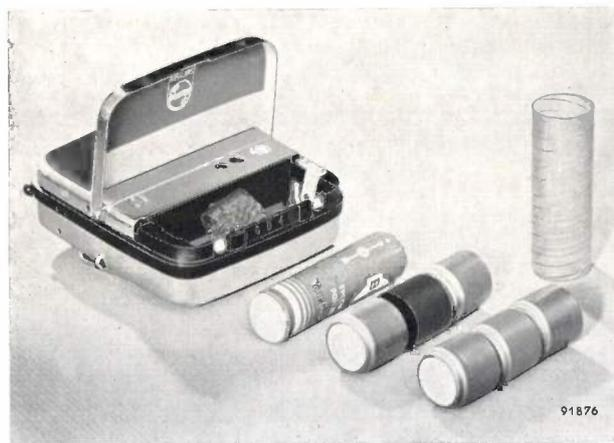
Fig. 2. The battery holder of the KL 5500 hearing aid, with the three types of batteries that may be used: a Leclanché dry cell (1.5 V), two mercury cells with filler piece (2.6 V) or 3 mercury cells (3.9 V).
