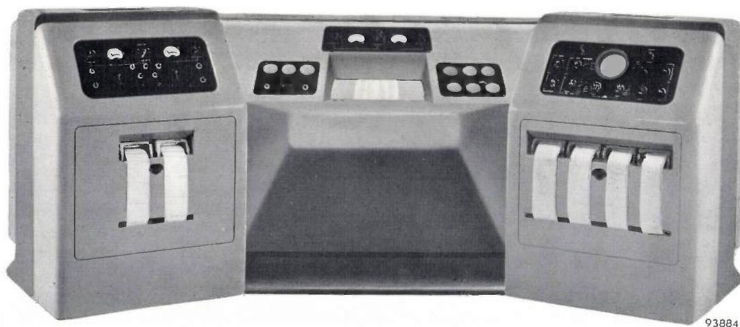
*Fig. 6.* The telemetering console. The left-hand unit contains wind-speed and height recorders, the right-hand unit encoders and temperature, pressure and humidity recorders and the centre unit a digital computer and teleprinter.
