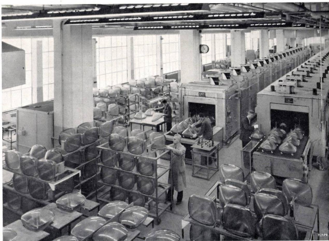
The envelope of a television picture-tube consists of three parts: the screen, "cone" and neck. When these parts are fused together, stresses are set up in the glass. To relieve these stresses, the envelopes are conveyed on a moving belt through a long annealing oven. The above photograph shows the process in operation in the new television tube factory in Eindhoven.
