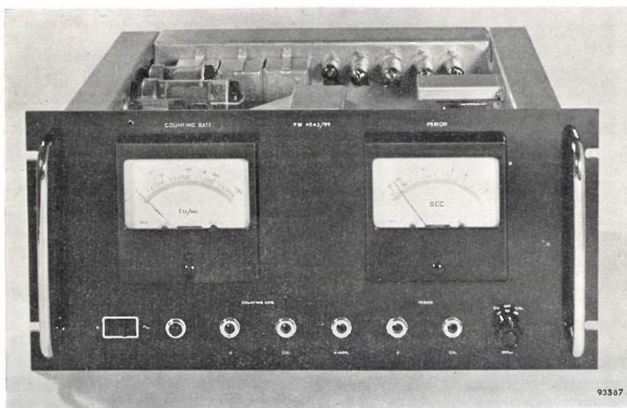
Fig. 8. Logarithmic count-rate and period meter PW 4043 for low neutron flux. The meter on the left indicates the number of pulses per second (scale 1 to  $10^4$ ), the meter on the right indicates the reactor period in seconds (scale from  $-30$  via  $\infty$  to 3 seconds; cf. fig. 10).
