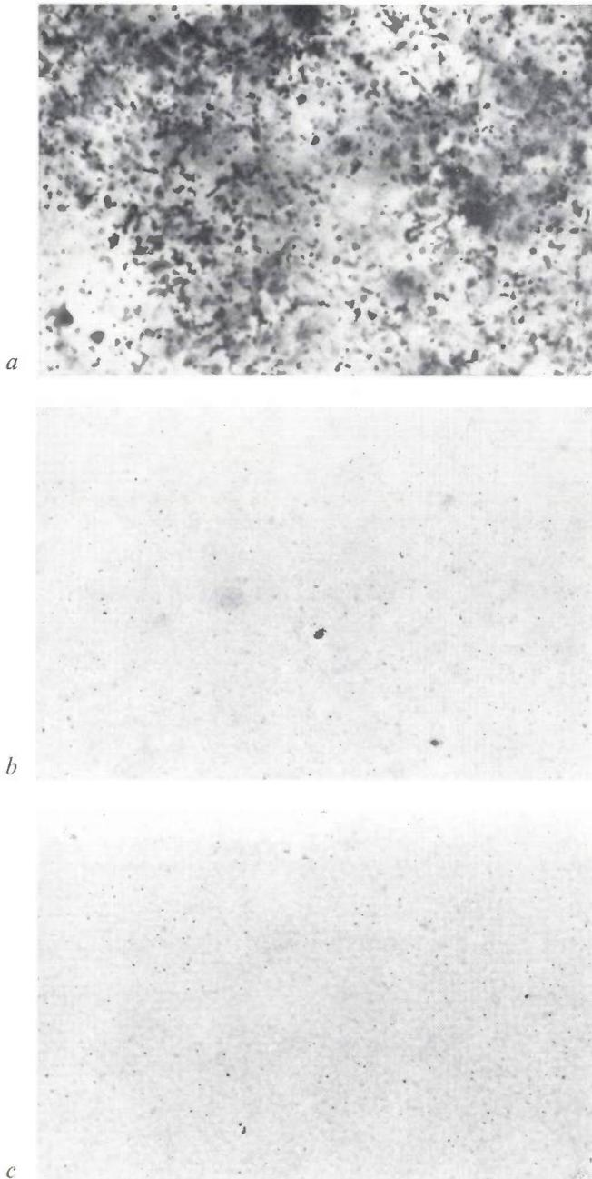
Fig. 5. Photomicrograph of a sample of PLZT (11/65/35), taken with transmitted light. *a*) Initial condition after conventional sintering. *b*) After hot pressing by our method (two hours, 1170 °C, in N<sub>2</sub> at 200 bars). *c*) After hot pressing under the same conditions, but now for 16 hours. Magnification 150×.
