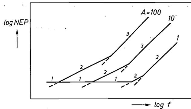
Fig. 3. Variation (schematic) of noise equivalent power  $NEP$  with frequency  $f$  for three values of the irradiated electrode area  $A$ . In region 1 the amplifier current noise is dominant; in 2 the Johnson (thermal) noise in the pyroelectric crystal and in 3 the amplifier voltage noise.
