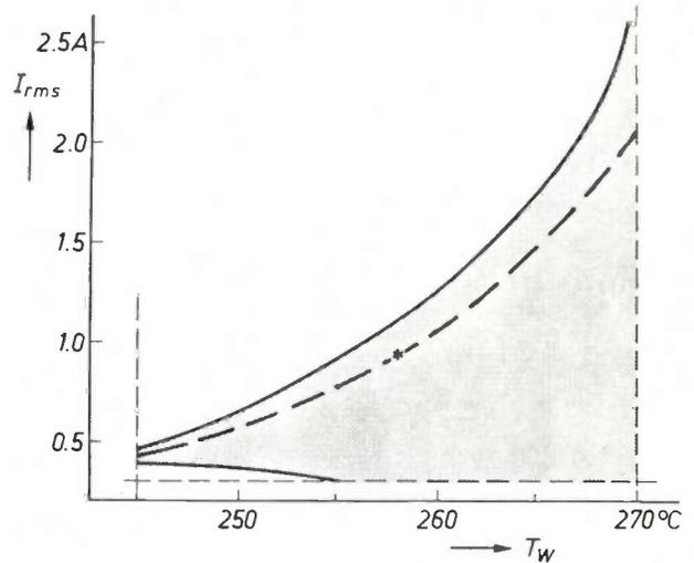
Fig. 12. The region in which, depending on the r.m.s. discharge current  $I_{rms}$  and the wall temperature  $T_w$ , a d.c. sodium discharge (grey area) or an a.c. sodium discharge (white area) is more efficient as a light source. The dashed line gives the conditions for which the difference between the two forms of discharge is greatest. The asterisk denotes the operating point of the 90-W SOX lamp.
