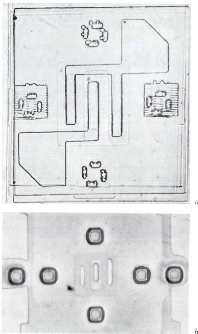
Fig. 12. Experimental *N-P-N* transistors made by electron exposure of PMCS resist, with emitter widths of 50  $\mu\text{m}$  (a) and 5  $\mu\text{m}$  (b). In (a) the central metal strip is the emitter connection, and the forked strip the base connection. The four surrounding patterns are location marks. The photograph (b) was made before metallization, and the PMCS passivating layer can be seen. Magnifications are 200 $\times$  in (a), 675 $\times$  in (b).
