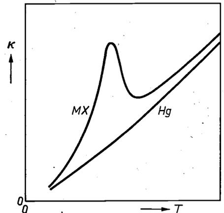
Fig. 7. Thermal conductivity  $\kappa$  as a function of temperature  $T$  for a metal-halide plasma (MX) and a mercury plasma (Hg), schematic.
