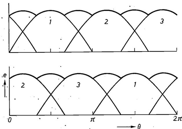
Fig. 4. The induced voltage  $e$  in the three rotor coils 1, 2 and 3; the top and bottom curves are for the two rotor paths;  $\theta$  indicates the angular position of the rotor in the stator. Each rotor coil forms part of both rotor paths in turn; commutation is assumed to be ideal. The thick line gives the resultant speed voltage.
