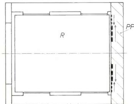
**Fig. 2.** Diagram of a thrust bearing for a cylinder (*R*), such as the rotor of a gyroscope, with a push-pull spiral-groove bearing (*PP*). One spiral-groove bearing is sufficient for the axial location of *R*.
