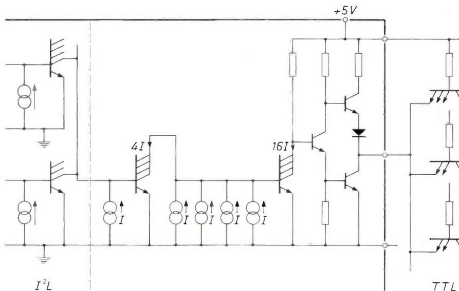
**Fig. 15.** Interface circuit integrated with I<sup>2</sup>L for connection to TTL, for which larger currents are necessary. The interface circuit comprises a current amplifier followed by a totem-pole output stage.
