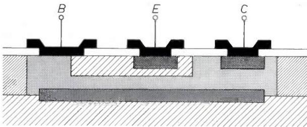
Fig. 10. Cross-section of a Schottky transistor. The base contact *B* extends over the *N*-type collector region and the two form a Schottky diode parallel to the base-collector junction. *E* emitter. *C* collector contact.
