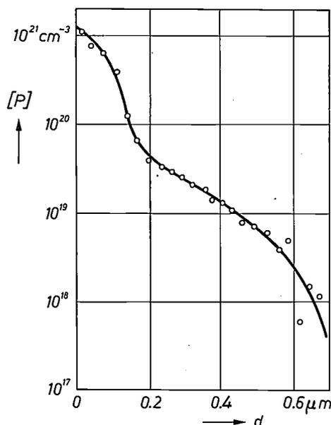
Fig. 8. Example of a 'tail' in a diffusion profile. At a depth *d* of about 0.15  $\mu\text{m}$  there is a kink in the concentration profile, followed by the tail. In this case phosphorus marked with a radioactive tracer was diffused into the silicon. (After D. B. Lee [32].)
