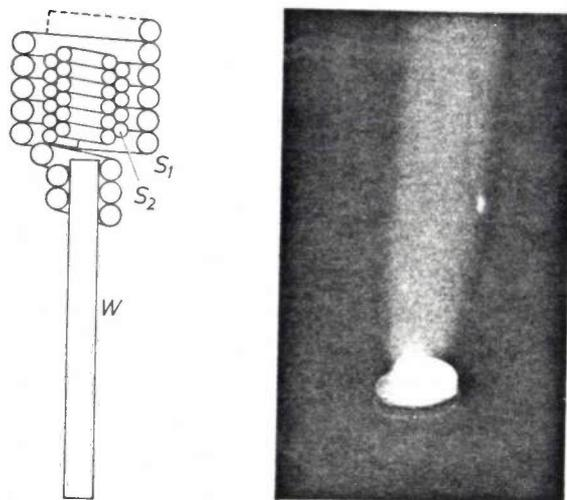
Fig. 5. Electrode of a 375-W HPI lamp. *Left*: schematic cross-section (magnification about  $5\times$ ). *W* tungsten rod. *S*<sub>1</sub> tungsten coil. *S*<sub>2</sub> tungsten coil in two layers, located in the gap between *W* and *S*<sub>1</sub> and kept in place by the bent end of *S*<sub>1</sub>. *Right*: the electrode in operation.
