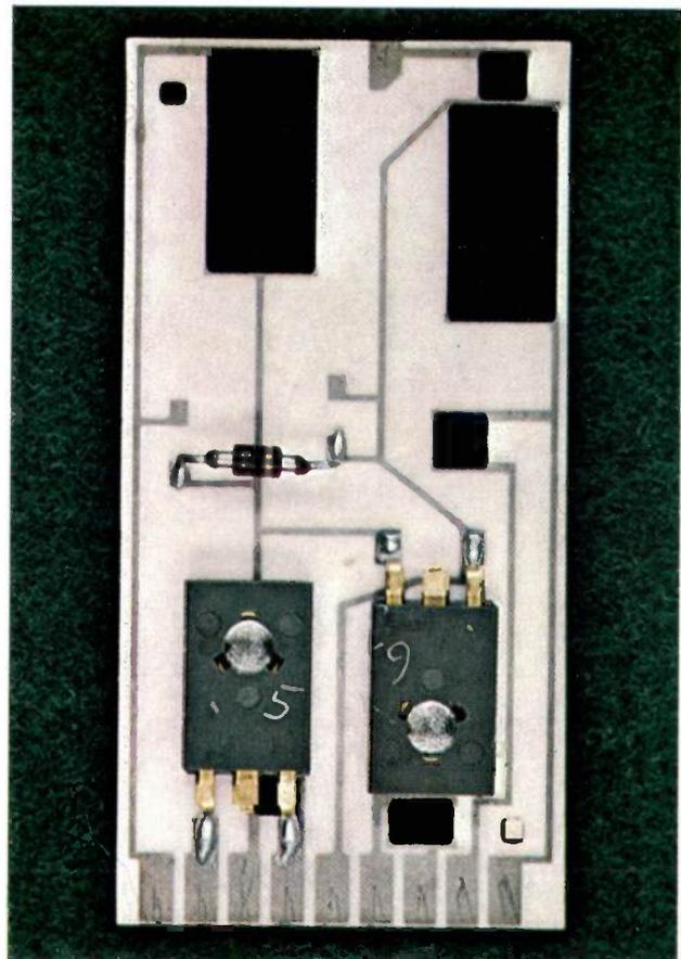
**Fig. 3.** Power amplifier ( $25 \times 50$  mm) for consumer electronics. The plug-in substrate carries six resistors (black), a diode and two power transistors. The two large resistors at the top are each rated at 3 watts.
