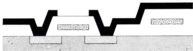
Fig. 3. Use of polycrystalline silicon as a gate (left) and as the lower layer of a double-layer interconnection pattern (right). The upper layer is of aluminium. The materials used are given in the key.
