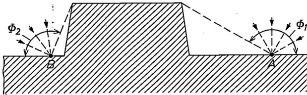
Fig. 12. Diagram illustrating the deepening of the 'ditches' formed during the etching as a result of back-diffusion. The solid angle  $\Phi_2$  through which ions back-diffuse to point *B* is smaller than  $\Phi_1$ , which is the corresponding solid angle for point *A*. This results in a higher etch rate at *B* than at *A*, and hence in a deeper ditch.
