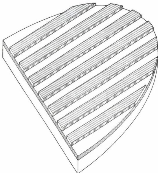
*Fig. 1.* The type of specimen on which most of the investigations described were carried out: a silicon chip covered with a thin coating of oxide, with an etching mask consisting of parallel strips of titanium or other substance on top of it. After ion etching, the specimen is broken at right angles to the longitudinal direction of the strips and the resultant cross-section is compared under a microscope with that of the unetched specimen.
