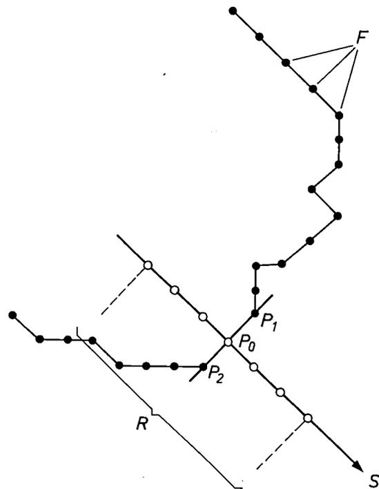
**Fig. 16.** Principle of fine searching for a cardiac contour. *F* coarse contour; this provides the initial input data. *S* the new search direction, constructed by the computer as a normal to the coarse contour. ( $P_{0,1,2}$  are additional construction points). *R* search interval; its size is determined by the maximum error in *F*.
