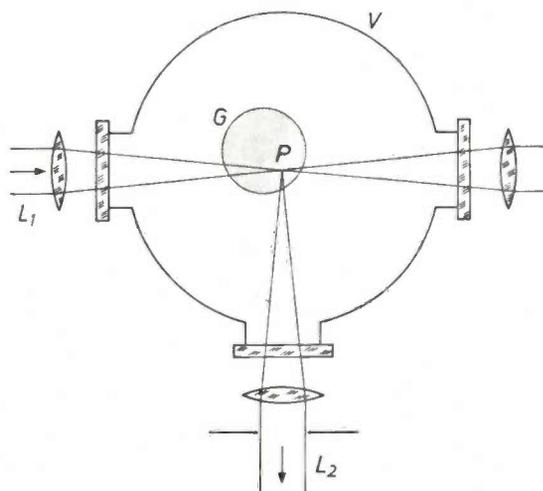
Fig. 2. Light-scattering measurement, schematic.  $G$  cross section of the discharge tube in the vessel  $V$ . The light of a laser beam  $L_1$  is focused at the point  $P$  under investigation, and the scattered light  $L_2$  is selected by a second optical system. The intensity of  $L_2$  is proportional to the concentration of the scattering particles in  $P$ .
