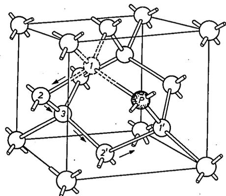
Fig. 3. The crystal lattice of silicon with a vacancy (*V*) and an impurity atom (*P*). It is shown how the direct exchange of an impurity atom with a nearest-neighbour vacancy can take place in this lattice (G. D. Watkins and J. W. Corbett [23]). The vacancy in the first nearest-neighbour position (No. 1) must make two jumps away from the *P* atom and then arrives at position No. 3; after this the vacancy returns to another nearest-neighbour position (No. 1).
