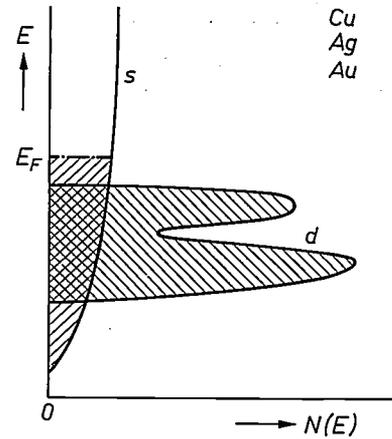
Fig. 6. Energy diagrams for the metals copper, silver and gold. In addition to the conduction band, which contains s-like electrons, there is a relatively narrow band of d states. This band is completely filled and makes no contribution to the conduction.
