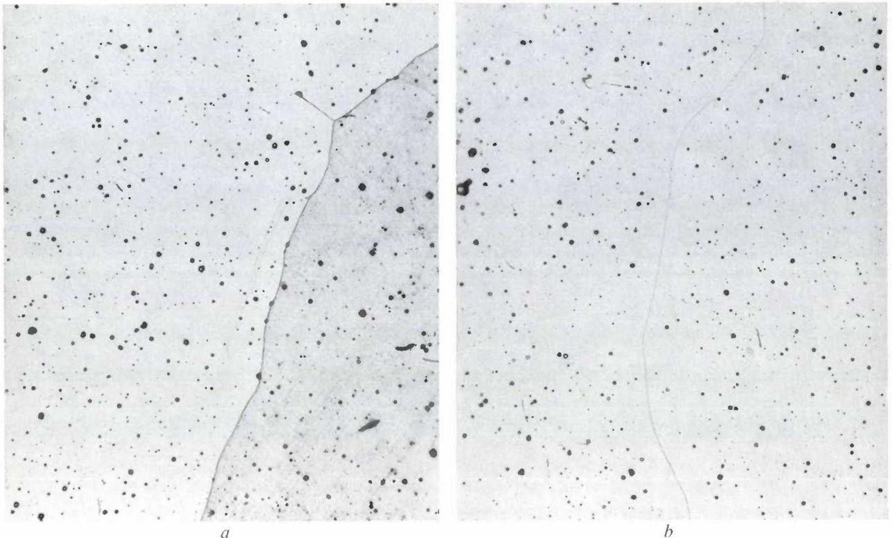
**Fig. 20.** The microstructure of a ferrite sintered with an anion deficit (see also fig. 17b). *a)* Before isostatic hot pressing. *b)* After isostatic hot pressing. Only the pores in the neighbourhood of a grain boundary have disappeared. The pressing does not affect the pores inside the grains (which are large, up to 1  $\mu$ m). (After Stassen, De Lau and Veenman [85].)
