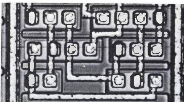
Fig. 12. Layout of  $I^2L$  circuit. The multicollector transistors are located on either side of the long, narrow *P*-type regions, the injectors, which are the common emitters of all the *P-N-P* current generators. The position of the base contact among the collectors can be chosen to suit the interconnection pattern. The transistors are surrounded on three sides by  $N^+$  separation regions.
