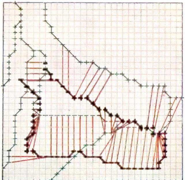
Fig. 15. The template is still some way away from the object. The distance lines are much longer than in the situation shown in fig. 14.
