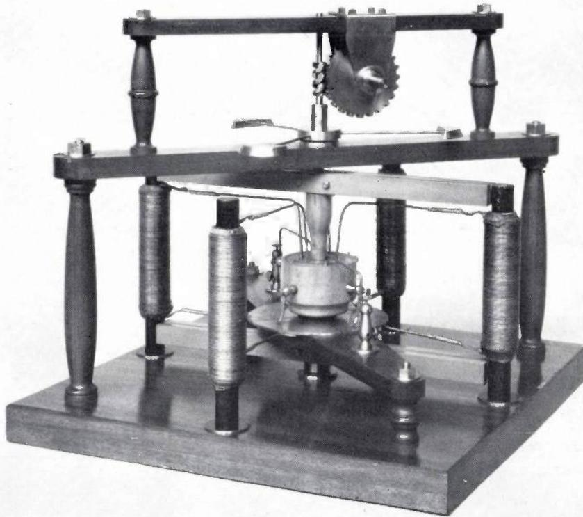
Fig. 5. Reconstruction of one of Sturgeon's motors. The rotor consists of two horizontal bar magnets, which rotate past the poles of four electromagnets. These are connected through a commutator, which consists of two concentric jars of mercury, four sliding contacts and a contact disc divided into four quadrants. (Crown Copyright. Science Museum, London.)
