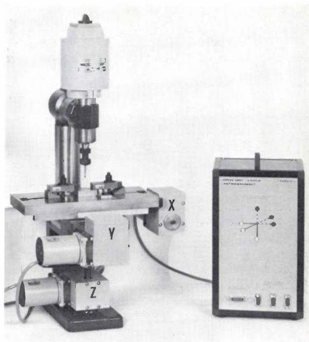
**Fig. 3.** Numerically controlled vertical milling machine, made by Terco, with drive unit. Three stepping motors (Philips PD 20) displace the workpiece along the *x*-, *y*- and *z*-axes. (Photo Terco AB, Skärholmen, Sweden.)
