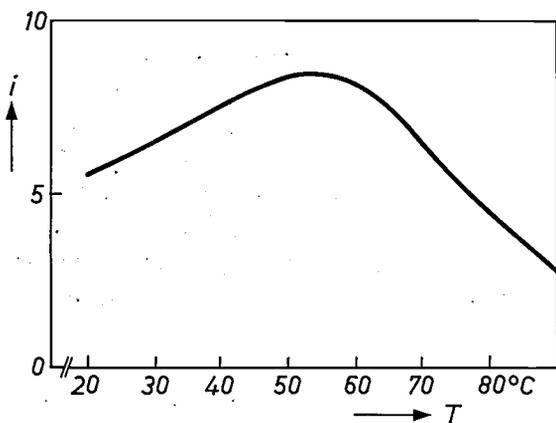
Fig. 9. The temperature dependence of the pyroelectric a.c. current  $i$  for an l-alanine-doped crystal (LATGS) grown from a solution containing 60 mol% of l-alanine. During the measurements the temperature of the crystal of the detector element was gradually raised, while the incident infrared radiation was chopped at a convenient frequency.
