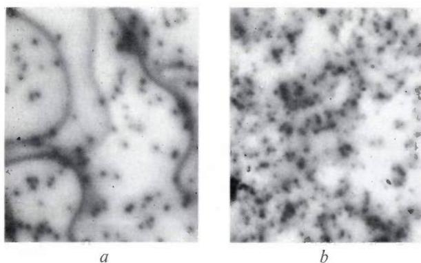
Fig. 11. Luminescence images of two nitrogen-doped GaP samples at widely different dopant concentrations. The wavy lines in *a*) are due to surface steps. Magnification  $270\times$ .
