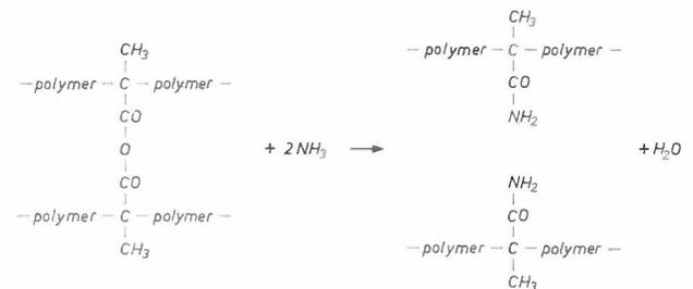
The separated chains then dissolve in the acetone just as PMMA does. We developed the acetone/ammonia mixture for metals that are attacked by fuming nitric acid.
