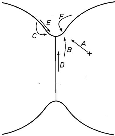
Fig. 12. Model for the geometry and the diffusion flux paths in the initial stage of sintering. *A, B* and *C* volume diffusion. *D* grain-boundary diffusion. *E* surface diffusion. *F* vapour transport. (After Johnson [41].)
