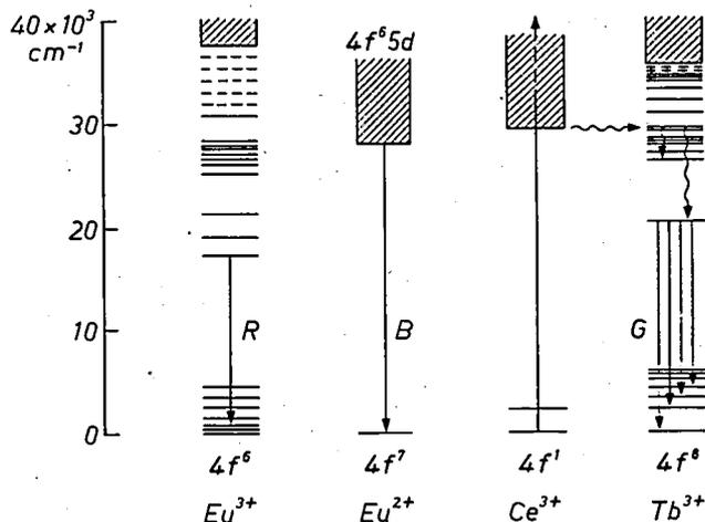
Fig. 12. Energy-level diagrams of the rare-earth ions used as activators in the phosphors for the new fluorescent lamps. The red emission of  $\text{Eu}^{3+}$  is a sharp line, the blue emission of  $\text{Eu}^{2+}$  is less sharp because a 5d state is involved. The green emission of  $\text{Tb}^{3+}$  consists of a number of sharp lines, and in practice corresponds to a band 80 nm broad.  $\text{Ce}^{3+}$  is used as a sensitizer in the newly developed green phosphor.
