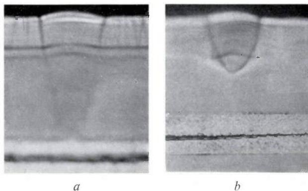
**Fig. 9.** Longitudinal sections through filaments with activated growth of nodules, *a*) starting from the tungsten substrate wire, *b*) from an imperfection in the boron layer.
