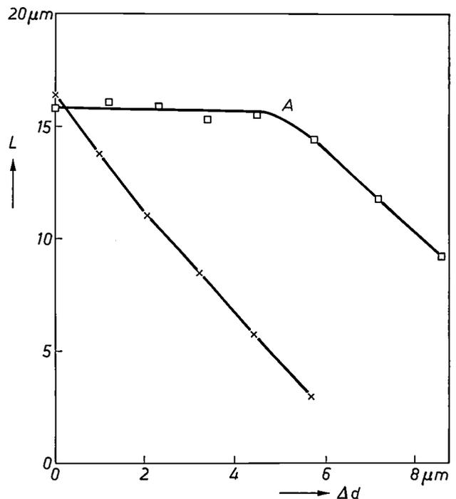
Fig. 14. The width  $L$  of the mask strips in fig. 1 as a function of the etch depth  $\Delta d$  in silicon, with a photoresist (Shipley AZ 1350 H) and titanium (upper curve) as mask materials. In the case of titanium the width of the strip does not start to decrease until point *A* is reached, i.e. only when the mask has been almost entirely removed by etching. This shows that titanium is considerably more suitable as a mask material than the particular photoresist it is compared with here.
