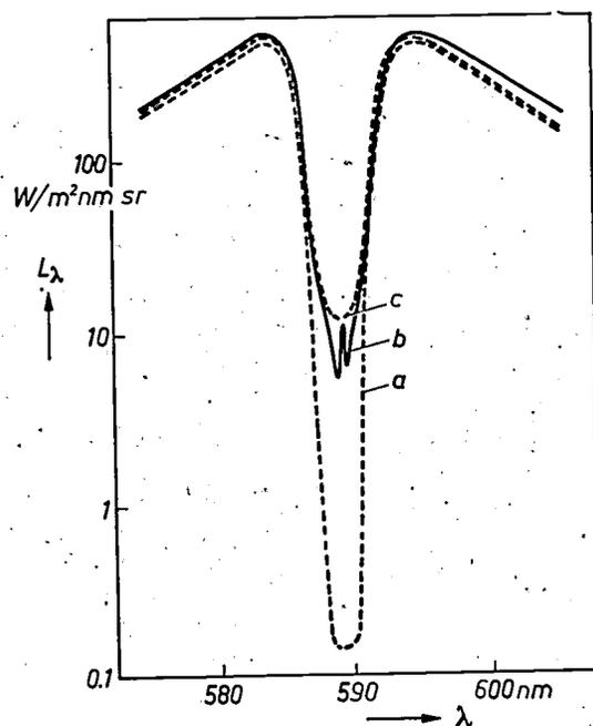
Fig. 9. The spectral radiance at the centre of the sodium D lines. *a* contour calculated on the assumption of local thermodynamic equilibrium. *b* measured contour. *c* contour calculated without assuming local thermodynamic equilibrium. The two separate emission minima revealed by the measurement may be a result of the effect of the tube wall on the plasma.
