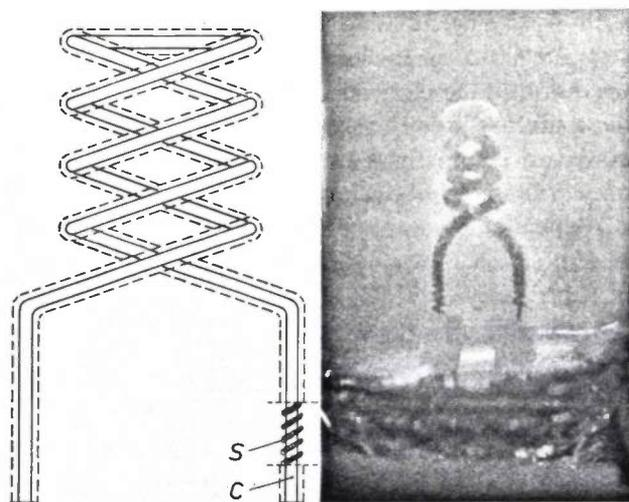
**Fig. 3.** *Left:* schematic representation of an electrode for an SOX lamp (magnification about 5×). Around a core C of tungsten wire, itself coiled, there is a coiled tungsten wire S. *Right:* the electrode in operation.
