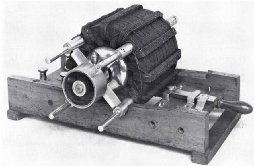
Fig. 21. Tesla's two-phase induction motor (1888). Neighbouring groups of three of the twelve stator coils are successively connected in series. The stator iron is laminated. (Crown Copyright. Science Museum, London.)
