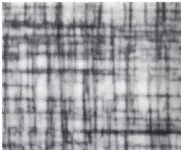
**Fig. 14.** Luminescence image of the dislocation network at the transition from GaAs to GaAsP. The dislocation density corresponds to values expected from the phosphorus-concentration gradient. Magnification  $1900\times$ .
