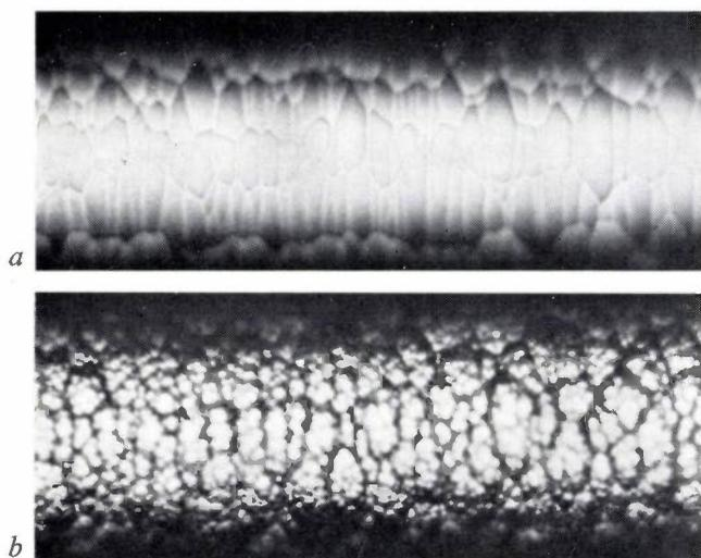
Fig. 11. *a*) Surface of a boron filament made at 1230 °C. *b*) As (*a*), but at 970 °C. The tensile strengths of these filaments were 4000 and 1500 N/mm<sup>2</sup> respectively.
