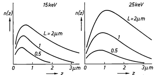
Fig. 5. Minority-carrier excess  $n(z)$  as a function of the depth  $z$  below the surface; this distribution results from the generation function  $g(z)$  given in fig. 4, taking diffusion and recombination into account. The concentration  $n(z)$  was calculated at two values of the primary electron energy  $E_0$  and for three values of the diffusion length  $L$ . Comparison with fig. 4 shows the effect of diffusion and the high surface-recombination rate.
