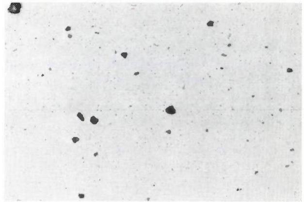
Fig. 6. Photomicrograph of a conventionally sintered wafer of BaTiO<sub>3</sub> ceramic. Magnification 150×.
