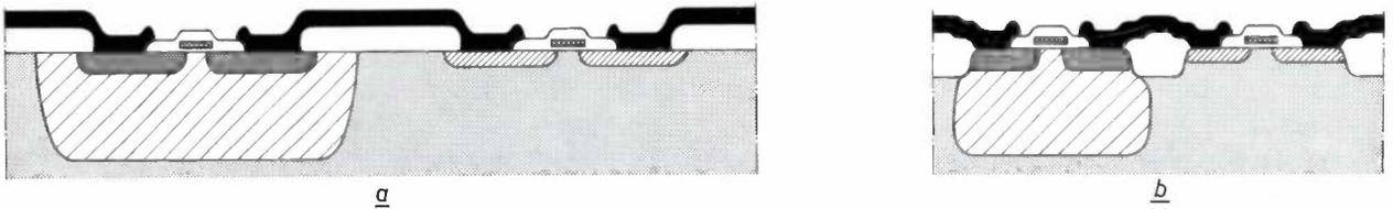
**Fig. 8.** Cross-section of a pair of complementary MOS transistors. The  $N$ -channel transistor is on the left, the  $P$ -channel one on the right. The gates are of polycrystalline silicon. *a)* Standard technology. *b)* LOCOS technology. Thick local oxidation is used as insulation; less chip area is consequently required.
