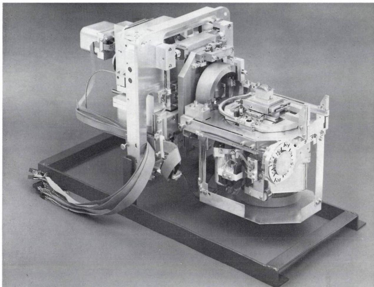
**Fig. 17.** The eucentric goniometer of the PSEM 500. The motor for driving the tilt movement can be seen at the upper left. The motors for the other rotation and translation movements are mounted in the lower right-hand part of the instrument. On top of this right-hand part is the specimen-holder with the specimen, in this case an integrated circuit. The supply leads for the various motors, and those for the specimen stage, are made in the form of flexible strip.
