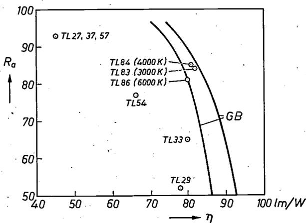
Fig. 13. The newly developed fluorescent lamps TL 83, TL 84 and TL 86, with the colour temperatures 3000, 4000 and 6000 K, together with some currently used lamps in the  $R_a$ - $\eta$  diagram. GB curves indicating what is theoretically feasible with a green band and two lines (see fig. 11).
