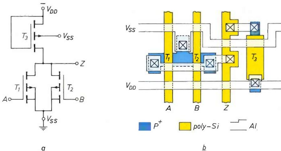
Fig. 1. Circuit diagram (a) and layout (b) of a NOR gate with two inputs A and B. The gate consists of three P-channel MOS transistors,  $T_1$ ,  $T_2$  and  $T_3$ , all of the enhancement type. Output Z is at ground potential if either or both of the inputs are negative.  $V_{SS}$  ground potential.  $V_{DD}$  negative supply voltage.
