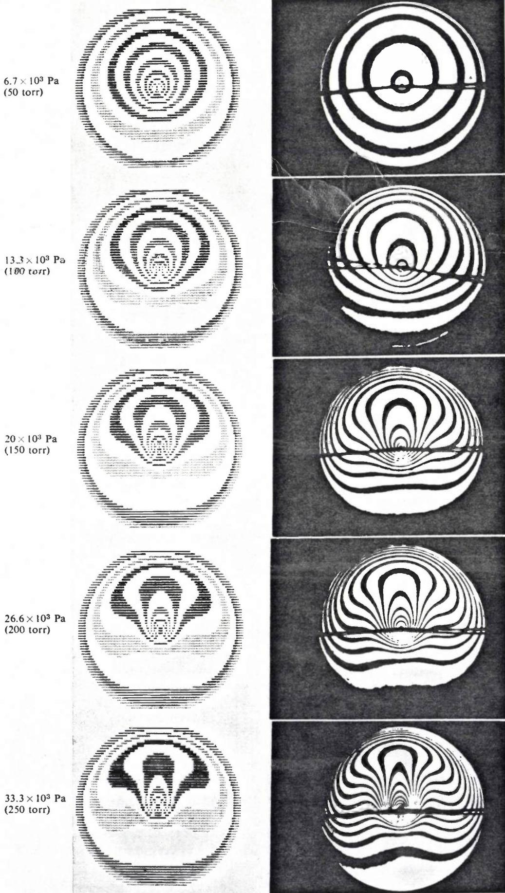
Fig. 1. Calculated temperature distributions (*left*) and interference patterns (*right*) in an axially symmetric argon-filled incandescent lamp (argon pressure  $p$ ) in a plane perpendicular to the filament. In this lamp each fringe represents an isotherm. The diameter of the tube is 4 cm, diameter of wire 200  $\mu$ m.
