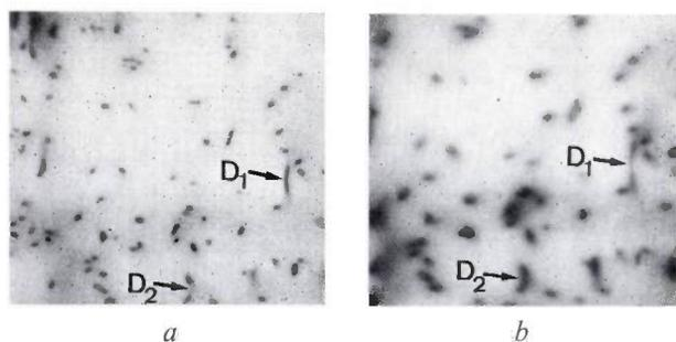
Fig. 8. Luminescence images of a GaAs sample at two values of primary-electron energy. *a*) 17 keV. *b*) 35 keV. The dislocation  $D_1$  is clearly and completely visible at low energy, whereas at high energy only the two ends of the dislocation can be seen. The dislocation must therefore be curved, with the convex side towards the specimen surface. Similar arguments show that dislocation  $D_2$  is also curved, but with the concave side towards the surface. Magnification 160 $\times$ .
