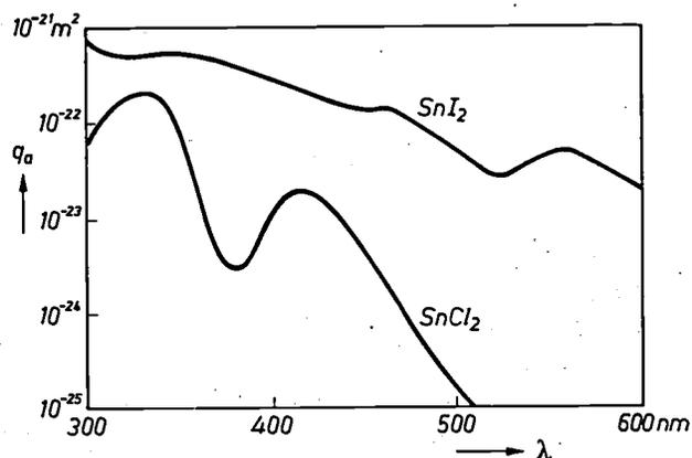
*Fig. 3.* Effective cross-section for photon absorption  $q_a$  of SnI<sub>2</sub> and SnCl<sub>2</sub> as a function of wavelength. The fact that the absorption of light by SnI<sub>2</sub> in the blue part of the spectrum is greater than in the red part is turned to advantage to give the colour temperature of the tin lamp a desired value.
