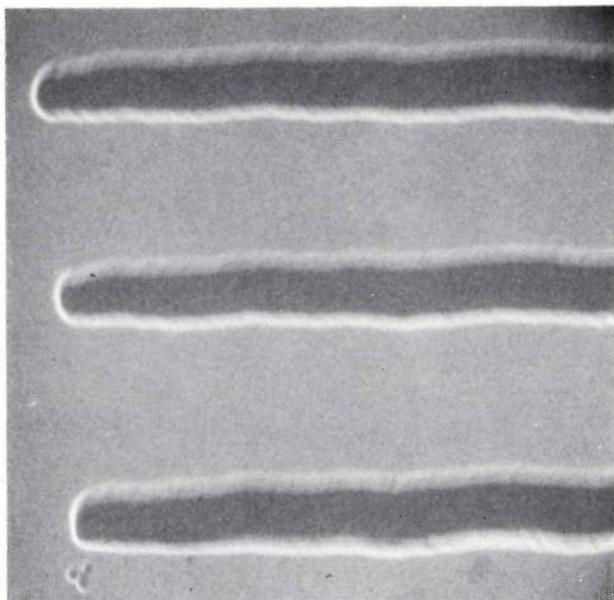
Fig. 4. Lines etched in a thermal-oxide film, the pattern being defined by a scanning electron-beam equipment in PMMA resist. Magnification 10 000  $\times$ . (Because the object was positioned obliquely in all the photographs reproduced in this article, the magnifications given are valid only for one direction, in this case the vertical direction.)
