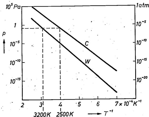
**Fig. 1.** The vapour pressure  $p$  of carbon and of tungsten, as functions of the reciprocal of the absolute temperature  $T$ . The vapour pressure of carbon is a summation over the vapour pressures of the molecular types  $C_2$ ,  $C_3$ ,  $C_4$ ,  $C_5$  and atomic carbon [1]. The vapour pressure of tungsten at 3200 K is approximately equal to that of carbon at 2500 K. The evaporation rate of the materials is directly proportional to their vapour pressure.
