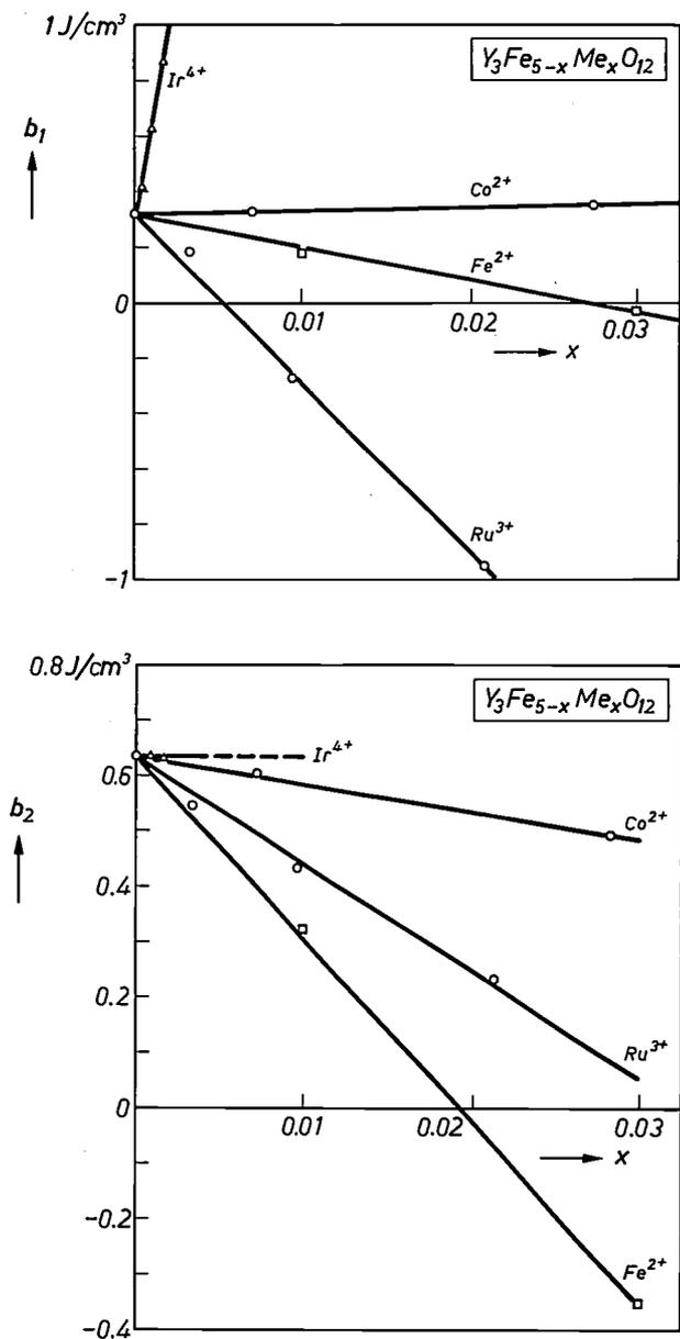
Fig. 4. The magnetoelastic constants  $b_1$  and  $b_2$  of  $Y_3Fe_{5-x}Me_xO_{12}$  at room temperature as a function of the concentration of strongly anisotropic Me ions. Me stands for  $Fe^{2+}$  [14],  $Co^{2+}$  [17]  $Ru^{3+}$  [23] or  $Ir^{4+}$  [24]. The magnetostriction constants  $\lambda_{100}$  and  $\lambda_{111}$  are related to  $b_1$  and  $b_2$  by  $\lambda_{100} = -0.41 \times 10^{-12} b_1$  and  $\lambda_{111} = -0.44 \times 10^{-12} b_2$ .
