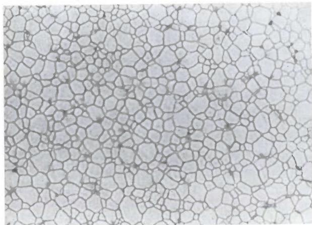
Fig. 4. Photomicrograph in reflected light of a wafer of the same material as in fig. 1 after isostatic hot pressing for two hours at 1170 °C in nitrogen at a pressure of 200 bars. The wafer has been thermally etched and polished. Magnification 800 $\times$ .
