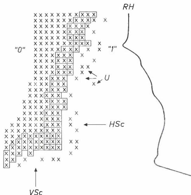
Fig. 5. The determination of the cardiac contour from a binary image field by searching for at least three successive '0' points (crosses). *U* '0' points caused by noise. *HSc* horizontal scan. *VSc* vertical scan. *RH* right half of the cardiac contour. The computer produces the binary field by application of a brightness threshold (*fig. 4*).
