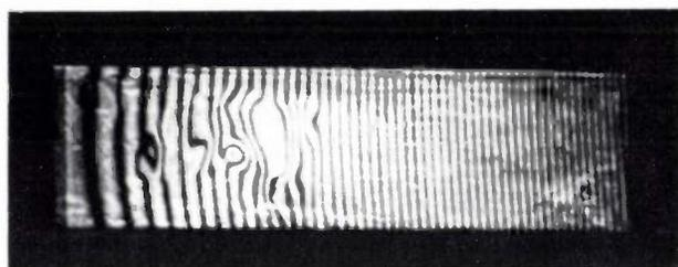
Fig. 7. Interference pattern on the double-hologram image of a bar with a weak spot. The bar is made up of two parts held together by adhesive, the plane of the joint lying in the plane of the paper. The irregularity in the interference fringes indicates a weak spot in the joint.
