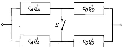
**Fig. 10.** Equivalent circuit (see *fig. 9*) of a ternary nickel alloy.  $c_A$  is the concentration of element A,  $c_B$  that of B. Matthiessen's rule is not valid here; it would only be valid if the switch *S* were closed, which it is not.
