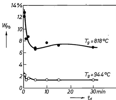
**Fig. 15.** Percentage weight of lead ( $W_{Pb}$ ) in YIG films grown on GGG substrates, as a function of the deposition time  $t_d$ , at two growth temperatures. The films were analysed with the aid of radioactive tracers.
