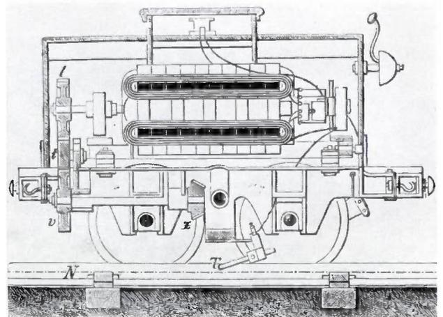
Fig. 20. Cross-sectional drawing of Siemens and Halske's electric locomotive (1879). A Siemens generator was used as the motor, and was coupled to the wheels by the gears *l*, *t*, *v*, *x*. The current was taken from a central live rail *N*.
