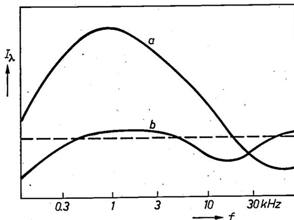
Fig. 6. Radiation output  $I_\lambda$  of a pulsed mercury discharge as a function of pulse frequency  $f$ . The outputs have been normalized to the output of a d.c. discharge at the same power (this level is indicated by a dashed line). Curve  $a$  gives the output at a wavelength of 436 nm, curve  $b$  the output at a wavelength of 254 nm.
