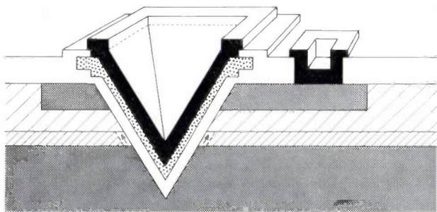
Fig. 6. Cross-section of a V-MOS transistor. The gate is deposited on the crystal faces of a V-shaped etch pit. The length of the channel (arrows) is determined by the thickness of the P-type layer.
