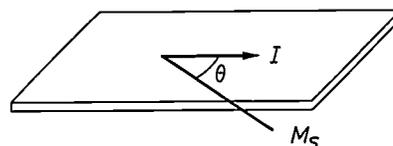
Fig. 1. The electrical resistivity of a specimen of a ferromagnetic metal depends, even at room temperature, on the angle  $\theta$  between the current  $I$  and the magnetization  $M_s$ . For a thin specimen (a film) the direction of  $M_s$  can be changed even by a weak field.
