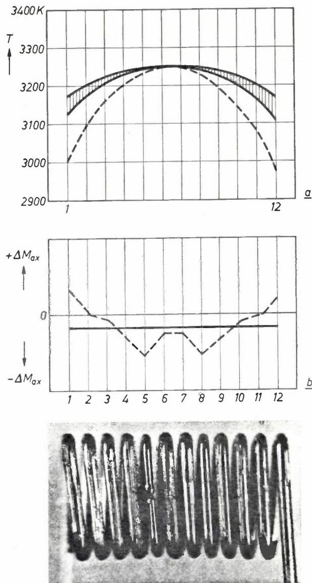
Fig. 1. Photograph of the filament in a projection lamp (12 V, 100 W) after about 80 hours of operation. Because of axial mass transport the greatest loss of material in the filament of this kind of lamp is not found at the centre, but in two turns symmetrically located on either side of it.
