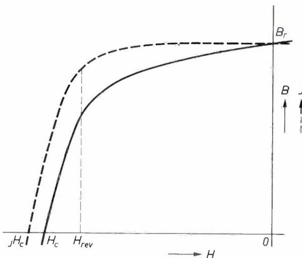
Fig. 2. Solid curve: demagnetization curve for a permanent magnet.  $B_r$  remanence.  $H_c$  coercive force. Dashed curve: corresponding variation of the magnetic polarization  $J$ .  $H_c$  field-strength at which the polarization  $J$  becomes zero.  $H_{rev}$  limiting field-strength for reversible demagnetization.
