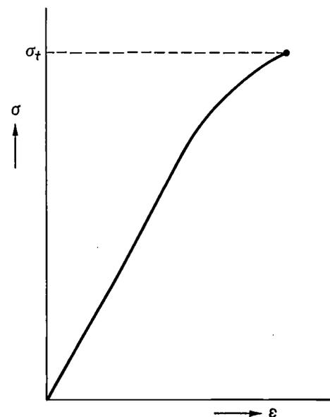
Fig. 1. The tensile stress  $\sigma$  as a function of the strain  $\epsilon$  (the 'stress-strain curve') of a test bar with a tensile load (schematic). The ratio  $\sigma/\epsilon$  in the linear initial part of the curve is the stiffness or Young's modulus  $E$  of the material. The tensile force at which the bar breaks, divided by the original cross-sectional area, is known as the tensile strength ( $\sigma_t$ ).
