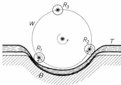
**Fig. 3.** The operating principle of the peristaltic pump. Three rollers *R*, mounted on bearings fastened to the wheel *W*, force liquid through the flexible tube *T* in the bed *B*. The pump is shown at the moment when *R*<sub>1</sub> has pinched the tube shut and *R*<sub>2</sub> has almost completely released pressure on it again.
