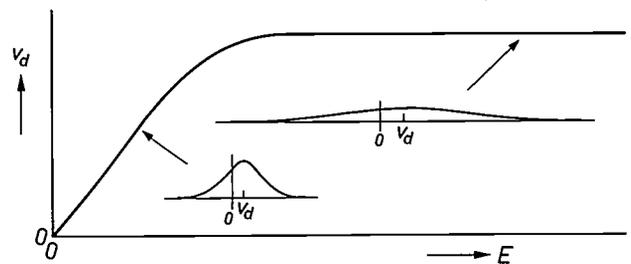
*Fig. 3*. Drift velocity  $v_d$  as a function of the field-strength  $E$  in the depletion layer. At low fields the relation between  $v_d$  and  $E$  is linear. As the field-strength is increased there comes a point where the drift velocity no longer increases with field-strength. The two inset diagrams show the distribution of actual velocities about the drift velocity (on a different scale) for two values of the drift velocity.
