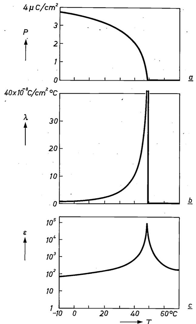
Fig. 5. The temperature dependence of the polarization  $P$ , the pyroelectric coefficient  $\lambda$  and the dielectric constant  $\epsilon$  for a crystal of pure TGS ( $\lambda = dP/dT$ ).
