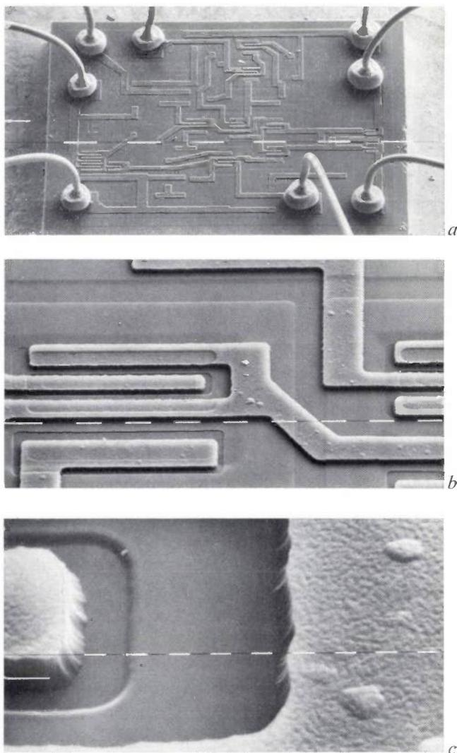
**Fig. 13.** Dashed line in the image to indicate the magnification. The relative position of the first dash indicates the length of the dashes. *a*) First dash above the line: dashes and spaces 100  $\mu\text{m}$ . *b*) First dash on the line: dashes and spaces 10  $\mu\text{m}$ . *c*) First dash below the line: dashes and spaces 1  $\mu\text{m}$ .
