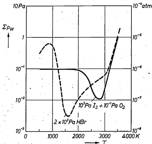
Fig. 1. Temperature dependence of the total effective tungsten pressure  $\Sigma p_w$  in a heterogeneous equilibrium system with  $I_2$  ( $10^3$  Pa) and  $O_2$  ( $0.1$  Pa) or with  $HBr$  ( $2 \times 10^3$  Pa).  $\Sigma p_w$  is the sum of the partial pressures of the gaseous tungsten compounds, when the number of tungsten atoms per molecule for each compound is taken into account.
