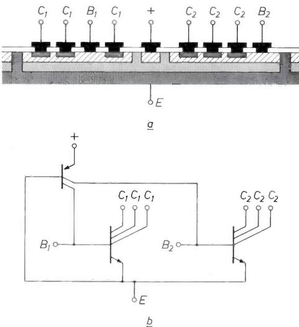
Fig. 11. *a*) Cross-section of two vertical *N-P-N* multicollector transistors based on the  $I^2L$  technique, combined with a lateral *P-N-P* transistor. The *N*-type region is the common emitter *E* of the vertical transistors; it is connected to the outside world via the  $N^+$  substrate. The *P*-type region connected to + is the emitter of the lateral *P-N-P* transistor. *b*) Schematic representation.
