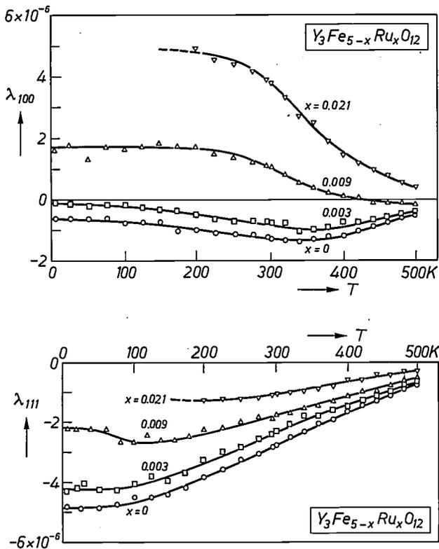
Fig. 13. Experimentally determined magnetostriction constants  $\lambda_{100}$  and  $\lambda_{111}$  for Ru-doped YIG as a function of temperature.
