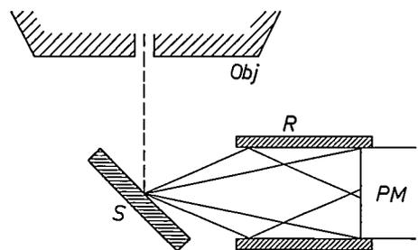
Fig. 7. The arrangement for cathodoluminescence experiments. *Obj* pole piece of the final lens of the scanning electron microscope. *S* sample. *R* reflecting screen. *PM* photomultiplier tube detecting the radiation resulting from electron bombardment of the sample.
