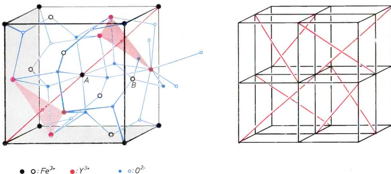
Fig. 1. Crystal structure of  $Y_3Fe_5O_{12}$  [3] (yttrium iron garnet or YIG). The diagram on the right shows a complete unit cell; the diagram on the left gives the details of an eighth part of the cell. The ordering of the ions in the complete cell is obtained when the octant on the left is made to overlap the octants on the right-hand figure so that the red diagonals coincide.
