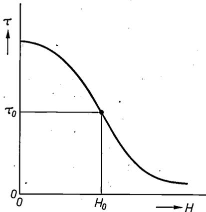
Fig. 3. Transmittance  $\tau$  of a photographic plate as a function of the exposure  $H$ . The exposure is the product of the intensity of the light and its duration. It is preferable to work only on the linear part of the curve, near the point of inflexion  $(H_0, \tau_0)$ .
