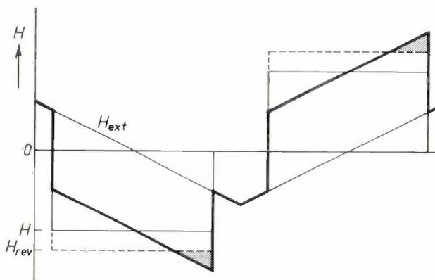
Fig. 3. Schematic developed view of a d.c. motor with permanent-magnet stator.  $N$  north pole.  $S$  south pole. The magnetic field  $H_{ext}$  excited by the rotor is added to the magnet's own demagnetization field  $H$  in the magnet. In the shaded region, the sum of these two fields exceeds the limiting field-strength  $H_{rev}$ .
