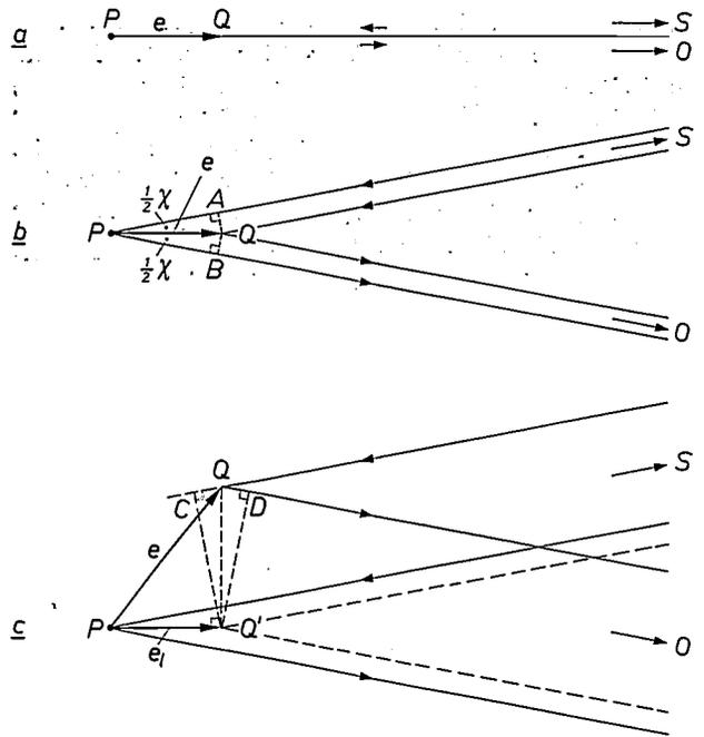
Fig. 5. Calculation of the change  $\Delta l$  in the optical path length between source  $S$  and observer  $O$  via a point in the surface of the object when this point is displaced from  $P$  to  $Q$ .
