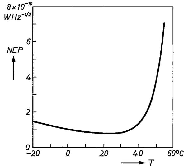
Fig. 18. The temperature dependence of the noise equivalent power  $NEP$  for a pyroelectric infrared detector with an l-alanine-doped mixed triglycine sulphate/selenate crystal: 70% sulphate, 30% selenate. Electrode area  $0.25 \text{ mm}^2$ , measurements made at 12.5 Hz.
