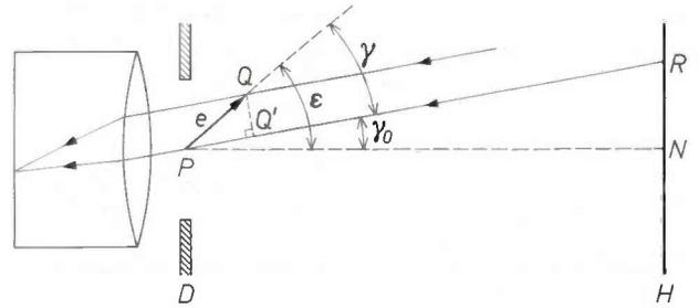
Fig. 10. Calculation of difference in optical path length from the interference pattern seen (fig. 9c) on the hologram  $H$  via the diaphragm  $D$ .  $P$  is the initial point and  $Q$  the final point of the displacement vector  $e$  at a certain location in the real image. An interference pattern is observed on the hologram because the difference  $PQ'$  in optical path length depends on the viewing direction  $PR$ .
