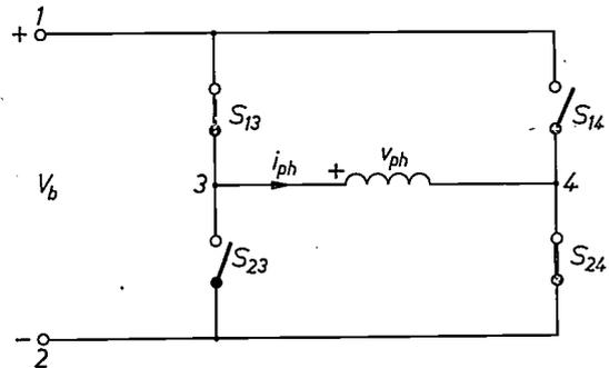
Fig. 1. Schematic circuit diagram for one phase winding of an electronically commutated d.c. machine.  $V_b$  supply voltage.  $v_{ph}$  voltage across phase winding.  $i_{ph}$  armature current in phase winding.  $S$  electronically controlled switches.
