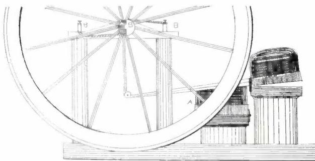
Fig. 15. Wright's motor (1840). The output stroke is again magnified by a lever; the armatures are hinged to the edge of the electromagnet.
