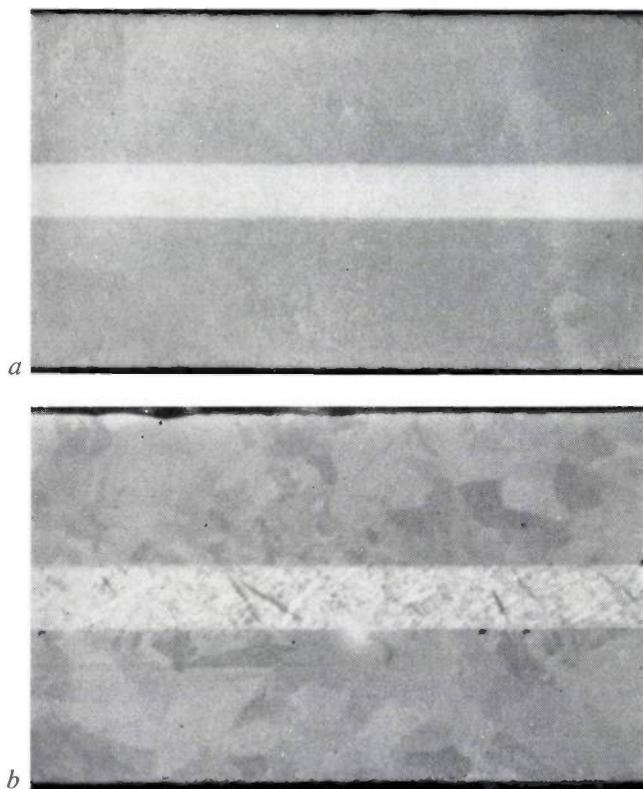
Fig. 6. *a*) Longitudinal section through a boron filament in which the boron is amorphous. *b*) As (*a*), but with crystalline boron. Strong filaments are invariably amorphous. Filaments of crystalline boron are weak. The sections were photographed with a polarizing microscope, which makes the structure in (*b*) visible.
