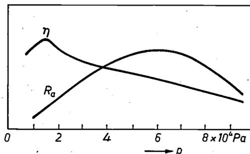
*Fig. 10.* Luminous efficacy  $\eta$  and general colour-rendering index  $R_a$  of a high-pressure sodium lamp (SON 400 W) as a function of the sodium pressure  $p$  <sup>[9]</sup>.
