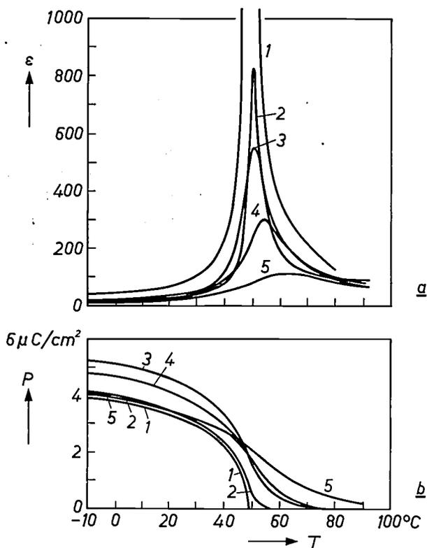
Fig. 8. The temperature dependence of the dielectric constant  $\epsilon$  and the polarization  $P$  for crystals of pure TGS (curve 1) and of alanine-doped TGS crystals grown from solutions containing 10 (curve 2), 20 (curve 3), 40 (curve 4) and 60 (curve 5) mol% of l-alanine respectively.
