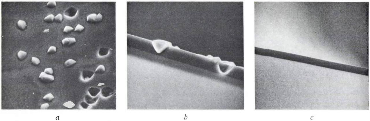
**Fig. 13.** Surface (*a*) and cross-section (*b*) of a film that has been grown at too high a degree of supersaturation. As a result individual crystals have formed on the film. *c*) Cross-section of a film made at a lower degree of supersaturation. These photomicrographs were made with a scanning electron microscope; magnification 2000 $\times$ . (Photograph J. L. C. Daams.)
