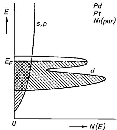
Fig. 7. Energy diagram of a transition metal (for Pd, Pt or Ni above the Curie temperature, i.e. paramagnetic). The situation is very similar to that of fig. 6, except that the d band is now not filled.
