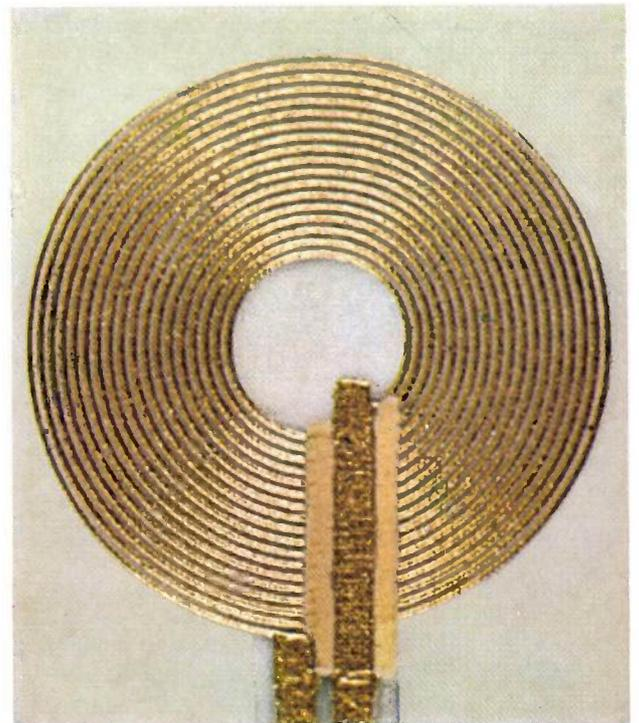
Fig. 5. FM modulation coil for a 2- to 3-GHz oscillator with YIG tuning. The gold spiral conductor is 60  $\mu\text{m}$  thick and 100  $\mu\text{m}$  wide, with a gap of 150  $\mu\text{m}$  between the turns.
