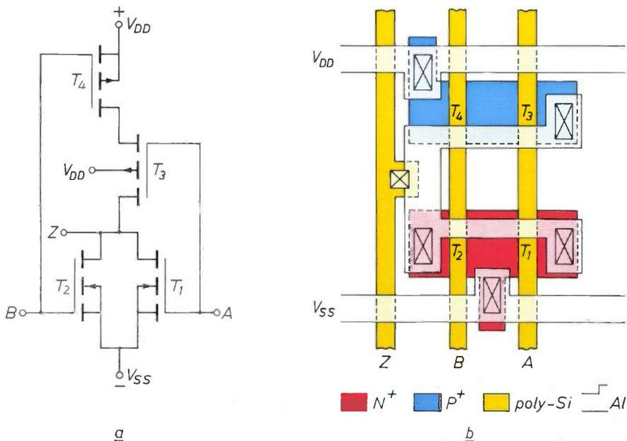
Fig. 7. NOR gate with complementary MOS transistors. Four transistors are required. a) Circuit diagram. b) Layout. Transistors  $T_1$  and  $T_2$  are formed in a P-type island but because of the LOC MOS technology employed this is not visible in the layout.
