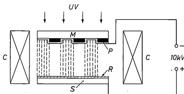
Fig. 2. Schematic diagram of a projection electron-beam apparatus using a photocathode. Ultraviolet light passes through a mask *M* with appropriate opaque areas on the photocathode *P*. Magnetic coils *C* produce an image of the pattern on the substrate *S*, which acts as an anode and is coated with electron resist *R*.
