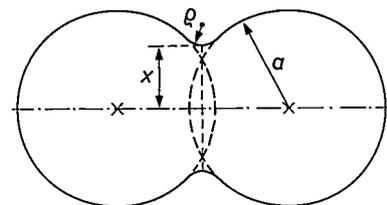
Fig. 10. In the initial stage of the sintering process neighbouring particles are bonded to one another through the formation of 'necks' (A. L. Stuijts [40]). The neck shown here has a radius of  $x$ , and the two particles are assumed to be spherical and of radius  $a$ . The surface of the neck has a radius of curvature  $\rho$ .
