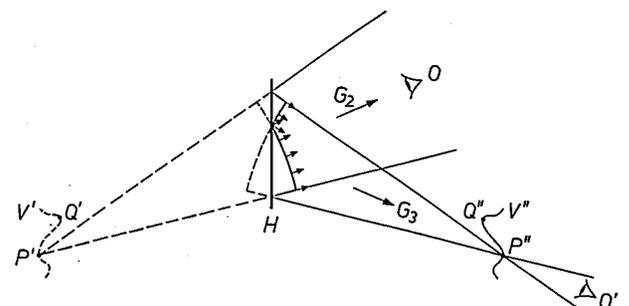
Fig. 4. Close to the hologram, the wavefronts in the beams  $B$  (or  $G_2$ ) and  $G_3$  of fig. 1 are mirror images of each other with respect to the plane of the hologram. Rays in  $G_2$  diverging from the points  $P'$  and  $Q'$  correspond to rays in  $G_3$  which converge to the corresponding points  $P''$  and  $Q''$ ; the virtual image  $V'$  thus corresponds to the real image  $V''$ .
