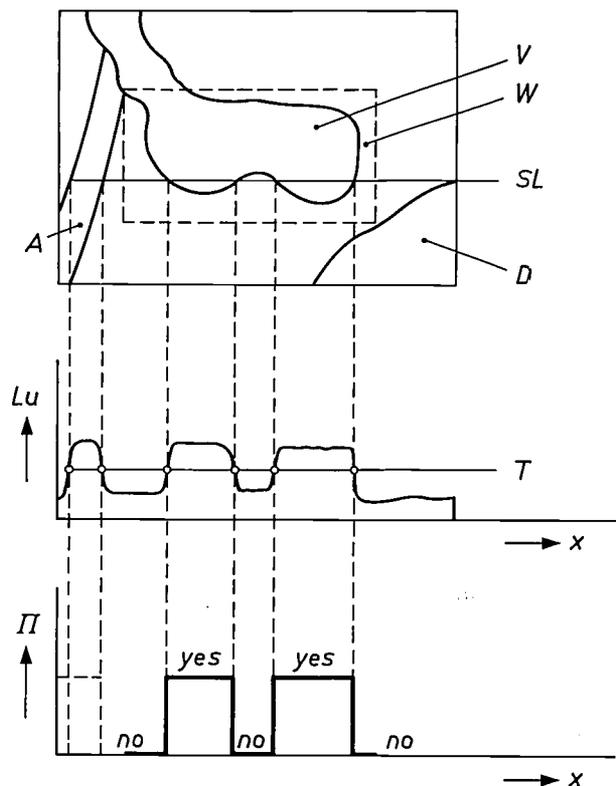
**Fig. 2.** Area measurement of a left ventricle ( $V$ ) from a video signal ( $Lu$ ). The threshold  $T$  and the window  $W$  can be adjusted manually.  $SL$  scan line.  $D$  diaphragm.  $A$  aorta. The logic signal  $\Pi$  indicates whether the object sought is present (yes) or not (no).  $x$  space coordinate. The signal from the aorta does not cause an error since it appears outside the window.
