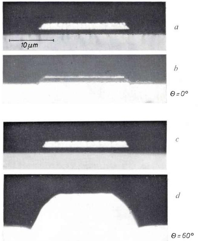
Fig. 16. Sections through 1.5- $\mu\text{m}$  titanium masks deposited on thermally oxidized silicon wafers. (a) and (c) show the situation before etching (b) the situation after etching vertically to the substrate surface and (d) after etching at an angle of  $60^\circ$ . The cross-sections clearly demonstrate the much greater etch depth (about 6  $\mu\text{m}$ ) that is obtainable in the last case.
