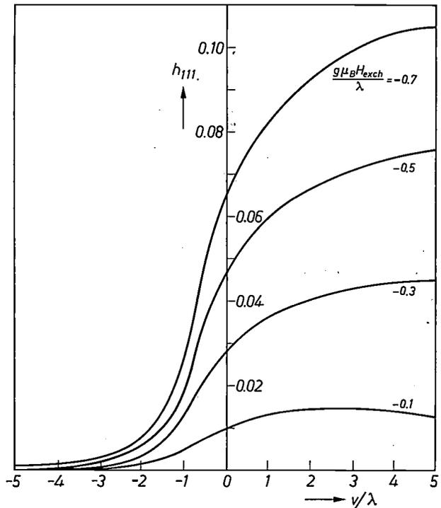
Fig. 12. Theoretical value of  $h_{100}$  and  $h_{111}$  for low-spin  $d^5$  ions at octahedral sites at  $T = 0 \text{ K}$  as a function of the ratio  $v/\lambda$ . The magnetostriction constants  $\lambda_{100}$  and  $\lambda_{111}$  are proportional to  $h_{100}$  and  $h_{111}$  respectively (see eq. 21).
