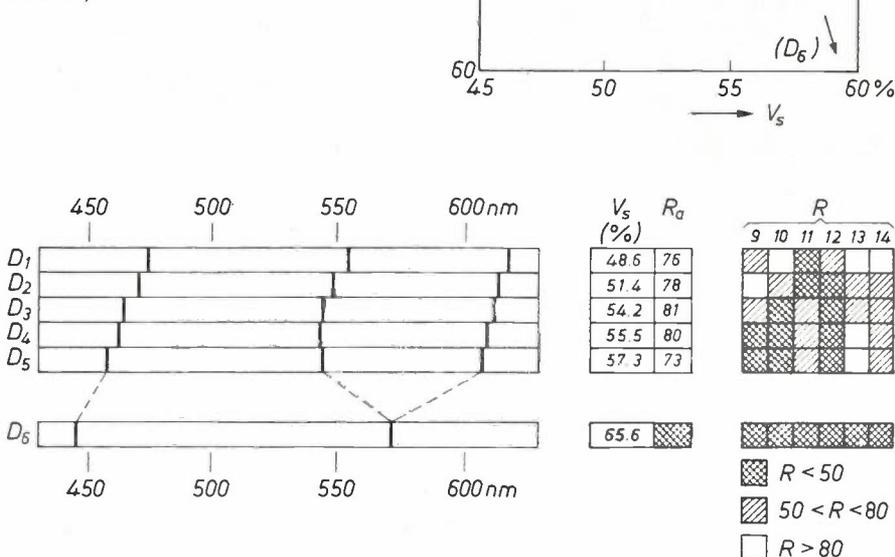
**Fig. 8.** *Right:*  $R_a$ - $V_s$  curves for the optimum three-line spectra at the chromaticities of six different CIE reference sources. *Below:* Optimum spectra and values of  $V_s$ ,  $R_a$ ,  $R_9$  to  $R_{14}$  corresponding to the maxima in the upper figure.
