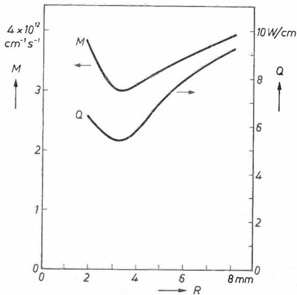
Fig. 3. A calculation of the number of tungsten atoms  $M$  leaving the filament per second, and the heat flow  $Q$  (both per unit of length) in axially symmetric argon-filled lamps as a function of the radius  $R$  for an argon pressure of  $10^6$  Pa (10 atm), a wire diameter of 1 mm and a wire temperature of 3200 K. The curves show a minimum at  $R \approx 3$  mm.
