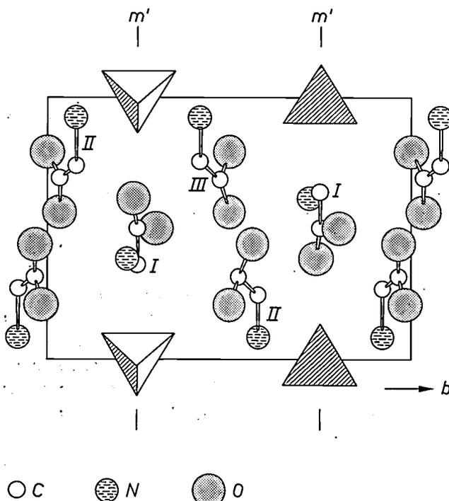
Fig. 4. Schematic structure of a triglycine-sulphate (TGS) crystal, seen along the  $c$ -axis. Glycine molecules occur at three different positions (indicated by  $I$ ,  $II$  and  $III$ ). The sulphate ions are represented schematically by tetrahedra. All the hydrogens have been omitted.  $m'$  represents the sets of pseudo mirror planes in which glycine- $I$  molecules are inverted on ferroelectric switching.
