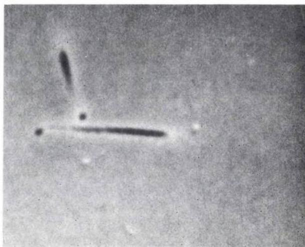
Fig. 10. Luminescence image of an Si-doped GaAs sample. Here again the dislocations are decorated. The segregation-free border is narrower than with GaAs; segregations are much smaller in size and are consequently not visible individually. Magnification 900 $\times$ .
