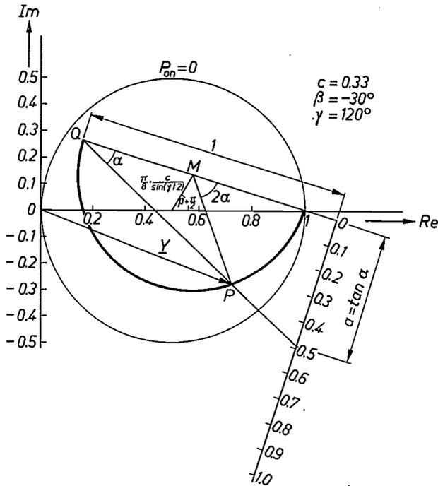
Fig. 8. Locus diagram of the quantity  $\underline{Y}$  in the complex plane;  $\underline{Y}$  is the normalized r.m.s. value of the fundamental component of the current. The working point  $P$  describes the semicircle from  $(1, 0)$  to  $Q$  as the normalized speed  $a$  runs from 0 to  $\infty$ . This speed  $a = \tan \alpha$  can be read off the scale. This curve refers to the same motor as curve 4 in fig. 5.
