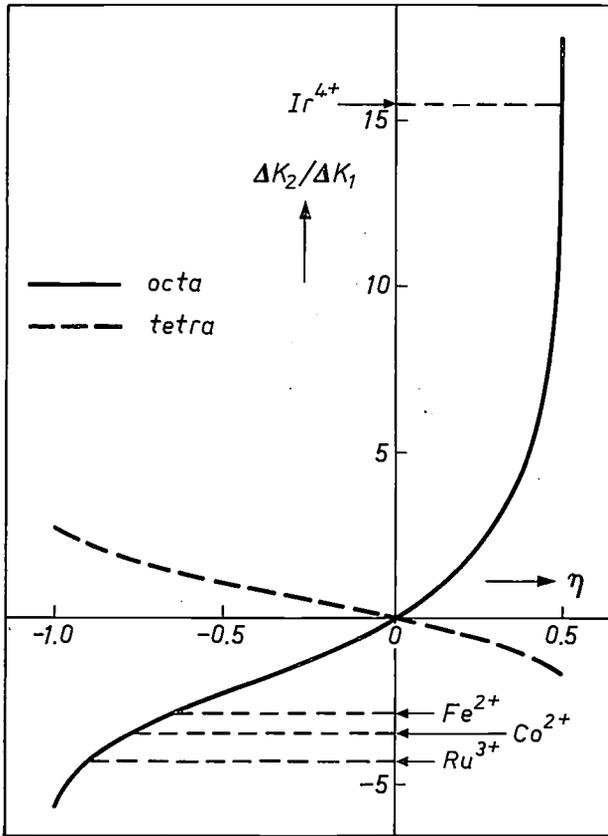
Fig. 9. Theoretical plot of  $\Delta K_2/\Delta K_1$  at low temperature for an ion with a doublet ground state given by eq. (14), as a function of the parameter  $\eta$ . The experimentally determined values of  $\Delta K_2/\Delta K_1$  for strongly anisotropic ions are indicated. The value of  $\eta$  for low-spin  $d^5$  ions is related in a simple way to  $v/\lambda$ . The figure is also valid for any ion with a ground state as given by eq. (14).
