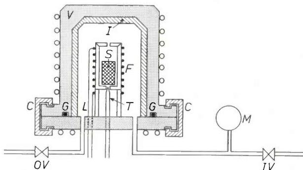
**Fig. 3.** Schematic cross-section of our apparatus for isostatic hot pressing. *V* water-cooled pressure vessel with sealing clamps *C* and gasket *G*. *I* heat insulation. *F* electric furnace. *S* ceramic sample. *T* thermocouple. *L* supply leads for the heating elements. *IV* gas inlet valve. *M* manometer. *OV* gas outlet valve.
