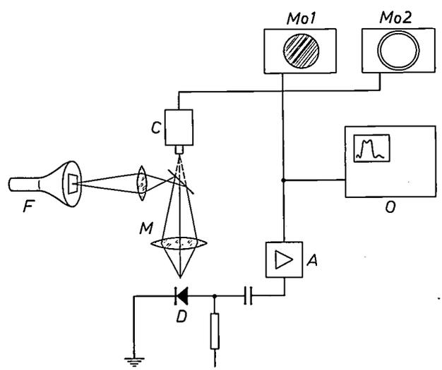
*Fig. 4*. Block diagram of the flying-spot microscope.  $F$  flying-spot scanning tube.  $M$  optical microscope.  $D$  diode under investigation.  $A$  amplifier for photocurrent.  $C$  television camera for observation of optical image.  $Mo1$  monitor for display of the distribution of the multiplication factor over the diode surface.  $Mo2$  monitor for display of the optical image.  $O$  oscilloscope for the display of the diode signal for one line of  $Mo1$ .
