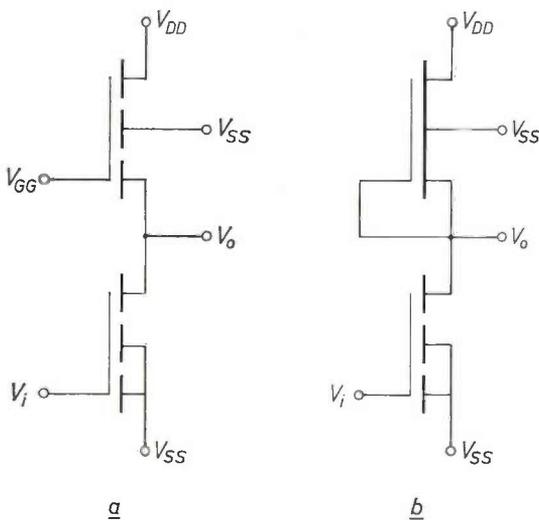
**Fig. 4.** Inverter circuit, *a*) with two MOS transistors of the enhancement type, *b*) with a depletion-type transistor as load. The shift in the threshold voltage of this depletion-MOS transistor was achieved by ion implantation.
