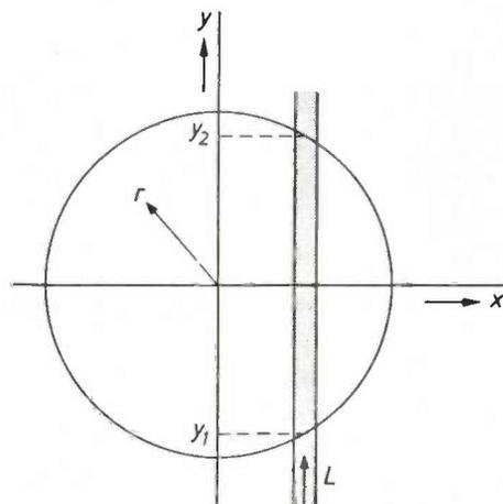
Fig. 1. Optical absorption measurement, schematic. The circle represents the gas discharge in cross-section.  $L$  laser beam. The quantity measured is the absorption integrated over  $y$  from  $y_1$  to  $y_2$ . If this integral is measured accurately enough as a function of  $x$  and given complete cylindrical symmetry, the absorption can be derived from it as a function of  $r$  by an Abel inversion. This procedure, however, may lead to considerable errors in the final result.
