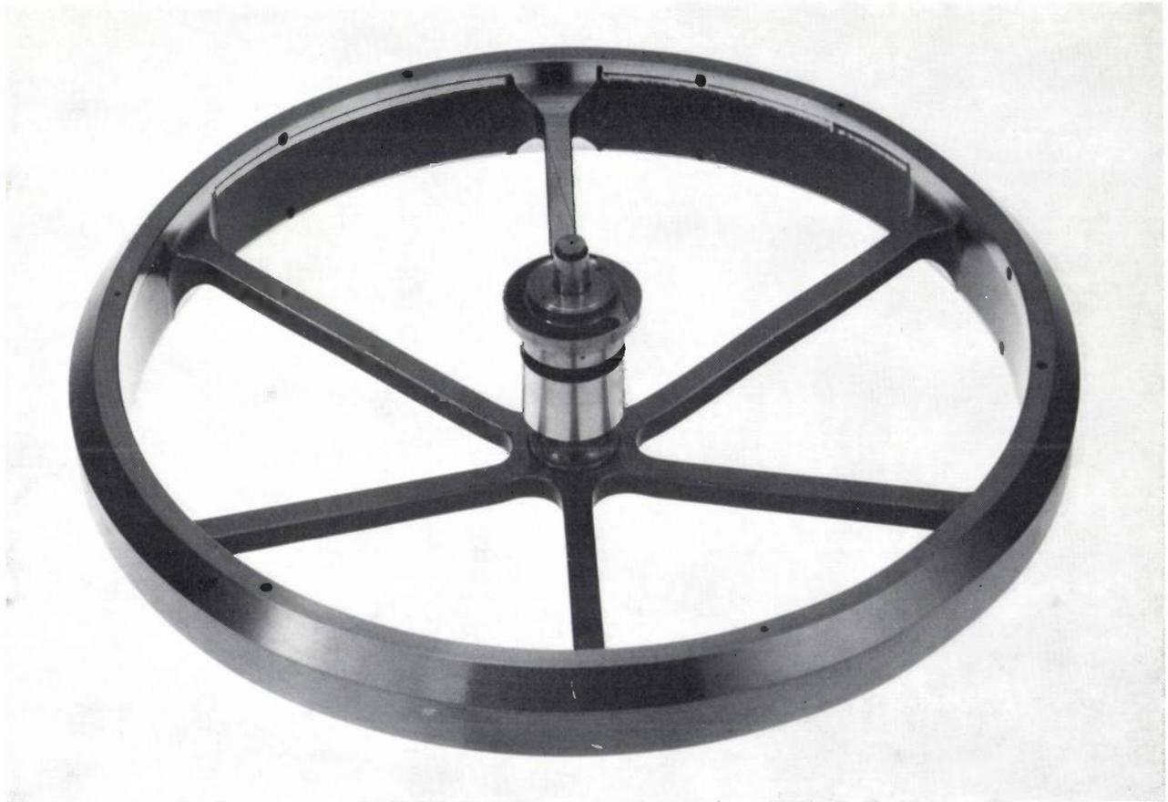
Fig. 2. A 'flywheel' for attitude stabilization of a space vehicle. The shaft is fixed to the vehicle and the bearing bush supports the wheel. The drive motor is not illustrated.
