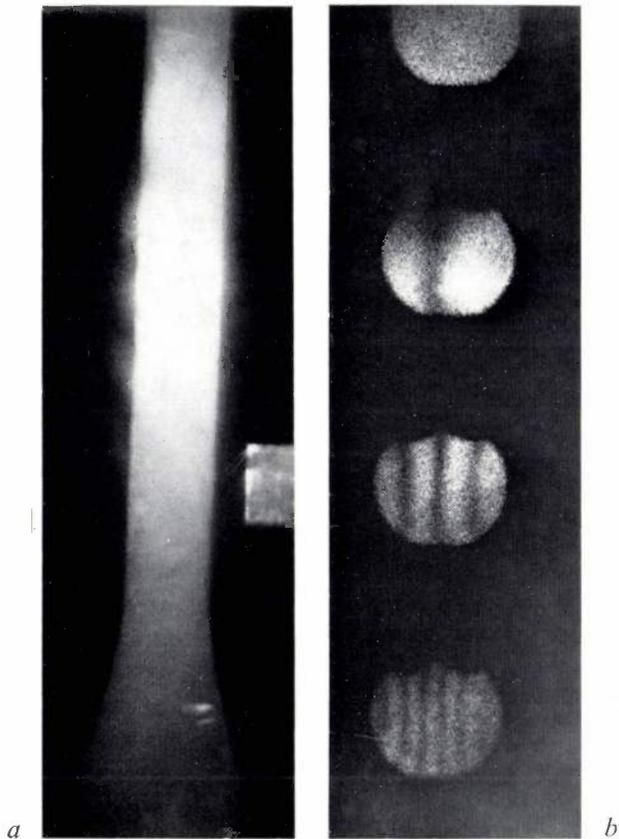
Fig. 11. Measurement of the lateral displacement of a bar subjected to a lateral force. *a*) Double-holographic image of the bar. The bar is clamped at the upper end and the force acts from left to right on the lower end. *b*) Interference patterns observed through a diaphragm of 0.5 mm diameter in the real image. The positions of the fields in (*b*) correspond to those in (*a*). The rather coarse speckle pattern in (*b*) is due to the small aperture (see caption to fig. 2).
