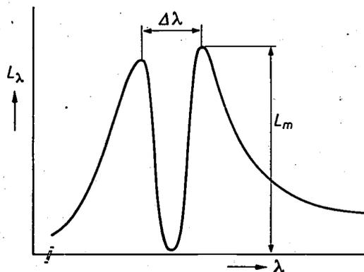
Fig. 5. Profile of a self-reversed spectral line. The difference in wavelength  $\Delta\lambda$  between the two maxima in the case of a resonance line is a measure of the particle density of the atoms in the ground state. In the case of a non-resonant line the maximum radiance  $L_m$  is a measure of the maximum temperature in the direction of observation.
