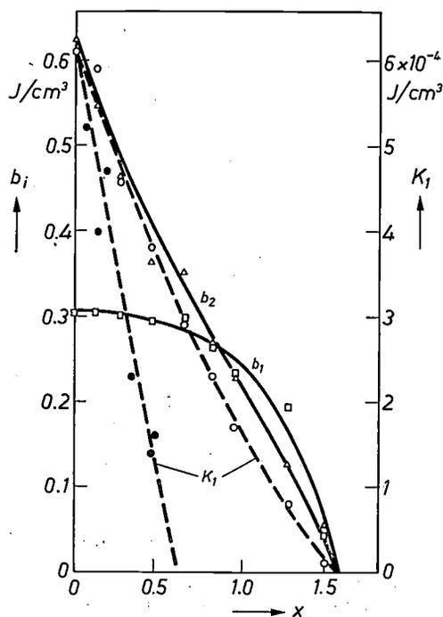
Fig. 2. The anisotropy constant  $K_1$  (right-hand scale) and the magnetoelastic constants  $b_1$  and  $b_2$  (left-hand scale) at room temperature, as a function of the quantity  $x$  of diamagnetic ions (Me) in  $\text{Y}_3\text{Fe}_{5-x}\text{Me}_x\text{O}_{12}$ . Me stands for In (points) [11] [12], which replaces  $\text{Fe}^{3+}$  at octahedral sites, or Ga (circles) [10], which mainly replaces  $\text{Fe}^{3+}$  at tetrahedral sites.
