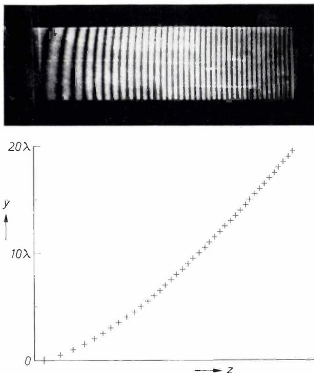
Fig. 6. Above: Example of an interference pattern on the image of a bar deformed under load (obtained from a double hologram). Below: Displacement  $y$  as a function of position  $z$  along the bar, derived from the interference pattern. Each fringe represents an increment of the displacement of  $\lambda/2$ .
