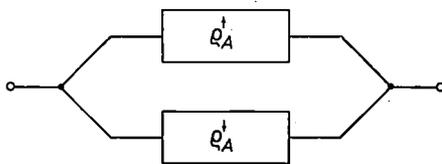
**Fig. 9.** The residual resistivity of a binary ferromagnetic alloy (metal A in nickel) in the two-current model. When electrons are scattered by the A atoms (the origin of the residual resistivity) the spin orientation remains unchanged, so that two kinds of moving electrons may be distinguished, each of which experiences resistance. The corresponding resistivities are denoted by  $\rho_A^\uparrow$  and  $\rho_A^\downarrow$ . These resistivities are sometimes very different.
