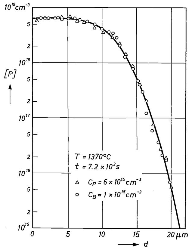
Fig. 1. A concentration profile for phosphorus in silicon, for both *P*-type material (the triangles) and *N*-type material (the circles). The horizontal scale indicates the distance  $d$  travelled by the diffusion, which started at the surface. The heat treatment was the same in both cases. The diffusion time and temperature are shown in the figure, and also the concentrations of the charge carriers in the starting material. (After R. N. Ghoshtagore [2].)
