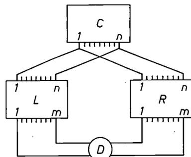
Fig. 1. Testing a simple logic circuit with  $n$  inputs and  $m$  outputs. A counter  $C$  generates the test patterns and simultaneously feeds them to the inputs of the circuit under test  $L$  and to a calibration circuit  $R$ . The output signals are fed to a comparator circuit  $D$ , which delivers a signal when the two responses are not identical.
