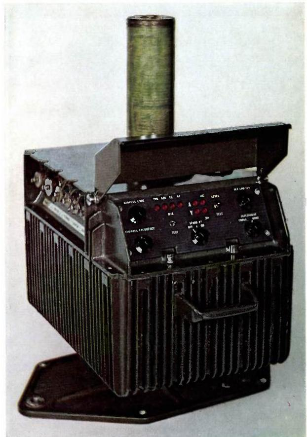
**Fig. 4.** The ground transponder (early military prototype). It weighs 20 kg and can withstand parachute dropping and manhandling over rough terrain. The control panel is seen at the front. The cylindrical omnidirectional antenna is mounted on top.
