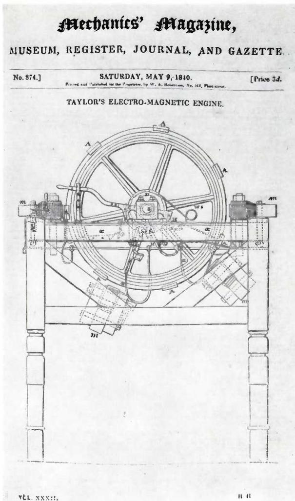
Fig. 12. Taylor's motor (1840). The rotor is a wooden wheel with seven soft-iron armatures *A*. Four electromagnets *m* are connected and disconnected in turn.
