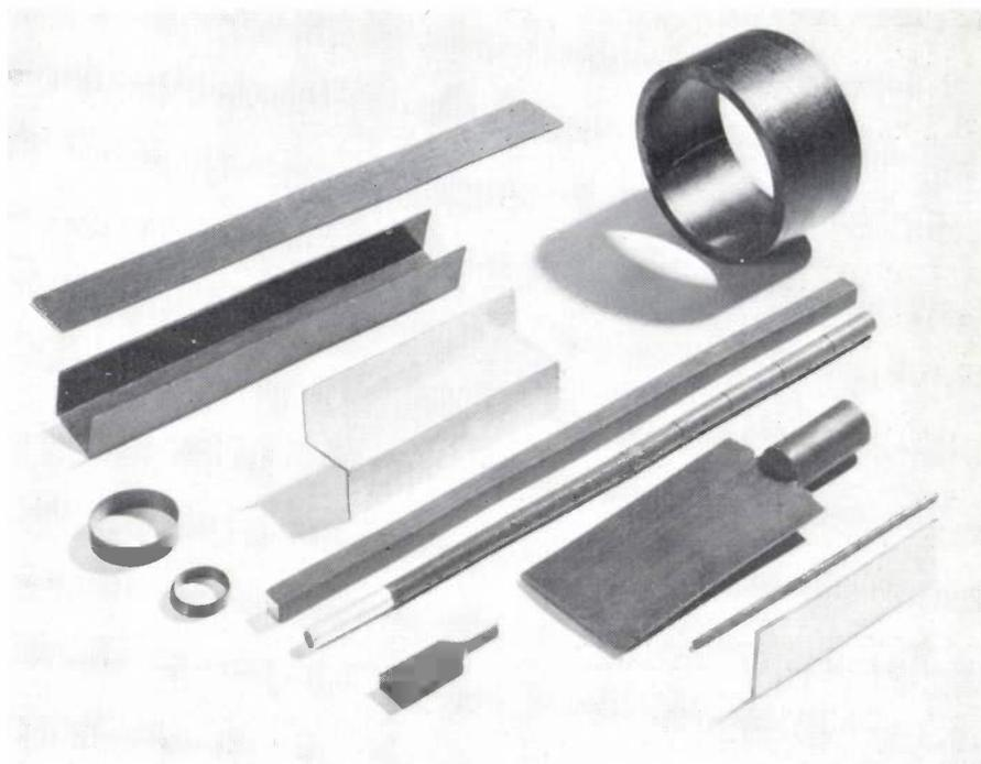
a laminate is obtained that is extremely strong and rigid in one direction. The strength and stiffness can be 'spread' over a range of directions by stacking the successive pre-pregs with their filaments at an angle, usually a right angle. Since the pre-pregs are very flexible, laminates of a great variety of shapes can be made from them (*fig. 14*).
