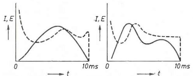
Fig. 14. Current  $I$  and field-strength  $E$  for a low-pressure sodium lamp (current : solid curve, field-strength : dashed curve). a) For a lamp connected to the conventional autoleakage transformer. b) For a lamp connected to the new ballast shown in fig. 13.
