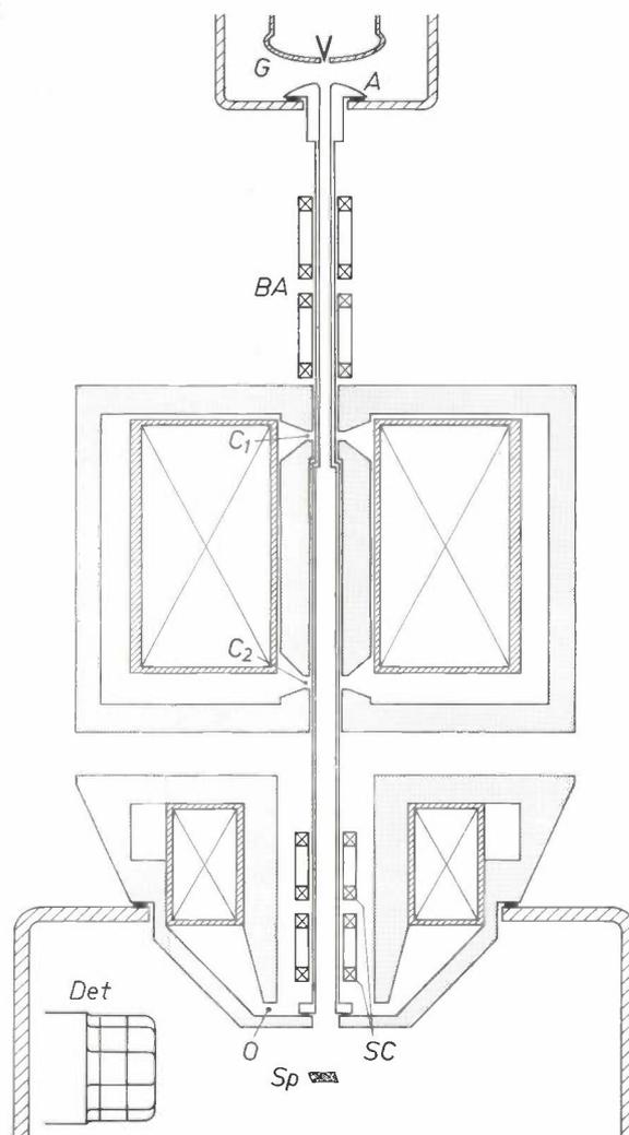
Fig. 2. Diagram of a scanning electron microscope (SEM). *G* electron gun. *A* anode. *BA* beam-alignment coils. *C*<sub>1</sub>, *C*<sub>2</sub> double condenser lens. *O* objective. *SC* scanning coils that produce the raster. *Sp* specimen. *Det* detector for secondary electrons. The vacuum chamber is enclosed by the wall of the emission chamber (which also includes the gun), the demountable inner lining of the electron-optical column and the wall of the specimen chamber.
