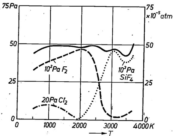
Fig. 4. The solid curve gives the total effective tungsten pressure in a heterogeneous equilibrium system with  $\text{SiF}_4$  ( $10^3 \text{ Pa}$ ),  $\text{F}_2$  ( $10^2 \text{ Pa}$ ) and  $\text{Cl}_2$  ( $20 \text{ Pa}$ ). The other curves refer to the corresponding systems with  $\text{SiF}_4$  or  $\text{F}_2$  or  $\text{Cl}_2$  separately.
