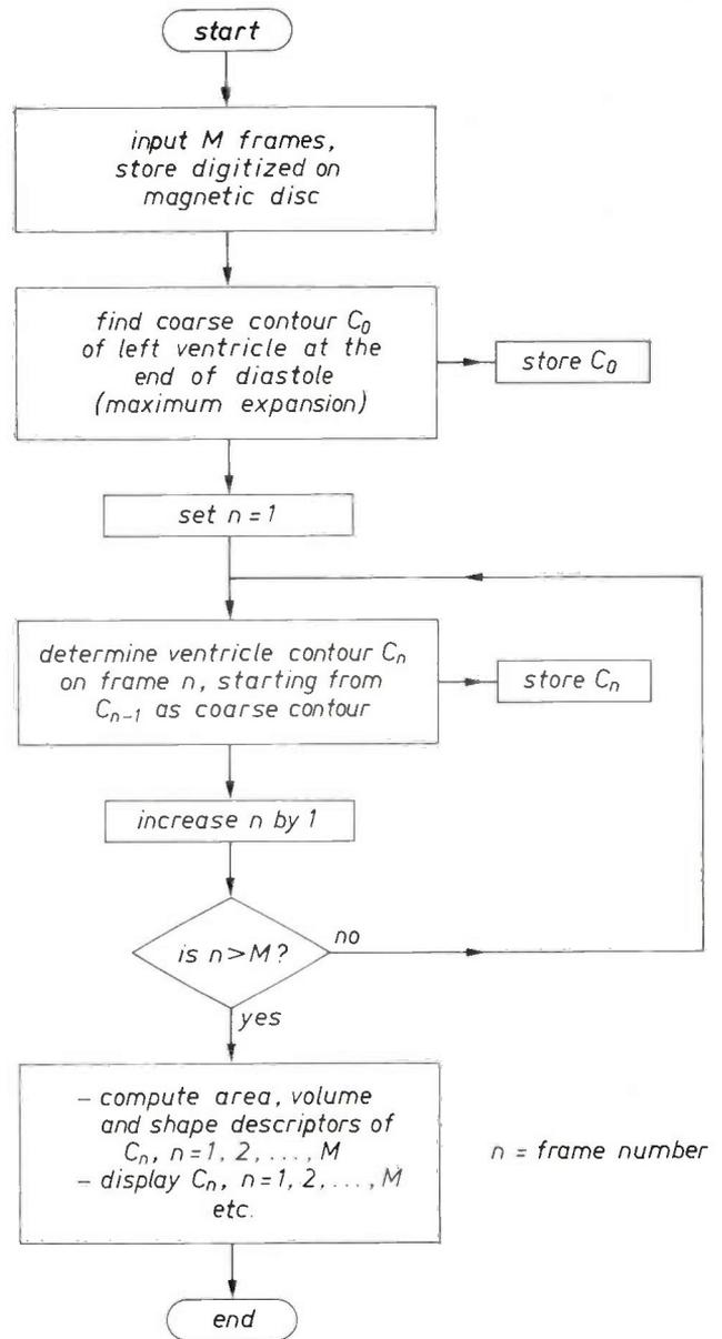
Fig. 11. Block diagram of the method for automatic determination of a left cardiac ventricle. The input information is on *M* X-ray frames; *n* is the frame number. The first step in the procedure is the coarse search; the high-resolution search occurs in the second, iterative step.
