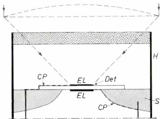
Fig. 13. Schematic cross-section of the optical unit of a pyroelectric infrared detector. *Det* wafer of a pyroelectric crystal. *EL* evaporated metal electrodes. *S* ceramic substrate, with aperture a little larger than the electrodes. *H* housing. *W* window. The electrodes are connected via strips of conducting paint *CP* to the input leads of an amplifier stage. The detector is usually used in combination with an optical system, e.g. a lens (as shown here) or an array of slits.
