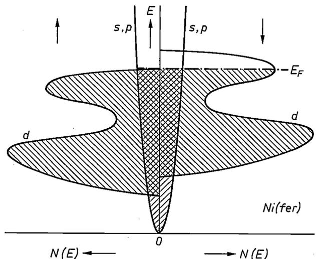
Fig. 8. Energy diagram of a ferromagnetic transition metal (Ni). The two possible orientations of the electron spins make it necessary to regard the band as split into two sub-bands. Even in the absence of a magnetic field these two sub-bands are not equally filled (see fig. 3b). The two s, p sub-bands remain to a first approximation equally filled.
