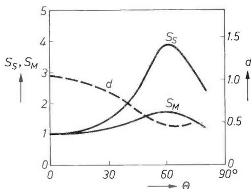
Fig. 15. The sputtering rates  $S_S$  and  $S_M$  of the substrate and mask materials as a function of the angle of incidence  $\theta$ , normalized for vertical incidence. Curve  $d$  is the relative depth, as calculated from  $S_S$  and  $S_M$ , which is necessary to obtain a certain etch depth. It can be seen that to attain this objective with the thinnest possible mask the angle of incidence must be about  $60^\circ$ .
