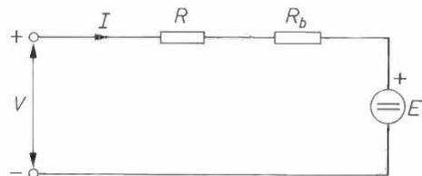
Fig. 3. Equivalent circuit of the d.c. motor.  $V$  supply voltage.  $I$  supply current.  $R$  diametral rotor resistance.  $R_b$  commutator resistance.  $E$  speed voltage (back e.m.f.) induced in the rotor coils.
