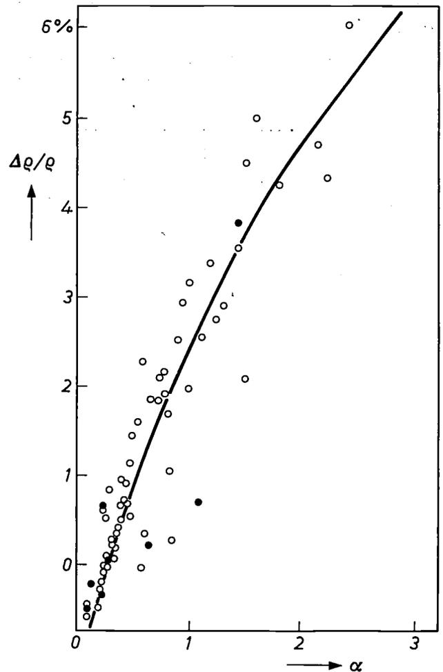
Fig. 12. The resistance anisotropy (see eq. 4) of nickel alloys at 4.2 K plotted as a function of  $\alpha$ , i.e. the ratio of the resistivities in the two sub-bands (see eq. 5). The circles refer to ternary alloys, the black dots to binary alloys. The measured points agree only approximately with the predictions from eq. (6).
