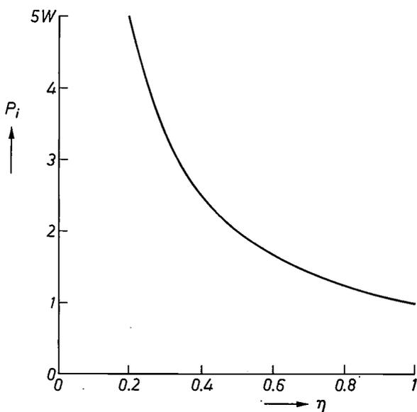
Fig. 6. The mechanical power  $P_i$  to be supplied for an output power of 1 watt, plotted against the efficiency  $\eta$ . The higher the efficiency, the less power can be gained by increasing the efficiency further.
