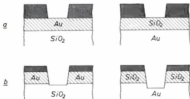
Fig. 5. Specimens consisting of a mask and a layer of gold (left) or SiO<sub>2</sub> (right) which has to be etched away from a substrate of SiO<sub>2</sub> or gold, a) before etching, b) after etching. The unwanted but unavoidable etching of the substrate is much deeper in the specimen on the right, because the etch rate of gold is higher than that of SiO<sub>2</sub>.
