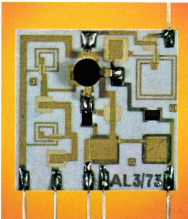
**Fig. 2.** Highpass UHF filter (Valvo GmbH). Two resistors (black), three inductors ( $\text{Al}_2\text{O}_3$ ;  $25 \times 25$  mm). The conductor leads cross at three places. A UHF transistor and six connecting leads can be seen attached to the substrate. The conductors and inductors are gold, the connector pads, the letters and numbers and the connections to the resistors are platinum/gold. Six printings and two firings were required in making this circuit.
