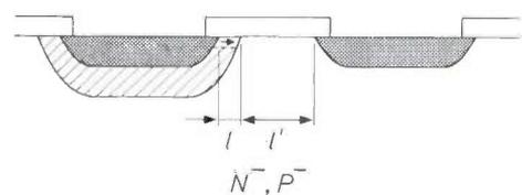
**Fig. 5.** Cross-section of a MOS transistor made with the aid of double diffusion (D-MOS technology). The length  $l$  of the channel equals the difference in lateral depth between the *P* and the  $N^+$  diffusions. There is a drift region of length  $l'$  next to the channel.
