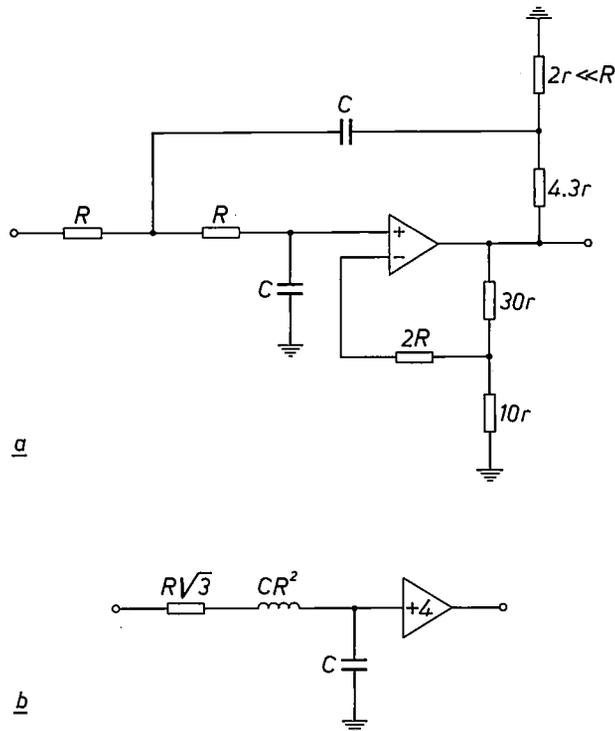
Fig. 16. Second-order Bessel lowpass filter [4]. This filter reduces digital noise in the velocity output and has a fast settling time without overshoot. Only two component values ( $R$  and  $C$ ) are used to fix the frequency-scale factor. With  $R = 220 \text{ k}\Omega$  and  $C = 1 \text{ }\mu\text{F}$  the half-power cut-off frequency is 0.57 Hz. a) Complete circuit diagram, b) equivalent circuit.
