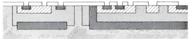
**Fig. 14.** Cross-section of an I<sup>2</sup>L circuit in which the use of a seven-mask technique makes N-type islands with a P<sup>+</sup> insulation (left) available for other forms of logic or analog circuits.
