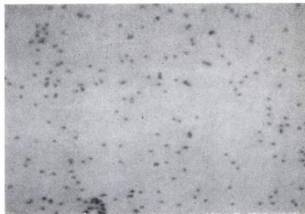
**Fig. 15.** Luminescence image of the surface of an epitaxial GaAsP-layer on a GaAs substrate. A low dislocation density has been obtained by careful adjustment of the gradients in the transition zone. Magnification  $160\times$ .
