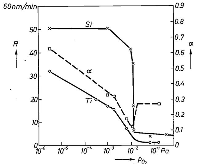
Fig. 13. The etch rates  $R$  of titanium and silicon and their ratio  $\alpha$  as a function of the partial pressure  $p_{O_2}$  of the oxygen added to the argon in which ion etching is performed. It is clear from the figure that for a given thickness of the titanium mask the largest etch depth in silicon is obtained for an oxygen pressure of about  $10^{-2}$  Pa.
