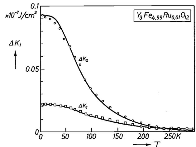
Fig. 11. Temperature dependence of the contribution  $\Delta K_i$  to the anisotropy from  $\text{Ru}^{3+}$  ions in YIG. The curves show the theoretical relation for  $v/\lambda = 1$  and  $gH_{\text{exch}} = 9.5 \times 10^8 \text{ A/m}$  ( $1.2 \times 10^7 \text{ Oe}$ ).
