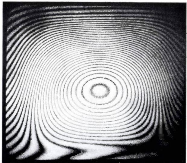
**Fig. 14.** Tests on a cathode-ray tube. The screen of the tube is cemented to the body of the tube. A double-holographic image can show whether a good adhesion has been achieved. The tube shown here has a weak spot on the lower edge. The mechanical stress consists of a small underpressure in the tube.
