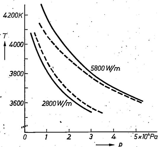
Fig. 6. Measured values (solid curves) and calculated values (dashed curves) for the temperature  $T$  at the axis of a sodium discharge as a function of the sodium pressure  $p$  for two values of the power dissipated in the discharge. The diameter of the discharge tube was 7.6 mm.
