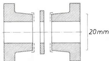
**Fig. 5.** Geometry of the test specimens — as specified in the ASTM<sup>[\*]</sup> Standard F 19-64 — used for tensile testing of the ceramic-to-metal bonds produced by sputtering composite metallization layers.
