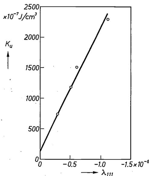
Fig. 16. In an epitaxial garnet film with [111] orientation the uniaxial anisotropy constant  $K_u$  depends linearly on the magnetostriction constant  $\lambda_{111}$ . The value of  $\lambda_{111}$  was varied by doping the garnet with  $\text{Ru}^{3+}$  ions. In this way the  $K_u$  of these films can be tailored to the requirements of the application.
