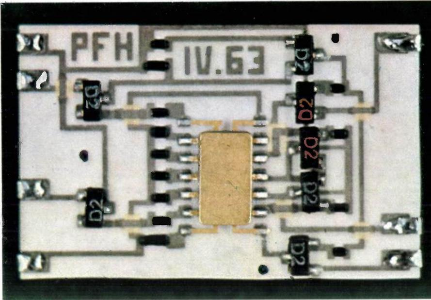
Fig. 4. Analog multiplier for industrial use. Besides the seven solder-bump connectors the substrate ( $18 \times 28$  mm) carries a monolithic IC in a flat package, seven SOT 23 transistors and fourteen resistors. The conductor leads cross at seven places.
