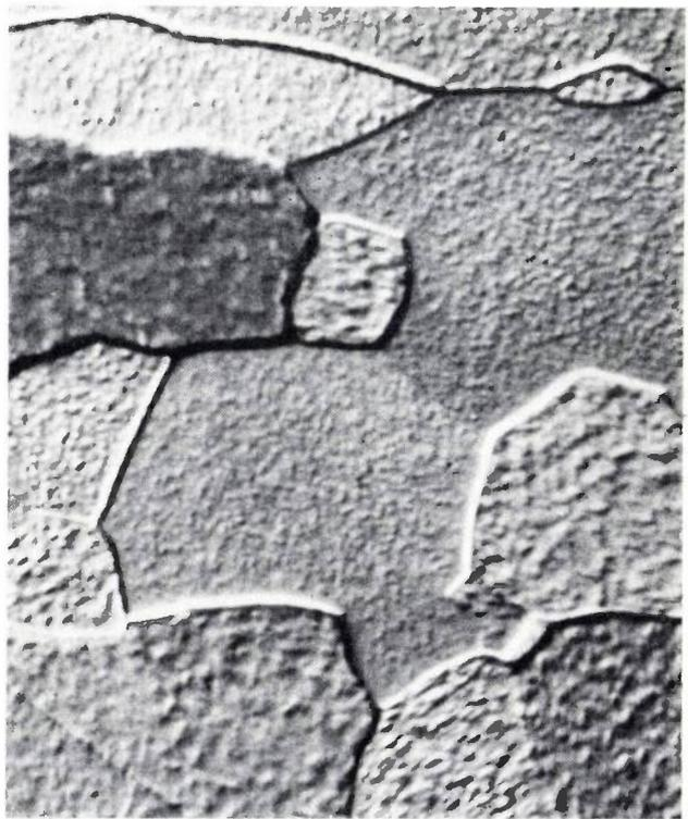
**Fig. 4.** SEM picture of a polished and etched tungsten surface. The grain boundaries are accentuated by shadows resulting from differences in height arising during the etching. The differences in the shade of grey are due to differences in crystal orientation between the grains. Magnification 575  $\times$ .
