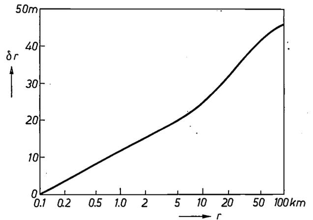
Fig. 14. Graph of predicted range error  $\delta r$  as a function of range  $r$ . As the range increases the signal grows weaker and crosses the detection threshold at a later point in time, thus increasing the range error. The range error is arbitrarily set to zero at a range of 100 m. In calculating the curve a rise time of 310 ns has been assumed for the ground receiver, and 460 ns for the air receiver.
