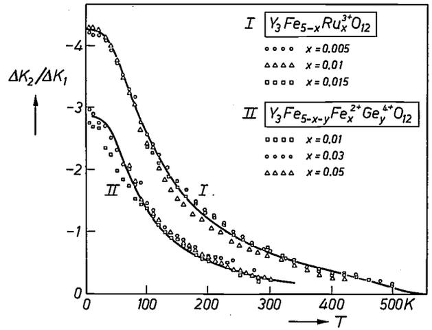
Fig. 10. Temperature dependence of  $\Delta K_2/\Delta K_1$  for YIG doped with  $\text{Fe}^{2+}$  and  $\text{Ru}^{3+}$ . The curves are theoretical and were calculated from eq. (19) with  $\eta$  and  $t$  as parameters.
