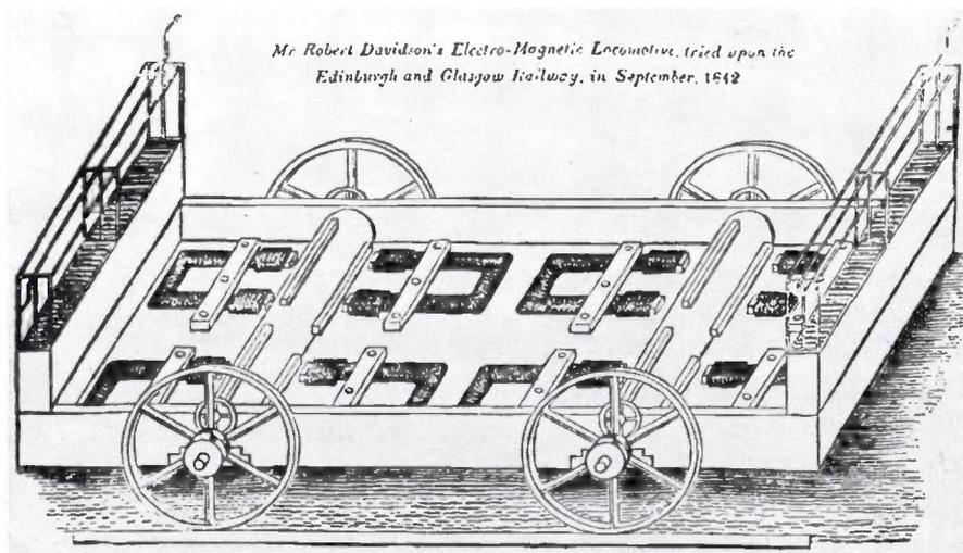
**Fig. 11.** Davidson's electric locomotive, operated experimentally in 1842 on the Edinburgh and Glasgow Railway. The drive was provided by the attractive force between horseshoe magnets and iron strips fixed in grooves in wooden cylinders around the axles. The batteries were arranged at each end of the carriage.
