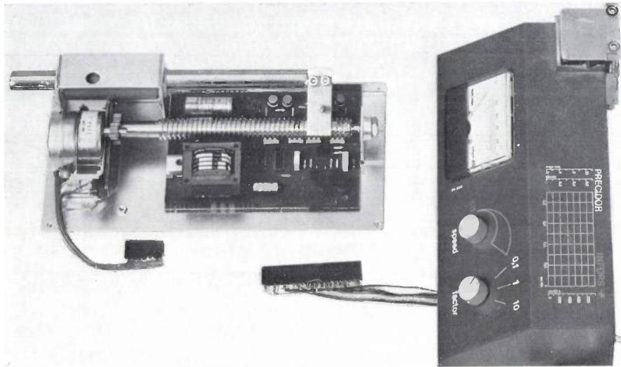
Fig. 1. 'Precidor' infusion pump, type 5003, made by Infors. *Left*: mechanism with Philips ID 04 stepping motor; *right*: the case. The motor drives a lead-screw, which transmits a linear motion to the piston of a syringe (not shown in the photograph). (Photo Infors AG, Binningen, Switzerland.)
