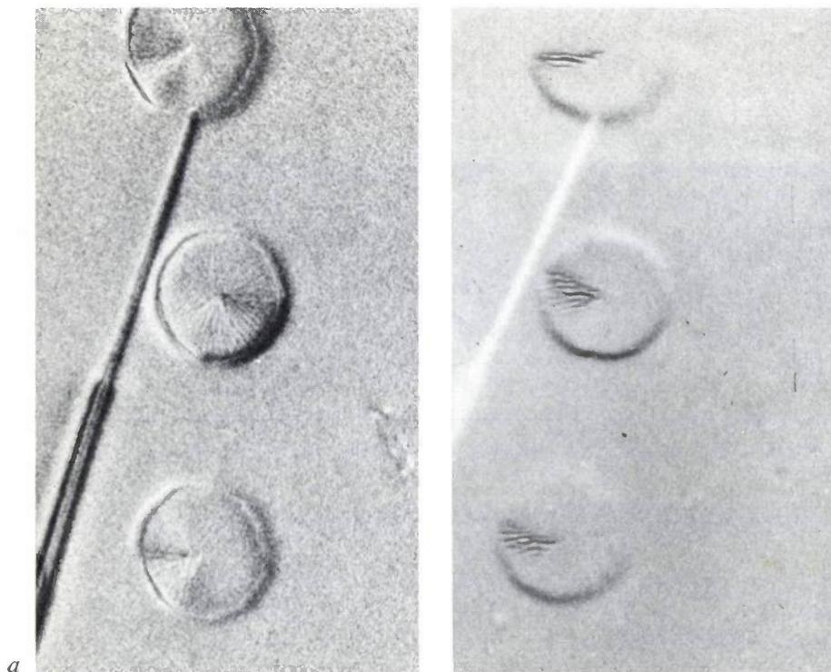
**Fig. 7.** *a*) Transmission topograph, *b*) reflection topograph of helices viewed end-on; *a*) comprises several turns of the helix, *b*) only part of one rotation. This explains why the spoke structure, assumed to lie in the helicoidal surface of the helix, is shown around the complete circle in *a*), but only in a triangular section in *b*).
