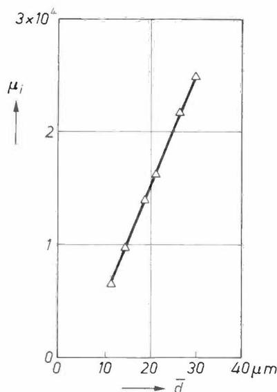
**Fig. 18.** The relative initial permeability  $\mu_i$  of an Mn-Zn-Fe<sup>2+</sup> ferrite, as a function of the average diameter  $\bar{d}$  of the crystallites. (After D. J. Perduijn and H. P. Peloschek<sup>[74]</sup>.)
