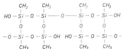
It has an average molecular weight of about 600, contains about 40% w/w silicon and about 10-12% w/w hydroxyl as silanol groups (OH groups linked to silicon). Pairs of the silanol groups become cross-linked on irradiation, producing the desired insolubility.
