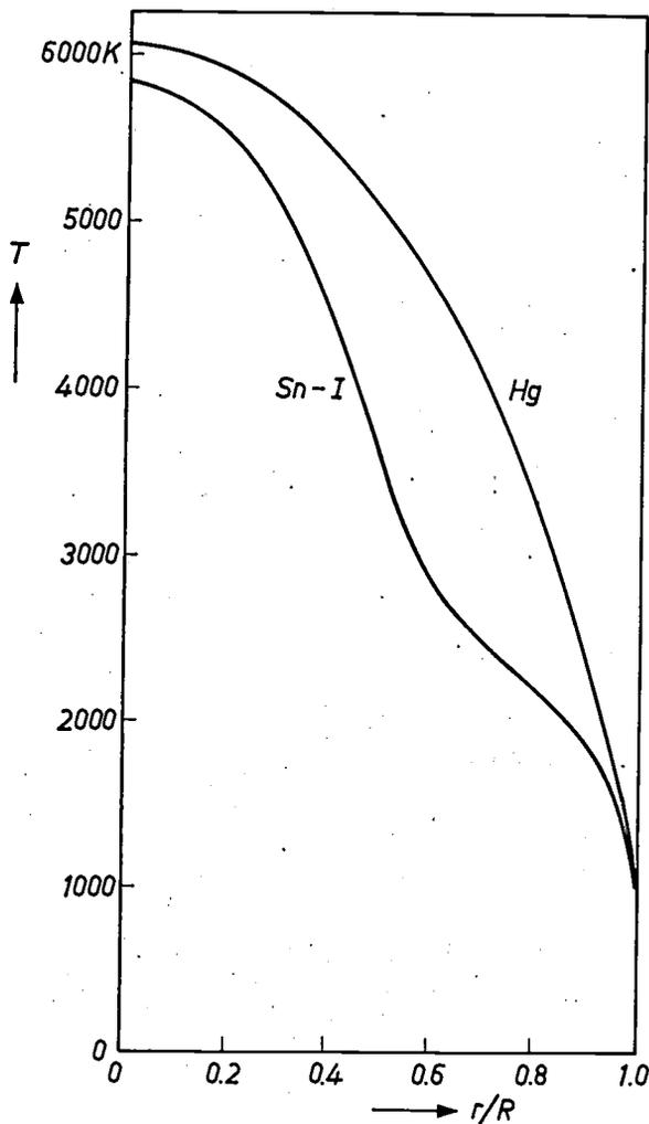
Fig. 5. The temperature profile in a tin-iodide discharge. The calculated temperature  $T$  is plotted as a function of the distance from the axis in a mercury plasma and in a pure tin-iodide plasma, for discharges of 60 W per cm in a tube with a radius  $R$  of 7.5 mm. The profile is narrower in tin iodide than in mercury.
