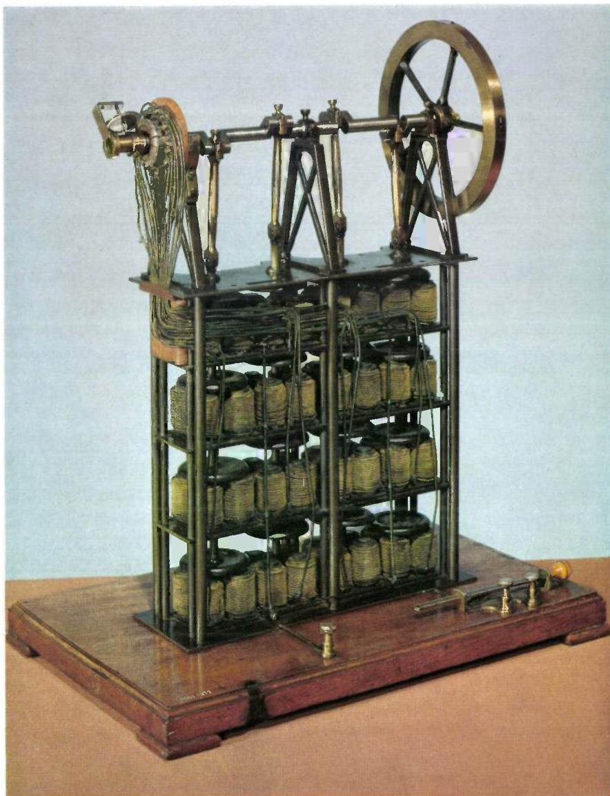
**Fig. 16.** An ingenious electromagnetic engine due to Allan, with four 'piston rods' (1852). Each piston rod is pulled downwards by four groups of electromagnets; these do not operate simultaneously but in sequence, thus magnifying the stroke. (Photo Science Museum, London.)
