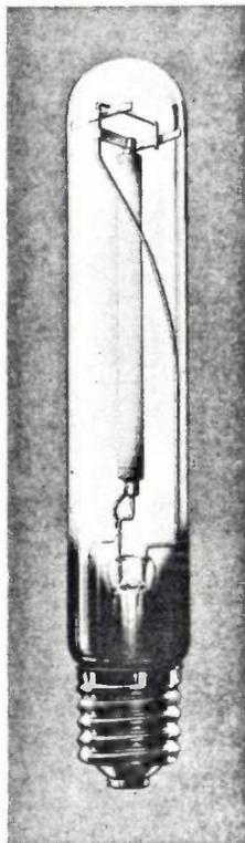
Fig. 2. A high-pressure sodium lamp. The central cylinder is the discharge tube, made from densely sintered alumina. The outer envelope, which is cylindrical here, is evacuated. Another type of envelope is shown in the introductory article [4].
