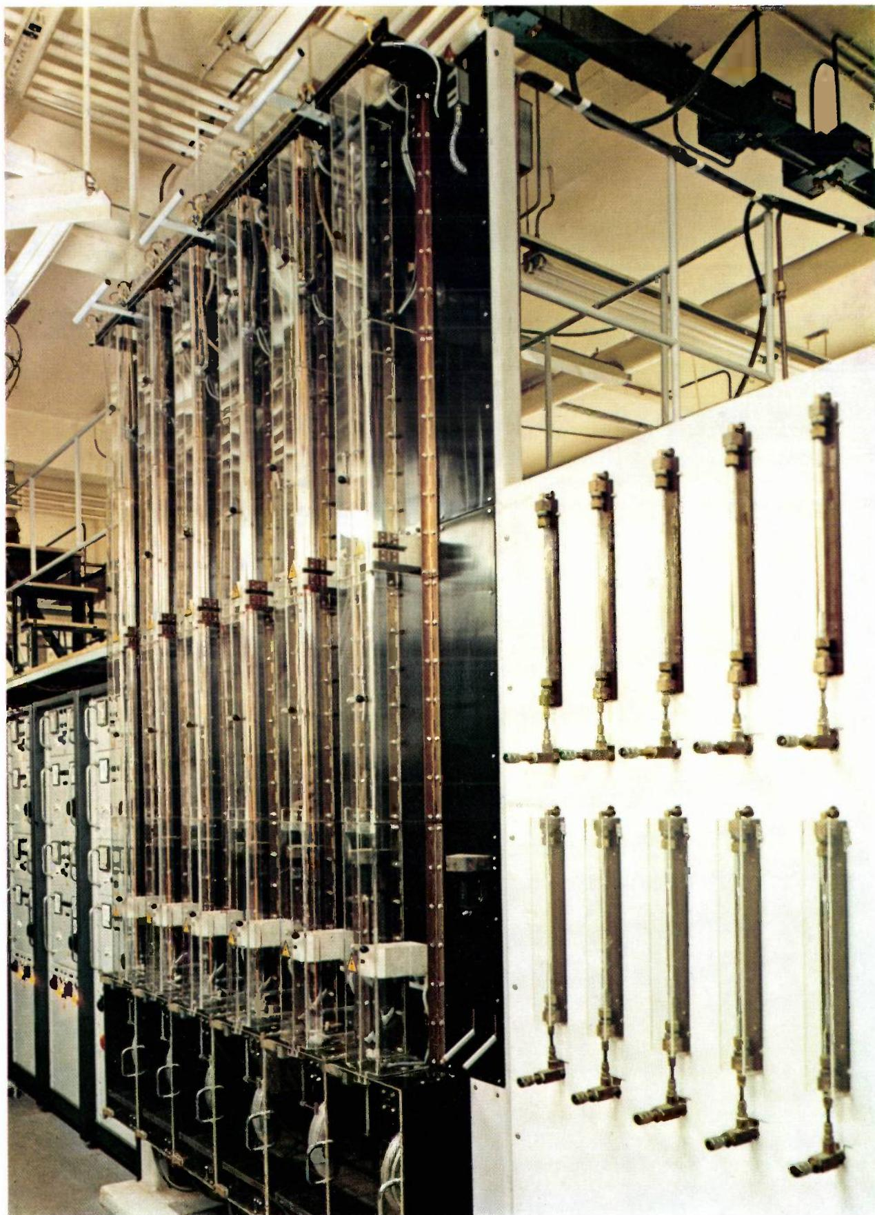
Fig. 5. A battery of boron-deposition reactors in which boron filament was produced continuously for several months.
