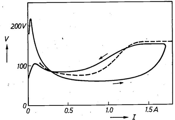
*Fig. 9.* Hysteresis in the current-voltage behaviour of a sodium discharge with a 50-Hz supply.  $V$  is the instantaneous value of the voltage,  $I$  that of the current. The arrows indicate the direction in which the point moves along the curve. The dashed curve is the d.c. voltage characteristic.
