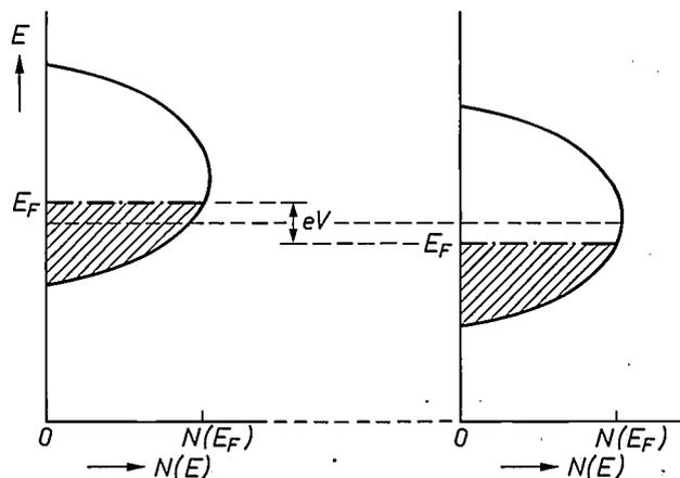
Fig. 4. The conduction band at the two extremities of a specimen (length  $L$ ) across which a voltage is applied. The conduction of electricity can be considered as a diffusion of electrons from left to right under the influence of the electric field  $V/L$ .
