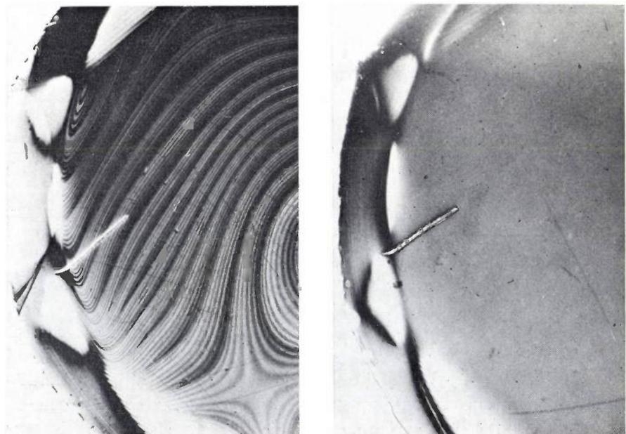
substrate surface, however, hardly affect the epitaxial film either, as is shown in *fig. 9*. This is because the film is sensitive to in-plane strains only, whereas the maximum displacement associated with a striation is perpendicular to its plane. Nearly flat striations mean a nearly flat growth interface, which is required in any case to prevent facet regions from occurring, as we saw above.
