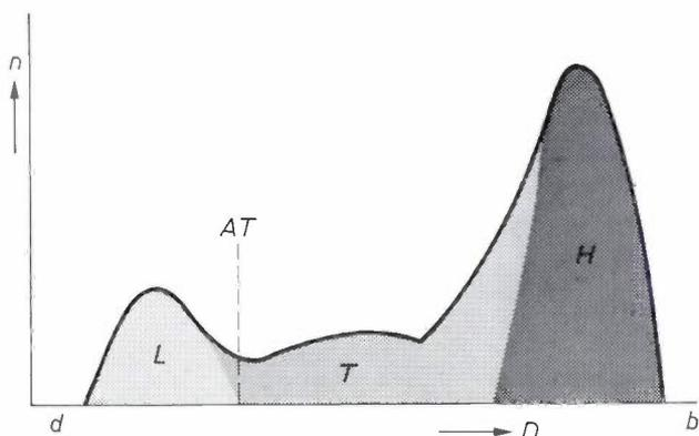
Fig. 4. The choice of an adaptive brightness threshold (*AT*) using the individual brightness distribution determined by the computer. The computer processes an X-ray image of the thorax and calculates a histogram of the resulting grey values (*D*, with *d* = dark and *b* = bright). The frequency of appearance *n* is plotted vertically. *H* heart. *T* tissue. *L* lungs.
