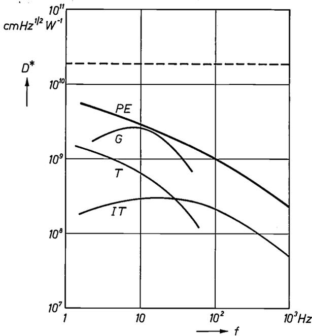
Fig. 16. The detectivity  $D^*$  (as a function of frequency) for various types of infrared detector: the pyroelectric element (LATGS crystal) of fig. 15 ( $PE$ ), a Golay cell ( $G$ ), a thermopile ( $T$ ) and an immersed thermistor ( $IT$ ). The dashed line indicates the theoretical upper limit for a thermal detector.
