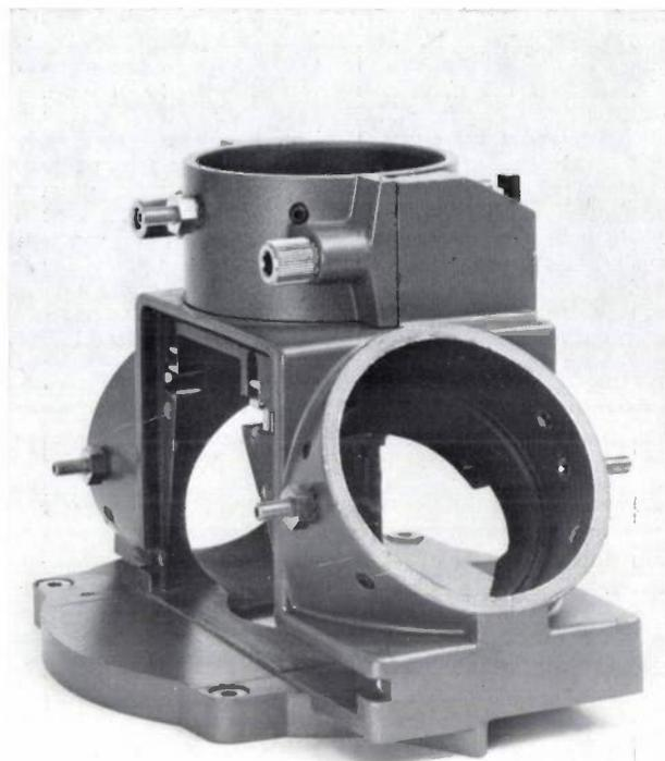
**Fig. 12.** Mount for pick-up tubes and colour-separation prism in a Philips television camera. The pick-up tubes are clamped in the cylindrical openings directed obliquely forwards, upwards and backwards in the photograph. The casting is shown with its flange on the table. This flange is often subject to local heating from the powerful lights in the studio.
