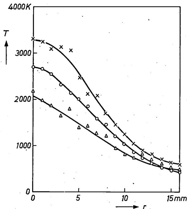
Fig. 3. The temperature  $T$  as a function of the radius  $r$  in discharges in neon of  $10^5$  Pa (1 atm), measured with Rayleigh scattering. The currents were 1 A ( $\Delta$ ), 2 A (O) and 3 A ( $\times$ ).
