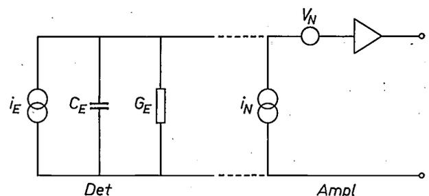
Fig. 2. Equivalent circuit of pyroelectric detector (*Det*) and amplifier (*Ampl*). The generator of the pyroelectric current is represented by  $i_E$ , the total capacitance of the detector element by  $C_E$  and its electrical conductance by  $G_E$ . The generators  $i_N$  and  $V_N$  represent the amplifier current noise and the amplifier voltage noise respectively.
