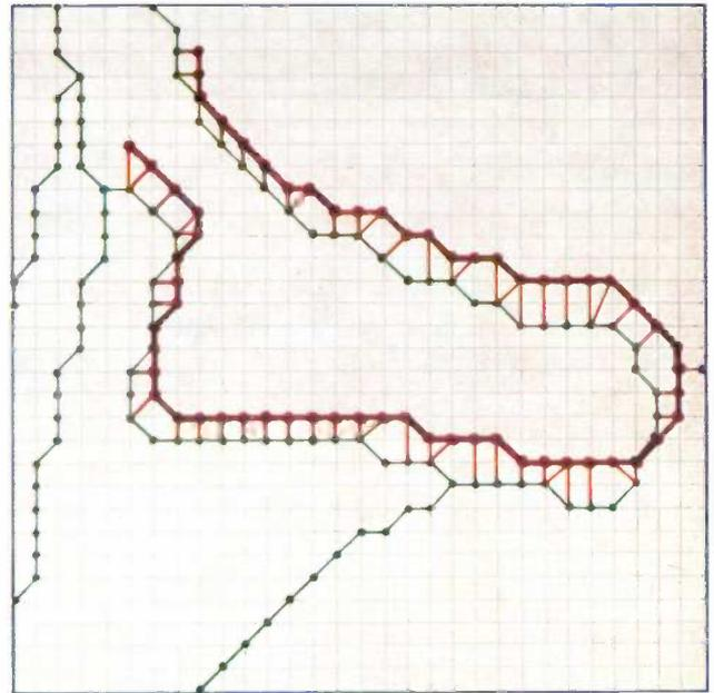
Fig. 14. The second method of coarse searching uses a template. A cardiac-ventricle template (the thick brown line) is shown as an example. This is 'moved' close to the object under investigation by the computer. The distance lines are therefore short. The case shown has been idealized; in practice the template and object will not have precisely the same shape.
