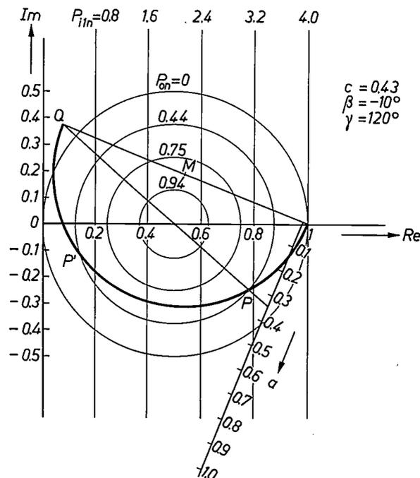
Fig. 9. Plot of  $\underline{Y}$  for a motor designed for a tape recorder (see fig. 5, curve 3).
