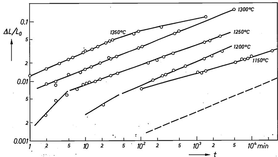
Fig. 13. The linear shrinkage  $\Delta L/L_0$  measured by R. L. Coble [43] at five temperatures when sintering compacted  $Al_2O_3$  powder, as a function of time in the initial stage of the process. The dashed line indicates the slope of a line  $\Delta L/L_0 \propto t^{2/5}$  (see eq. 10).
