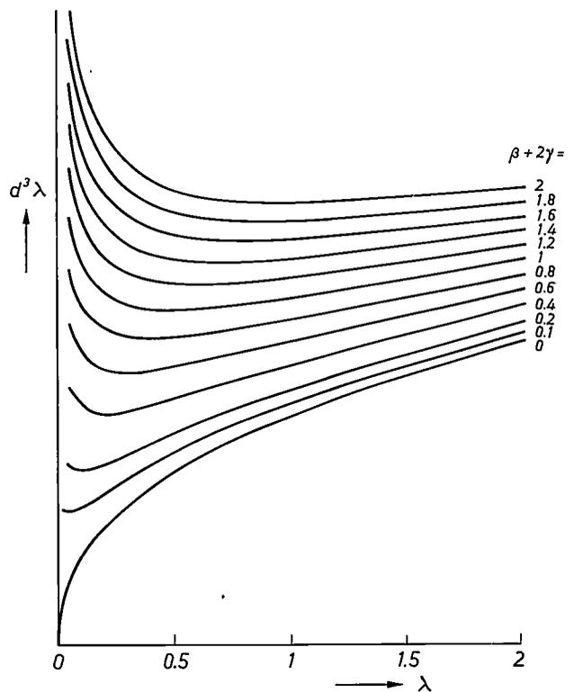
Fig. 9. The required rotor volume (proportional to  $d^3\lambda$ ) as a function of the ratio  $\lambda$  of length to diameter. There is a minimum at  $\lambda = (\beta + 2\gamma)/2$ ;  $\gamma$  is a measure of the length of the curved portions of a winding.
