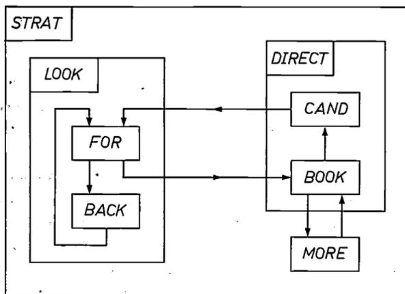
Fig. 5. Diagram of the procedures that together form the strategy STRAT for generating the test patterns for a combinational network. The procedures FOR (forward) and BACK, together forming LOOK, generate the test patterns; MORE investigates the total fault-detection capacity of the test patterns found; BOOK and CAND, together forming DIRECT, determine which new faults will require a search for a test pattern.
