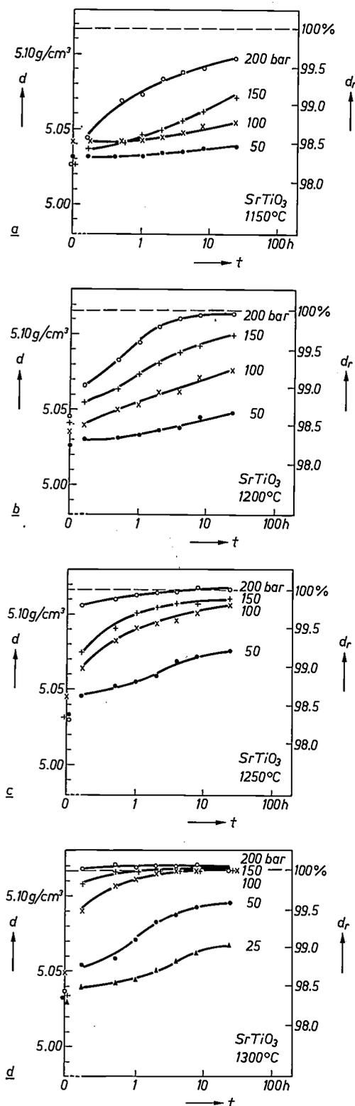
Fig. 8. Shrinkage behaviour of conventionally sintered  $\text{SrTiO}_3$  ceramic which has been hot pressed at 1150 °C (a), 1200 °C (b), 1250 °C (c) and 1300 °C (d) in  $\text{N}_2$  at a pressure which varies from 25 to 200 bars.
