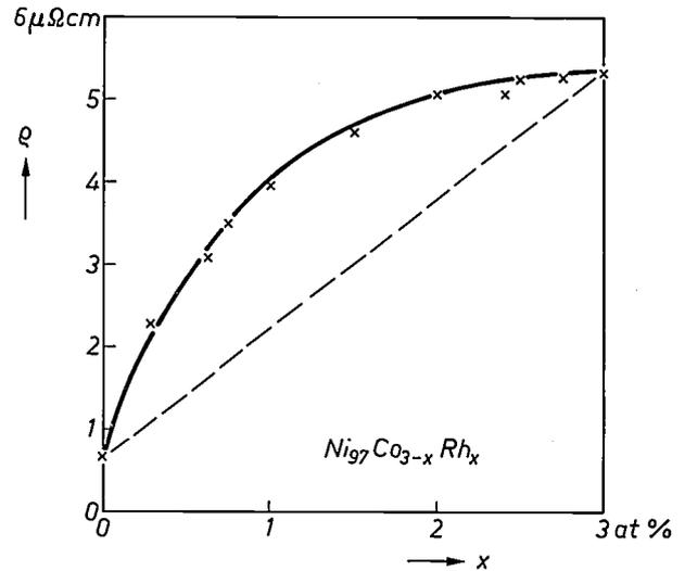
**Fig. 11.** Residual resistivity of ternary alloys of nickel with Co and Rh. The total concentration of Co and Rh taken together is maintained at 3%. The dashed line corresponds to Matthiessen's rule.
