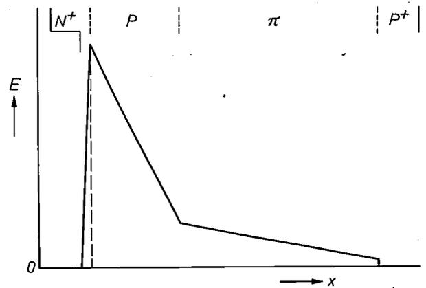
*Fig. 2*. The field-strength  $E$  in an  $N^+P\pi P^+$  diode as a function of position  $x$ . The  $\pi$  layer is a very weakly doped  $P$  layer. The  $N^+P\pi P^+$  structure gives a field across the  $P$ - $N$  junction region that is sufficiently high for the avalanche effect to occur there although the total voltage across the diode (i.e. the area under the curve) is not excessive.
