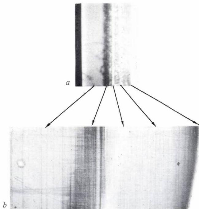
**Fig. 13.** Luminescence images of an epitaxial GaAsP layer grown on a GaAs substrate. *a*) A cleavage plane perpendicular to the growth plane of the layer. At the centre there is a high concentration of dislocations due to the 1.4 per cent mismatch in lattice constants between GaAs and GaAsP. *b*) Image of a surface ground at an angle of  $2^\circ$  to the growth plane. The variations in dislocation density can clearly be seen here. Magnification  $540\times$ .
