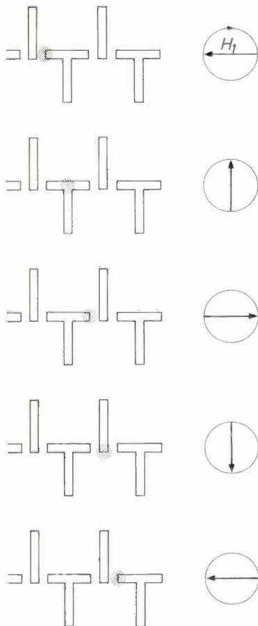
**Fig. 2.** To move a bubble in a well defined manner through a magnetic plate, strips of permalloy, in the form of tees alternating with bars, are applied to the plate. In a circularly polarized in-plane field  $H_1$  the bubble progresses steadily, always seeking the closest north pole.
