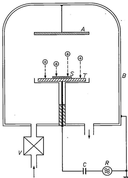
Fig. 3. Schematic diagram of a device for r.f. cathode sputtering. *B* bell-jar of conducting material with a vacuum pump connected at the lower right (to reduce the pressure to about  $10^{-4}$  Pa); argon is admitted via valve *V* until a pressure of about 1 Pa is reached. *R* r.f. source. *C* capacitor. *A* anode in electrical contact with the bell-jar. *T* target cathode with the substrate *S* attached.
