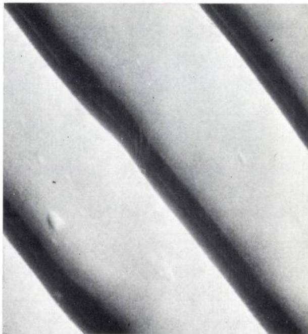
Fig. 7. Scanning-electron micrograph of narrow grooves (dark) in a film of cross-linked methacrylate as in fig. 6. The resist is heated for 15 minutes at 200 °C, exposed at 40  $\mu\text{C}/\text{cm}^2$ , and developed for 2 minutes in methyl isobutyl ketone. It can be seen that the edges are undercut. Magnification 12 000  $\times$ .
