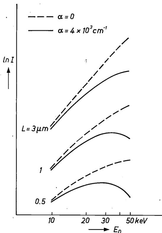
Fig. 6. Calculated total luminescence intensity  $I$  as a function of primary-electron energy. Calculations were made for three values of the diffusion length  $L$  and in each case for both zero and finite values of the absorption coefficient  $\alpha$  for recombination radiation.
