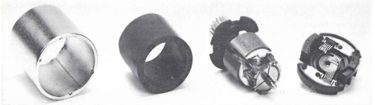
**Fig. 1.** A small d.c. commutator motor, taken apart. From left to right: steel outer housing, plastoferrite ring magnet, rotor with three teeth and three flat commutator segments, bearing cap with brushes and electrical connections.
