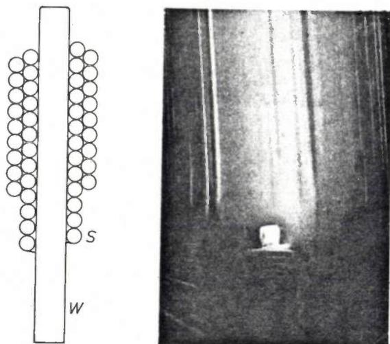
Fig. 4. Electrode of a 400-W HP lamp. *Left*: schematic representation of construction (magnification about  $5\times$ ). *W* tungsten rod. *S* tungsten coil in two layers. *Right*: the electrode in operation.
