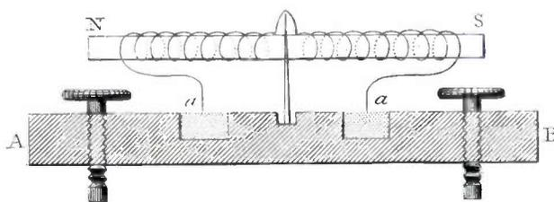
Fig. 7. Ritchie's rotary motor (1833). Current is supplied to the electromagnet *NS* through the mercury in two semicircular grooves *a* in the baseboard. The motor would rotate in the Earth's magnetic field.
