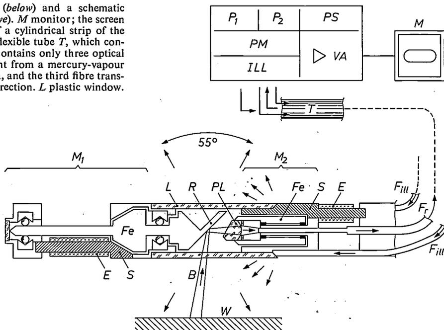
monitor. The motor dissipates 70 mW, which is easily removed by natural convection.
