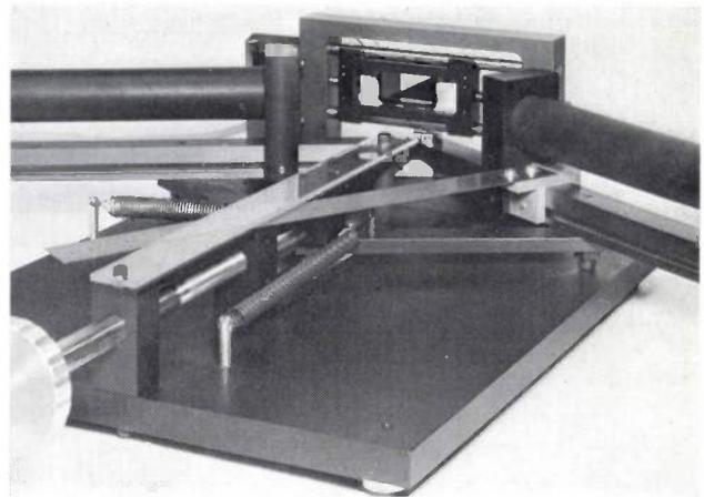
If the angle of incidence differs from the Brewster angle, the thin film also contributes to the intensity of the *p*-component and the voltmeter pointer is set into oscillation by the intensity difference. Since the natural frequency of the pointer (about 1 Hz) is equal to the frequency at which the slide moves back and forth, there is a clear observable indication even at very small intensity differences. The method is most sensitive when the film thickness is  $\frac{1}{4}\lambda$  [4].
