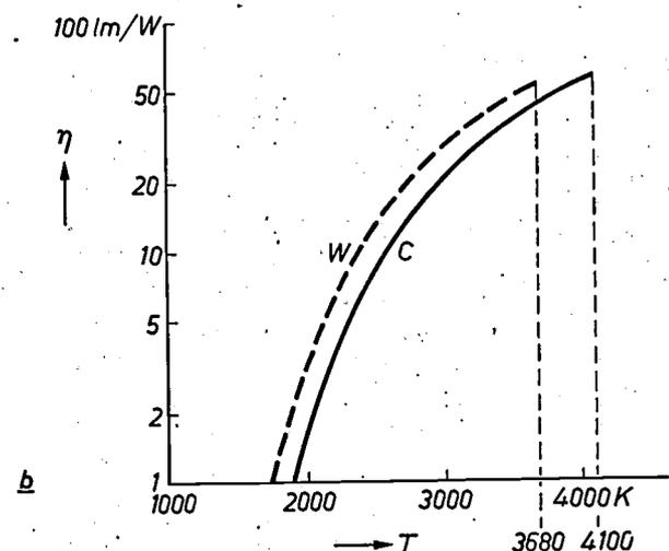
**Fig. 2.** a) The luminance  $L$  for carbon and for tungsten as a function of absolute temperature  $T$ . Carbon sublimates at about 4100 K. Tungsten melts at 3680 K. b) As (a), for the luminous efficacy  $\eta$ .
