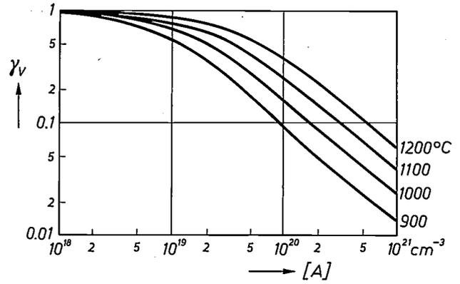
Fig. 5. As fig. 4, but now for the activity coefficient  $\gamma_V$  of a vacancy in silicon. (After Hu [30].)
