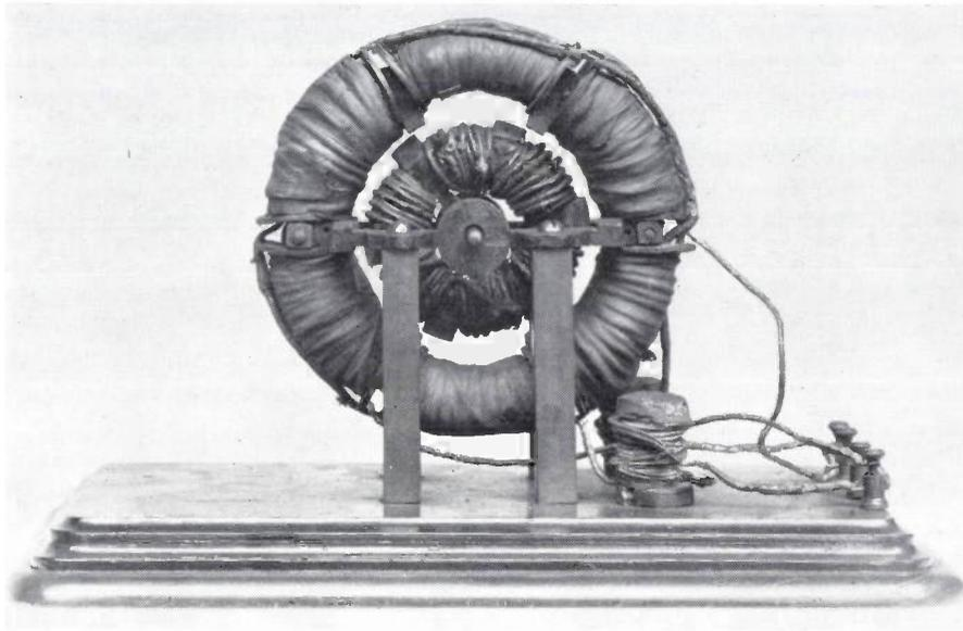
Fig. 22. Langdon Davies's induction machine for a single-phase supply (1891). Four of the six stator coils are connected directly to the supply, two via a resistance. (Lent to the Science Museum, London, by the Langdon Davies Motor Co.)
