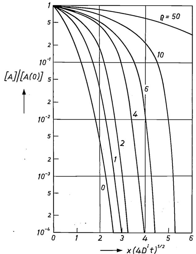
Fig. 6. Calculated concentration profiles for the diffusion of a donor A in silicon. The diffusion source is assumed to be a constant surface concentration  $[A(0)]$ ; the apparent diffusivity is given by eq. (7) in the text. The parameter  $\rho$  indicates the extent to which the material is non-intrinsic;  $\rho = [A(0)]/2n_i$ . (After Hu and S. Schmidt [31].)
