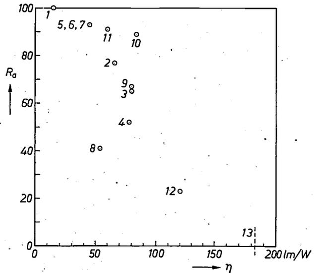
Fig. 1. Combinations of the general colour-rendering index  $R_a$  and luminous efficacy  $\eta$  in the lamps of Table I.
