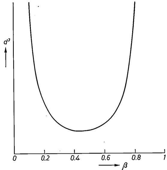
Fig. 8. The required rotor volume (proportional to the third power of the diameter  $d$ ) has a minimum at a certain ratio  $\beta$  of tooth width to rotor diameter. The ratio of rotor length to rotor diameter is assumed to be constant.
