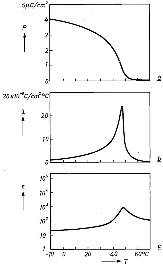
Fig. 7. The temperature dependence of the polarization  $P$ , the pyroelectric coefficient  $\lambda$  and the dielectric constant  $\epsilon$  for a crystal of l-alanine-doped TGS (LATGS). The polarization  $P$  does not go directly to zero at the Curie temperature ( $49^\circ\text{C}$ ) and the peak in the  $\epsilon$  curve is much lower than in the case of TGS (see fig. 5).
