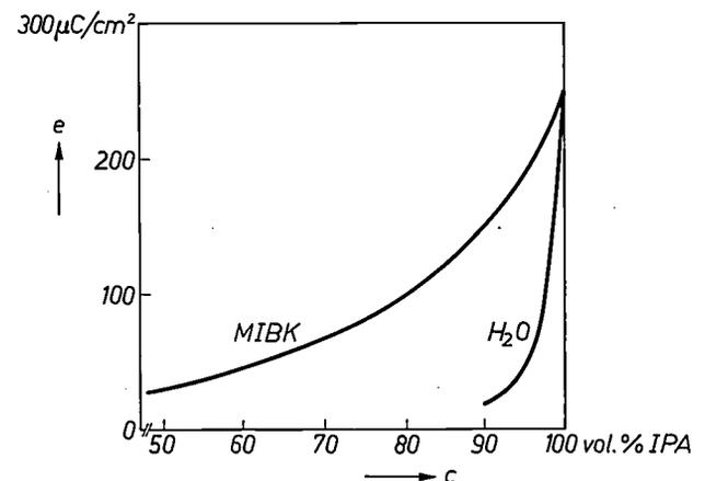
Fig. 3. The minimum electron exposure  $e$  required to form a developable image as a function of the composition  $c$  of the developer, which in one case consists of isopropyl alcohol and water, and in the other of isopropyl alcohol and methyl isobutyl ketone.
