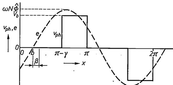
Fig. 3. The voltage  $v_{ph}$  across a phase winding and the induced voltage  $e$  as functions of the electrical phase angle  $x$ .  $b$  phase angle.  $\beta$  phase difference between the induced voltage and the fundamental of the supply voltage.  $\omega$  angular frequency.  $N\hat{\Phi}$  maximum linked flux.
