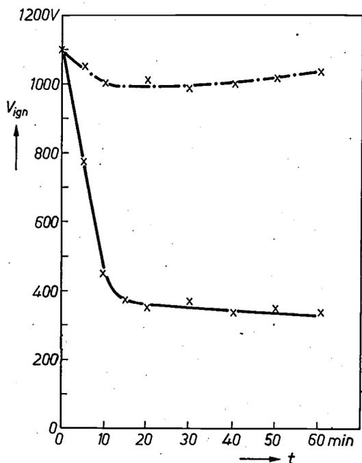
Fig. 3. The ignition voltage  $V_{ign}$  as a function of the operating time  $t$  for argon-filled 400-W HPI lamps made without outgassing, both with (solid curve) and without the getter described in the article. It can be seen that when the getter is used the ignition voltage decreases by a factor of three within 20 minutes.
