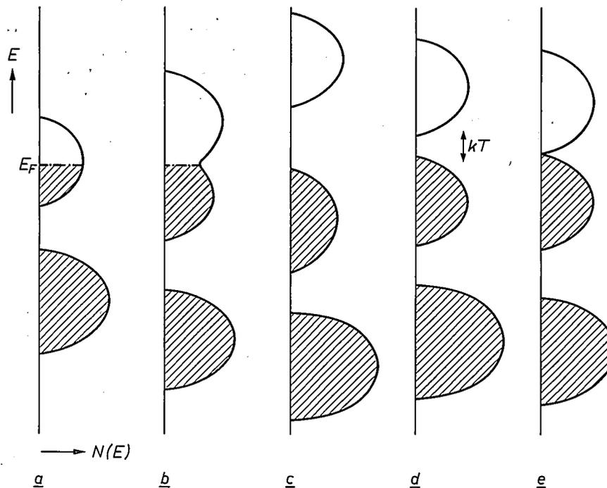
Fig. 5. Energy diagrams as in fig. 3 ( $N(E)$  vs  $E$ ). a) Metal in which only one energy band is of importance for the conduction. b) Metal in which two bands are involved. c) Insulator. d) Semiconductor. e) Semimetal. The semiconductor differs from the insulator only because the empty band is within the reach of a small number of electrons by thermal excitation.
