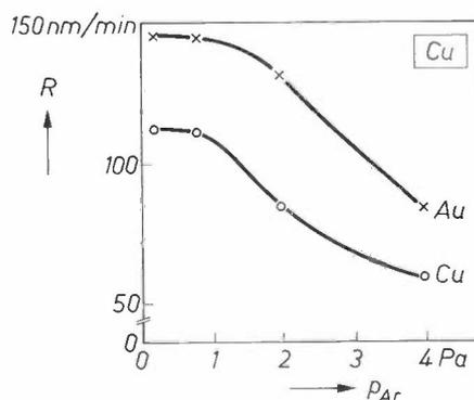
Fig. 8. The etch rate  $R$  of gold and copper substrates, both on a copper target, measured as a function of the argon pressure  $p_{Ar}$  in a cathode-sputtering equipment, at constant ion-current density. As a result of increasing back-diffusion the etch rate decreases markedly with increasing argon pressure.
