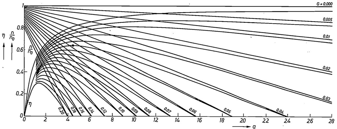
Fig. 5. Curved lines: The efficiency  $\eta$  as a function of  $a = T/T_d$  (where  $T$  is the delivered torque and  $T_d$  the loss torque), with  $G$  as parameter. For the motor shown in fig. 1,  $G = 0.04$  and the maximum efficiency is 0.64. Straight lines: speed-torque characteristics.  $n$  speed.  $n_0$  reference speed.
