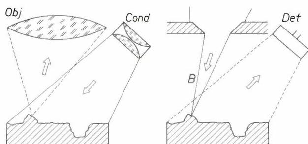
The objective *Obj* produces an image of the specimen surface; each point of the surface corresponds uniquely to a point of the image.
