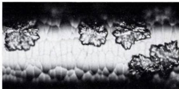
Fig. 8. The surface of a filament formed at a temperature above the critical temperature (the grey region in *fig. 7*). The boron in the patches of different structure is crystalline ( $\beta$ -rhombohedral).
