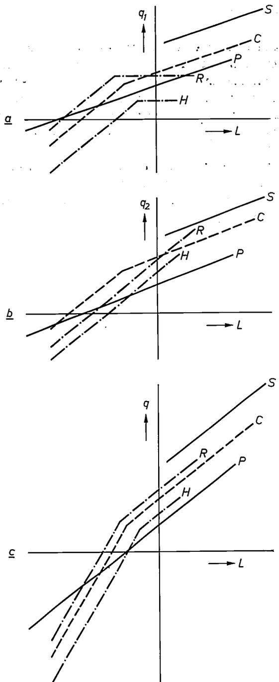
**Fig. 6.** Variation of the figures of merit with the linear dimension  $L$ . The discontinuity in some of the curves occurs at the critical dimension  $L_c$  at which magnetic saturation starts. *a*) The power-to-weight ratio  $q_1$ , *b*) the figure of merit  $q_2$ , which is related to the efficiency, *c*)  $q$ , the product of  $q_1$  and  $q_2$ .
