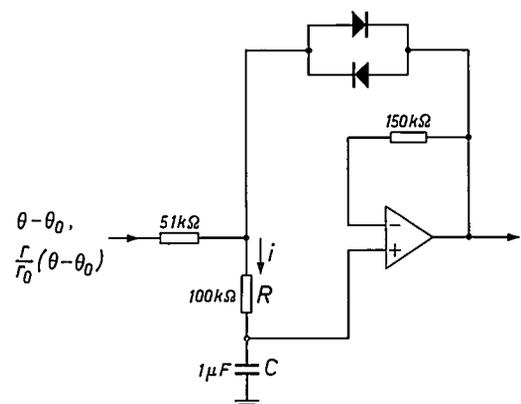
*Fig. 11.* Rate-of-change limiter circuit. For slowly varying signals the charging current  $i$  is small and the voltage  $iR$  developed across the resistor  $R$  is smaller than the forward voltage drop across the silicon diodes (450 mV). Limiting occurs when  $iR \geq 450$  mV. The rate of change of voltage is then limited to  $450 \text{ mV}/RC = 4.5 \text{ V/s}$ .
