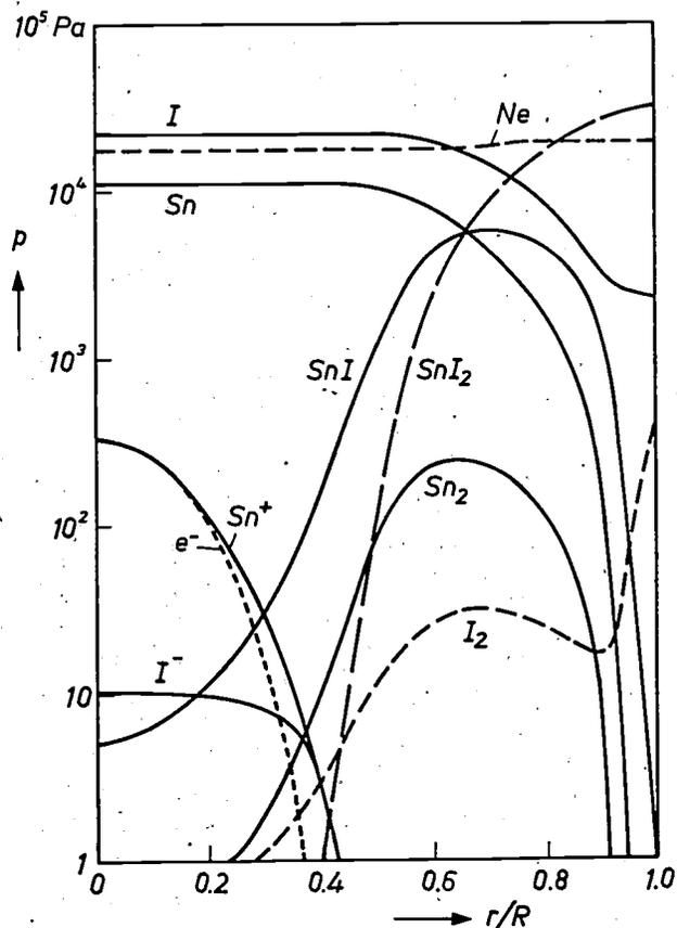
*Fig. 4.* Composition of the plasma in an Sn-I discharge determined from model calculations [5]. The partial pressure  $p$  of the components is plotted as a function of the distance  $r$  from the axis ( $R$  radius of the tube). The continuum of *fig. 1d* consists to a small extent of recombination radiation ( $e^- + \text{Sn}^+ \rightarrow \text{Sn}$ ) from the centre of the discharge, but most of it is molecular radiation from SnI in a sheath around the axis.
