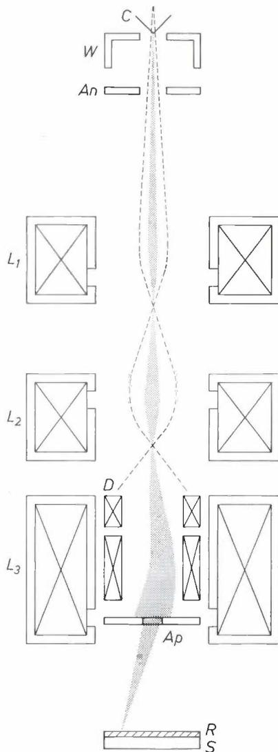
**Fig. 1.** Schematic diagram of a scanning electron-beam apparatus. *C* cathode. *W* Wehnelt cylinder that modulates the intensity of the electron beam. *An* anode. *L*<sub>1</sub>, *L*<sub>2</sub> and *L*<sub>3</sub> magnetic lenses. *D* deflection coils. *Ap* aperture. *S* substrate, coated with resist. *R*.
