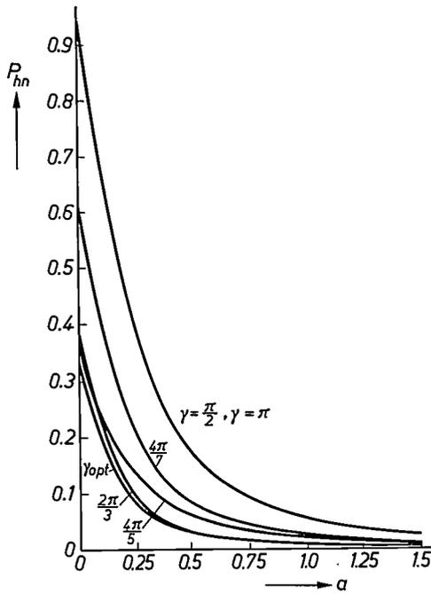
Fig. 6. The losses  $P_{hn}$  (normalized) that arise at higher harmonics as functions of the (normalized) speed  $a$ , for various values of the switching angle  $\gamma$ . The curve for  $\gamma_{opt}$  represents the theoretical minimum losses;  $\gamma_{opt}$  is itself a function of  $a$  (see fig. 7).
