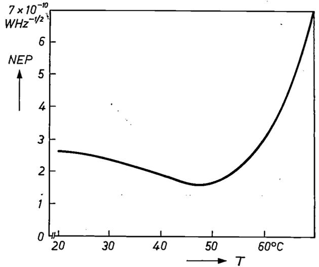
Fig. 17. The temperature dependence of the noise equivalent power  $NEP$  for a pyroelectric infrared detector with a highly l-alanine-doped TGS crystal, measured at 125 Hz with  $A = 0.25 \text{ mm}^2$ . The lowest  $NEP$  values are found at about 50 °C.
