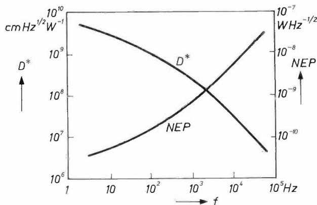
Fig. 15. The frequency dependence of the noise equivalent power  $NEP$  and the detectivity  $D^*$  for a detector with an LATGS crystal as pyroelectric element. ( $D^* = A^{1/2}/NEP$ ;  $A$  is the area of electrode exposed to radiation.)
