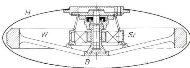
Fig. 3. A simplified transverse cross-section of the flywheel illustrated in fig. 2. *H* housing. *W* wheel, with bearing bush *B*. The stator *Sr* of the driving motor is concentric with the bearing bush.
