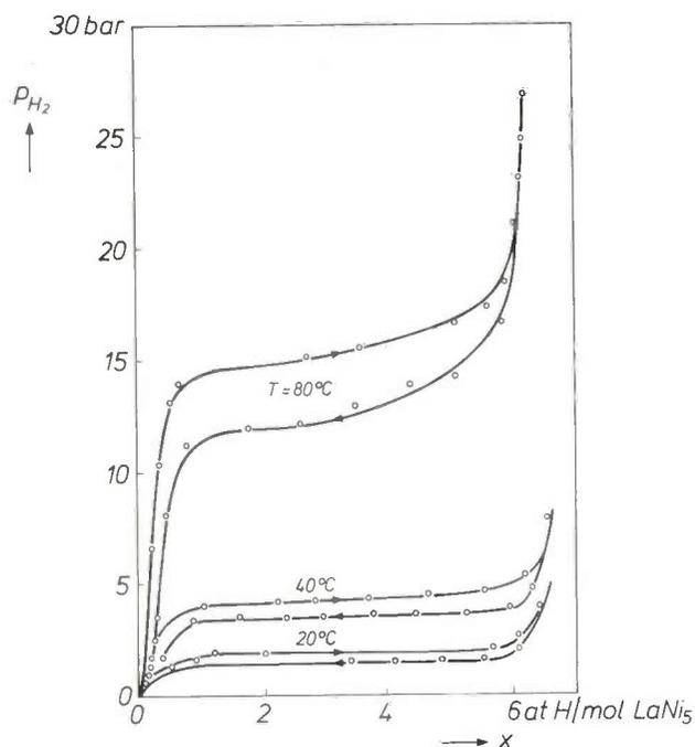
Fig. 5. Absorption and desorption isotherms (hydrogen pressure  $p_{\text{H}_2}$  as function of the concentration of hydrogen atoms  $x$ ) of the  $\text{LaNi}_5\text{-H}_2$  system at 20, 40 and 80 °C.
