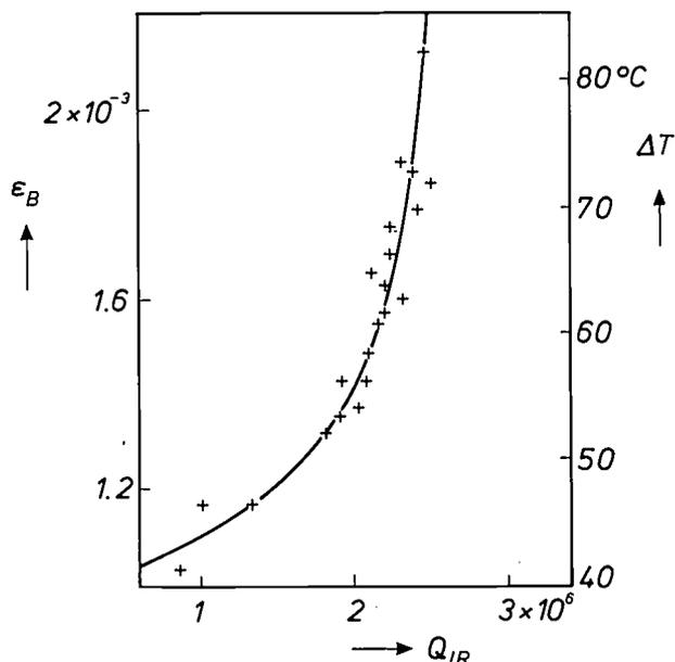
Fig. 6. Breaking strain  $\epsilon_B$  (left-hand axis) and the temperature shock  $\Delta T$  (right-hand axis) as a function of  $Q_{IR}$ . Samples were placed in a hot bath at a temperature  $T_B$  for 30 minutes and then transferred quickly to a cold bath at  $T_C$ . The samples of one batch were tested with increasing temperature difference  $\Delta T = T_B - T_C$ . The infrared quality factor  $Q_{IR}$  was measured for each sample.
