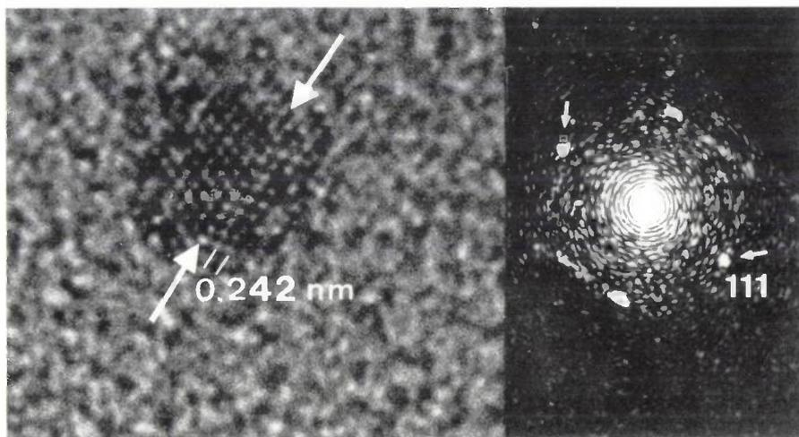
Fig. 4. *Left*: TEM micrograph of a metallic nucleus consisting of no more than a few hundred palladium atoms (obtained on a titanium-oxide layer a few microns thick, supported by a silicon-nitride film a few tens of microns thick). It can clearly be seen that the nucleus has a crystalline structure, in which the familiar effect of 'twinning' has taken place (the mirror plane corresponds to the direction of the arrows). *Right*: TEM diffraction micrograph of the nucleus [5].
