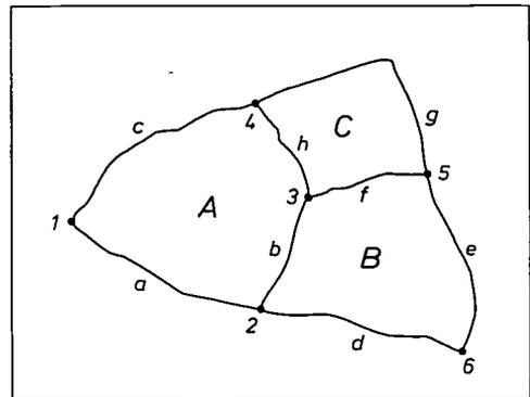
Fig. 3. Some concepts from topology [6]. 1 to 6 0-cells (nodes). a to h 1-cells (chains). A to C 2-cells (areas inside concatenated chains).
