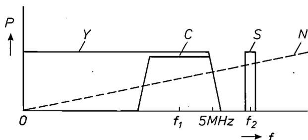
Fig. 1. General diagram of the frequency spectrum  $P$  of a colour-television signal in one of the current systems PAL, NTSC and SECAM.  $Y$  luminance information.  $C$  colour information.  $S$  sound information.  $N$  triangular noise resulting from frequency modulation.  $f_1, f_2$  subcarrier frequencies for  $C$  and  $S$  respectively.
