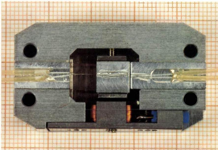
**Fig. 13.** Photograph of the interior of the relay *REL* in *fig. 12*. The optical fibres are bonded by adhesive into V-grooves, which are made in a single operation in both the housing and the armature during manufacture. This means that there is no need for extremely tight tolerances. Set-screws on either side determine the two extreme positions of the armature. The two leaf springs that attach the armature to the housing are hardly visible in this photograph.
