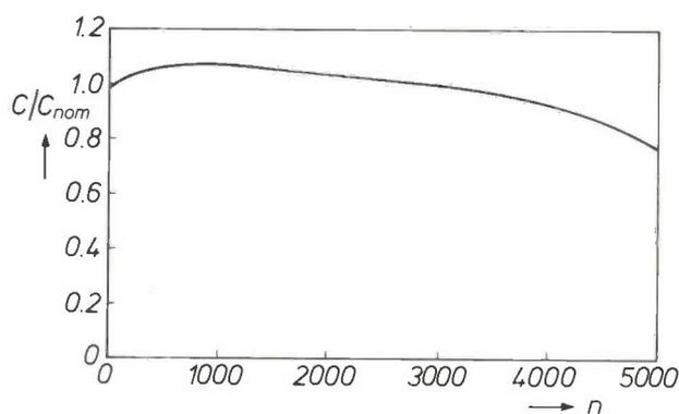
Fig. 19. The relative storage capacity  $C/C_{nom}$  of an experimental nickel-hydride cell as a function of the number of charge/discharge cycles  $n$ . The hydride electrode is oversized by a factor of 1.85 with respect to the nickel electrode.  $C_{nom}$  is 300 mAh.
