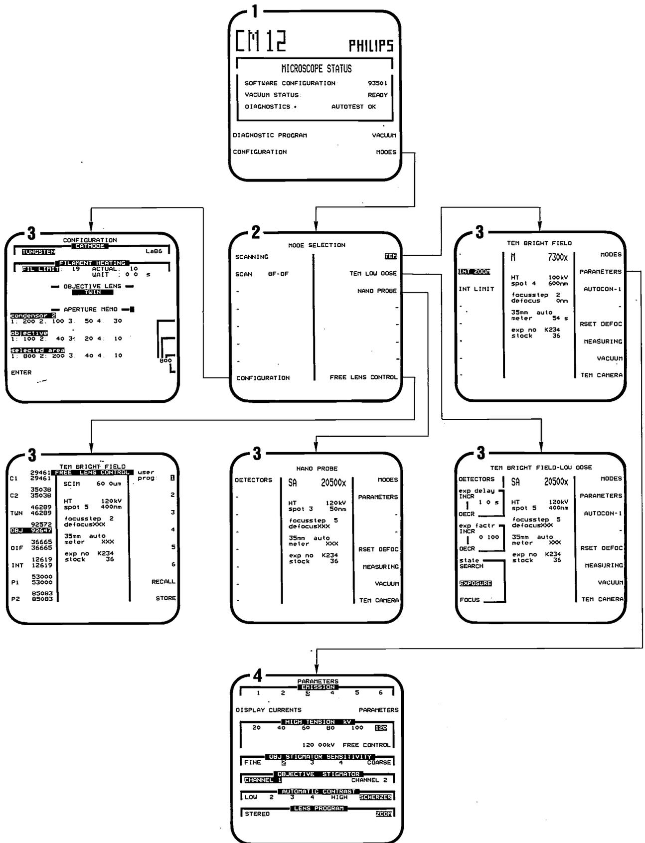
Fig. 12. The hierarchy of some of the many 'pages' that can be displayed on the control screen. The number at the upper left of each page indicates the level. The mode is selected from the options on a page at level 2. The mode to which the instrument is set can be seen from a page at level 3. The field in the centre then gives the settings of the parameters; the fields on either side indicate the functions of the soft keys. Parameters are changed via a page at level 4.
