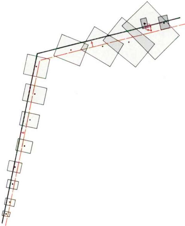
**Fig. 9.** A position correction after the computer has recognized the road pattern. This pattern is compared with the routes *A-C-D-F-H* and *A-C-E-G-H* on the map, see fig. 8, and the second route is rejected. Best-fitting straight lines (red dashes) through the consecutive centres of VLPAs yield two vectors. The resultant gives the displacement of the centre of the last VLPA, and the positional uncertainty immediately becomes smaller. It grows again as the distance travelled increases.
