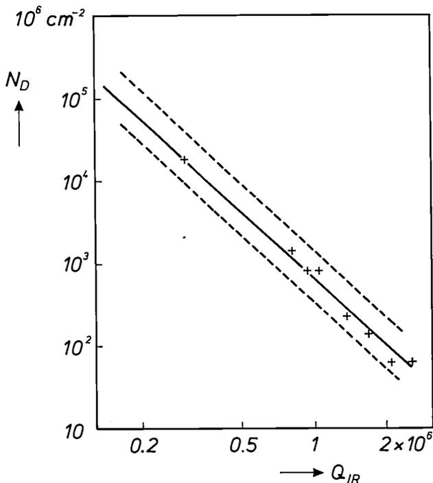
Fig. 4. Overall median dislocation density  $N_D$  as a function of the infrared quality factor  $Q_{IR}$  (continuous line and crosses). For any supplier the logarithm of the dislocation density has a Gaussian distribution. Results for the two most extreme suppliers are indicated by dashed lines.
