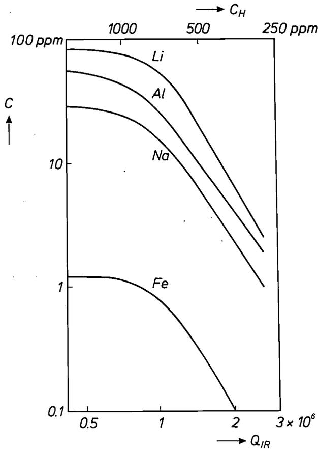
Fig. 3. Overall median impurity concentrations  $C$  as a function of  $Q_{IR}$ . The data are for the  $z$ -zone of crystals. Material grown on other faces is much less pure. For any supplier the distribution of  $\log C$  at a given  $Q_{IR}$ -value is approximately Gaussian.
