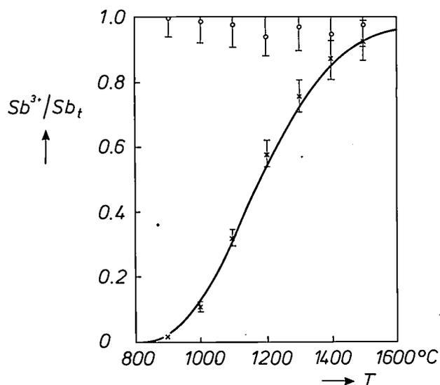
**Fig. 6.** The ratio  $Sb^{3+}/Sb_T$  for 'raw-materials samples' (crosses) and 'powdered cullet samples' as a function of the temperature to which the samples have been subjected for 20 hours.
