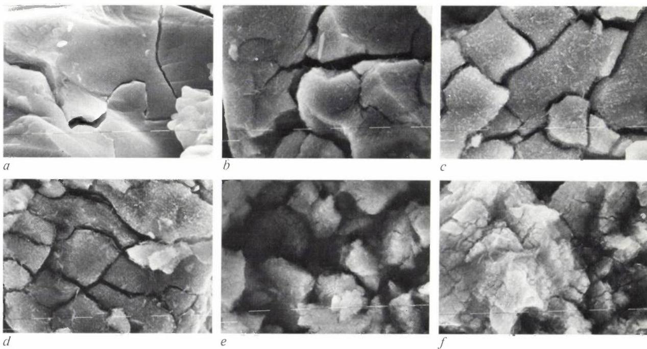
**Fig. 12.** SEM micrographs of  $\text{LaNi}_5$  electrodes after repeated charging and discharging. The results are shown after zero (a), 12 (b), 25 (c), 63 (d), 176 (e) and 359 (f) charge/discharge cycles. One 'dash' represents 1  $\mu\text{m}$ .  $\text{La}(\text{OH})_3$  needles, which are visible from (b) onwards, have completely overgrown the original material in (f).
