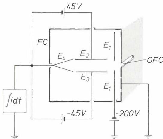
*Fig. 7.* Diagram of the cross-section of the Faraday cup *FC* with opening *OFC*; see *fig. 5*, and with the electrodes  $E_{1-4}$ . Electrode  $E_4$  captures the ions from the beam. The result of the measurement with the current integrator connected to  $E_4$  is a measure of the implantation dose.  $E_1$  repels secondary electrons from outside the cup. The charged particles captured by  $E_2$  and  $E_3$  contribute to the measured result.
