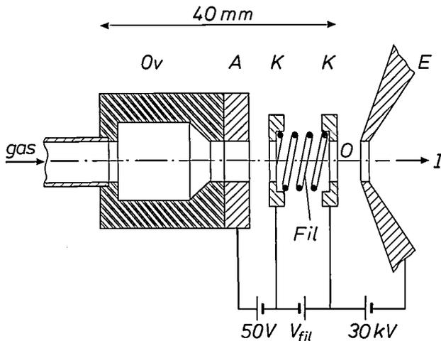
Fig. 8. The hollow-cathode source. *Ov* oven. *A* anode. *K* cathode, consisting of two parts. The two parts are connected by the filament *Fil*.  $V_{fil}$  filament voltage. *E* extraction electrode. *I* ion-beam current. The source contains a plasma that protrudes from the extraction aperture *O*.
