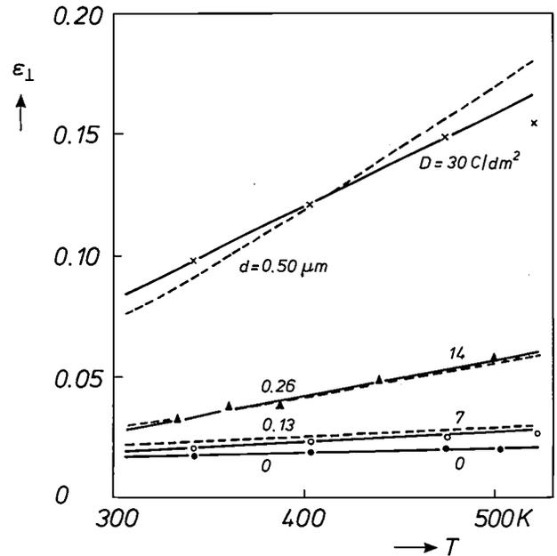
Fig. 12. Temperature dependence of the thermal emissivity  $\epsilon_{\perp}$  for black-cobalt coatings with different electrolytic thicknesses  $D$  (continuous curves) and calculated for different geometrical thicknesses  $d$  (dashed curves). It is seen that  $\epsilon_{\perp}$  depends linearly on the absolute temperature  $T$ , and that the slope increases for thicker coatings.
