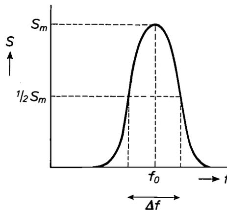
Fig. 1. Plot of the mechanical distortion  $S$  of a quartz plate in response to an applied alternating voltage of frequency  $f$ . The fundamental frequency of this plate is  $f_0$  and  $\Delta f$  is the width of the response at half the maximum value of the response. These quantities determine the electrical quality factor  $Q_e (= f_0/\Delta f)$ .
