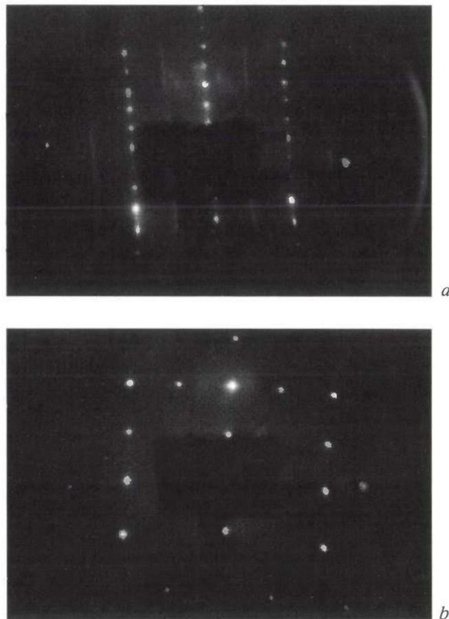
Fig. 5. LEED patterns from a (001) GaP substrate (a) and a silicon film (b). The patterns indicate that when silicon is deposited the surface reconstruction changes from  $(4 \times 2)$  to  $(2 \times 1)$ .
