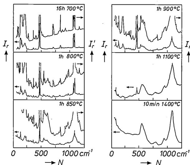
Fig. 3. Raman spectra of mixes consisting of 15 mol% of  $\text{Na}_2\text{CO}_3$ , 10 mol% of  $\text{BaCO}_3$  and 75 mol% of  $\text{SiO}_2$  that have been heated for different times and at different temperatures (shown top right) and then quenched to room temperature. The intensity  $I_r$  is shown as a function of the wave number  $N$  in arbitrary units; at the four lowest temperatures it is also shown with a unit five times as large ( $I_r'$ ).
