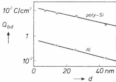
Fig. 17. Amount of charge transferred per unit area up to breakdown ( $Q_{bd}$ ) plotted as a function of the thickness  $d$  of the oxide film for MOS capacitors with a polysilicon and an aluminium gate. In polysilicon,  $Q_{bd}$  is a hundred times higher. In both cases,  $\log Q_{bd}$  decreases linearly with  $d$ .
