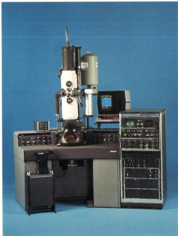
**Fig. 3.** The EM 420 transmission electron microscope complete with all accessories. The Dewar vessel immediately to the right of the column contains liquid nitrogen for cooling the energy-dispersive X-ray detector (*EDX* in *fig. 2*); below this and to the right is the electronic unit for displaying the X-ray spectrum. On the extreme right is the STEM unit. This, like most other accessory units, is integrated into the latest electron microscope, CM12/STEM; see *fig. 4*.
