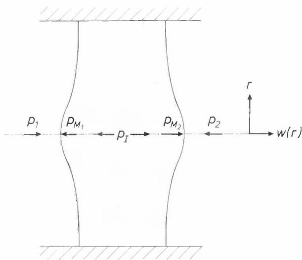
**Fig. 3.** Definition of some of the quantities used in calculating the output quantity  $1/C_1 - 1/C_2$  as a function of the differential pressure  $\Delta p = p_2 - p_1$  (equation 5).  $p_1$  pressure of the liquid in the transducer,  $p_{M1}$ ,  $p_{M2}$  resultant pressures on the diaphragms.  $r$  radius with respect to the axis of symmetry.  $w(r)$  deflection of a diaphragm as a function of  $r$ , with  $w = 0$  in the undeflected state.
