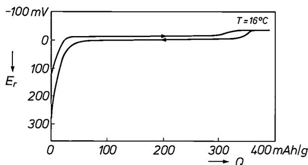
Fig. 8. Charge and discharge curve for an  $\text{LaNi}_5$  electrode, with respect to the reversible hydrogen electrode, as a function of the charge  $Q$ , measured in  $6\text{ M KOH}$  at  $16^\circ\text{C}$ .
