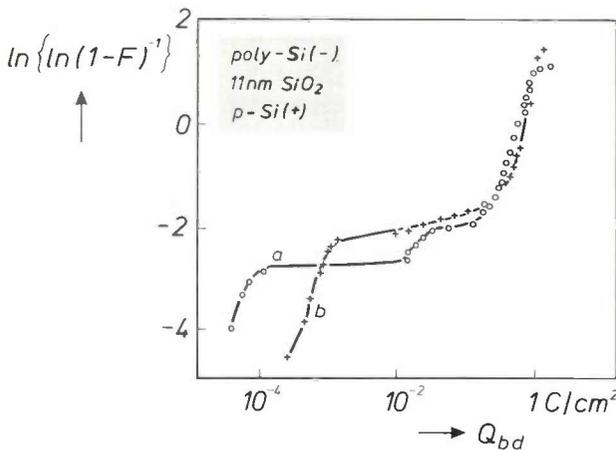
Fig. 12. Breakdown distribution for MOS capacitors as a function of the integrated charge transferred per unit area ( $Q_{bd}$ ) at a constant current of  $40 \mu\text{A}$  (curve *a*) and at a constant voltage of  $12.9 \text{ V}$  (curve *b*). Beyond  $Q_{bd}$  values greater than  $0.01 \text{ C/cm}^2$  the curves are virtually coincident.
