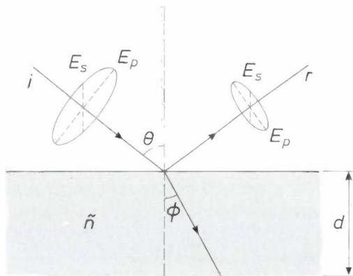
**Fig. 2.** Schematic representation of the reflection of elliptically polarized light at the surface of a layer. The parallel and perpendicular components  $E_p$  and  $E_s$  of the electric vector of the reflected light beam (*r*) differ from those of the incident beam (*i*). The ratio of the reflectances of the two components depends on the angle of incidence  $\theta$ , the angle of refraction  $\phi$  and the complex index of refraction  $\tilde{n}$  and the thickness  $d$  of the layer.
