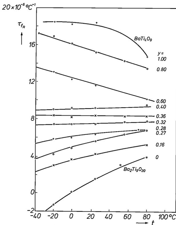
Fig. 4. Temperature coefficient  $\tau_{f_R}$  for the resonant frequency  $f_R$  of ceramic samples as a function of temperature  $t$ . Each curve corresponds to a different value of the molar content  $y$  of  $\text{BaTi}_4\text{O}_9$  in the two-phase ceramic  $(\text{Ba}_2\text{Ti}_9\text{O}_{20})_{1-y}-(\text{BaTi}_4\text{O}_9)_y$ .
