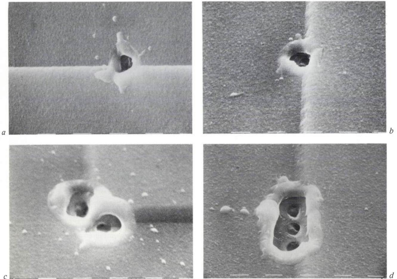
**Fig. 8.** Scanning electron micrographs (scale division 1  $\mu\text{m}$ ) of craters formed during breakdown of MOS capacitors for different current values: *a*) 10 nA. *b*) 100 nA. *c*) 1  $\mu\text{A}$ . *d*) 10  $\mu\text{A}$ . The dimensions of the craters are virtually independent of the current. The craters usually form at corners and edges of the device.
