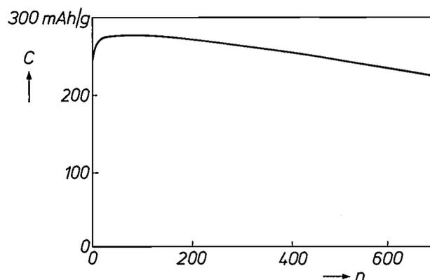
Fig. 15. The storage capacity  $C$  of an electrode of  $\text{La}_{0.8}\text{Nd}_{0.2}\text{Ni}_{2.5}\text{Co}_{2.4}\text{Si}_{0.1}$  as a function of the number of charge/discharge cycles  $n$ . The improvement in stability with respect to  $\text{LaNi}_5$  is clear from a comparison with fig. 9.
