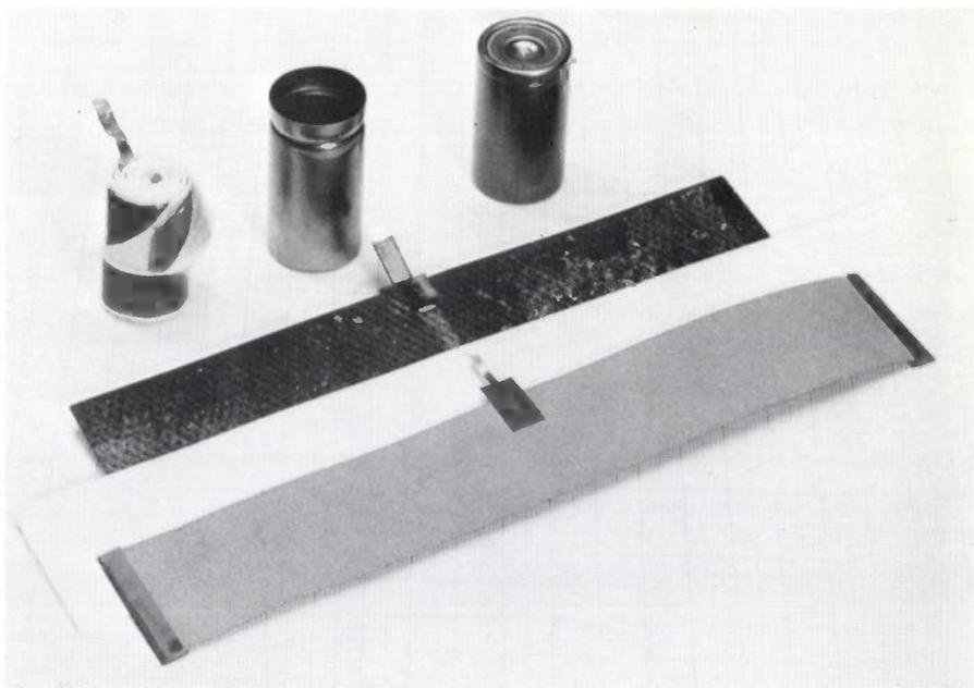
Fig. 21. Illustrating the second manufacturing step. A hydride electrode (grey; see the lower strip in fig. 20) is rolled up with a sintered nickel electrode (black) and a separator (white) to form a cylindrical battery. After addition of electrolyte the battery is hermetically sealed.
