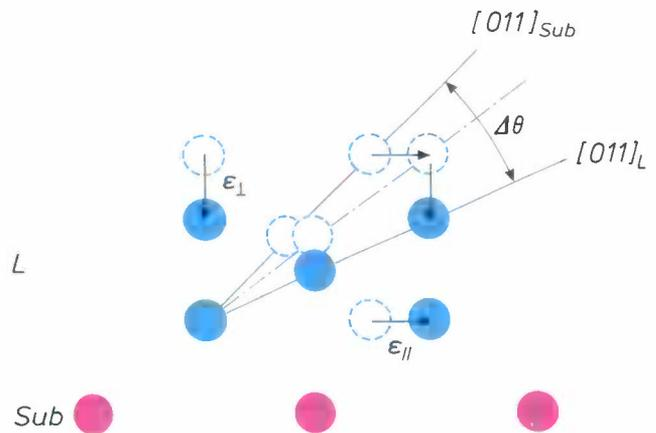
**Fig. 14.** Schematic illustration of the tetragonal lattice distortion in a film  $L$  with a smaller lattice constant than the substrate  $Sub$ . The parallel elongation by the coherency strain  $\epsilon_{||}$  induces a perpendicular stress  $\epsilon_{\perp}$  leading to a contraction (Poisson effect). The resulting tetragonal distortion corresponds to a tilt  $\Delta\theta$  in the [011] direction with respect to the substrate.
