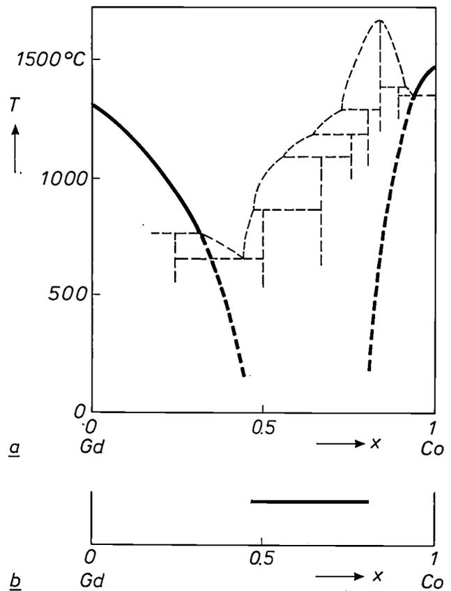
Fig. 8. Prediction of the composition range of an amorphous phase for the system gadolinium-cobalt; see also figs 6 and 7. *a*) Extrapolation of the liquidus curves in the phase diagram. *b*) The range thus found.
