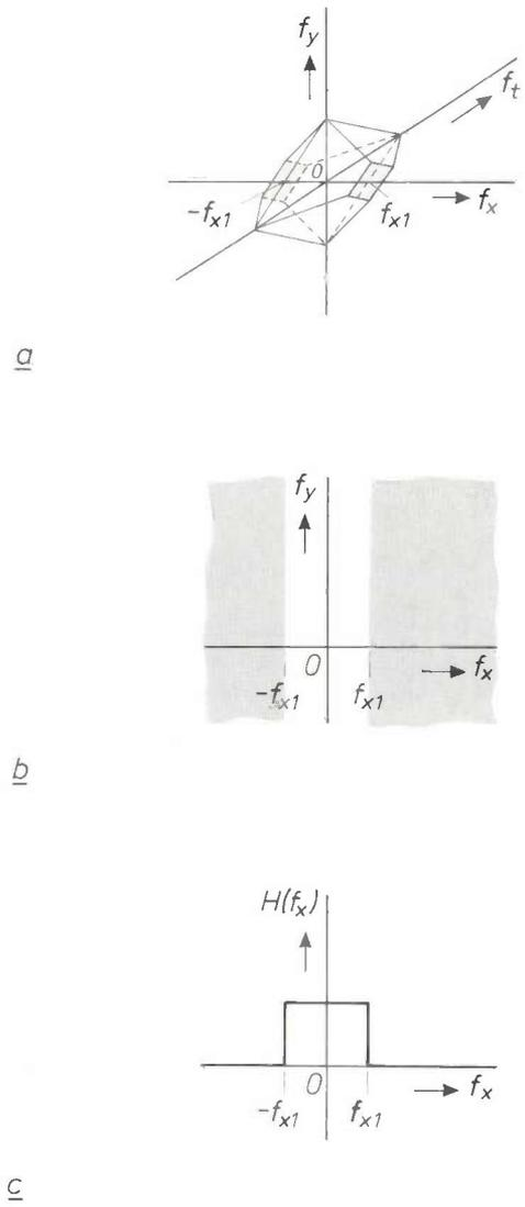
Fig. 9. a) An ideal horizontal lowpass filter with cut-off frequency  $f_{x1}$  restricts the spectrum of fig. 8a in the  $x$ -direction to the interval  $(-f_{x1}, f_{x1})$ . b) Two-dimensional representation of the ideal horizontal lowpass filter. c) Conventional one-dimensional representation  $H(f_x)$  of the same filter characteristic.
