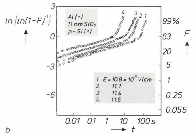
**Fig. 11.** a) Breakdown distribution for MOS capacitors with a high defect density. The arrows indicate the values of the field  $E$  at which time-dependent tests were carried out. b) Breakdown distribution in time-dependent tests on capacitors of (a) for four different field-strengths  $E$ . The sudden increases in the curves occur at about the same value of  $F$ .
