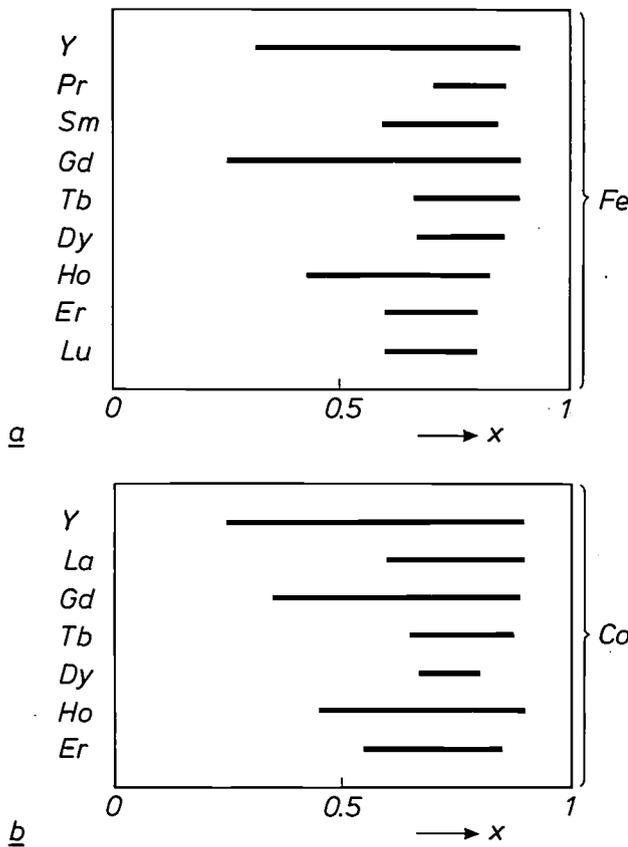
Fig. 7. Composition ranges in which amorphous material was found on quenching from the vapour phase *a*) for the combination of iron with yttrium and rare earths, *b*) for cobalt with yttrium and rare earths<sup>[2]</sup>.
