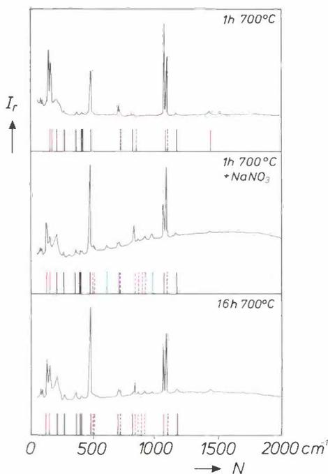
Fig. 5. As in fig. 4, but here the sample without  $\text{NaNO}_3$  has been heated again for a further 16 hours (below). Heating for one hour with  $\text{NaNO}_3$  (centre) is always found to produce more reaction products than heating for 16 hours without  $\text{NaNO}_3$ .
