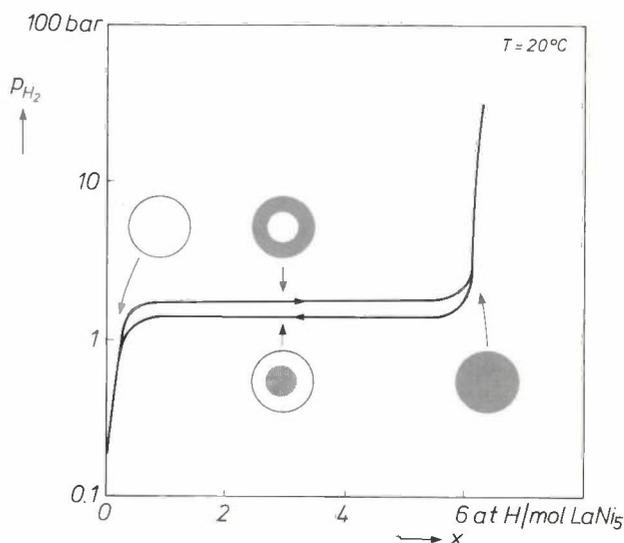
Fig. 18. Schematic representation of the phase boundary shift between the hydrogen-poor and hydrogen-rich phases in  $\text{LaNi}_5$  grains on charging and discharging. The hydrogen-poor phase is white, the hydrogen-rich phase is shown grey.
