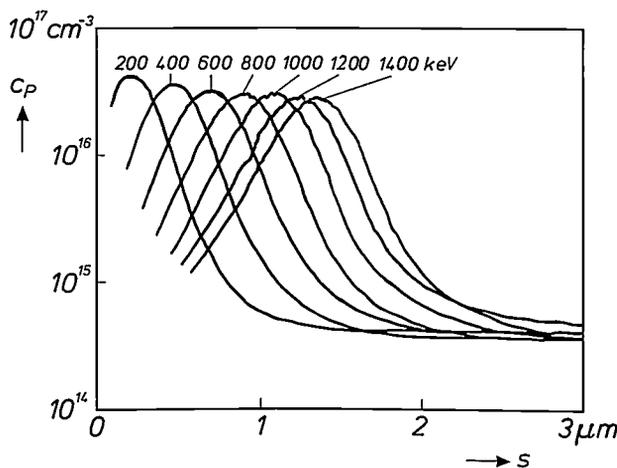
Fig. 15. Result of concentration-profile measurements made by the CV method [12]. The concentration  $c_p$  of phosphorus implanted in silicon is plotted as a function of the depth  $s$ . The different curves correspond to implantation energies from 200 to 1400 keV. Virtually any implantation profile can be obtained by combining a number of these or other curves.
