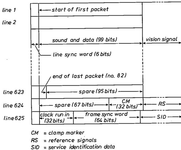
**Fig. 4.** General arrangement of a complete frame for a member of the MAC/packet family ('D2-MAC'), corresponding to a complete television picture of 625 lines. The intervals that correspond to one line period are shown here one above the other; in fact the picture information occupies about 5/6 of the line period (see *fig. 2*).
