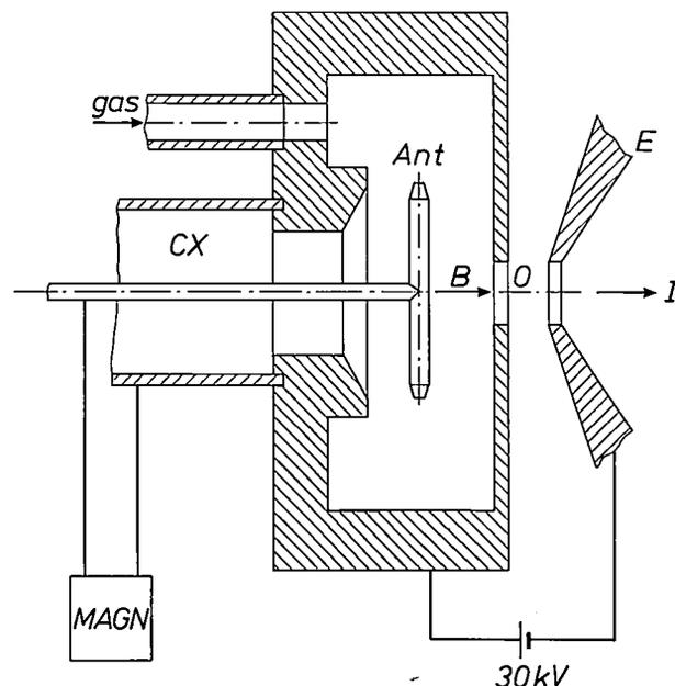
**Fig. 12.** The microwave source. This source is connected by a coaxial line *CX* to a magnetron *MAGN*, which supplies microwave energy to the plasma in the source. *Ant* antenna. See the captions to *figs 8 and 9*.
