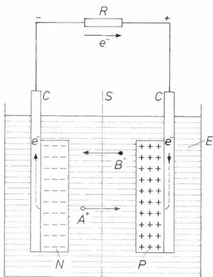
Fig. 3. Diagram of a current-producing galvanic cell.  $P$  active positive electrode material.  $N$  active negative electrode material.  $e$  electrons.  $E$  electrolyte.  $A^+$  positive ions.  $B^-$  negative ions.  $C$  current collectors.  $S$  separator.  $R$  external load.
