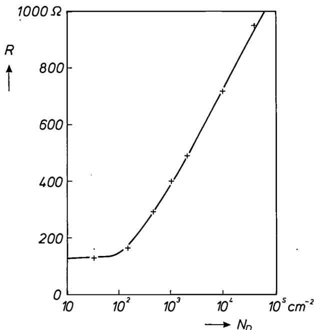
Fig. 5. A plot of the median equivalent series resistance  $R$  of devices as a function of dislocation density for 1.3 Mhz devices. An oscillator can be represented as an LC-circuit with a resistance in series. The quality factor  $Q_e$  of the device decreases with increasing equivalent resistance  $R$ . High dislocation densities imply a high  $R$  and thus a low  $Q_e$ .
