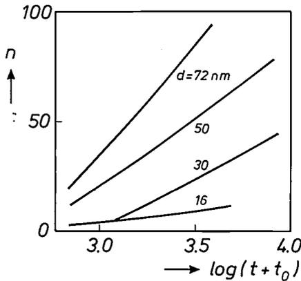
Fig. 3. Number of trapped charge carriers ( $n$ ) in arbitrary units plotted against  $\log(t + t_0)$ , see text, for different thicknesses  $d$  of the  $\text{SiO}_2$  film. These data are also derived from Young's results [6]. In all cases a straight line is found, as predicted by eq. (6).
