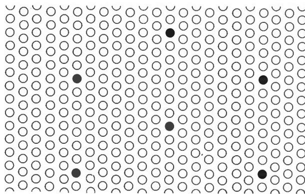
Fig. 2. Diagram of the atomic arrangement in the (111) surface of annealed silicon (the  $7 \times 7$  structure). The diagram shows the arrangement for a minimum deviation of the positions of the atoms, corresponding to a diffraction pattern as in fig. 1, with open circles for the normal positions and filled circles for the deviant positions<sup>[2]</sup>.
