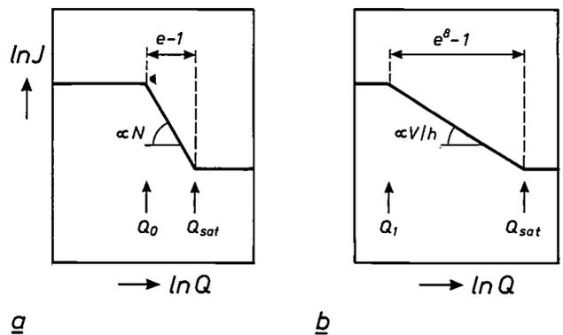
Fig. 4. Schematic curve of  $\ln J$  as a function of  $\ln Q$  as given by the first-order approximation (a) and after taking into account the Coulomb repulsion between injected electrons and electrons already trapped (b); see text. The main difference is that the sloping section in (a) is much steeper and the saturation point ( $Q_{\text{sat}}$ ) is reached much earlier than in (b).
