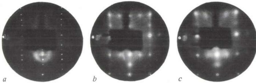
Fig. 6. LEED patterns from a (001) GaAs substrate (a) and Si films of thickness 1.4 nm (b) and 14 nm (c). On deposition, the surface reconstruction changes from  $c(8 \times 2)$  to  $(2 \times 1)$ ; the diffraction spots become more diffuse, indicating more crystal defects. The distance between the spots indicates that the 1.4-nm film has almost the same lattice constant as GaAs, whereas the lattice constant of the 14-nm film is 4% less and has the same value as for bulk Si.
