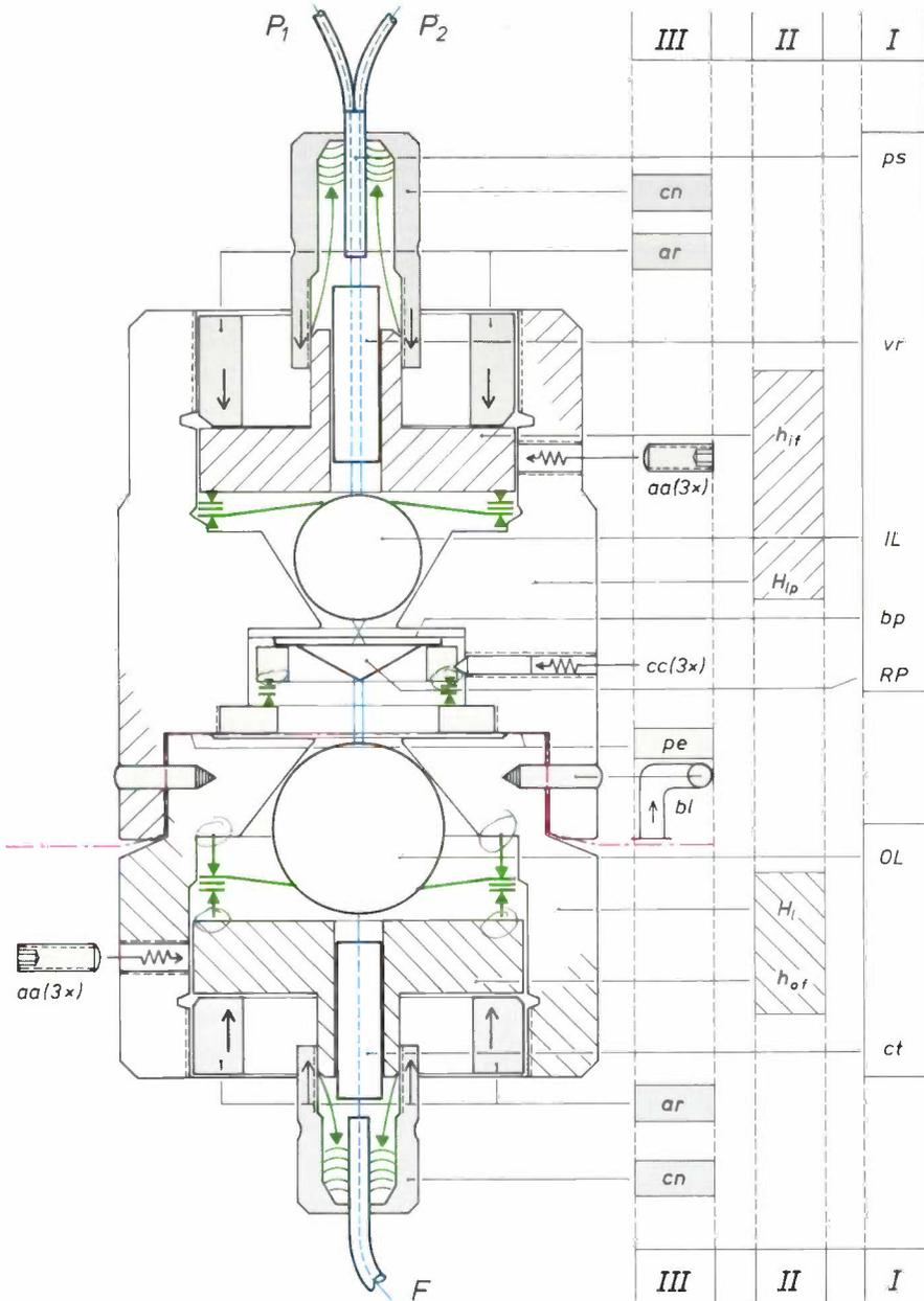
Fig. 5. Simplified diagram of the construction of a prism multiplexer with two input pigtailed ( $P_1$ ,  $P_2$ ; see also fig. 2a).  $F$  output fibre. The three groups of symbols refer to the signal path (I), the housing (II) and the localization mechanisms and components (III).
