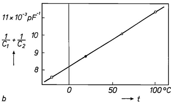
Fig. 6. a) The quantity  $1/C_1 + 1/C_2$  as a function of the differential pressure  $\Delta p$ , again with the temperature  $t$  as parameter. b) The quantity  $1/C_1 + 1/C_2$  as a function of the temperature  $t$  at  $\Delta p = 0$ .
