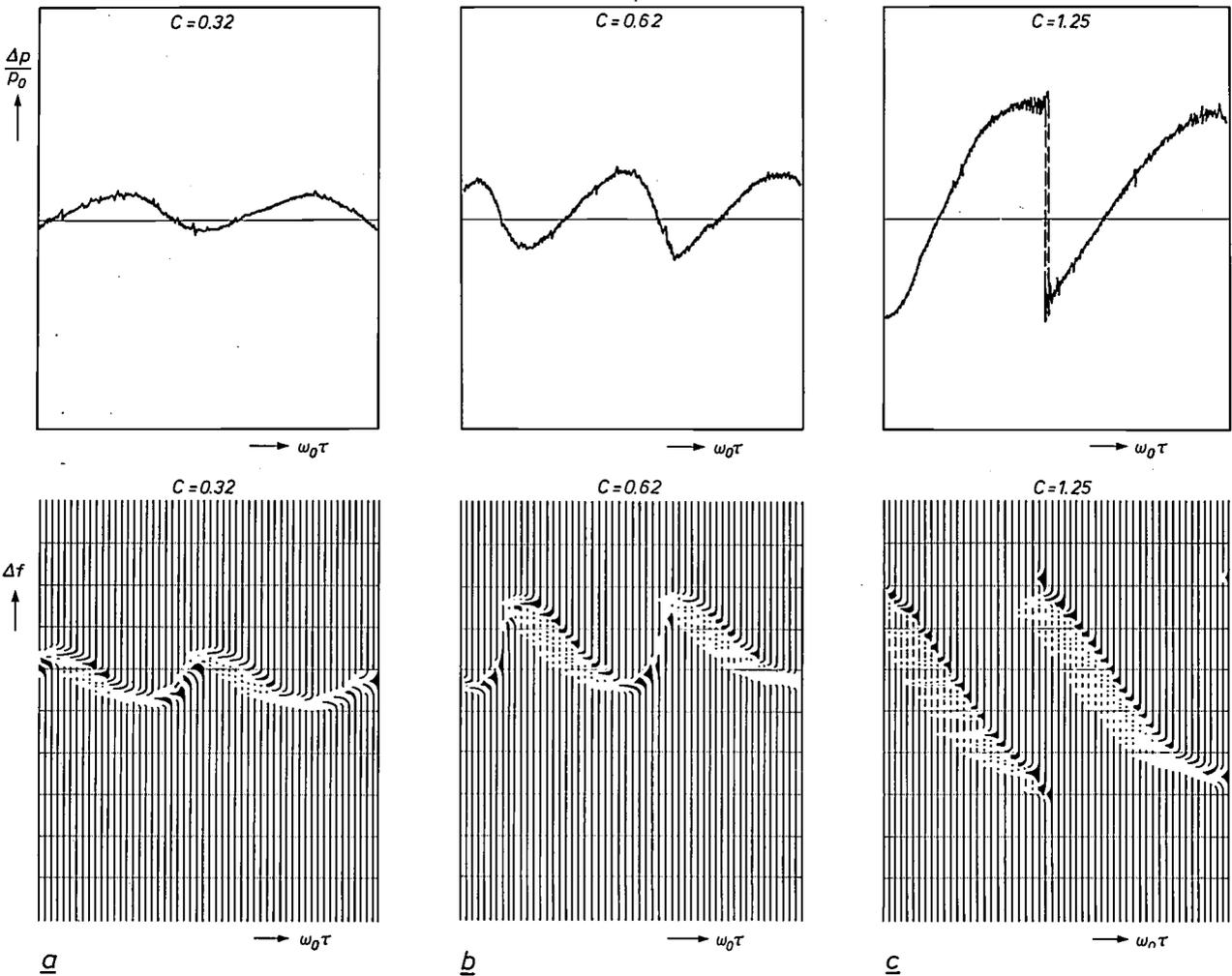
Fig. 9. The change in frequency ( $\Delta f$ ) and the relative power change ( $\Delta P/P_0$ ) of the laser radiation as a function of the phase ( $\omega_0 \tau$ ) of the feedback radiation for three values of the feedback. The factor  $C$  takes account of both the feedback fraction and the matching between the external and internal laser cavities. As  $C$  increases the feedback increases. a)  $C = 0.32$ . b)  $C = 0.62$ . c)  $C = 1.25$ .
