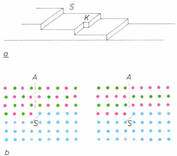
Fig. 1. *a*) Schematic representation of a surface of a single-crystal substrate showing steps *S* and a kink *K*. *b*) Two examples of atomic arrangements for a binary compound (e.g. GaAs) grown epitaxially on a substrate containing only one type of atom (e.g. Si). The difference in bonding leads to anti-phase boundaries *A* at steps *S* in the substrate surface.
