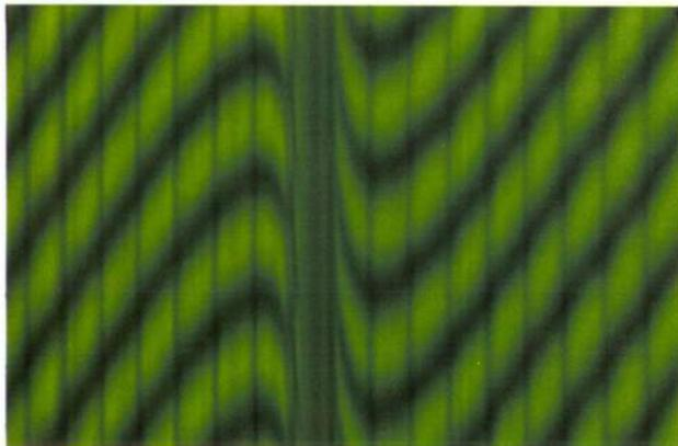
Fig. 7. Example of an interference pattern as observed near the absorption line at 546 nm (the transition from  $7^3S_1$  to  $6^3P_2$ ). The vertical pattern of fringes is due to interferences that occur in the dye laser between two partially reflecting surfaces, and is used for calibrating the wavelength scale. The distance between two vertical fringes corresponds to 0.03 nm.
