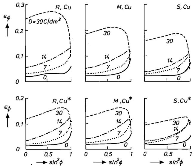
Fig. 6. Directional thermal emissivity  $\epsilon_\phi$  at 133 °C plotted against  $\sin^2\phi$  for black-cobalt coatings of different electrolytic thickness  $D$ . The substrates used are rough (R), medium (M) or smooth (S) and they are coated with 1 μm of copper from a cyanide solution (Cu) or 5 μm of bright copper (Cu\*). It can be seen that the coating thickness is the most important parameter for the directional emissivity.
