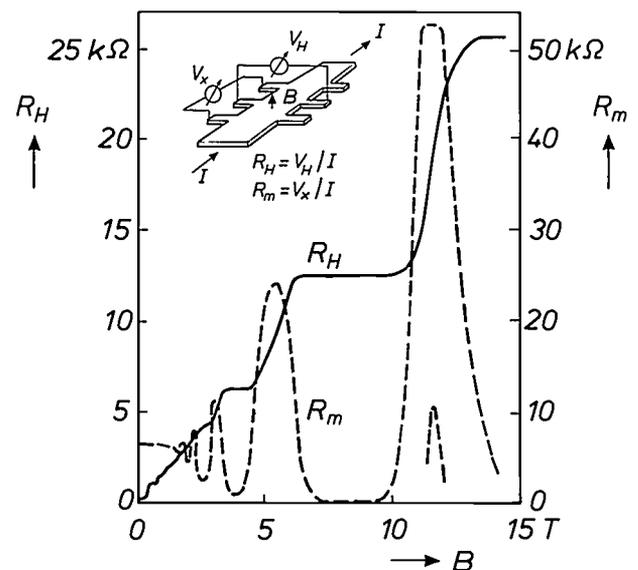
Fig. 20. Quantized Hall effect for a modulation-doped heterostructure based on  $\text{Al}_{0.3}\text{Ga}_{0.7}\text{As}$  and GaAs, with a two-dimensional electron gas. The Hall resistance  $R_H$  ( $V_H/I$ ) and magnetoresistance  $R_m$  ( $V_x/I$ ), measured at 4 K, are given as a function of the magnetic flux density  $B$  (in the  $z$ -direction). At certain values of the flux density there is a plateau in the curve for  $R_H$  and there is a minimum for  $R_m$ .
