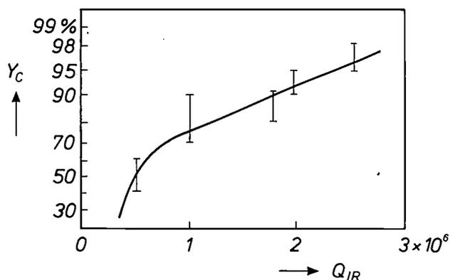
Fig. 7. Yield  $Y_C$  of unbroken 0.5 mm thick plates in a production process as a function of  $Q_{IR}$ . The data are for plates made with reciprocating slurry saws. When rotating wheels are used, yields are worse [6]. Note that the graph was drawn on probability paper so that the scale of  $Y_C$  varies in a nonlinear manner.
