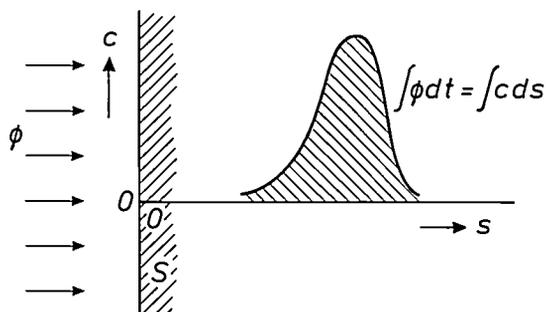
Fig. 1. Diagram of a concentration profile. *S* sample, typically a silicon slice, whose surface intersects the plane of the diagram at the vertical axis. *c* concentration of implanted ions. *s* depth from surface.  $\phi$  ion-flux density. *t* time.
