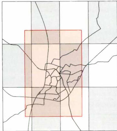
**Fig. 10.** Partitioning of the map into 'parcels' — the white and grey rectangles. When the computer requests map data from the rectangle shown red, a list of addresses (the directory) supplies the location of the sectors on the Compact Disc where the nine blocks with information about the required nine parcels are stored.
