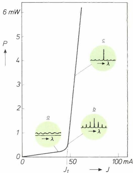
Fig. 5. Optical power  $P$  of the laser as a function of the current  $J$ . The spectrum of the laser is shown for a number of current values. *a*) Spontaneous-emission spectrum, *b*) multimode spectrum, *c*) single-mode spectrum.
