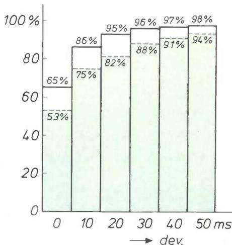
**Fig. 11.** The percentage of 'automatic' phoneme boundaries that deviate by less than an indicated multiple of 10 ms from the 'non-automatic' phoneme boundaries. The dashed lines with the corresponding percentages indicate the results of the second method, the continuous lines give the results of the combination of the two methods. In total 979 phonemes boundaries were determined in 90 words.
