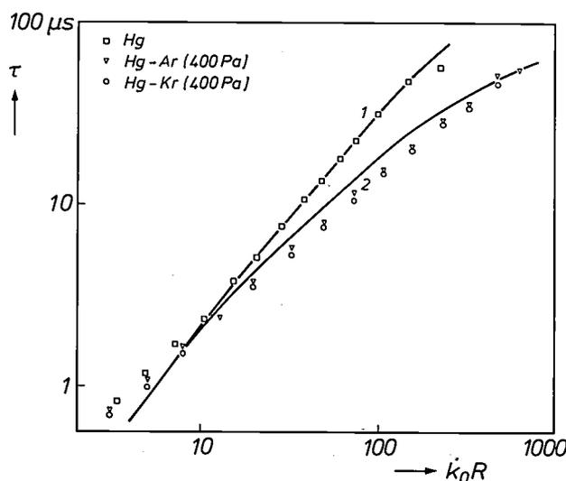
Fig. 3. The effective radiation lifetime ( $\tau$ ) of the  $6^3P_1$  level of mercury atoms in a mercury discharge, a mercury/argon discharge and a mercury/krypton discharge as a function of  $k_0R$ . The pressure of the inert gas is 400 Pa in both cases and the diameter of the tube is 36 mm. The continuous lines relate to the lifetime calculated from the theory due to P. J. Walsh <sup>[10]</sup>, for a mercury discharge (1) and for a mercury/argon discharge (2).
