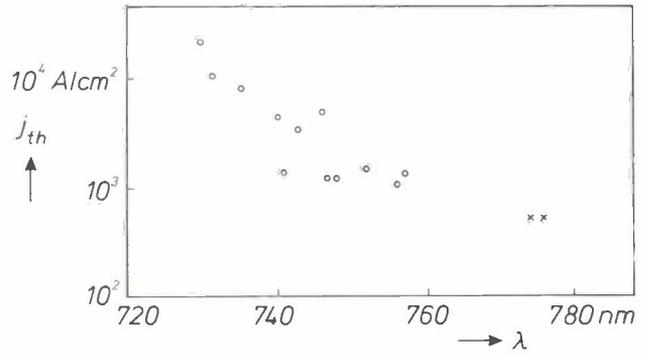
Fig. 12. Threshold current density  $j_{th}$  plotted against laser emission wavelength  $\lambda$  at room temperature for four-well lasers obtained from the same wafer (circles) and for two single-quantum-well lasers (crosses). The pulse duration was  $2\ \mu\text{s}$  with a repetition rate of 500 Hz. The shorter the emission wavelength, the higher the threshold for laser operation. No laser operation was detected below  $730\ \text{nm}$ .
