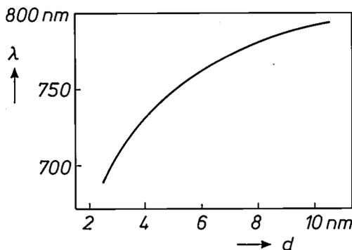
Fig. 7. Calculated relation between well thickness  $d$  and emission wavelength  $\lambda$  corresponding to the recombination of electrons and heavy holes in the  $n = 1$  state, for a rectangular GaAs quantum well between  $\text{Al}_{0.54}\text{Ga}_{0.46}\text{As}$  barriers. For a decrease in thickness from 12 to 2.5 nm the calculated reduction in wavelength is from 800 to 680 nm.
