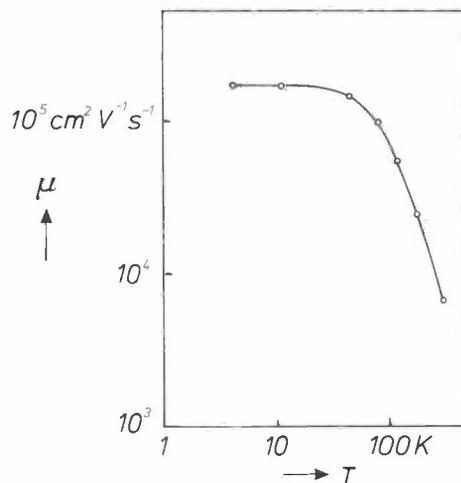
**Fig. 18.** Decrease in the electron mobility  $\mu$  with temperature  $T$  for a modulation-doped heterostructure based on  $\text{Al}_{0.35}\text{Ga}_{0.65}\text{As}$  and GaAs with a spacer thickness of  $15 \text{ nm}$ .
