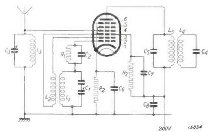
Fig. 1. Circuit diagram of the octode. The circuit  $L_1, C_1$  is tuned to the auxiliary oscillation.  $L_2, C_2$  to the incoming signals,  $L_3, C_3$  and  $L_4, C_4$  to the intermediate frequency.
