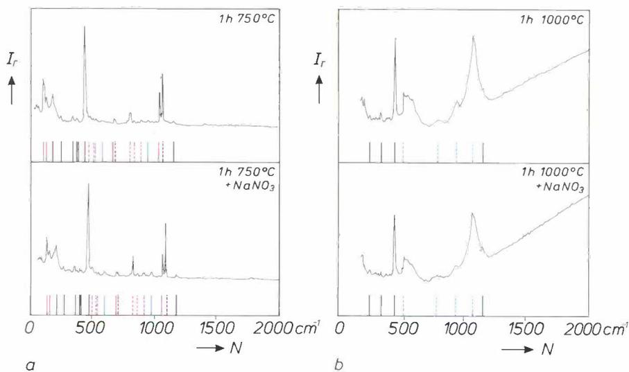
Fig. 4. As fig. 3, but here the spectra shown below originate from samples with added  $\text{NaNO}_3$ . The peaks here have been identified as originating from  $\alpha$ -quartz (short black vertical line),  $\text{Na}_2\text{CO}_3$  (black dashed line);  $\text{BaCO}_3$  (red line),  $\text{Ba}_2\text{SiO}_4 + \text{Na}_2\text{Si}_2\text{O}_7$  (red dotted line),  $\text{BaSiO}_3$  (blue line) and liquid disilicate (blue dashed line).
