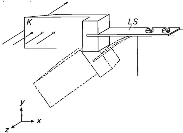
Fig. 6. The knife-edge  $K$ , which is connected to the system by a leaf spring  $LS$ , is correctly positioned by energizing a magnet. The movement takes place in the direction of the edge ( $y$ -direction), perpendicular to the optical axis ( $z$ -direction) and takes 50 ms. The edge of the knife is ground to prevent unwanted reflections in the direction of the diode array.
