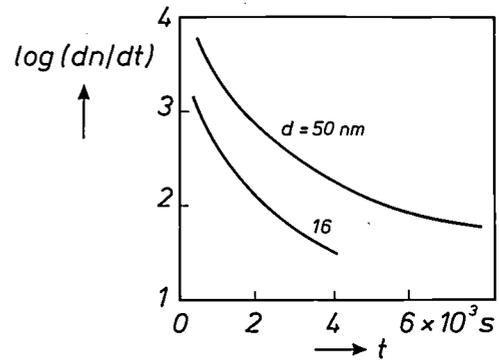
Fig. 2. Logarithm of the trapping rate  $dn/dt$  for charge carriers in  $\text{SiO}_2$  as a function of the duration  $t$  of the applied voltage, for two thicknesses  $d$  of the oxide film. The data are derived from results reported by D. R. Young [6]. The first-order approximation, which predicts the straight lines given by eq. (2), is clearly not applicable here.
