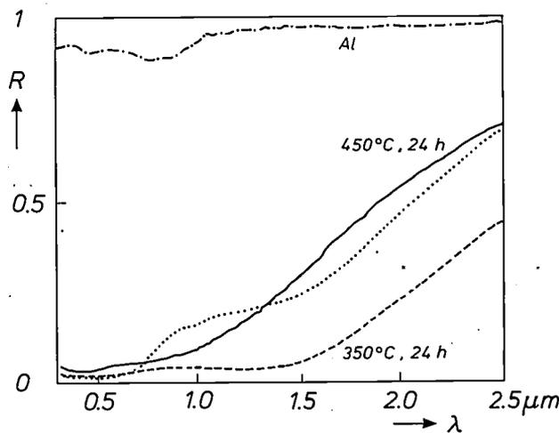
Fig. 5. Effect of vacuum annealing on the reflectance in the solar wavelength range, for a cobalt coating of 14 C/dm<sup>2</sup> on smooth steel coated with 5 μm of bright copper. Annealing for 24 h at 350 °C (dashed curve) results in an appreciable decrease in reflectance as compared with the non-annealed coating (dotted curve). After annealing for a further 24 h at 450 °C (continuous curve) the original near-infrared reflectance is almost completely restored.
