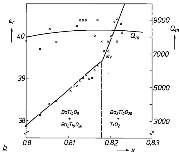
Fig. 3. Part of the phase diagram of the quasi-binary system  $BaO-TiO_2$  [6].  $t$  temperature.  $x$  molar quantity of  $TiO_2$ . b) Relative permittivity  $\epsilon_r$  and Q-factor  $Q_m$  as a function of  $x$ , as the result of a number of measurements with the arrangement of fig. 1a. The regions for the two-phase ceramics  $BaTi_4O_9 - Ba_2Ti_9O_{20}$  and  $Ba_2Ti_9O_{20} - TiO_2$  are separated by a dashed line.
