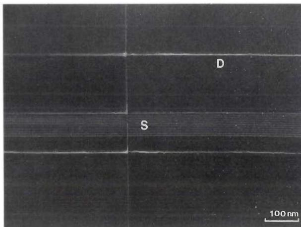
**Fig. 9.** Transmission electron micrograph of a planar section of an MBE-grown Si film 100 nm thick on (001) GaP, showing dislocations *D* along the interface and stacking faults *S* intersecting the Si film.
