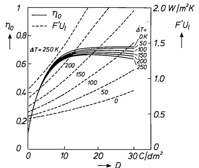
Fig. 13. Calculated performance of a solar collector (VTR 361 tubes with heat pipe and an aluminium reflector). The conversion efficiency  $\eta_0$  and the heat-loss coefficient  $F'U_1$  (see text) are plotted against the electrolytic thickness  $D$  of optimized coatings for different values of the average difference  $\Delta T$  between the heat-transfer fluid temperature in the upper heat pipe and the ambient temperature.
