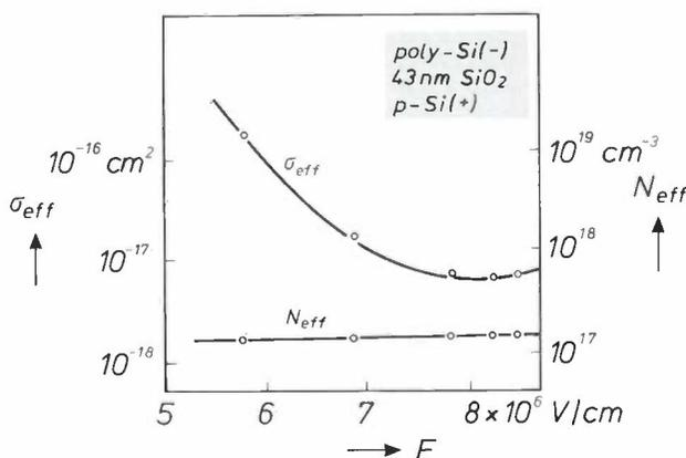
Fig. 6. Effective cross-section  $\sigma_{eff}$  for electron trapping in the  $SiO_2$  film of the MOS device in fig. 5, and the effective density  $N_{eff}$  of the trapping centres, as a function of the applied field-strength  $E$ . Whereas  $N_{eff}$  is independent of  $E$ , the value of  $\sigma_{eff}$  first decreases with  $E$  until a virtually constant value is reached at high  $E$ .
