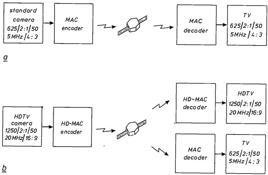
Fig. 5. a) With standard equipment for encoding and decoding MAC signals good television quality can be obtained via broadcasting satellites. b) By using an HDTV camera and an HD-MAC encoder at the transmitting end it is possible — depending on the receiving equipment — to obtain both a standard-quality display and the much better 'high-definition' quality.
