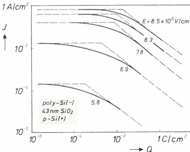
Fig. 5. Log-log plot of the current density  $J$  measured in a MOS device as a function of the charge transferred per unit area ( $Q$ ) for different field-strengths  $E$ . As eq. (13) indicates curves with two asymptotes (dashed lines) are obtained:  $\ln J$  is constant at low  $Q$  and decreases linearly with  $\ln Q$  at high  $Q$ .
