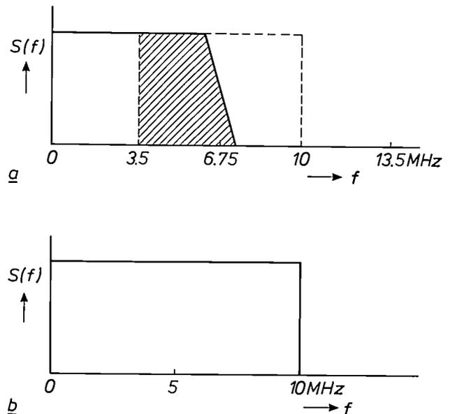
Fig. 15. a) If sub-Nyquist sampling ('subsampling') is used, a 'constructive' form of aliasing is obtained. Here this takes place in the frequency range between about 3.5 and 6.75 MHz. b) By applying the correct 'interpolating' filter operations we can reconstruct the original frequency components from this. The original frequency band from 0 to 10 MHz thus becomes available again without distortion.
