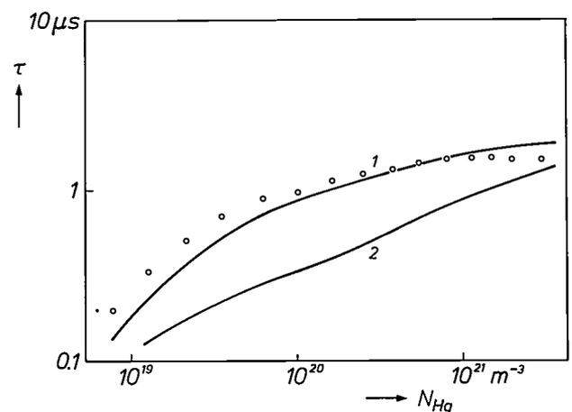
Fig. 5. The effective radiation lifetime ( $\tau$ ) of the  $6^1P_1$  level of mercury atoms in a mercury/argon discharge with a diameter of 36.5 mm, as a function of the mercury vapour density  $N_{\text{Hg}}$ . The circles indicate our experimental results, the continuous lines 1 and 2 are calculated lifetimes [13]. For the calculation of curve 2 complete spectral redistribution was assumed, but not for curve 1.
