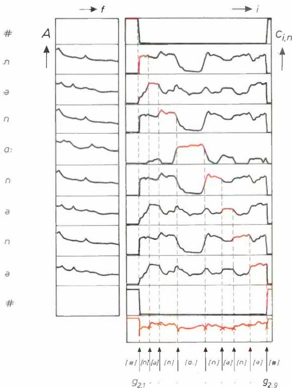
Fig. 6. The spectral states, the associated reference spectra  $n$  and the correlation  $c_{i,j}$  between the reference spectra and the test spectra in the word 'nanaanene'. The arrows below indicate the boundaries  $g_{2,n}$ , as determined subject to the condition that the total sum of the correlations between the boundaries must be as large as possible.  $A$  is the amplitude,  $i$  the test spectrum and  $f$  the frequency.
