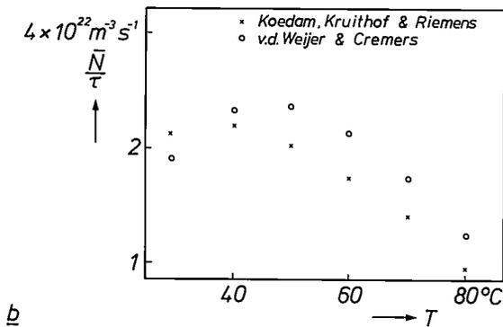
Fig. 11. a) The measured radiation outputs [20] at a wavelength of 254 nm as a function of the wall temperature  $T$  of the tube of a mercury discharge (diameter 38 mm, discharge current 450 mA), and the values that we calculated from the density  $N$  and the lifetime  $\tau$ . b) The measured radiation output [21] at a wavelength of 254 nm of a mercury/argon discharge (diameter 36 mm, argon pressure 400 Pa, discharge current 400 mA) and our calculated values.
