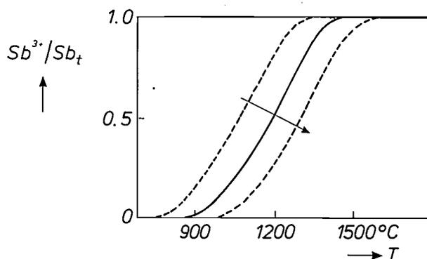
Fig. 7. The ratio  $\text{Sb}^{3+}/\text{Sb}_T$  for raw-materials samples as a function of the temperature to which the samples have been subjected for 20 hours, at varying values of the initial oxygen activity (increasing in the direction of the arrow).
