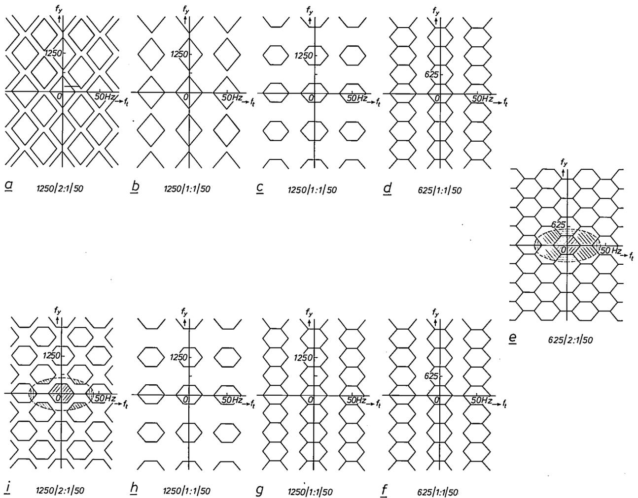
**Fig. 12.** Two-dimensional spectra in the  $(f_t, f_y)$ -plane at various points in the block diagram of fig. 11. The letters *a*, *b*, ... correspond in these two figures. (In this figure the limits of human visual perception appear as an ellipse instead of a circle as a result of the altered scale division in the vertical direction.)
