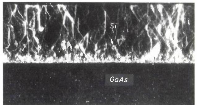
**Fig. 13.** Dark-field cross-sectional TEM image along the [110] direction of 200-nm MBE-grown Si on (001) GaAs. The Si film has a high density of dislocations, whereas no defects are observed in the GaAs substrate. Many dislocations run in  $\langle 112 \rangle$  directions.
