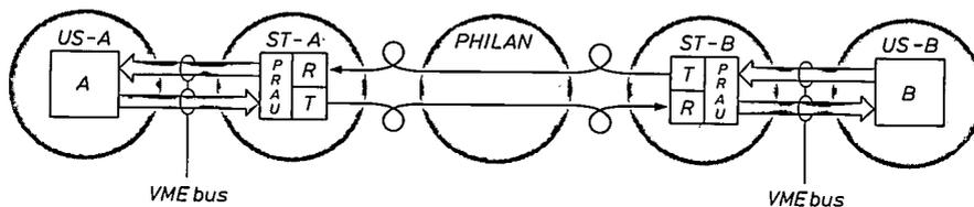
Fig. 9. Simplified representation of a packet-switched link between users *US-A* and *US-B*. Between each user and the corresponding station *ST* electrical signals are exchanged via a standardized connection, called a VMEbus. The stations are connected by fibre-optic cables with the rest of the PHILAN system (not further specified here). *PRAU* ring access unit for packet-switched traffic. *R* optical receiver. *T* optical transmitter.
