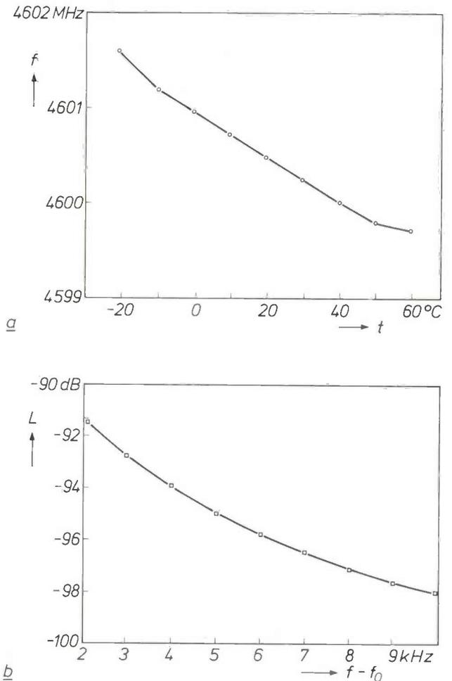
Fig. 12. a) Plot of the frequency  $f$  as a function of temperature  $t$  for the oscillator with transmission-type resonator in fig. 11b. (The corresponding temperature coefficient of  $-5.1 \times 10^{-6} \text{ }^\circ\text{C}^{-1}$  can be improved by using a somewhat different composition for the resonator material.) b) The (single-sideband) power density spectrum of the phase noise of the oscillator with reaction-type resonator in fig. 11a. See also the caption to fig. 9.
