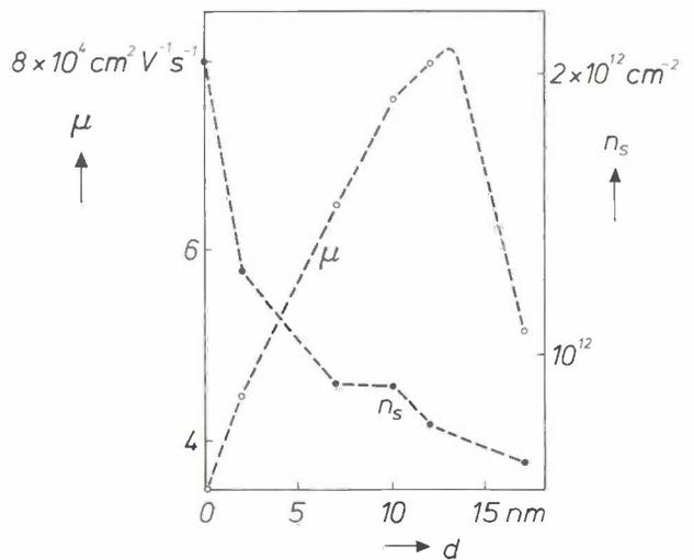
**Fig. 17.** Effect of spacer thickness  $d$  on the electron mobility  $\mu$  at  $77 \text{ K}$  and the sheet electron density  $n_s$ , determined by Hall measurements on the modulation-doped heterostructures of *fig. 16*<sup>[19]</sup>. With increasing spacer thickness the sheet electron density decreases monotonically, whereas there is a maximum in the electron mobility.
