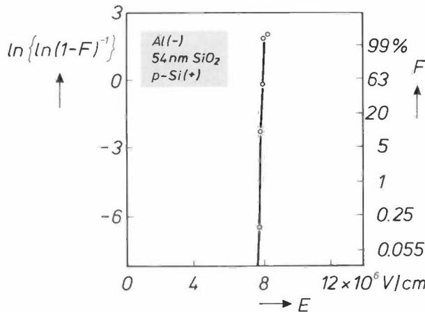
**Fig. 10.** Breakdown distribution for 16000 capacitors, each with an area of  $0.02 \text{ mm}^2$ . The capacitors contain so few defects that they only give intrinsic breakdown, and all of them fail at virtually the same field-strength.
