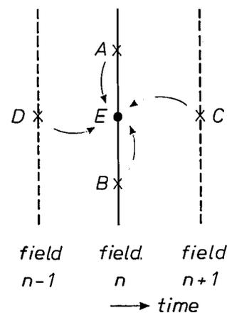
Fig. 16. Calculation of the missing line *E* in scan conversion (the picture lines are perpendicular to the plane of the diagram). If *E* is calculated from *A* and *B* we have intra-field processing. If *E* is calculated from *C* and *D* we have inter-field processing. If all four of *A*, *B*, *C* and *D* are used, we are performing spatio-temporal processing.
