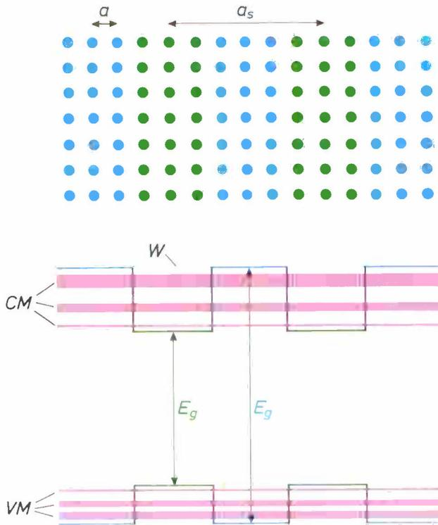
Fig. 1. Atomic arrangement and energy-band diagram of a superlattice consisting of alternate ultra-thin layers of two semiconductors with different band gaps  $E_g$ . In addition to the normal lattice period  $a$ , there is also a superlattice period  $a_s$ . At the interfaces the band-gap difference creates potential wells  $W$ , which split the valence and conduction bands into valence minibands  $VM$  and conduction minibands  $CM$ .
