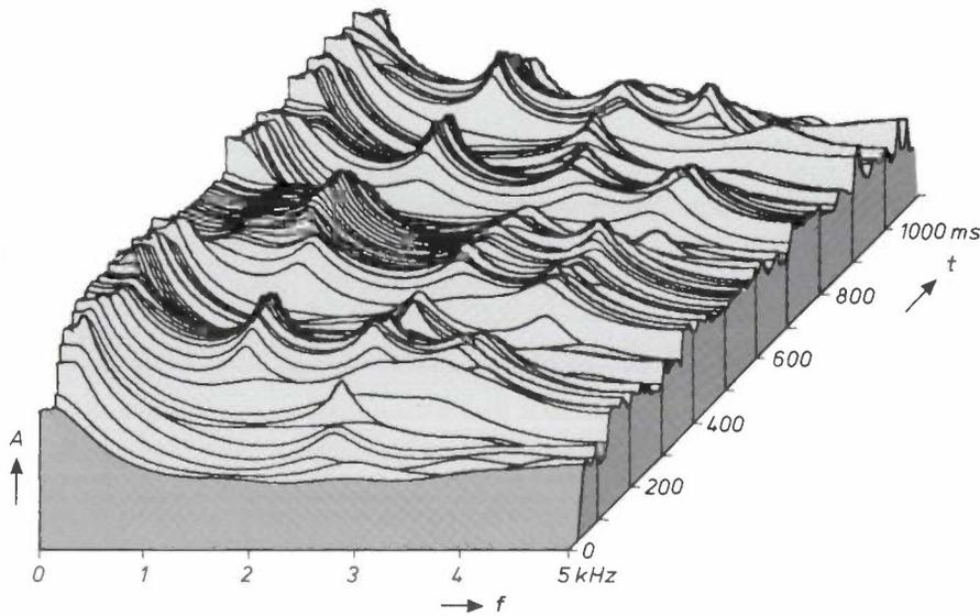
Fig. 3. The spectra (the amplitude  $A$  as a function of frequency  $f$ ) as determined every 10 ms from the speech signal of the word 'nenaanene'. In most spectra five maxima can be recognized. These are the formants, and their heights and positions vary with time. These signals give the basis for dividing the utterance into steady-state parts.
