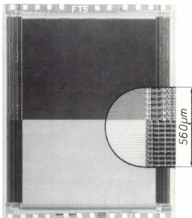
**Fig. 8.** The accordion imager. The storage section (the light region) is smaller than the image section (the dark region). The storage section is shielded from light by an aluminium layer. The n-channels are vertical, the CCD electrodes horizontal. On the left and right are the shift registers, which generate the voltages on the CCD electrodes. *Insert:* enlarged view of the transition from image section to storage section.
