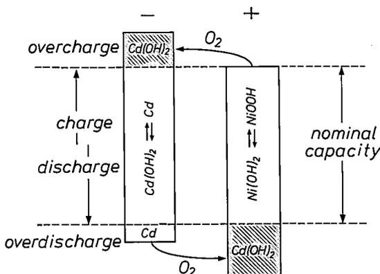
Fig. 4. Diagram illustrating the protection from overcharging and overdischarging in a sealed cadmium battery, introduced in about 1950. Adding  $\text{Cd}(\text{OH})_2$  to both electrodes introduces an oxygen cycle during both overcharging (blue region) and overdischarging (red region). The added  $\text{Cd}(\text{OH})_2$  is indicated by hatching. An excess of cadmium (red) is also added at the cadmium electrode; this is explained on p. 32.
