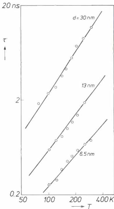
Fig. 13. Log-log plots of the luminescence decay time  $\tau$  against the absolute temperature  $T$ , for three quantum wells of GaAs (thickness  $d$ ) between two layers of  $\text{Al}_{0.33}\text{Ga}_{0.67}\text{As}$ . The exponent of the temperature dependence can be derived from the slopes of the lines.
