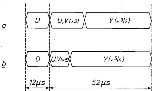
Fig. 2. In the MAC system each line period of  $64 \mu s$  contains one of the two colour-difference signals  $U$  or  $V$  and the luminance signal  $Y$  in a compressed form, one after the other. Two combinations of compression factors are possible: a) 3 and  $3/2$ , or b) 5 and  $5/4$ . The rest of the line period (the flyback time  $D$ ) is used for sound signals, synchronization signals, etc.
