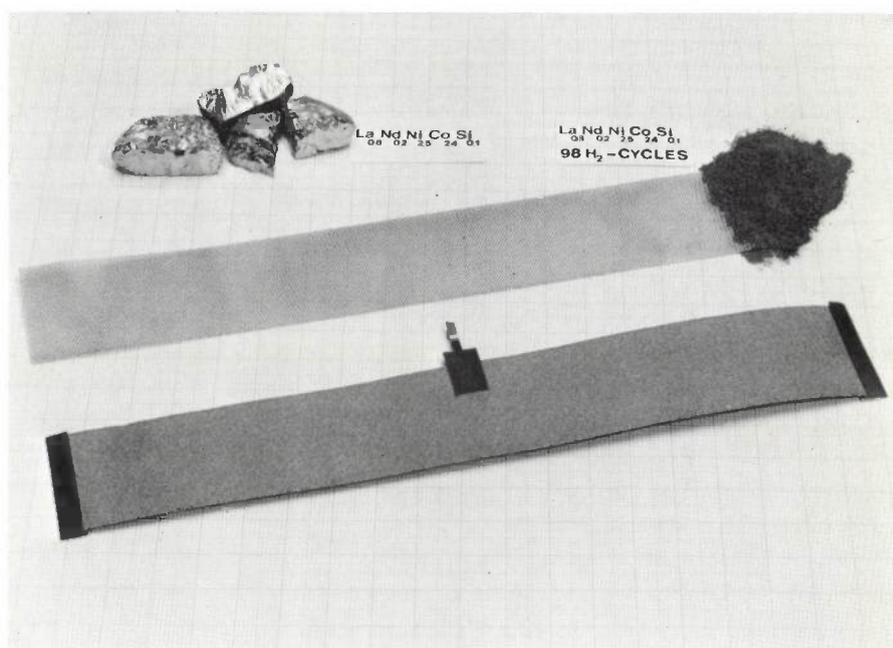
Fig. 20. One of our methods of manufacturing the hydride electrode. Metal castings of composition  $\text{La}_{0.8}\text{Nd}_{0.2}\text{Ni}_{2.5}\text{Co}_{2.4}\text{Si}_{0.1}$  (top left) are pulverized by repeated absorption and desorption of hydrogen gas (top right) and the resultant powder is applied as a paste to a strip of expanded nickel.
