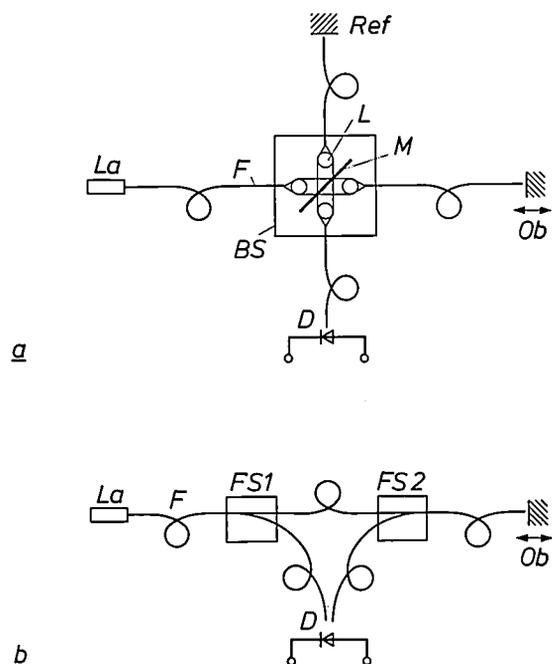
**Fig. 1.** Schematic diagram of a Michelson interferometer in which the light path is determined by optical fibre. *a*) Version with a conventional beam-splitter. *La* laser. *D* detector. *Ref* reference plane. *Ob* object whose movement is measured (in the direction indicated). *F* fibres. *BS* beam-splitter. *b*) Version with two fibre-splitters *FS1* and *FS2*. Other symbols as under (*a*).
