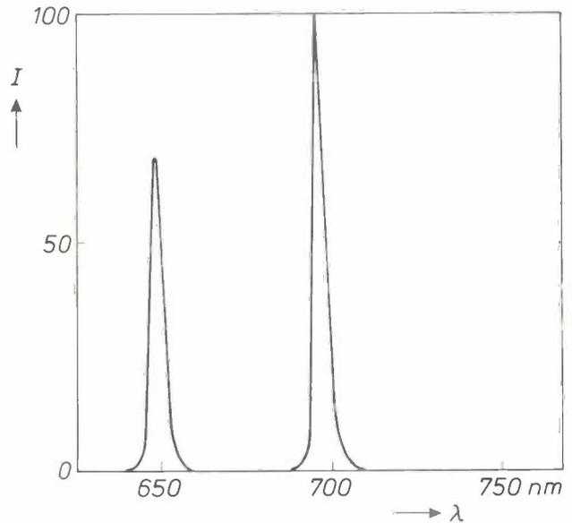
Fig. 13. Photoluminescence spectrum at 4 K on excitation with 514.5-nm argon-laser radiation of a sample containing two  $\text{Al}_{0.2}\text{Ga}_{0.8}\text{As}$  quantum wells of thickness 3 and 8 nm and  $\text{Al}_{0.5}\text{Ga}_{0.5}\text{As}$  barriers. The combination of a narrow well and Al incorporation gives a very short emission wavelength.
