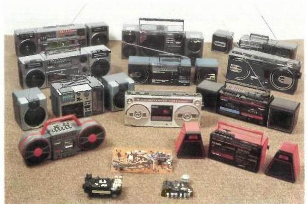
**Fig. 4.** Family of stereo cassette recorders all based on two types of drive mechanism for the cassettes (foreground) and a circuit board (behind it). Depending on the type of recorder, all of the electronic components on the board are used, or only some of them.
