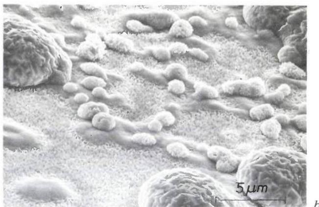
**Fig. 9.** SEM micrographs of two coatings, showing the effect of annealing for 24 h at  $450^\circ\text{C}$  in poor vacuum, with an insufficient coating of copper on the steel substrate. For a cobalt coating of  $60 \text{ C/dm}^2$  on  $1 \mu\text{m}$  of cyanidic copper (a) large outgrowths are formed. For a coating of  $14 \text{ C/dm}^2$  on  $0.5 \mu\text{m}$  of cyanidic copper (b) many outgrowths of different sizes are observed.
