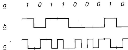
Fig. 11. *a*) Arbitrary bit stream consisting of ones and zeros. *b*) Corresponding 'uncoded' binary signal; a '1' is represented by a high level and an '0' by a low level. *c*) The same bit stream after biphasic encoding. A '1' is now represented by a sequence of a high level and a low level, an '0' by the reverse. This encoding gives a transmission signal with a better frequency spectrum, and the required clock signal is easier to recover at the receiver end.
