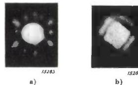
Fig. 3. a) The diffraction pattern of a natural pearl always exhibits a sixfold symmetry.
