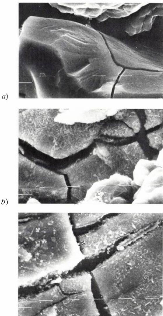
Fig. 16. SEM micrograph of  $\text{La}_{0.8}\text{Nd}_{0.2}\text{Ni}_{2.5}\text{Co}_{2.4}\text{Si}_{0.1}$  electrodes after zero (a), 41 (b) and 666 (c) charge/discharge cycles. One 'dash' represents 1  $\mu\text{m}$ .
