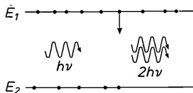
Fig. 1. Laser action can occur when the energy level  $E_1$  of the atoms or molecules of a material contains more electrons than the lower energy level  $E_2$ . An incident photon of energy  $h\nu = E_1 - E_2$  causes the emission of a second photon with the same energy and phase as the original photon.
