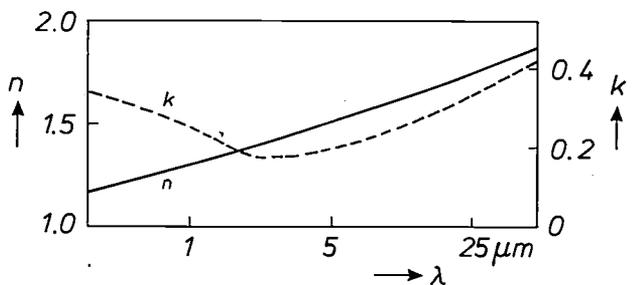
Fig. 3. Refractive index  $n$  and absorption index  $k$  of black-cobalt coatings as a function of the wavelength  $\lambda$ . Whereas  $n$  increases monotonically with  $\lambda$ , there is a minimum for  $k$  at about 2.5  $\mu\text{m}$ .
