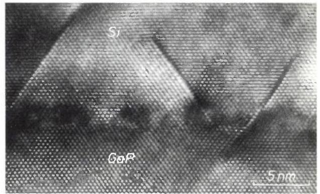
**Fig. 11.** High-resolution electron microscopy (HREM) cross-sectional image along the [110] direction of MBE-grown Si on (001) GaP, showing dissociated 60° dislocations close to the interface.
