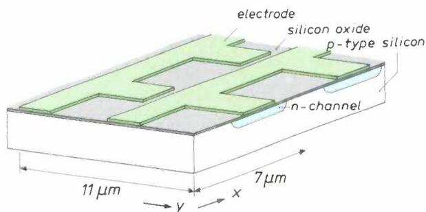
**Fig. 7.** Diagram showing the arrangement of the CCD electrodes and n-channels in the image section of the accordion imager. The electrodes are shaped in such a way that they do not cover the entire surface but leave some of the p-type material and a part of the n-channels accessible to incident light. This increases the blue sensitivity of the sensor. The polysilicon electrodes absorb light strongly in the blue wavelength range.
