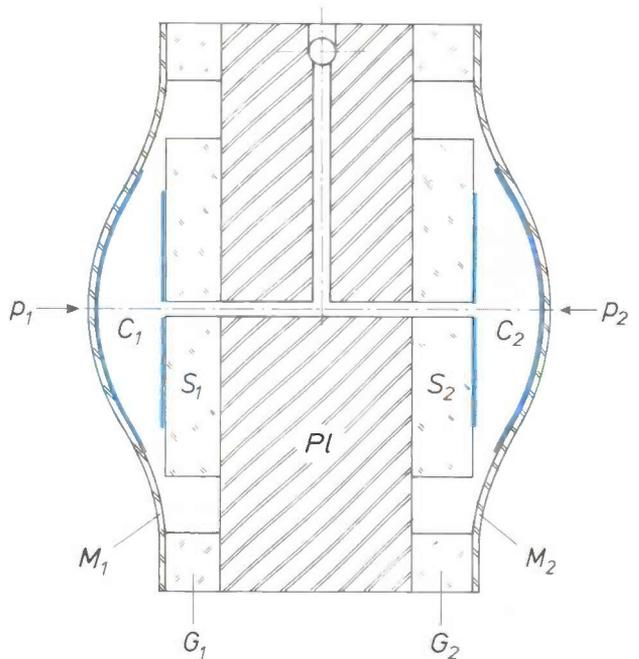
Fig. 4. Construction of the differential-pressure transducer.  $G_1$ ,  $G_2$  glass-solder rings.  $S_1$ ,  $S_2$  layers forming substrates for the inner electrodes.  $G_1$ ,  $G_2$ ,  $S_1$  and  $S_2$  are applied by screen printing (as in thick-film technology). See also the caption to fig. 1.
