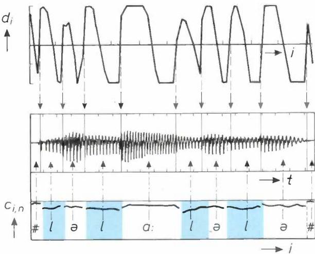
Fig. 9. The distance function  $d_i$ , the speech signal and the correlation  $c_{i,n}$  between the spectral states  $\{ \#, [l], [ə], [l], [a:], [l], [ə], [l], [ə], \# \}$  and the spectra for the word 'lelaalele'. The phoneme boundaries finally determined are shown in the speech signal.
