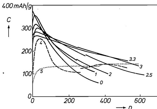
Fig. 13. The effect of substituting cobalt for nickel in  $\text{LaNi}_5$  on the curve for the storage capacity  $C$  as a function of the number of charge/discharge cycles ( $n$ ). The number of nickel atoms replaced by cobalt atoms is shown beside each curve. The optimum effect is found when 3.3 nickel atoms are replaced by cobalt.
