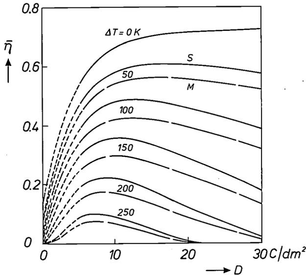
Fig. 14. Annual efficiency  $\bar{\eta}$  of a Philips evacuated tubular collector as a function of the electrolytic coating thickness  $D$ , calculated for two different European climatic zones (S Southern Europe, M Central Europe) and for different values of the mean operating temperature difference  $\Delta T$ . The optimum coating thickness can be derived for a given application with a known value of  $\Delta T$ .
