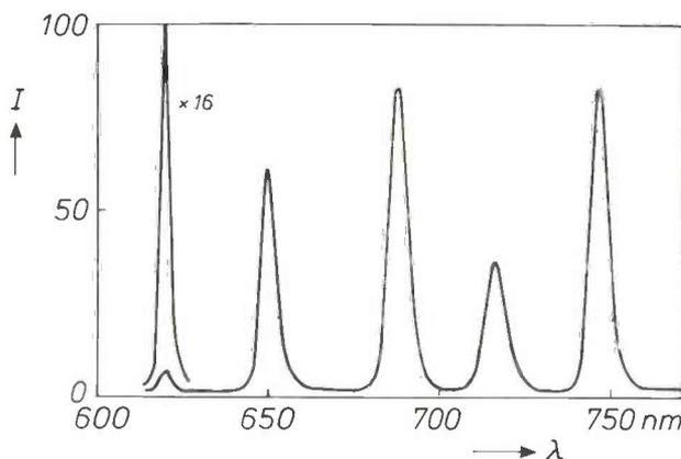
**Fig. 10.** Photoluminescence spectrum of a sample with five GaAs quantum wells, excited at 4 K with an argon laser emitting at 514.5 nm. The thinnest well, with an estimated thickness of only about 0.6 nm, has a weak emission peak at a very short wavelength (620 nm).
