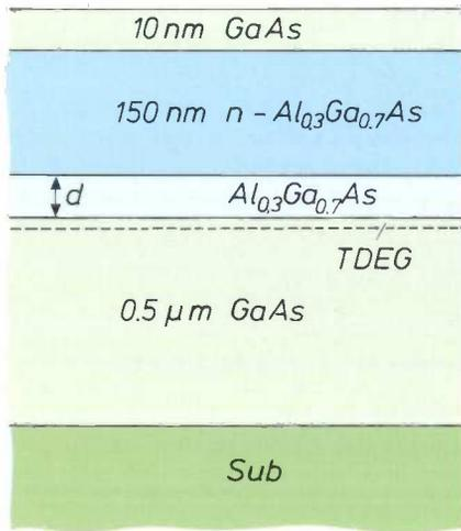
**Fig. 16.** Cross-section of a typical modulation-doped heterostructure on a Cr-doped semi-insulating GaAs substrate. Below the spacer of thickness  $d$  a two-dimensional electron gas (TDEG) is formed. The  $n\text{-Al}_{0.3}\text{Ga}_{0.7}\text{As}$  layer contains  $7.5 \times 10^{17} \text{ cm}^{-3}$  of Si atoms.
