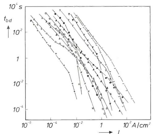
Fig. 13. Log-log plot of the time to breakdown ( $t_{bd}$ ) against current density  $J$ , for MOS capacitors with differences in the gate (aluminium or polysilicon), in the thickness of the  $\text{SiO}_2$  film (between  $10$  and  $50 \text{ nm}$ ) and in the manufacturing process. If the current densities are not too high, straight lines with a slope of about  $-1$  are obtained.
