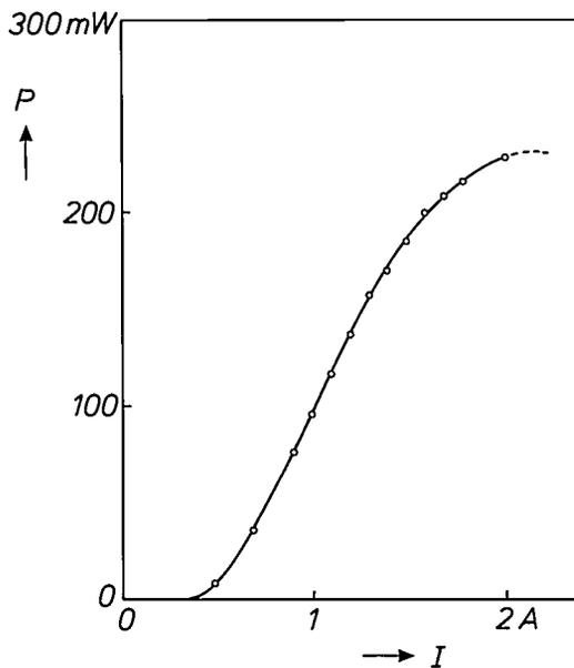
Fig. 14. Power  $P$  emitted per facet as a function of current  $I$  for a quantum-well laser of the type shown in fig. 11b with  $l = 500 \mu\text{m}$ , operating at room temperature and emitting at 775 nm. The threshold current is 0.50 A, corresponding to a current density of 660 A/cm<sup>2</sup>. A maximum power of 230 mW is obtained.
