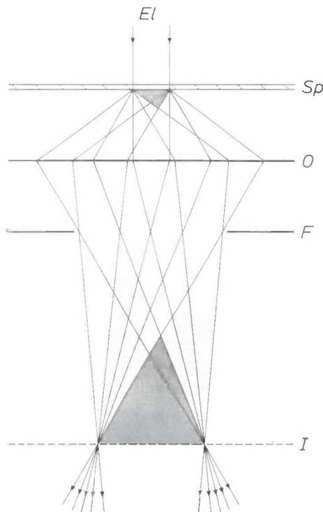
Fig. 6. Ray diagram for a high-resolution TEM micrograph. The electron beam  $EI$  is incident on the specimen  $Sp$  in the direction of (say) the [110] axis. The beams produced by diffraction from the crystal planes are focused by an objective lens  $O$  on to the back focal plane  $F$ . The diffraction pattern formed by the combination of a large number of diffracted beams results in an image of the crystal lattice at the image plane  $I$ .
