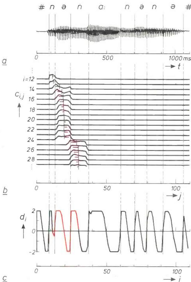
Fig. 5. The speech signal (a), the correlation  $c_{i,j}$  for a part of the speech signal (b) and the distance function  $d_i$  (c) derived from the correlation. The lines indicating the phoneme boundaries derived from the zero crossings (from - to +) of the distance function are extended to the speech signal.
