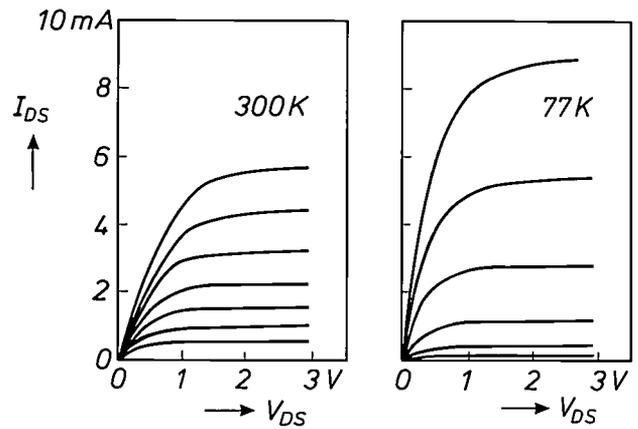
Fig. 19. Characteristic curves of drain-source current  $I_{DS}$  plotted against drain-source voltage  $V_{DS}$  for a HEMT device at 300 and 77 K, with the gate voltage varying in steps of 200 mV. The transconductance, derived from the spacings between the curves, increases threefold from 300 to 77 K.
