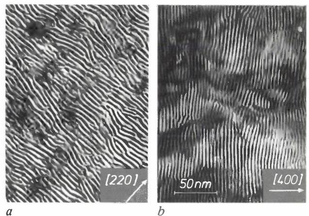
**Fig. 12.** Bright-field TEM images of a planar section of an Si film 200 nm thick on (001) GaAs for diffraction at (220) planes (*a*) and (400) planes (*b*). Both images show Moiré fringes, approximately perpendicular to the diffraction vector in the [220] and [400] directions. The periodicity corresponds to the 4% lattice mismatch. The distortions of the fringes are due to the presence of dislocations, which are more pronounced in (*a*) than in (*b*).
