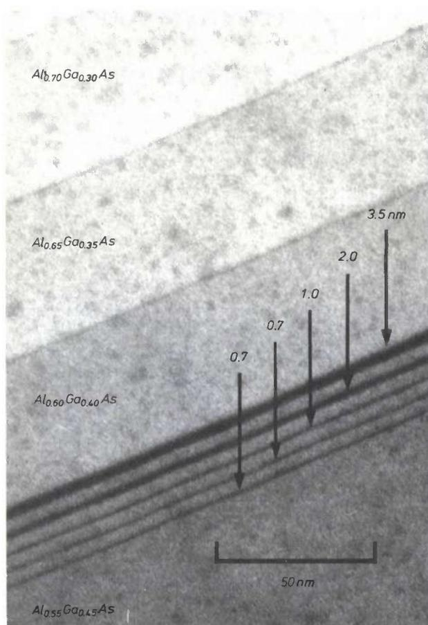
Fig. 8. TEM dark-field image, with  $I_{002}$ , of the bottom part of the multilayer structure of fig. 3. The GaAs layers (dark) have a thickness ranging from 0.7 to 3.5 nm. The  $\text{Al}_x\text{Ga}_{1-x}\text{As}$  layers become brighter as  $x$  increases; an increase of 0.05 is clearly visible.
