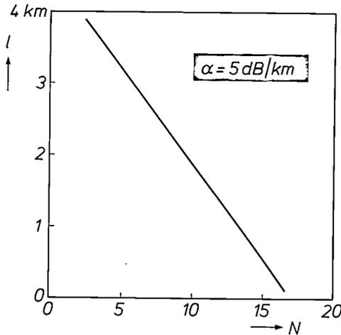
Fig. 6. For each connection point some attenuation of the signal circulating in the ring must be taken into account. In PHILAN the number of connection points  $N$  per meander and the maximum meander length  $l$  are related by the straight line shown (for a fibre-optic cable with an attenuation of 5 dB/km and a maximum permissible total attenuation in wall receptacles and glass fibre of just over 22 dB).
