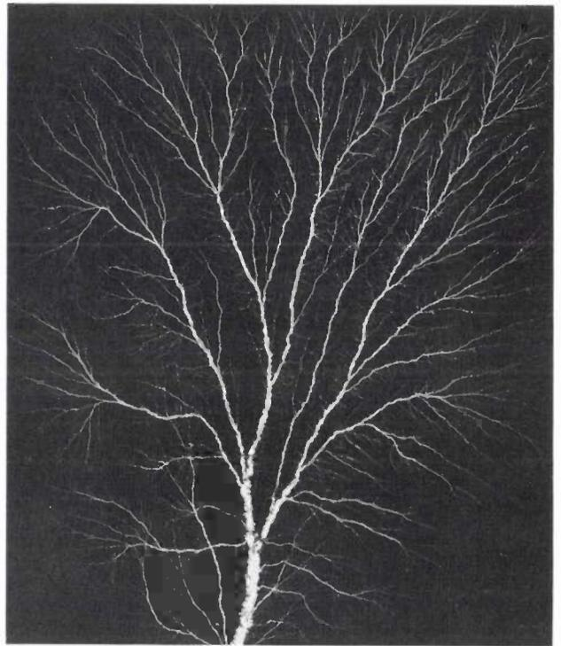
Fig. 18. Tree-shaped discharge pattern after injection of 3-MeV electrons into an insulator that was then earthed at a central point<sup>[16]</sup>.
