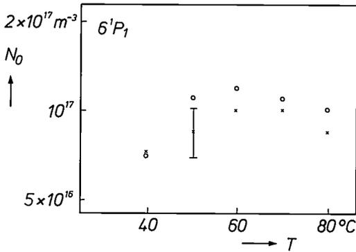
Fig. 10. The density  $N_0$  at the  $6^1P_1$  level as a function of the mercury vapour pressure in a mercury/argon discharge. The diameter of the discharge tube was 15 mm, the discharge current was 500 mA and the argon pressure was 400 Pa.  $\circ$  Calculated densities,  $\times$  experimental data. The vertical line indicates the experimental error.
