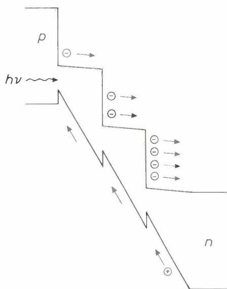
**Fig. 3.** Energy-band diagram of a 'staircase' superlattice for an avalanche photodiode<sup>[4]</sup>. The electrons generated by the incident photons can only ionize the atoms in the crystal at the steps in the conduction band. The creation of new electrons therefore occurs at well-defined positions in the lattice. This reduces the statistical fluctuations in the electron multiplication.
