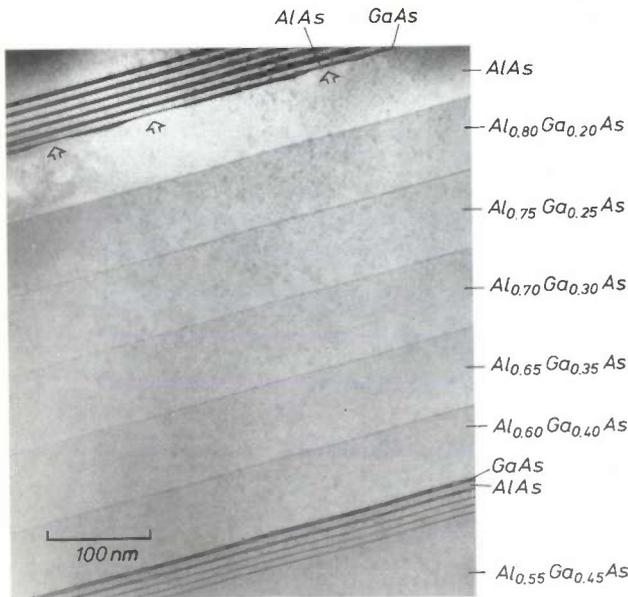
Fig. 7. TEM dark-field image, with (002) diffraction, of a multilayer structure of  $\text{Al}_x\text{Ga}_{1-x}\text{As}$  grown as in the diagram of fig. 3. Layers with low  $x$  (Al-poor) appear dark compared with layers with high  $x$  (Al-rich), as indicated by eq. (8). The arrows indicate undulations at the AlAs surface.
