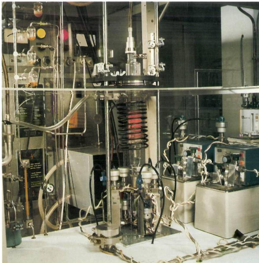
**Fig. 2.** Part of the experimental MO-VPE arrangement for growing layers of  $\text{Al}_x\text{Ga}_{1-x}\text{As}$ . The reactor with gas inlet at the bottom is shown at the centre, and the valves for admitting the various components are arranged around it radially. The substrate is heated to the required temperature in the reactor by r.f. induction in the susceptor. The thermostatic baths with bubbling vessels containing the metal-organic compounds are on the right.
