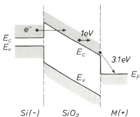
Fig. 16. Energy diagram for electron transfer in a MOS capacitor.  $E_v$  upper edge of the valence band.  $E_c$  lower edge of the conduction band.  $E_F$  Fermi level of the metal. The energy gain for an electron is much greater in the transition to the metal  $M$  than in migration in the conduction band of SiO<sub>2</sub>.
