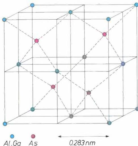
Fig. 5. Unit cell of  $\text{Al}_x\text{Ga}_{1-x}\text{As}$ . The Al/Ga atoms form a face-centred cubic lattice: they are situated at the corners of the unit cell and at the centre-points of the six faces. The As atoms fill half the number of the available tetrahedral interstices. The coordinates of the atoms in the unit cell are given in equation (4). The lattice constant is 0.566 nm.
