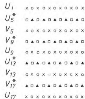
**Fig. 18.** Quincunx sampling is also used for each of the two colour-difference signals in HD-MAC. Because only one of the two difference signals is transmitted in each line, the sampling pattern shown here is obtained. (The symbols have the same significance as in *fig. 14* and *fig. 17*.)
