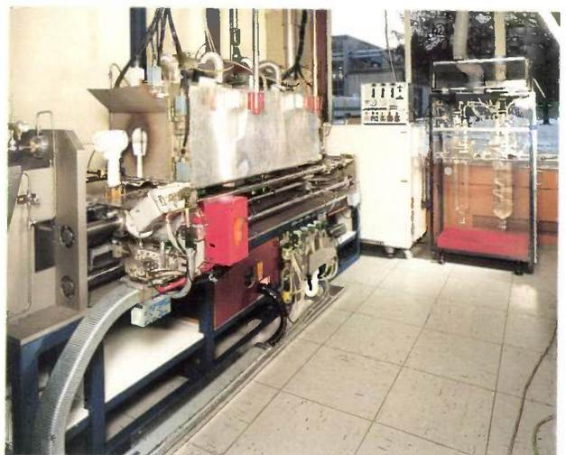
Fig. 7. a) Diagram of the PCVD process. *GSS* gas-supply system. *MWC* microwave cavity. *PL* plasma. *PU* pump system. *CU* control unit. *QT* quartz-glass tube. *F* furnace. b) The laboratory arrangement. The cavity can be seen on the left of the furnace insulation; it is white and encloses the quartz-glass tube.
