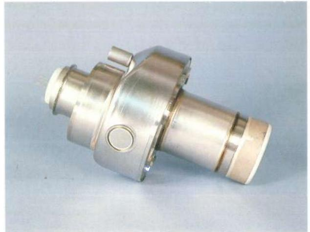
Fig. 1. The new Philips MRC200 diagnostic X-ray tube with an anode mounted in spiral-groove bearings lubricated by liquid metal. The anode diameter is 200 mm. The rated input is 85 kW<sup>[7]</sup>.
