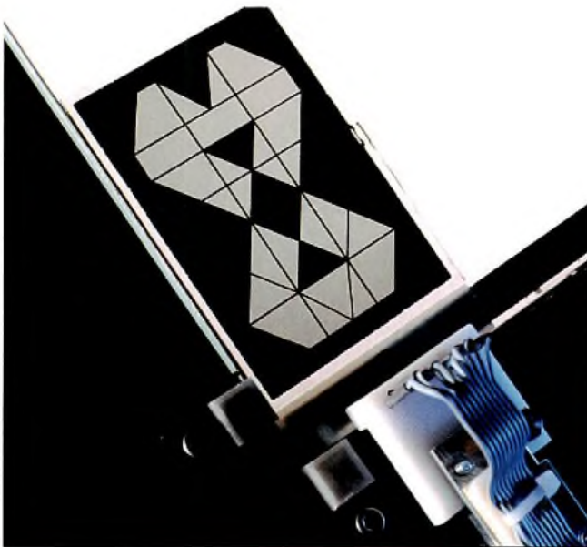
Before the chip-on-glass bond is cured, the module undergoes a full functional test
