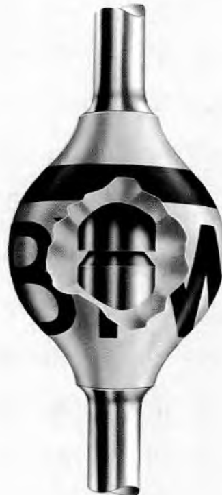
Cut-away view of a SOD-57 glass-bead diode package as used for the BYW54 family showing the robust, hermetic construction used
