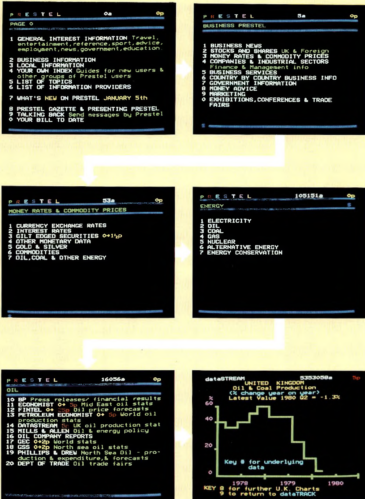
Fig.3 Typical sequence of Prestel displays, illustrating the page selection process
