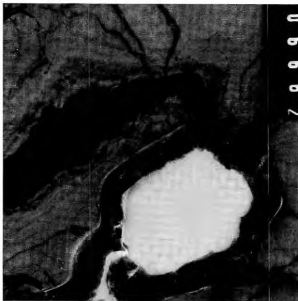
Fig.4 Electron photomicrograph (about 60 000x) showing oxide layer in one of the anode pores
