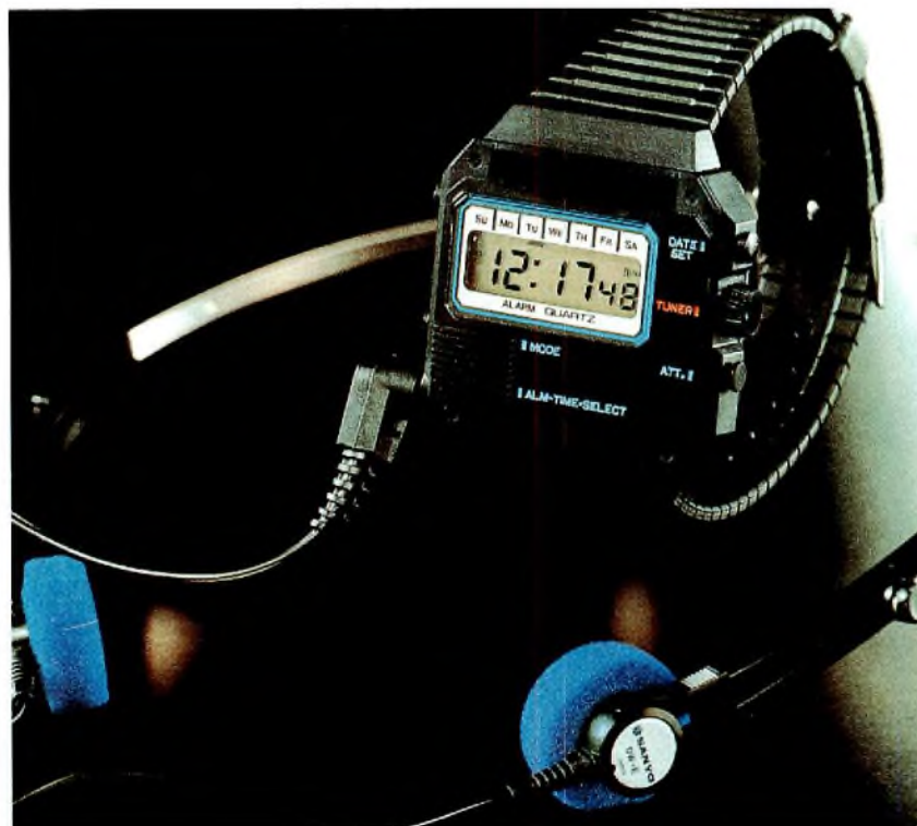
The TDA7000 allows f.m. radios to be made small enough to fit inside a pencil, a cigarette lighter, or a wristwatch
