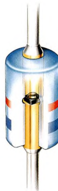
Fig.6 Glass encapsulated diode
