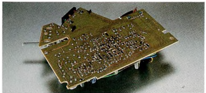
Fig.3 Typical example of a mixed print: in this video camera viewfinder, leaded components are on one side of the board and SMDs on the other
