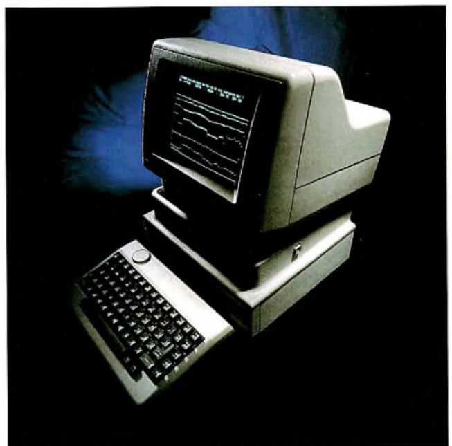
68000 — computing power for Hewlett Packard's HP9816
