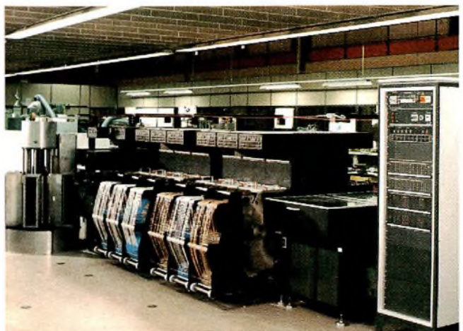
Fig.4 Simultaneous/sequential placement machine with a capacity of more than 200 000 SMDs an hour. Each of the quick-change tape magazines has a capacity of 32 reels with up to 10 000 SMDs per reel
