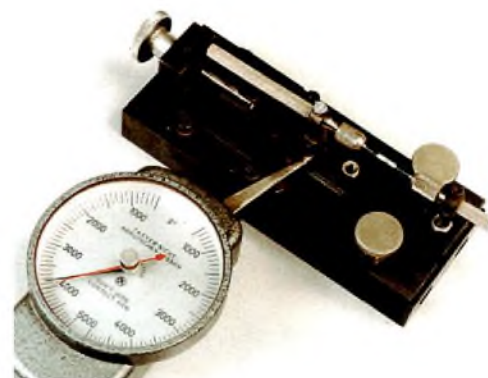
Regular tensile stress testing of our reed switches helps ensure that their high performance will be unimpaired by the handling they receive during assembly into finished products
