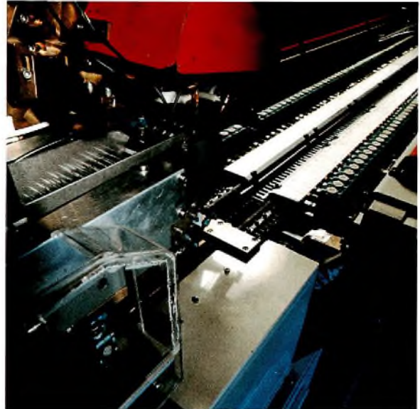
Computer-controlled sorting of varicaps into groups with similar capacitance ratio
