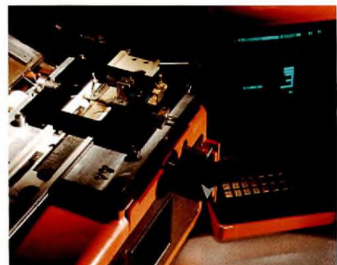
Modern, computer-controlled test equipment, such as the plating-thickness measuring facility, plays a vital part in our quest for even higher quality reed switches
