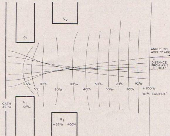
Fig. 8—Equipotentials and electron paths in cathode  $G_1$ - $G_2$  space, normal voltages, zero  $G_1$  bias.
