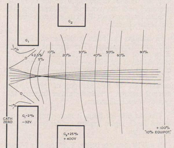
Fig. 7—Equipotentials and electron paths in cathode  $G_1$ - $G_2$  space, normal voltages.
