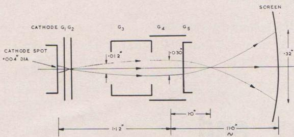
Fig. 16—Beam under cathode test conditions showing magnification of cathode spot.
