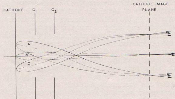
Fig. 17—Idealised picture of formation of cathode image.
