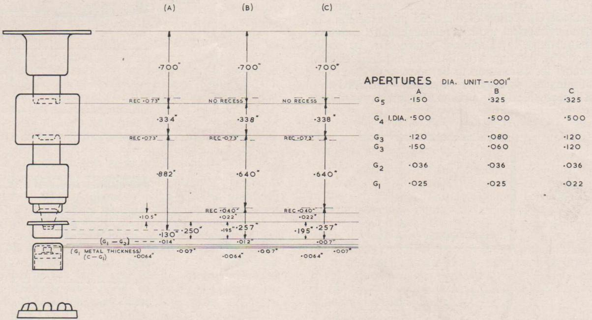
Fig. 1—Dimensions of three CRT guns.
