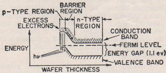
Fig. 9—Energy model of a silicon solar cell.
