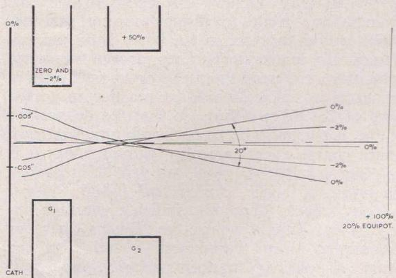
Fig. 9—Electron paths in cathode  $G_1$ - $G_2$  space, cathode test voltages.
