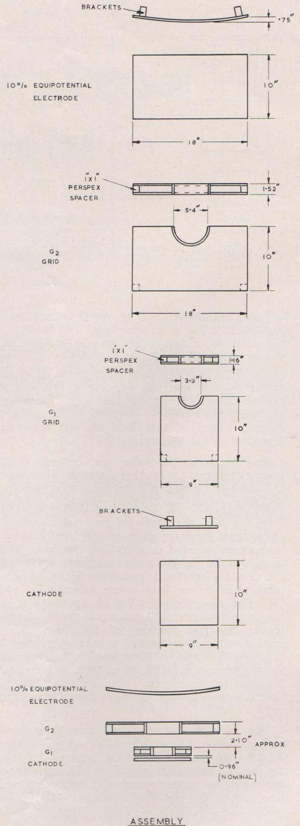
Fig. 4—150-times scale models, cathode  $G_1$ - $G_2$ -section.
