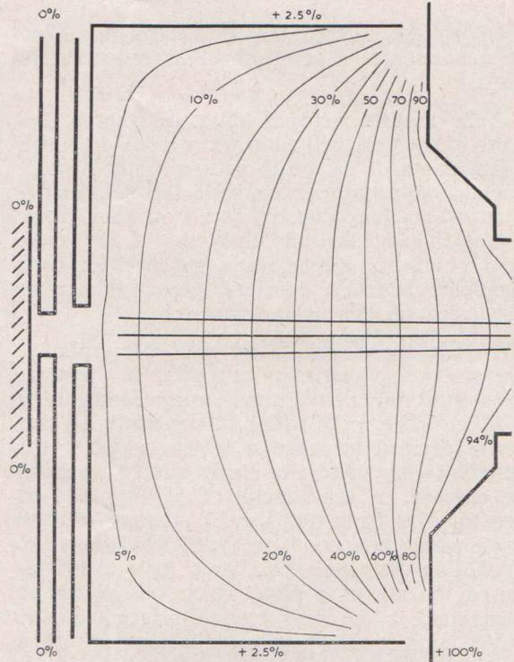
Fig. 5—Equipotentials in G<sub>2</sub>-G<sub>3</sub> space, normal voltages.
