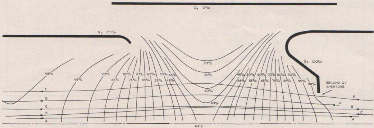
Fig. 12—Equipotentials and paths through final lens, normal voltages.
