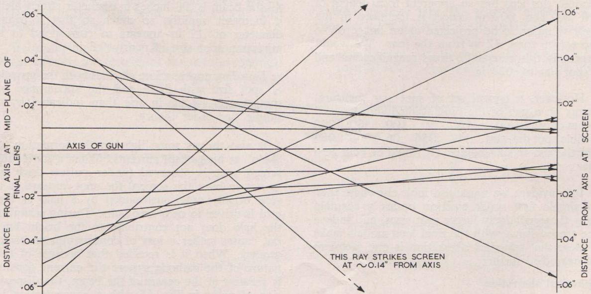
Fig. 15—Aberration of final lens (factor S-T = 80).
