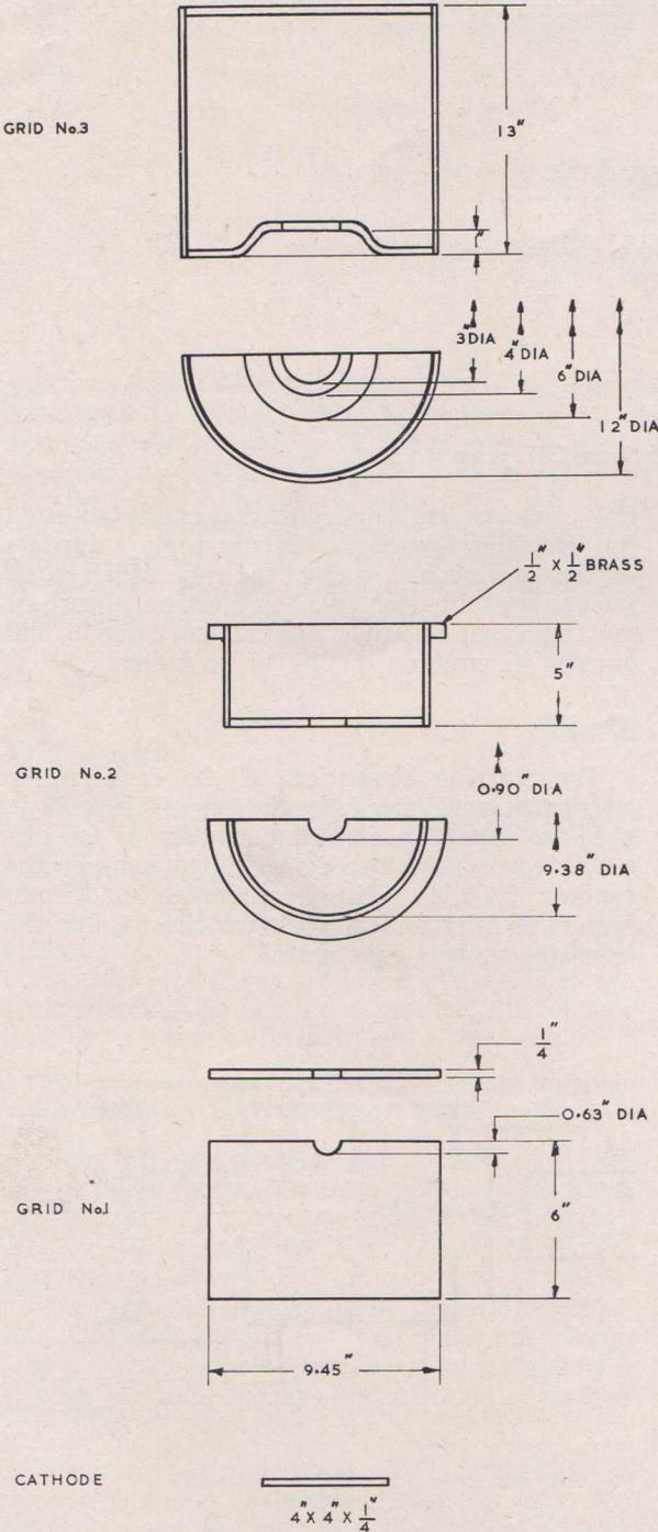
Fig 3—25-times scale model.
