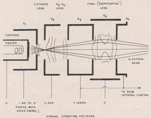
Fig. 2—Picture tube gun schematic.
