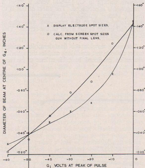
Fig. 11—Measurements of beam diameter, normal voltages.
