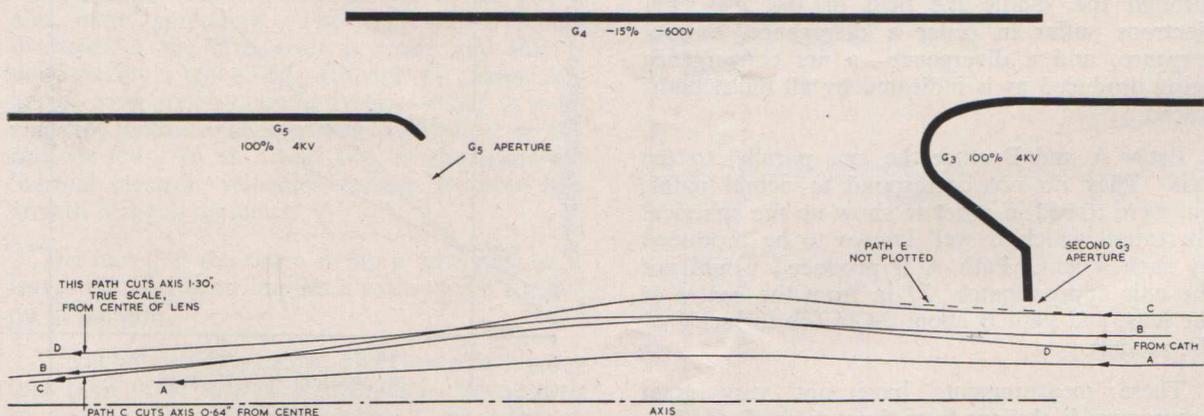
Fig. 13—Paths through final lens, cathode test voltages.
