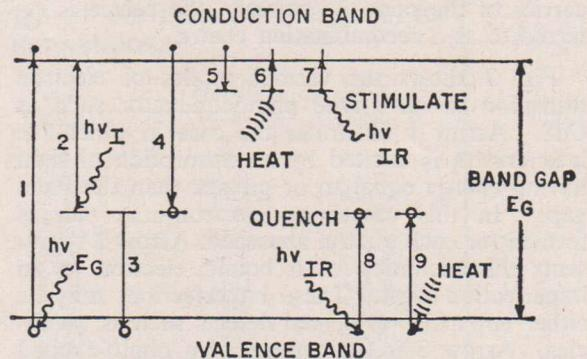
Fig. 7—Basic electronic processes in an n-type photoconductor such as CdS.
