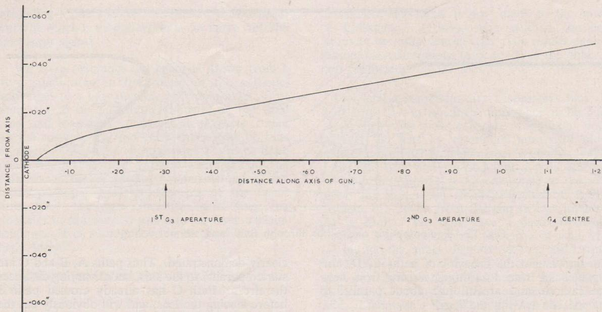
Fig. 10—Beam profile in 8235 gun, normal voltages, zero  $G_1$ .
