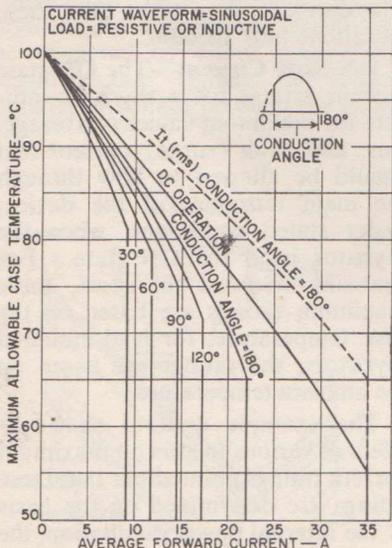
Figure 15. Current rating chart for the RCA-2N3873 SCR.
