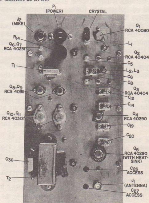
Figure 3: Top view of transmitter.
