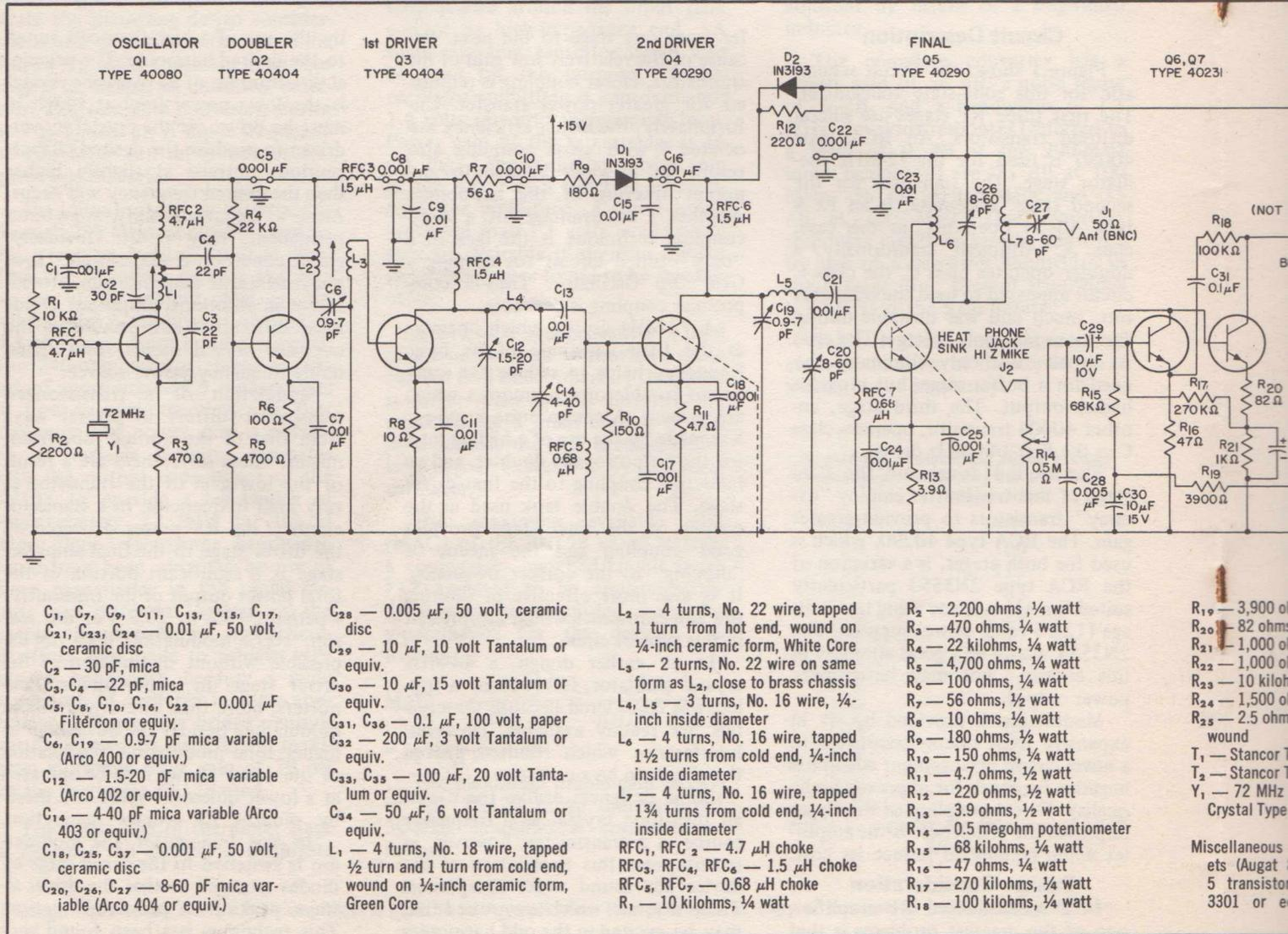
Figure 1: Schematic diagram and parts list of the WB2EG
