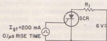
Figure 25. Test circuit used to determine turn-on time of thyristors.
