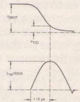
Figure 26. Initial ON-state voltage and current waveforms for the 2N3873 SCR.
