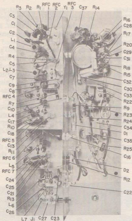
Figure 4: Bottom view of transmitter, showing RF section above and modulator section below.
