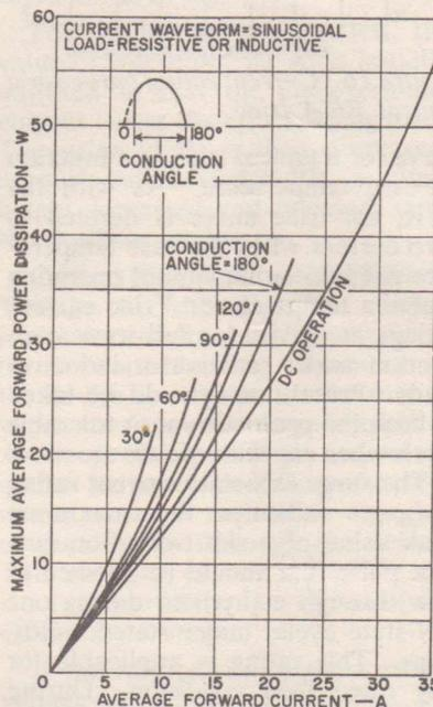
Figure 14. Power-dissipation rating chart for the RCA-2N3873 SCR.
