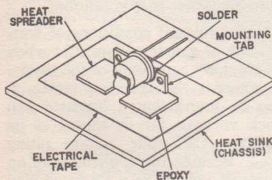
Figure 9. Typical heat-sink isolation technique for a chassis-mounted two-lead TO-5 thyristor.
