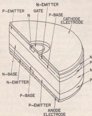
Figure 12. Cross-section of a typical triac pellet.
