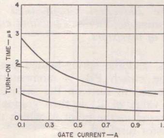
Figure 24. Turn-on time characteristics for the RCA-2N3873 SCR.
