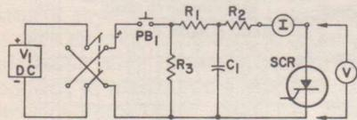
Figure 13. Test circuit used to determine dc forward- and reverse-voltage-blocking capabilities and leakage current of thyristors.
