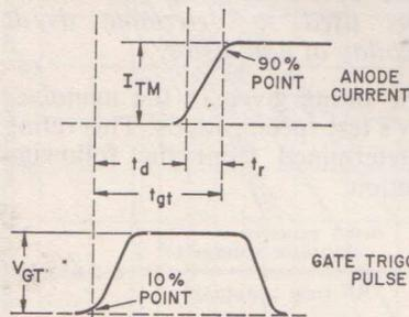
Figure 23. Gate current and voltage turn-on waveforms for a thyristor.
