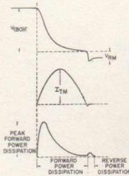
Figure 27. Instantaneous power dissipation in a thyristor during turn-on.
