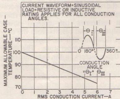
Figure 16. Current rating curve for a typical RCA triac.
