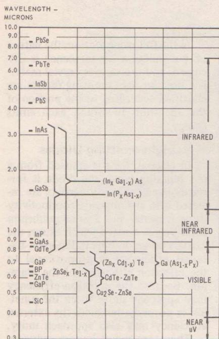
Fig. 1 - Various crystal materials and the portion of the spectrum in which they emit radiation.
