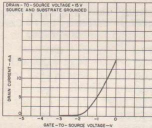
Fig. 1 - Drain current as a function of gate-to-source voltage for the 3N128 vhf MOS transistor.
