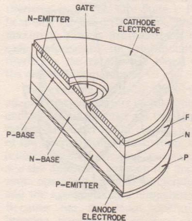
Figure 11. Cross-section of a typical SCR pellet.
