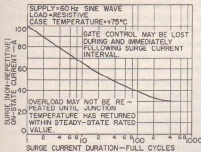
Figure 18. Surge-current rating chart for a typical triac.
