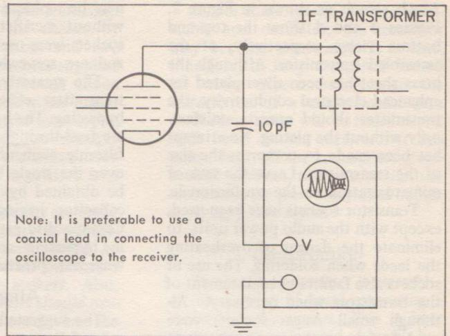
Figure 5: Schematic diagram showing method used by WB2EGZ to connect the signal from the transmitter to an oscilloscope.
