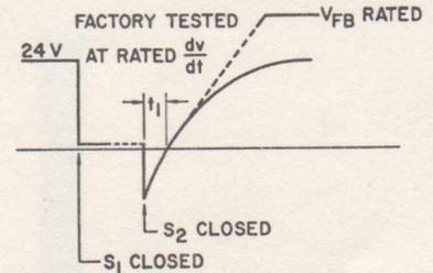
Figure 29. Test circuit and voltage waveforms used to determine turn-off times of thyristors.
