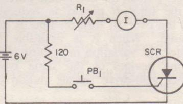
Figure 20. Test circuit used to determine holding and latching currents of thyristors.
