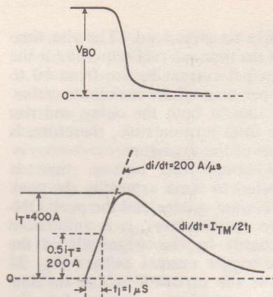
Figure 19. Voltage and current waveforms used to determine  $di/dt$  rating of the RCA-2N3873 SCR.
