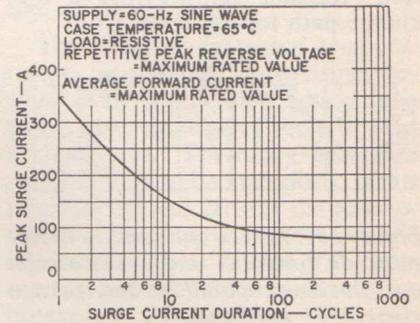
Figure 17. Surge-current rating curve for the RCA-2N3873 SCR.
