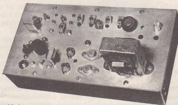
Figure 2: Assembled transmitter, showing RF section at upper left and modulator section at lower right.
