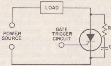
Figure 22. Diagram showing use of RC network to improve the  $dv/dt$  capability of an SCR.
