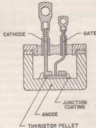
Figure 10. Cross-section of RCA press-fit thyristor package.
