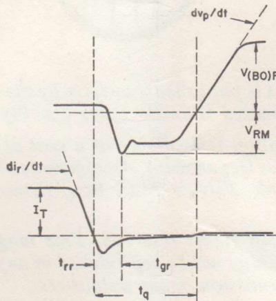
Figure 28. Circuit-commutated turn-off voltage and current waveforms for a thyristor.
