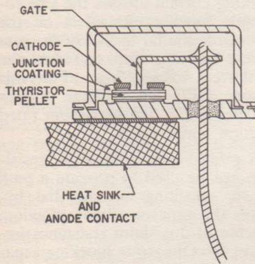
Figure 8. Cross-section of RCA two-lead TO-5 thyristor package.
