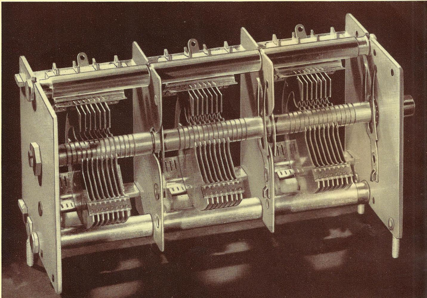
**The Laboratory Type Variable Tuning Condenser, Showing the Isolantite Insulators, Heavy Plates and Wide Spacing to Eliminate Microphonics (Full Size)**
