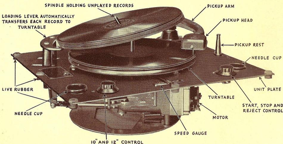
reproduction. On the other hand, a much heavier pickup causes the needle to bear down on the record with too much force, and if undue wear on record grooves is to be avoided, the needle must be replaced after playing only 2 or 3 sides. The Scott pickup weighs just 3½ ounces and this comparatively light weight not only reduces surface noise and record wear to a minimum, but also enables you to play the entire capacity of the changer without once changing the needle.
