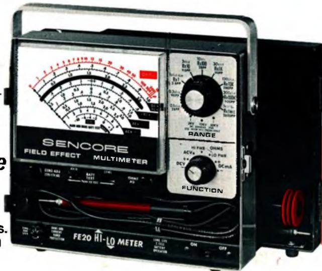
Uses low voltage on ohmmeter (on low PWR position) to measure in-circuit resistances:
