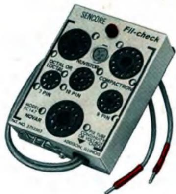
Check continuity of all tube filaments including the new Compactrons, Novars, 10-pins, Nuvisitors and the new Decals. Test leads for CRT filament checking. Also, doubles as neon voltage indicator. TV cheater cord is used to power unit as a check on the cord to insure 115 volts AC on TV.
