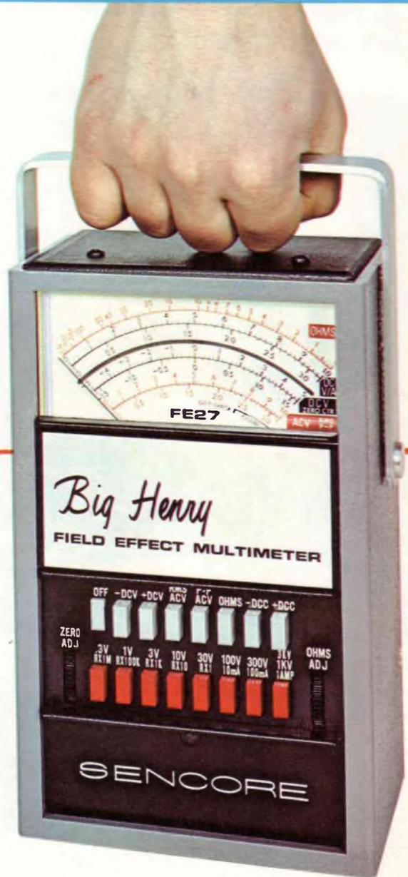
**DC Volts:** 0-0.3, 1, 3, 10, 30, 100, 300 1KV, 3KV, full scale, positive and negative. Zero center ranges: All positive and negative, 0.15, 0.5, 1.5, 5, 15, 50, 150, 500, 1.5KV. Input resistance: 15 megohms shunted by 58 pf. Accuracy: 1.5%. AC rejection: 30DB minimum.
