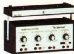
**Resistors:** 24 overlapping values from 10 ohms to 5.6 megohms. 1 watt up to 10K, 1/2 watt over 10K.
