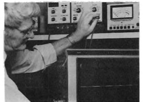
Fig. 9: Injecting the VA62 horizontal keying pulse into the Sandcastle test point unblanks the CRT to show the true symptom. In this case, the single horizontal line tells us we have a vertical problem.
