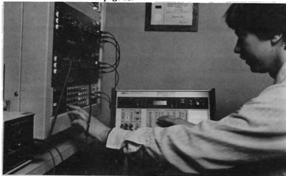
Fig. 4: Each secondary standard used at Sencore is regularly checked against our prime standards.
