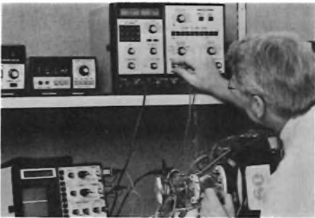
Fig. 10: The patented Sencore Ringing test accurately tests the deflection yoke to complete the tests of the vertical circuits.
