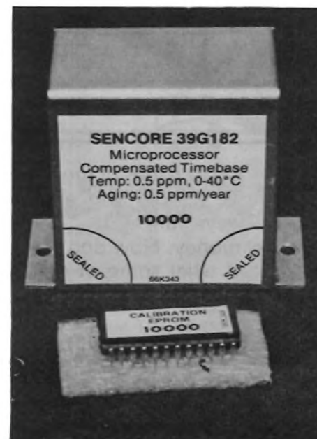
Fig. 6: To recalibrate the FC71 you simply exchange the old timebase and memory chip with a new, freshly calibrated set.
