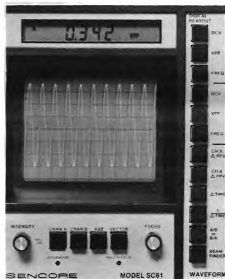
Fig. 2: The SC61's digital readout provides you with all the waveform's essential parameters with just a push of a button.
