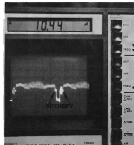
The Delta Time function of the SC61 quickly tells you if the width of the horizontal blanking interval is correct.
