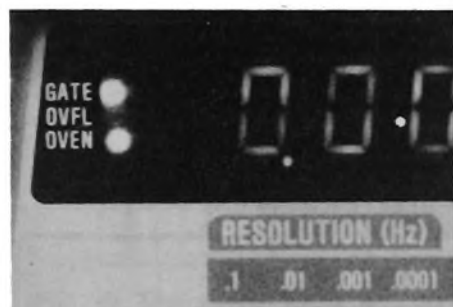
Fig. 4: Oven compensated timebases draw power continuously to keep the crystal at a constant temperature.
