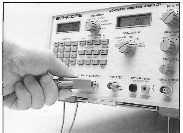
Fig. 10: Plug one end of the connector into the end of the computer monitor's cable and the other end into the CM2000's SYNC & VIDEO OUTPUT jack.
