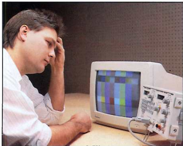
Fig. 2: The first step in servicing computer monitors is trying to recreate the customer's complaint. This will help you assess the nature of the problem.
