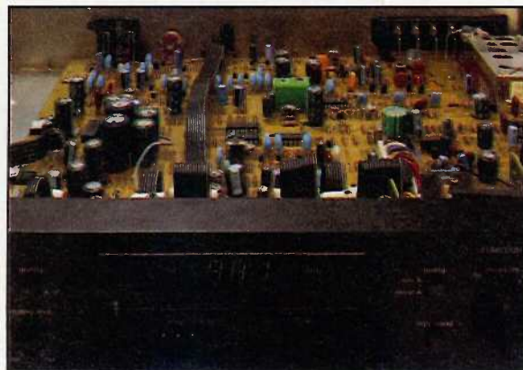
Fig. 2: Capacitors and inductors are abundant in modern circuits because they cannot be contained in ICs.
