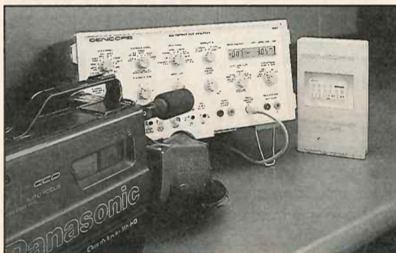
Fig. 3: The Servo Performance Test Lead and VC93 let you test the camcorder servos without even opening the camcorder.
