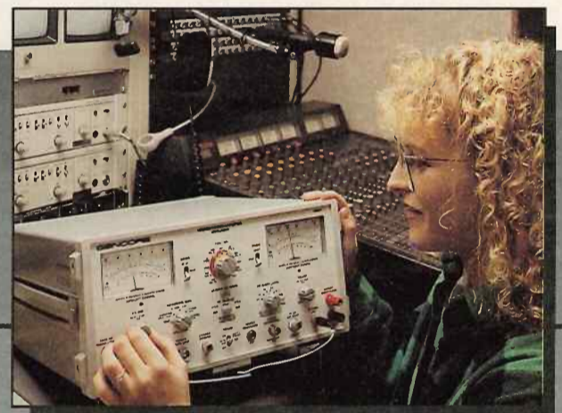
Fig. 2: Performance testing the TV tuning system with the VG91 gives you a clear understanding of the symptoms and helps isolate the problem.
