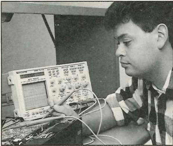
Fig. 6: Set the SC3100 TRIGGER MODE switch to "AUTO" so you always see a trace on the CRT – even when the trigger circuits aren't locked.
