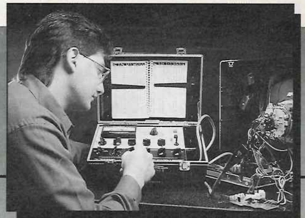
Fig 4: The CM2000 lets you test computer monitor high voltage regulation by simply changing the polarity of the Raster pattern.
