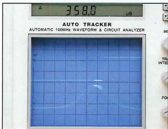
Fig. 8: The SC3100's Delta Bar quickly measures the Tracking Fix adjustment time delay between the two signals.
