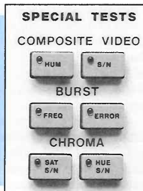
Fig. 5: The six special tests complement waveform and vector measurements to provide efficient video camera service.
