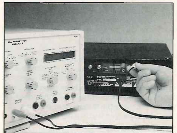
Fig. 2: The VC93 All Format VCR Analyzer lets you analyze VCR servo operation without taking the cover off the VCR.
