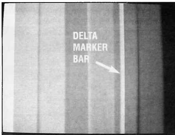
Fig. 10: The CVA94 provides a video monitor Delta Bar Marker synchronized with the CRT Delta Bar to make signal measurement selections quick and easy.
