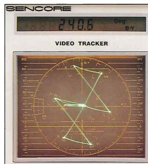
Fig. 2: The CVA94 "Video Tracker's" direct digital readout simplifies chroma measurements for easier and faster camera servicing.
