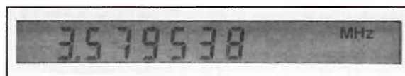
Fig. 7: The Burst Freq and Burst Error tests allow you to quickly check a camera's reference oscillator without opening the camera.
