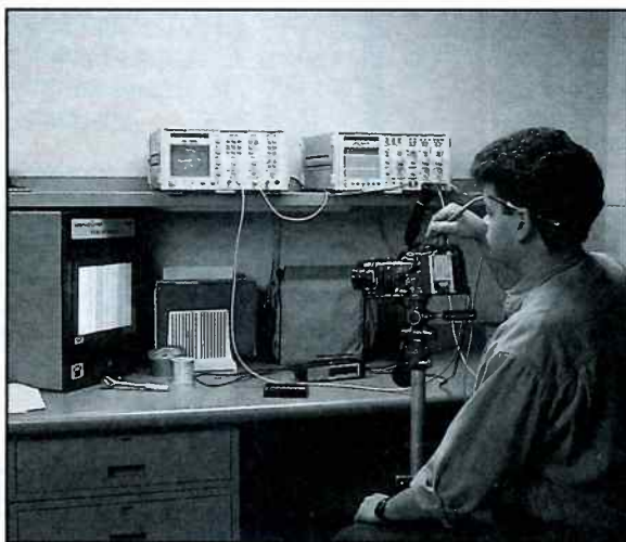
Fig. 9: You can trigger your scope (SC3100 "AUTO TRACKER") to the CVA94 so all waveforms are precisely triggered, no matter where you trace a signal.
