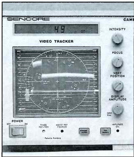
Fig. 3: The special video S/N test easily identifies noisy camera video signal sources with an automatic, digital readout of the results.
