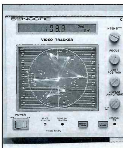
Fig. 5: Use the "Video Tracker" to measure a camera's chroma phase. A good camera's red signal output should be within 15^\circ of 103^\circ .
