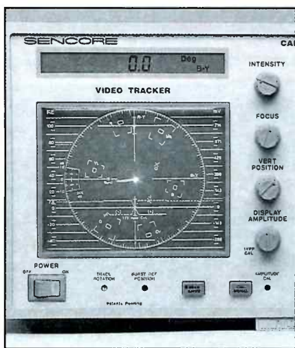
Fig. 4: The "Video Tracker" shows only the burst reference vector extending to the left of center indicating good white balance with the camera focused on a non-colored pattern.
