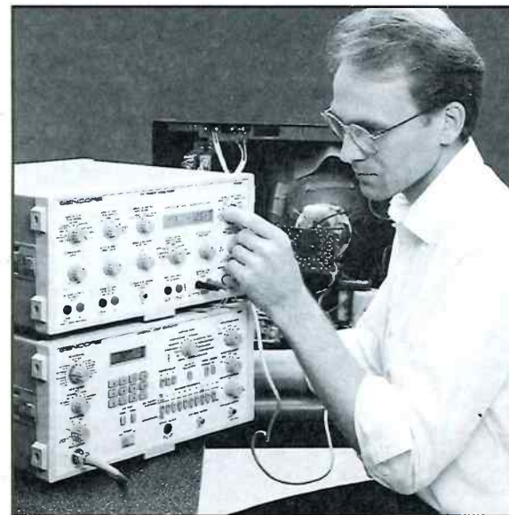
Fig. 4: The VG91 Universal Video Generator and TVA92 TV Video Analyzer give you all the signals you need to troubleshoot video circuits with the time proven divide-and-conquer technique.
