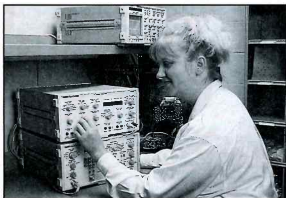
Fig. 7: Troubleshooting with the VG91 and TVA92 is like having a miniature TV station with all the signals required to substitute into any TV stage.
