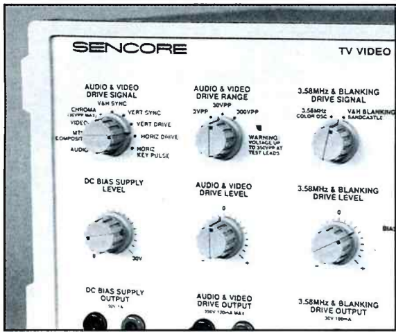
Fig. 5: The TVA92 TV Video Analyzer drive signal levels and polarities are adjustable so you can adjust to any circuit.
