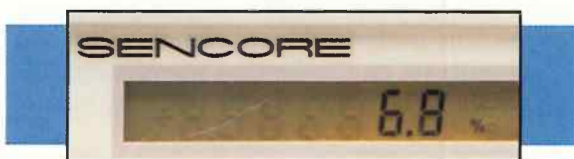
Fig. 4: The special Hum test quickly identifies low frequency ripple problems.
