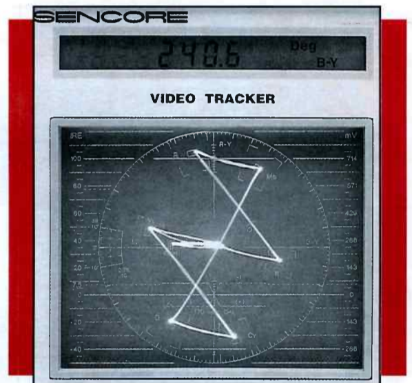
Fig. 1: The CVA94 "Video Tracker's" direct digital readout simplifies chroma measurements for easier and faster camera servicing.
