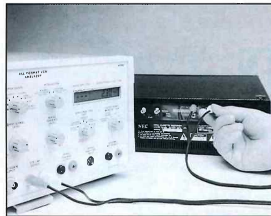
Fig. 5: Standard and troubleshooting signals from the VC93 All Format VCR Analyzer help you narrow down VCR defects in the least amount of steps possible.
