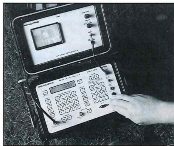
Fig. 4: The battery operated, portable SL750A lets you analyze signals anywhere your testing takes you.
