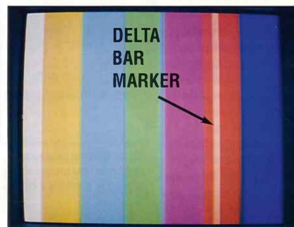
Fig. 7: The CVA94 provides a video monitor Delta Bar Marker synchronized with the CRT Delta Bar to make signal measurement selections quick and easy.
