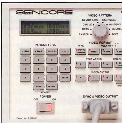
Fig. 2: The sync and pixel rates are programmable to match the monitor's input requirements.
