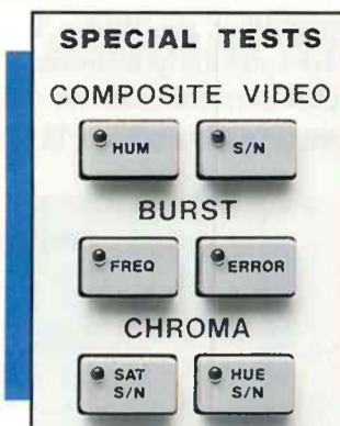
Fig. 3: The six special tests complement waveform and vector measurements to provide efficient video camera service.
