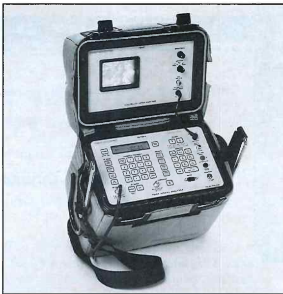
Fig. 3: The SL750A's exclusive color LCD display lets you look at the signal to confirm good picture quality to you and your customer. (photo shown is black & white)
