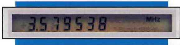
Fig. 5: The Burst Freq and Burst Error tests allow you to quickly check a camera's reference oscillator without opening the camera.
