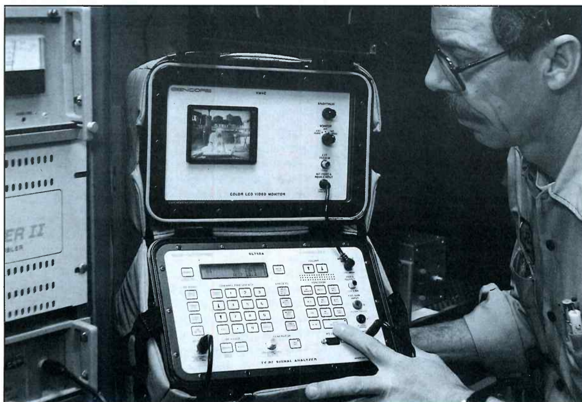
Fig. 2: The SL750A "CHANNELIZER" TV-RF Signal Analyzer helps you quickly pinpoint RF/video problems in any RF distribution system.
