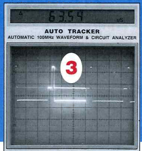
Fig. 2: The "AUTO TRACKER" provides three different ways to test a signal: 1) Autotracking digital readouts, 2) the CRT, and 3) the Delta digital tests.
