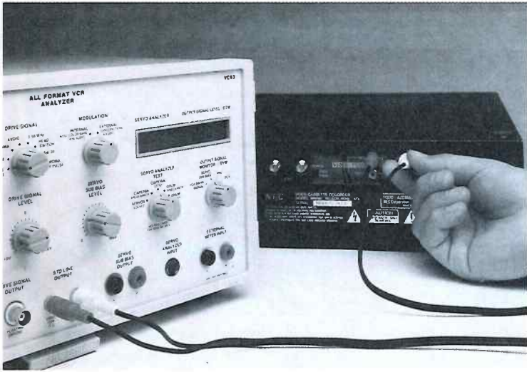
Fig 5: Chris uses his VC93 to performance test every VCR that crosses his bench.
