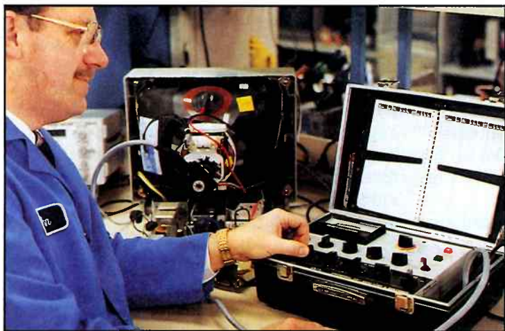
Fig 6: The CR70 "BEAM BUILDER" has increased the CRT rejuvenation yield at Nulogix from 50% to approximately 80%.
