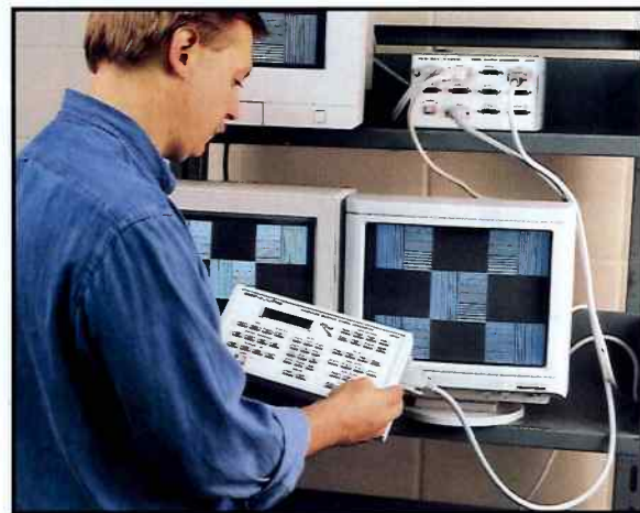
Fig. 3: Use the CM125 on your burn-in rack or monitor display to thoroughly test monitors without phosphor burn.
