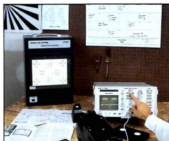
Fig. 4: Use the VR940's Registration/Response Chart to check and adjust a camera's registration and frequency response.
