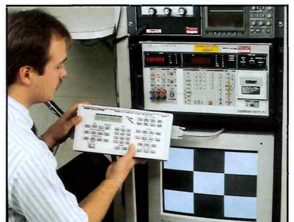
Fig. 2: Use the new CM125 "Pix Pak" for testing and aligning computer monitors in the field.
