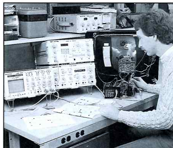
Fig. 5: You can measure if the timing in the horizontal output stage is causing shutdown with the TVA92 TV Video Analyzer's Horiz Output Load tests.
