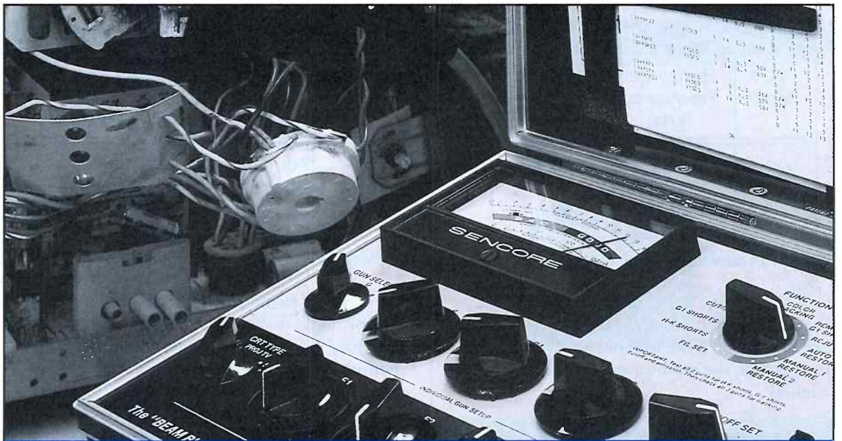
Fig. 1: Use the CM125 "Pix Pak" to perform a final quality test before you send the computer monitor back to the customer.
