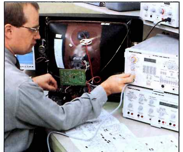
Fig. 4: Testing and aligning the AFT circuit using the VG91 Universal Video Generator is a critical part of troubleshooting a tuning problem.
