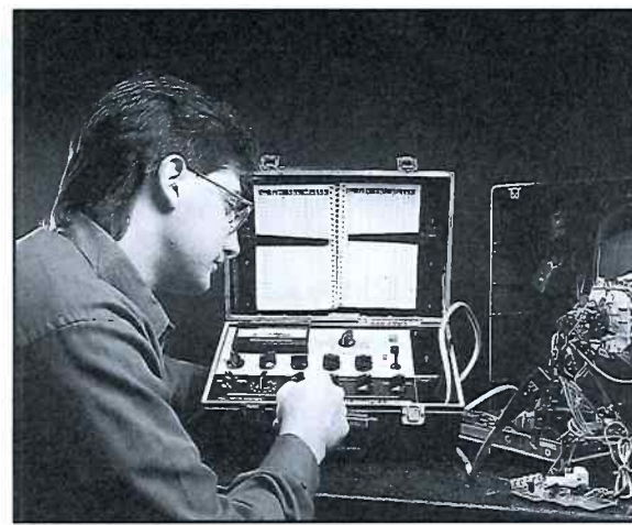
Fig. 3: Restoring a CRT with one of the five levels of the CR70's Progressive Restoration lets your customer keep an older set running, while generating value added billing for you.
