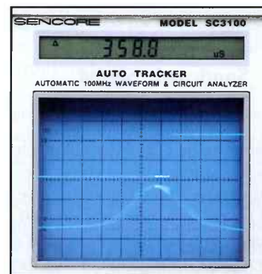
Fig. 7: The SC3100's Delta Bar quickly measures the Tracking Fix adjustment time delay between the two signals.
