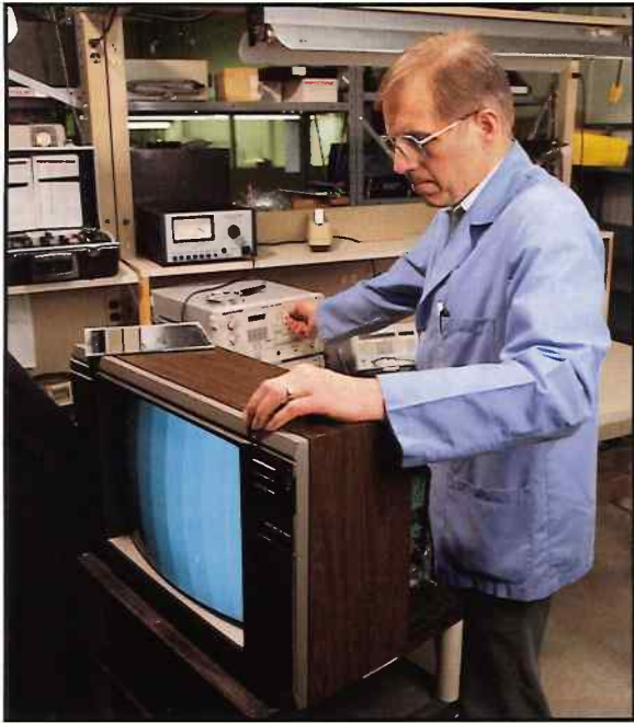
Fig. 4: The VG91's 10 Bar Staircase pattern lets you set CRT controls without jumper wires or setup switches.
