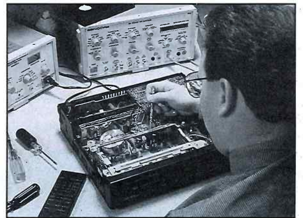
Fig. 1: A quick visual inspection of the VCR can locate many common problems including worn belts, idlers, etc.
