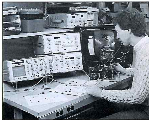
Fig. 2: The TVA92 detects high current loading and shorted conditions in the horizontal output circuit without even turning on the TV.
