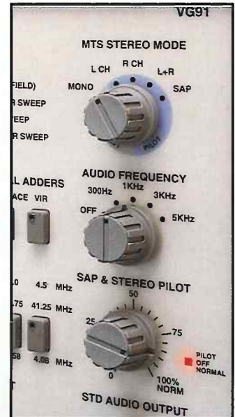
Fig. 5: Use the Mono/MTS Stereo/SAP generator of the VG91 to test tuner, IF and audio circuits of a TV-video system.
