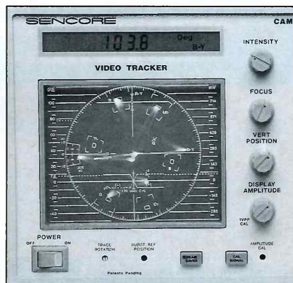
Fig. 4: Use the "Video Tracker" to measure a camera's chroma phase. A good camera's red signal output should be within 15° of 103°.
