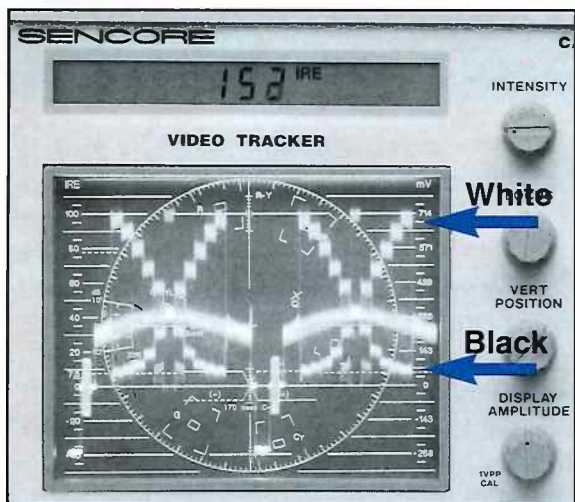
Fig. 2: The CVA94 shows the resultant video waveform of the VR940's Gray Scale Chart testing a camera's luminance levels to see if they are adjusted properly.
