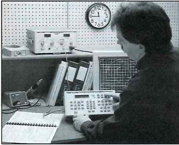
Fig. 1: Use the CM125's CIRCLE/CROSS pattern for testing a computer monitor's display centering and linearity.
