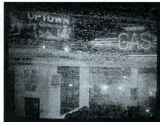
Fig 1: A noisy playback picture can mean a problem in the video head circuitry, servos, and even tape path alignment. With the right test equipment you can isolate these tough dog problems quickly.
