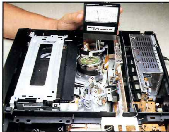
Fig. 5: Be sure to check the alignment of the entire tape path, including the tape tension.
