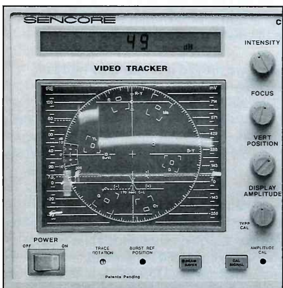
Fig. 3: The special video S/N test easily identifies noisy camera video signal sources with an automatic, digital readout of the results.
