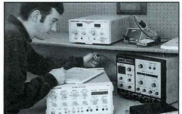
Fig. 3: The VC93 can be connected directly to the VA62 or VA62A for enhanced troubleshooting capabilities.
