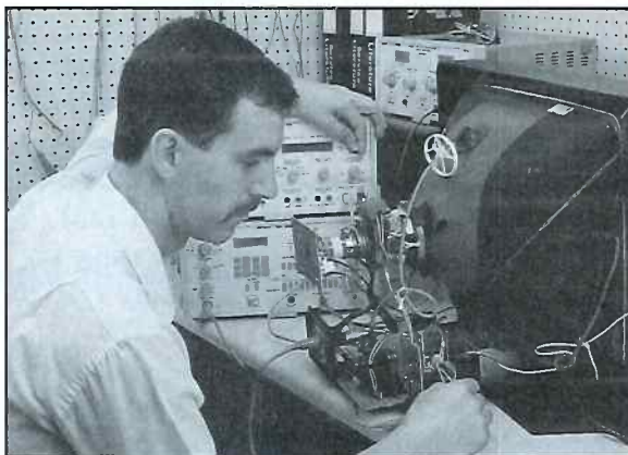
Fig. 4: Horizontal output transistors often fail from surrounding circuit defects. The TVA92's Dynamic Tests and Horizontal Output Device Sub & Drive help you isolate these problems.
