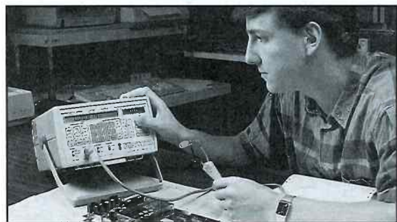
Fig. 5: The LC102 "AUTO-Z" tests for all capacitor failures and automatically tells you if the capacitor is "GOOD" or "BAD."
