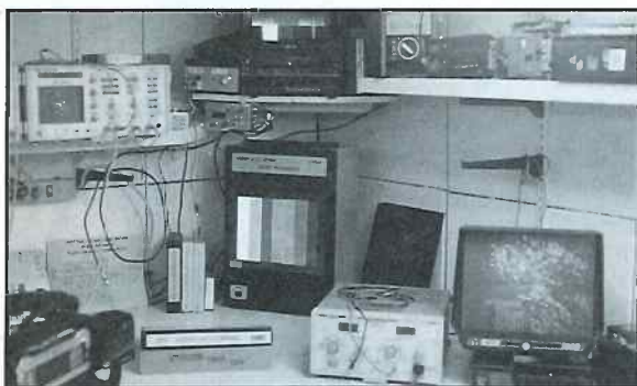
Fig. 2: JOB ELECTRONICS specializes in camcorder repair with the Sencore CVA94 "Video Tracker" and VR940 Video Reference.
