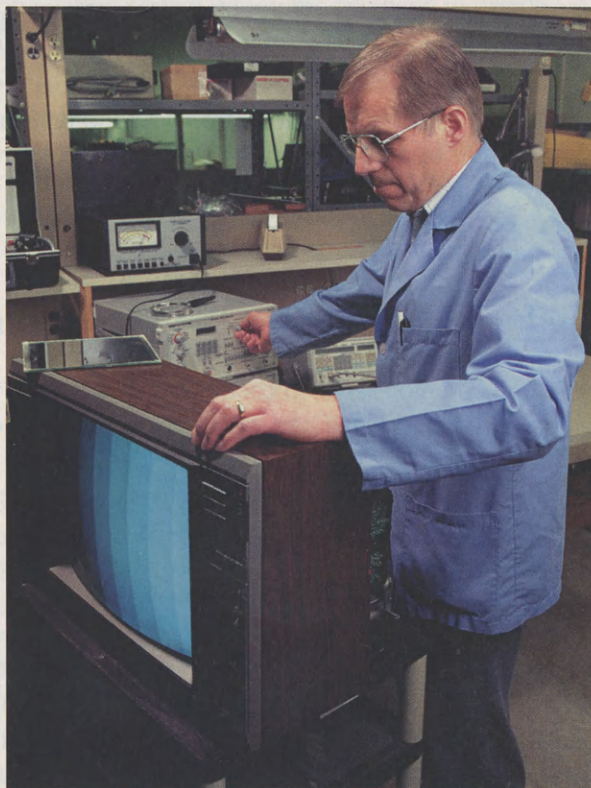
Fig. 6: After the repairs have been made, be sure to run a complete performance test again to make sure you don't miss any problems.
