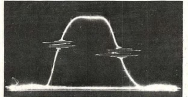
Horizontal markers aid in accurate positioning of carrier markers.
