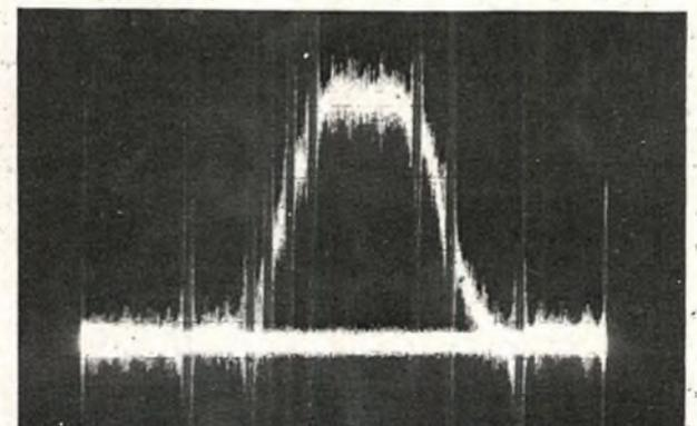
Excessive marker height causes noise on curve and difficulty in accurately locating markers.
