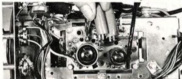
Antenna terminals make fast, easy connection for RF response checks.
