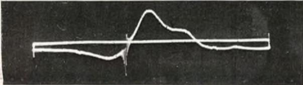
Pre-injection markers can cause severe overloading and curve distortion.
