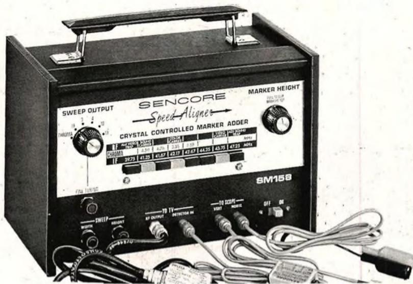
Sencore all solid-state sweep marker generators are constructed to provide the necessary signals for sweep alignment and troubleshooting. The SM158 and SM152 have these common specifications:
