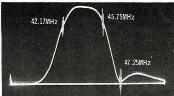
Typical link response curve after link adjustment.
