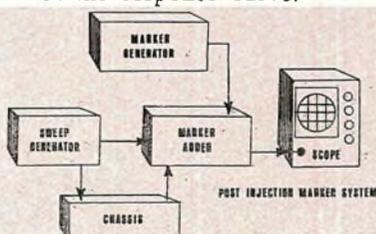
The post-injection marker system allows you to use more markers than with the preinjection system, have more marker amplitude without interfering with the response curve, and eliminates the problem of interference.
