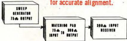
A good test of the impedance match of a sweep generator is to connect it to the receiver and then "milk" or "wipe" the cable from the generator to the receiver with your hand. Any body capacity effects that alter the shape of the curve, indicate standing waves on the line. Put the Sencore sweep generators to this test and they will stand out from all others on the market as the quietest. The use of shielded and low impedance cables on sweep generators is also part
