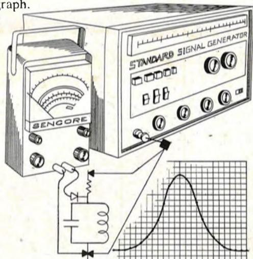
Response check of simple tuned circuit and response curve obtained.
