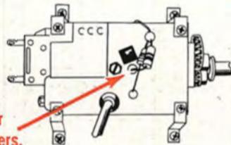
Mixer test point located near square opening on most tuners.
