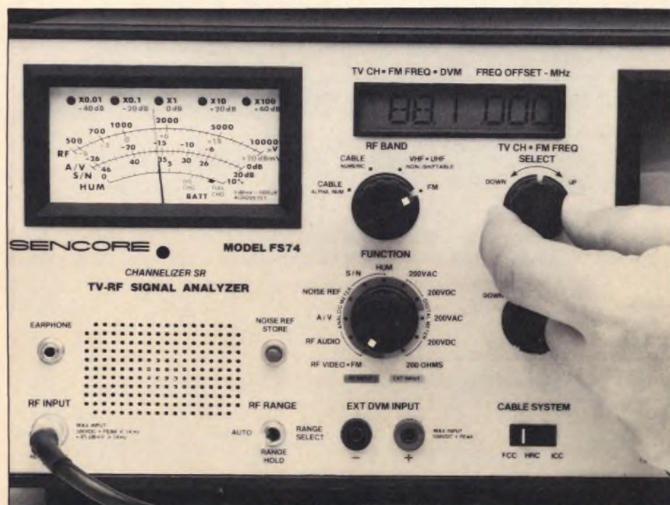
Fig. 1: The frequency coverage of the FS74 "CHANNELIZER" (5 MHz to 890 MHz) makes it ideal for tracing interference. Here, an FM station at 88.1 MHz is monitored to confirm a severe cable ingress problem.
