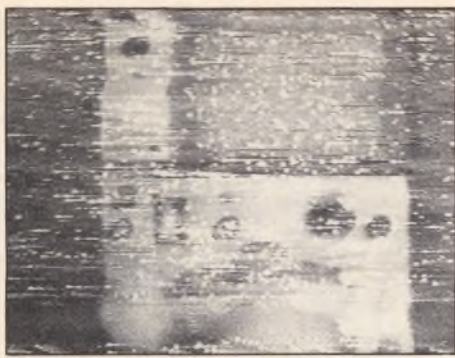
Fig. 3: Servo problems cause the picture to randomly tear. Use the audio to determine whether the problem is in the capstan or cylinder servo section.
