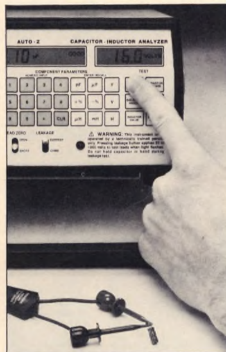
Figure 2. Press the LC77's touch sensitive keypad to select automatic capacitor-inductor tests.
