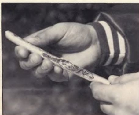
Fig. 3: Problems that are particularly hard to find in large systems may be caused by worn and frayed cable cr as in this case, damage caused by squirrels.
