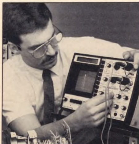
Fig. 2. When troubleshooting most TV's, you'll increase your chance of success by monitoring the horizontal output transistor (HOT) waveform with the SC61 Waveform Analyzer.
