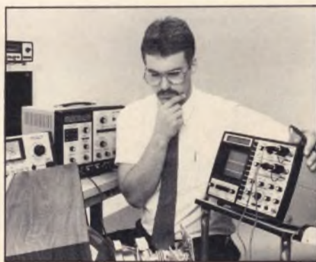
Fig. 1. Troubleshooting a TV set without a schematic requires a new approach. Find the easiest test points and use the VA62's preset drive ranges: 3 VPP for ICs and 30 VPP for transistors.
