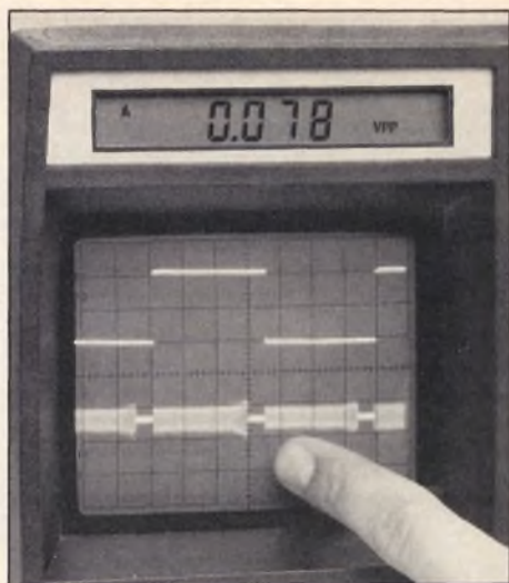
Fig. 12: Aligning the servos properly prevents audio information drop off, as the head switches to the next channel.
