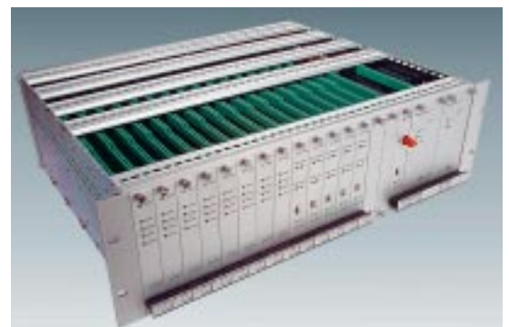
Fig. 7: D19m chassis with power supply
