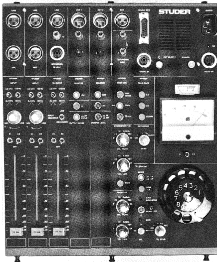
Studer 069, reporting unit for radio transmissions «in the field» via land line.
