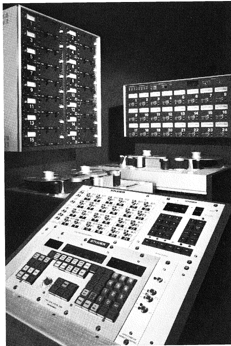
Studer remote control systems for modern tape recorders: TLS 2000 tape-lock system for electronic synchronisation and electronic editing, remote audio-channel control and auto-locator with 20 stored tape addresses.
